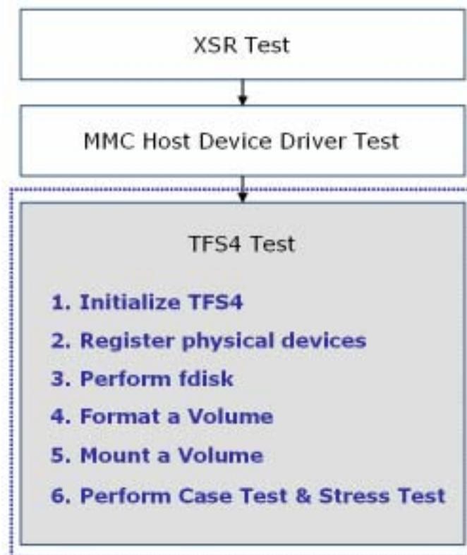
**Figure 5-2. TFS4 Test Sequence**
