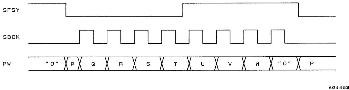
SBSY is output for each subcode block. It is high during the S0 and S1 synchronization cycles. Its falling edge indicates the end of synchronization and the start of EIAJ-format data within the subcode block.
