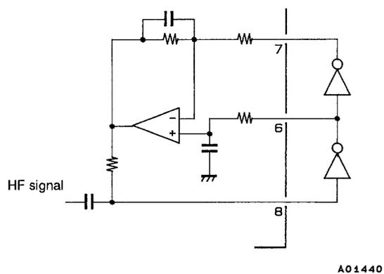
**PLL Clock Regeneration Circuit (pin 4: PDO, pin 3: AI, and pin 2: AO)**
