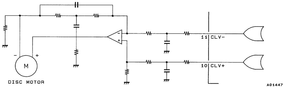
Note: \* For constant linear velocity servo control commands, the TOFF pin is low only in the CLV mode; otherwise it is high. Control of the TOFF pin by command is effective only in the CLV mode.
