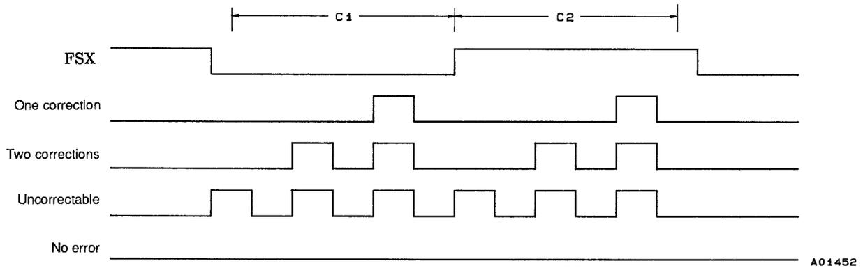
The 7.35 kHz FSX frame synchronization signal is divided down from the reference clock. The status of error correction in each frame is output on EFLG, as shown in the figure, where the number of high pulses in each FSX period indicates the quality of the replay signal.
