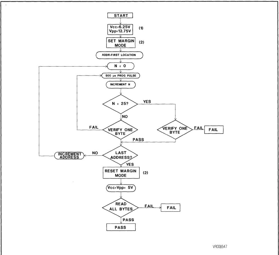
NOTES : 1.  $V_{CC}$  must be maintained at 6V during the whole programming algorithm between set and reset MARGIN MODE operation. A drop of  $V_{CC}$  below 4V could reset the internal MARGIN MODE flip-flop giving place to insufficient programming margins.
