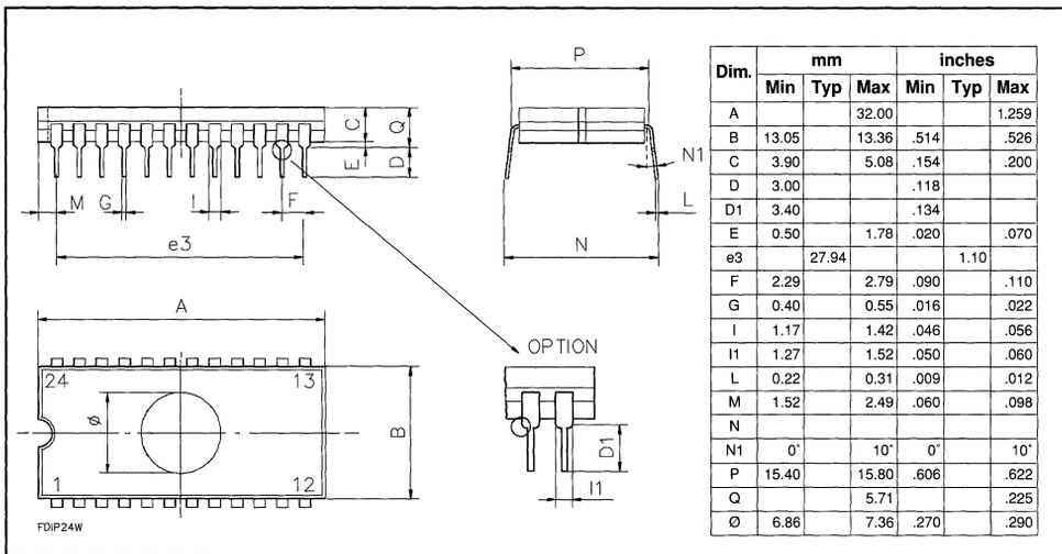
**Figure 7 : 24-PIN CERAMIC DIP BULL'S EYE - SKINNY - 300 MILS**
