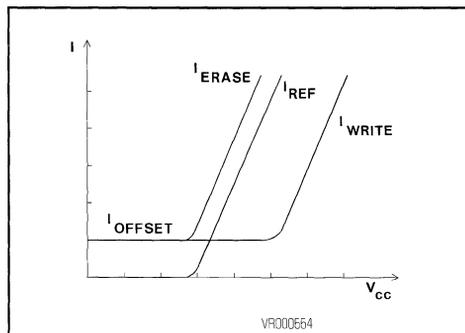
The final result is that a threshold shift of about 1V for a written cell is enough to allow proper sensing in a very wide  $V_{CC}$  operating range (figure 6).
