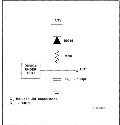
A.C. Testing : Inputs are driven at  $V_{OH}$  for a logic "1" and  $V_{OL}$  for a logic "0". Testing measurements are made at  $V_{IH}$  for a logic "1" and  $V_{IL}$  for a logic "0". Rise/Fall time  $\leq 10$  ns.
