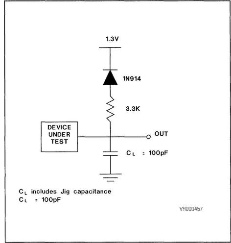
A.C. Testing : Inputs are driven at V<sub>OH</sub> for a logic "1" and V<sub>OL</sub> for a logic "0". Testing measurements are made at V<sub>IH</sub> for a logic "1" and V<sub>IL</sub> for a logic "0". Rise/Fall time ≤ 10 ns.
