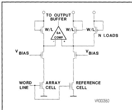
If the addressed cell is erased its current is the same as the reference cell's current and the unbalance at the inputs of the comparator (higher voltage on right side = 1) is obtained by connecting lower impedance load on the right side than on the left.
