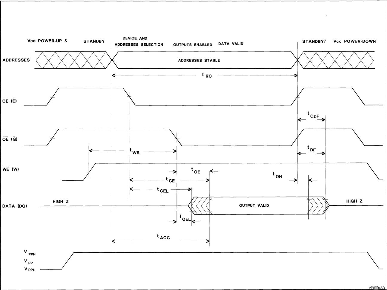
Figure 7 : A.C. Waveforms for Read Operations
