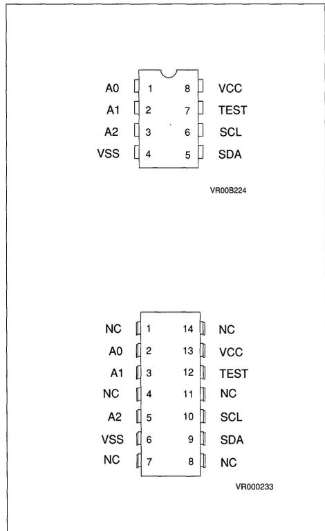
The 4K bits memory capacity is divided in two pages of 256 words of 8 bits. All memory operations are synchronized on an external strobe: SCL bus. The Read and Write operations are initiated by a Start instruction sent on the SDA bus by the master device.
