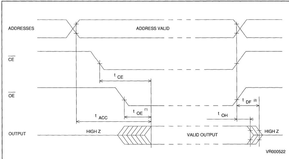
NOTES : 1.  $\overline{OE}$  may be delayed up to  $t_{ACC} - t_{OE}$  after the falling edge  $\overline{CE}$  without impact on  $t_{ACC}$ .
