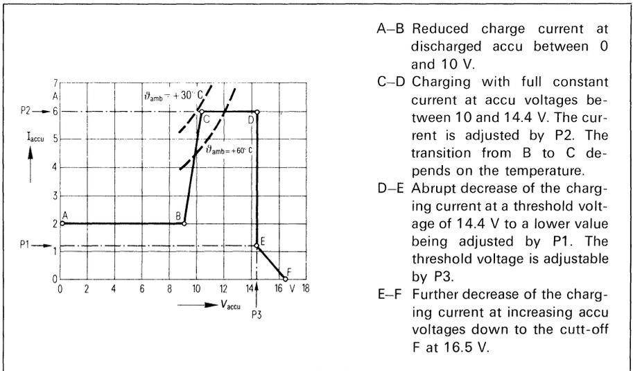
A-B Reduced charge current at discharged accu between 0 and 10 V.
