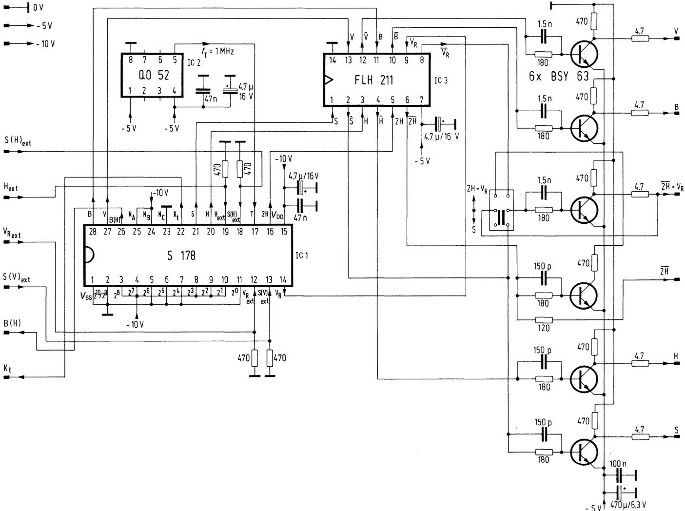
All important pulses are generated either as pulse composition (synchronous pulse composition S, blanking pulse composition B) or as separate pulses ( $V$ ,  $H$ ,  $\overline{2H}$ ,  $2H+V_R$ ). They are available at transistor output stages driven by the TTL-IC FLH211. Besides that the horizontal blanking pulses B ( $H$ ) and the clamping pulses  $K_t$  are generated. The fan out for the output stage of these two pulses is one TTL-input each.
