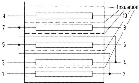
Winding schematic for transformer Tr 3
