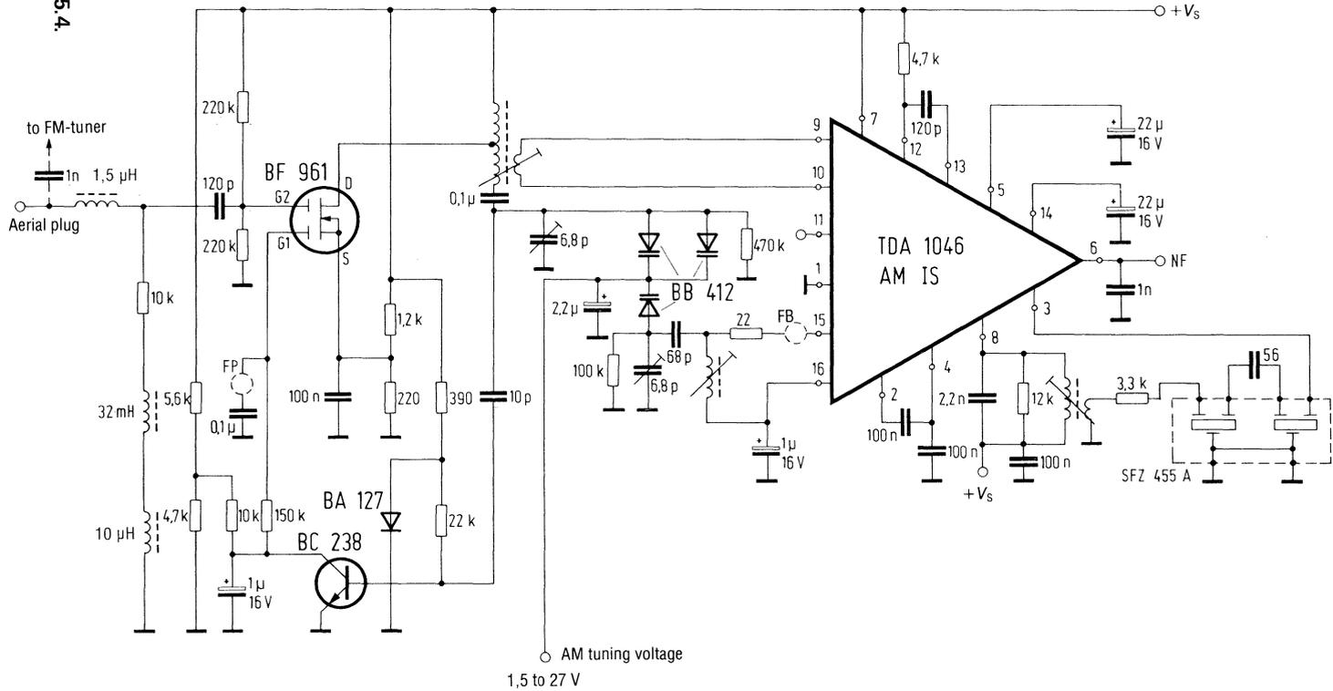
signal level at the capacitance diode of the oscillator circuit is kept constant to a value of approx.  $800 \text{ mV}_{pp}$  by means of the internally controlled oscillator.
