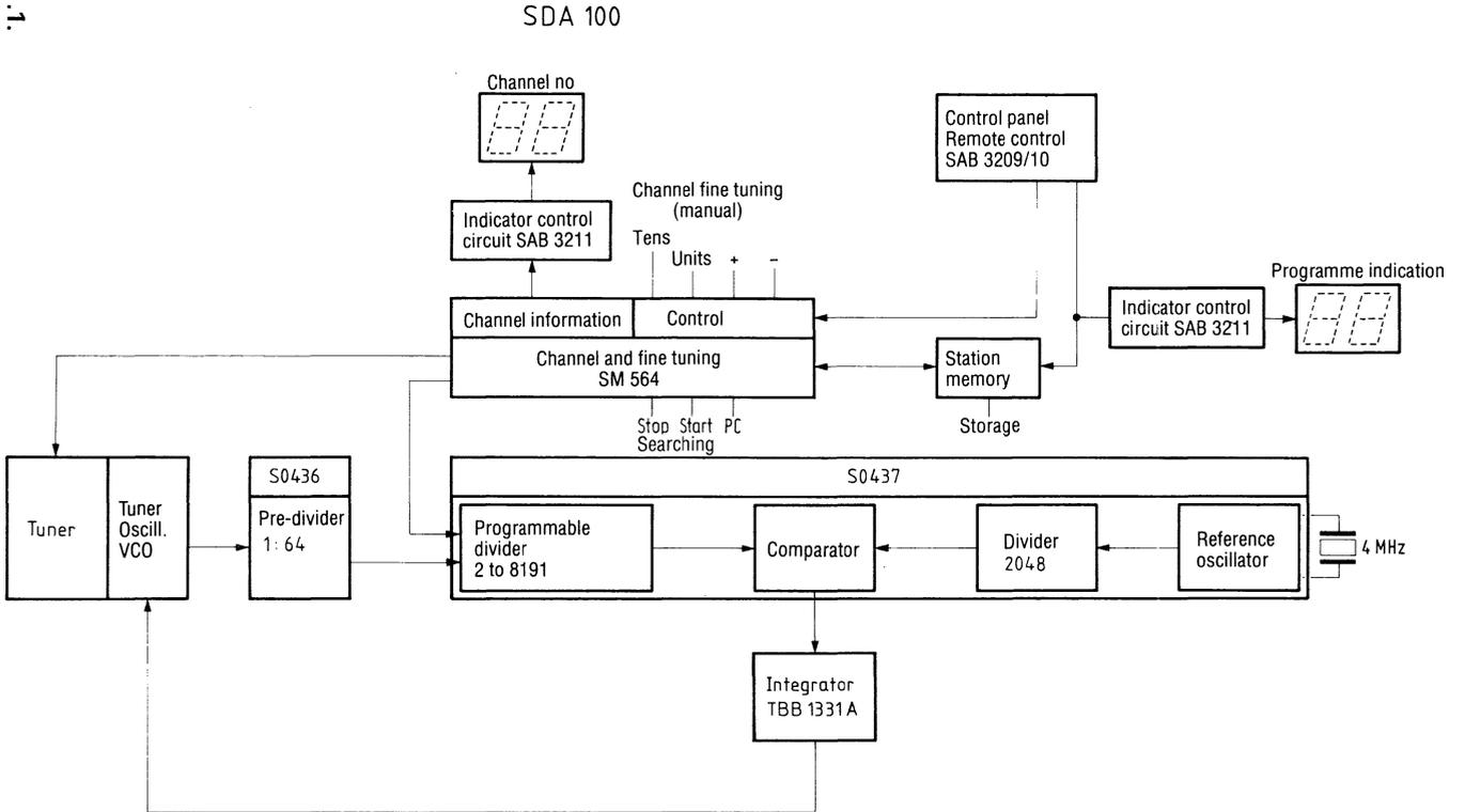
It is electrically programmable and converts the tuning information to a frequency information which determines the dividing factor of the PLL-divider and which is serially transferred to the PLL-circuit. The total channel numbers are stored in the station memory, i.e., each address of the memory corresponds to a TV station.
