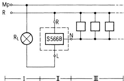
**Fig. 6.1.2.** Arrangement of parallel-connected control devices
