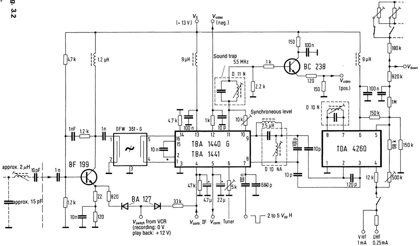
TBA1440 to a gain minimum by an impressed IF control-voltage of approx. 3 V. Because of the internal control amplifier the tuner is also downward-controlled.
