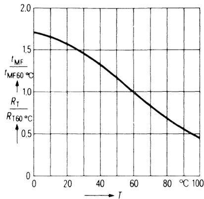
This analog value cannot be directly applied to the microcomputer. The thermistor resistance has to be converted in a proportional time period. This can be achieved by the cheap timer-IC TDB 0555 B. Then, in turn, the time is converted in a binary number by the microcomputer.
