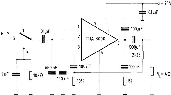
Switch S in position 2 for noise measurement.
