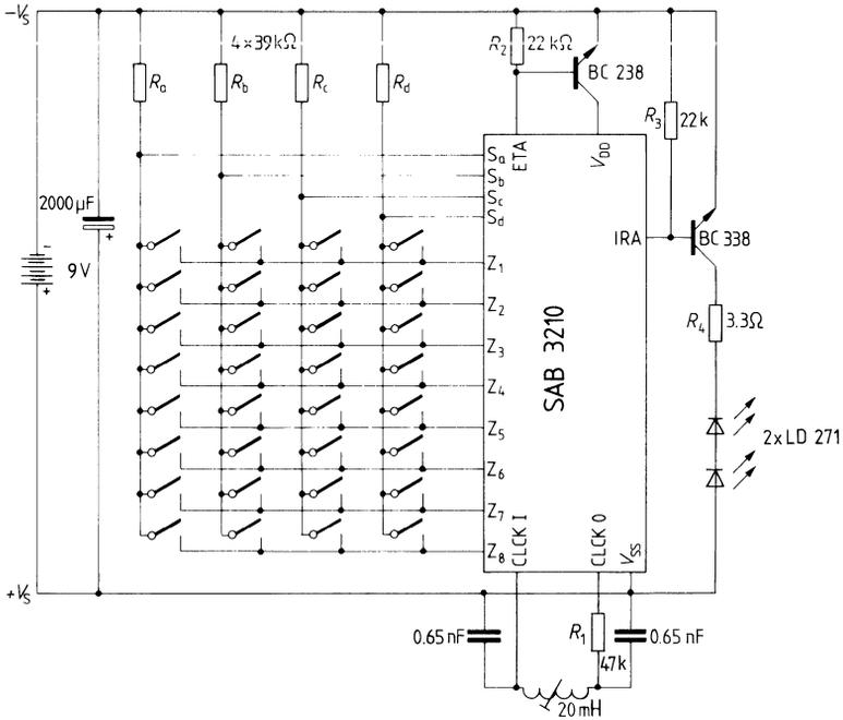
**Expanded external connection of the SAB 3210 for 60 instructions (example)**
