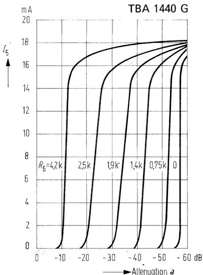
**Tuner control current versus attenuation**
