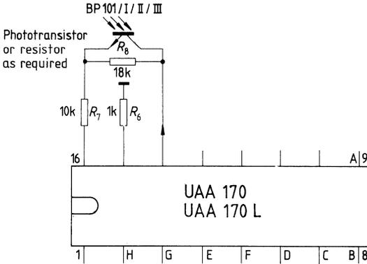
Pins 14, 15, and 16 serve to determine the diode current. Corresponding to the desired light intensity, the forward current of the diodes is linearly variable in the range  $I_f$  approx. 0 to 50 mA. The resistance at pin 15 defines the adjusting range. The resistances between pin 14 and 16 determine the current.
