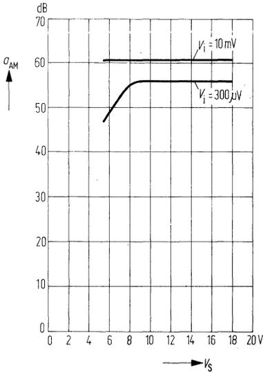
**AM suppression versus input voltage**
