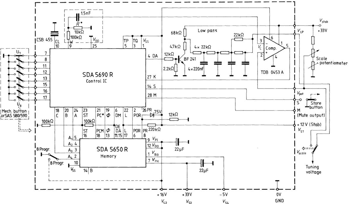
• The width of the window to retrieve the station can be set with the help of R.
