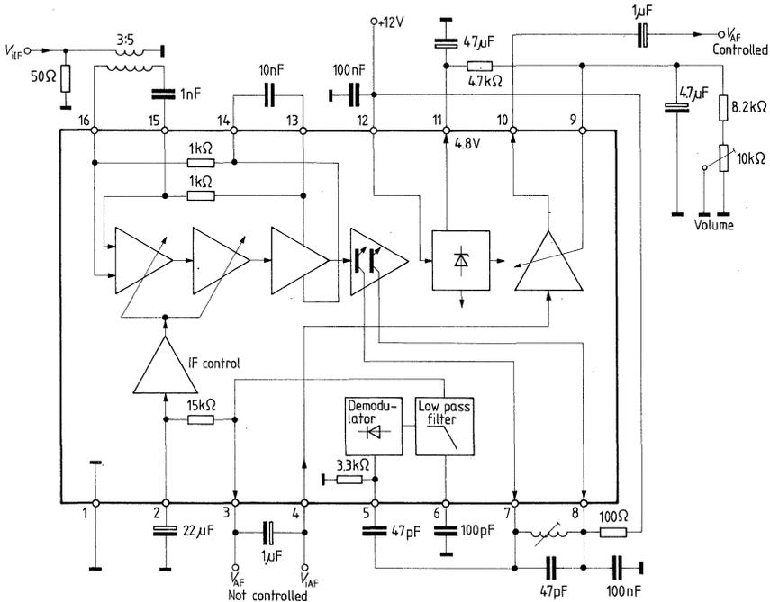
Application circuit for  $f_{i\text{IF}} = 39.2 \text{ MHz}$
