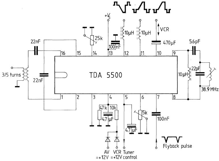
Highly amplifying controlled video IF amplifier including demodulator, low-ohmic video outputs for positive- and negative-going signal, gated control, AFC output, and delayed tuner control.
