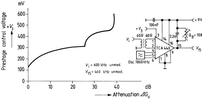
The input is not power matched and can be driven with a higher resistance.  $V_i$  is chosen such that a constant  $V_{15}$  is obtained (50 mV<sub>pp</sub>).
