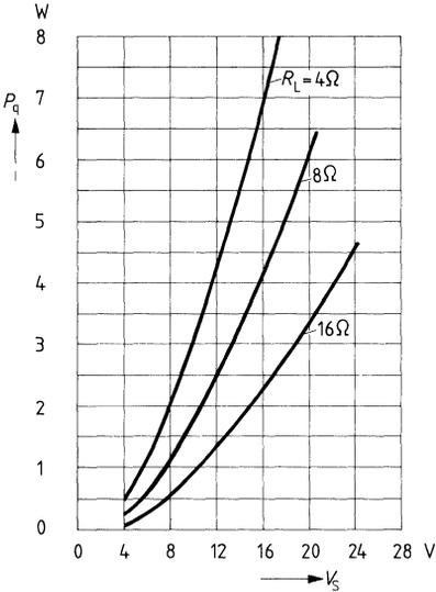
**Max. power dissipation versus supply voltage at sine-shaped driving**
