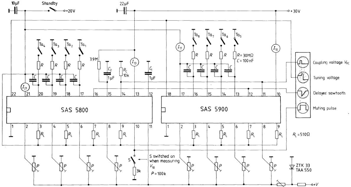
SAS 5800 is absolutely necessary for testing SAS 5900;
