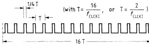
**Actuating a button (e.g. 1a),  $f_{CLKKI} = 500 \text{ kHz}$**
