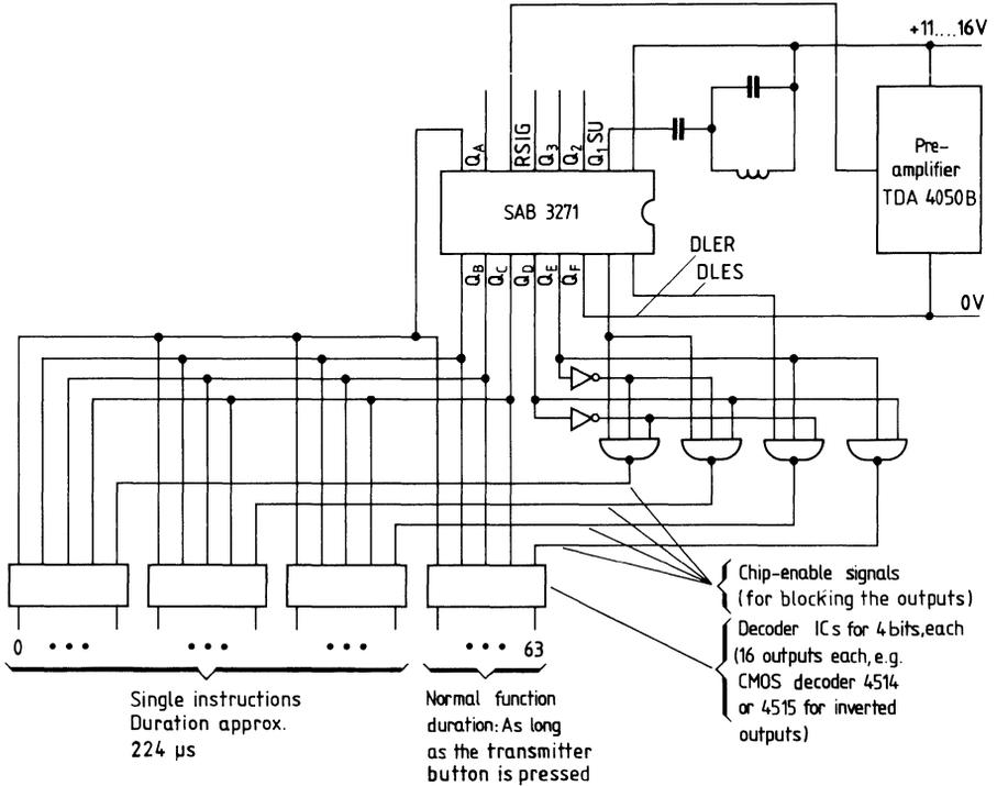
With this circuit all instructions of the instruction table but the end instruction (instr. No. 62) and the not allowed instruction (instr. No. 63) can be obtained in decoded form, whereby instructions 33, 34, and 35 are already decoded in the circuit (outputs  $Q_1$ SU,  $Q_2$ ,  $Q_3$ ). If DLES is used, single instructions or the normal function will be generated.
