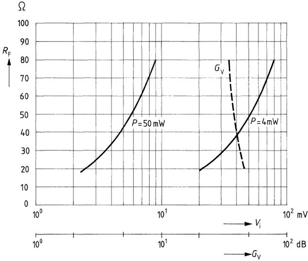
**Output power versus feedback resistance and input voltage**
