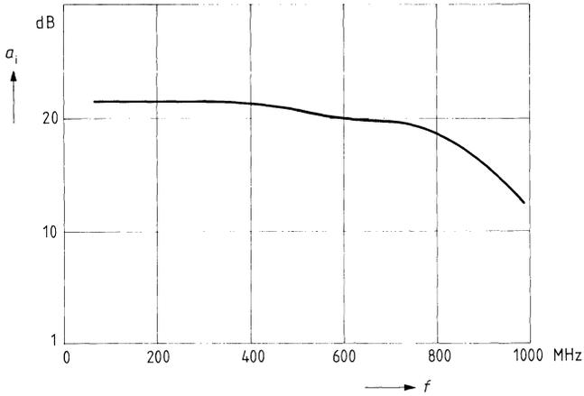
Input sensitivity versus input frequency  $V_i = f(f)$
