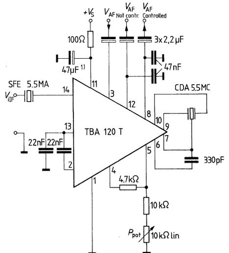
1) Omitting the electrolytic capacitor  $47 \mu\text{F}$  on pin 11 changes volume-control range.
