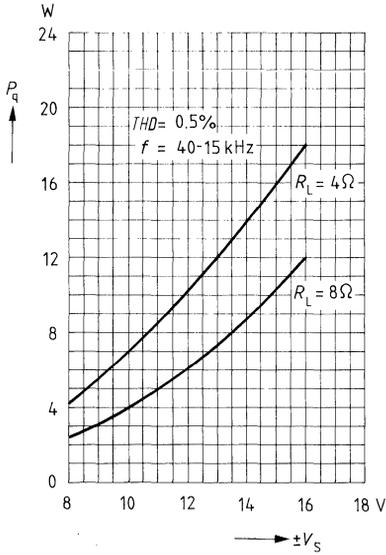
**Output power versus supply voltage**
