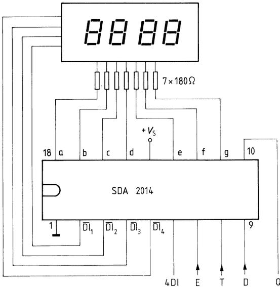
At 2-digit operation ( $\overline{DI}_1$  and  $\overline{DI}_2$ ), 4 DI is grounded
