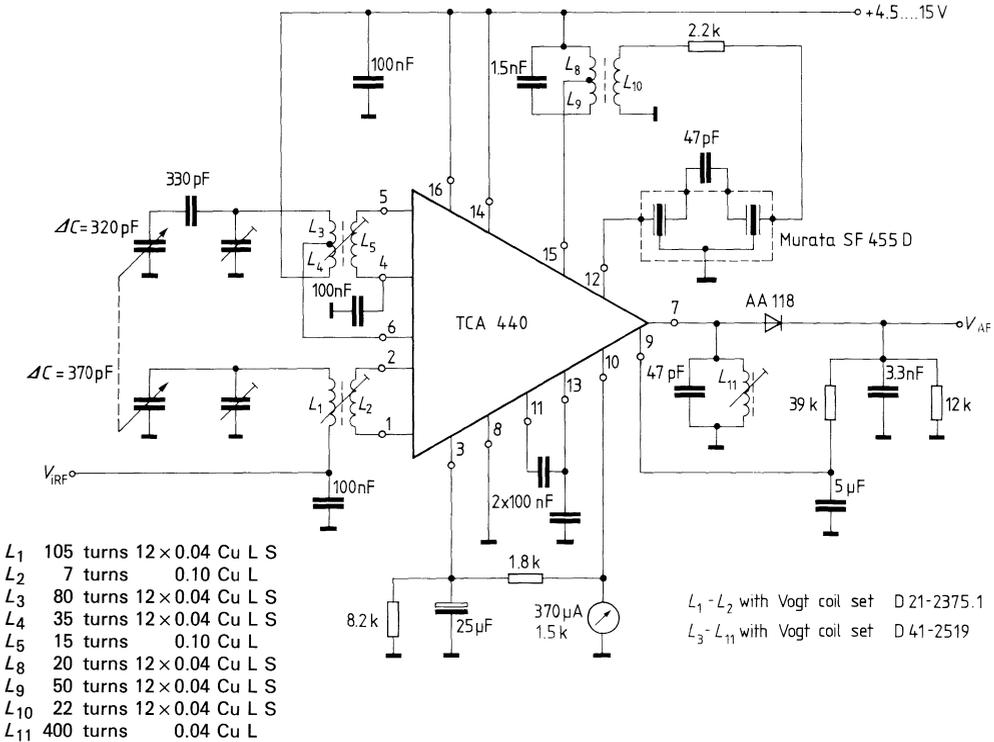
**Test figures for application example for MW**
