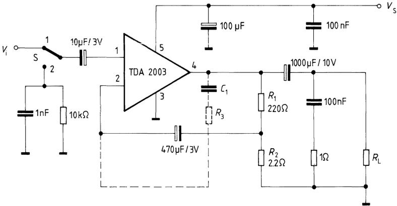
Switch S in position 2 for noise measurement
