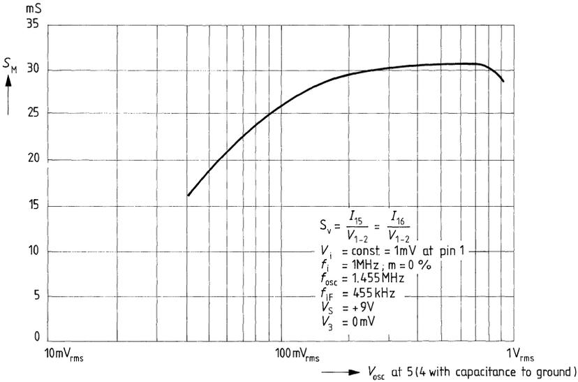
**Measured values for application example for MW using BB 113**
