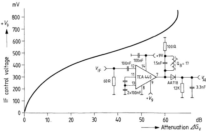
$V_{IF}$  (469 kHz;  $m = 80\%$ ;  $f_{mod} = 1 \text{ kHz}$ ) is chosen such that always a constant  $V_{AF}$  is obtained (200 mV<sub>rms</sub>).
