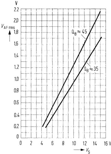
**AF output voltage and total harmonic distortion versus input voltage**
