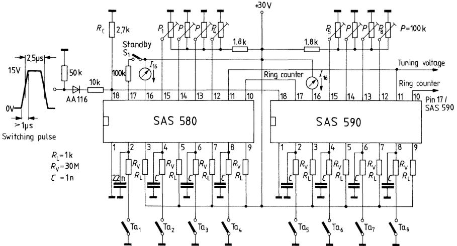
SAS 580 is absolutely necessary for testing SAS 590;
