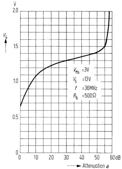
**Tuner control current versus attenuation**
