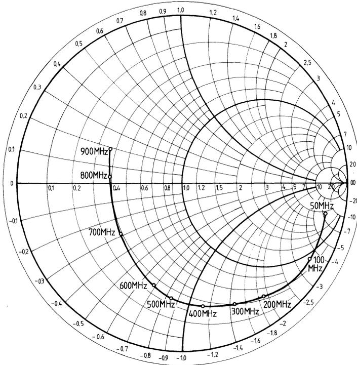
Decoupling of the VHF and UHF input versus input frequency  $\alpha_i = f(f)$
