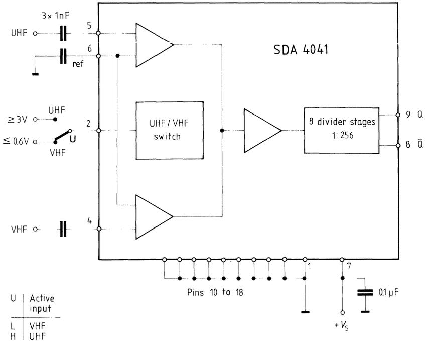
Pins 10 to 18 are internally interconnected by means of a metal web, they are also connected to the chip body. They are intended for cooling and ground connection.
