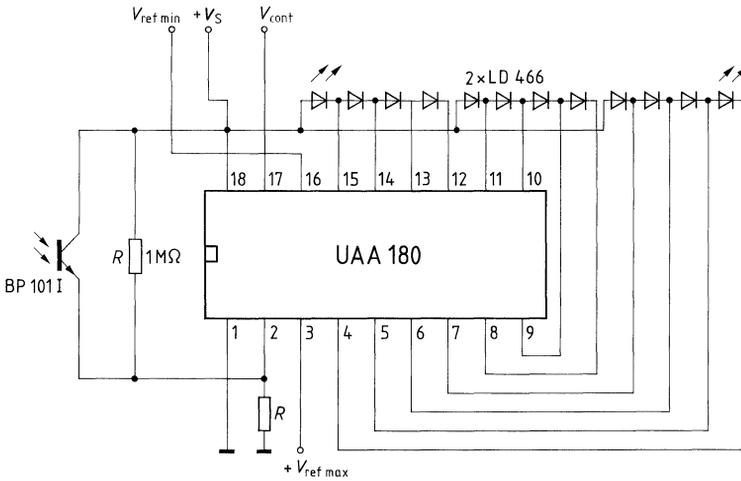
If a quartet does not need the full number of display diodes and if the first wired diodes shall be left luminous at full driving, bridges have to be inserted replacing the missing LEDs. Otherwise the first diodes of the quartet switch off with exceeding their display range.
