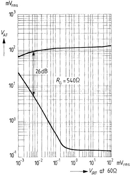
**Signal to noise ratio versus RF input voltage switching position ②**
