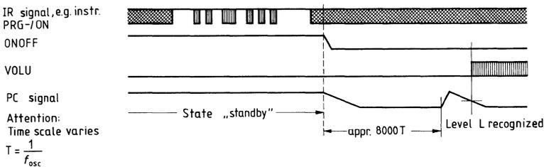
Example b) ONOFF is connected to  $V_{DD}$  during the supply voltage rise via wiping contact
