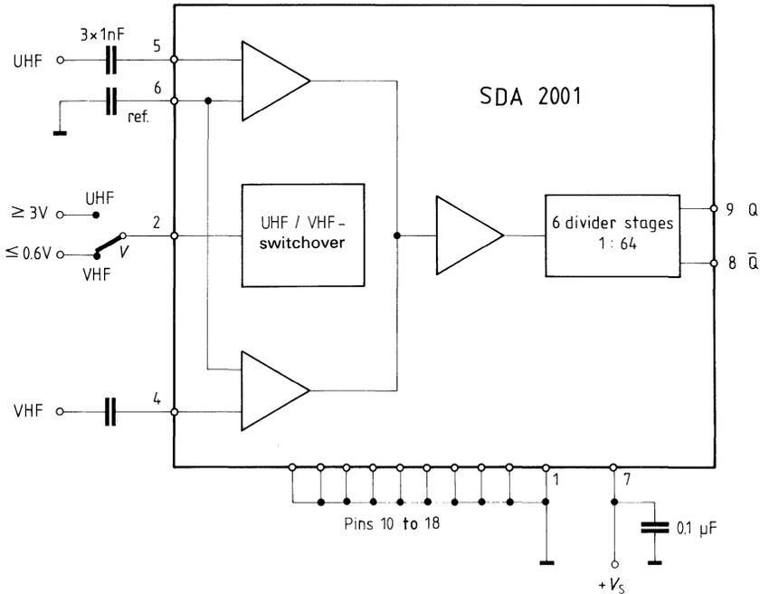
Block diagram incl. internal pin configuration
