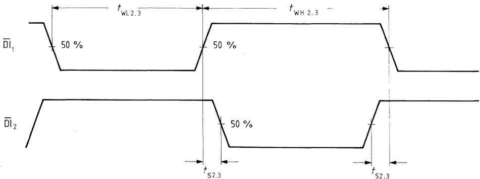
Timing diagram: Set-up and hold times
