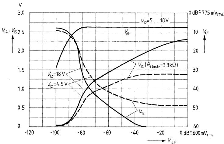
**AF output voltage, noise voltage versus input voltage**
