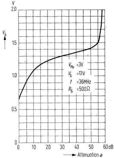
**Tuner control current versus attenuation**
