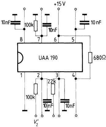
**Measuring circuit for dynamic measurements**
