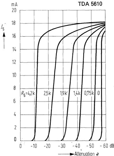
**Tuner control current versus attenuation**
