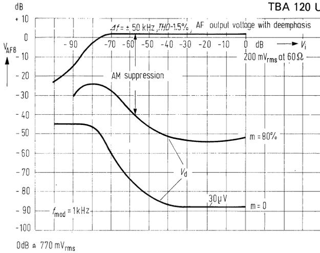
**AF output voltage and disturbance voltage versus input voltage**
