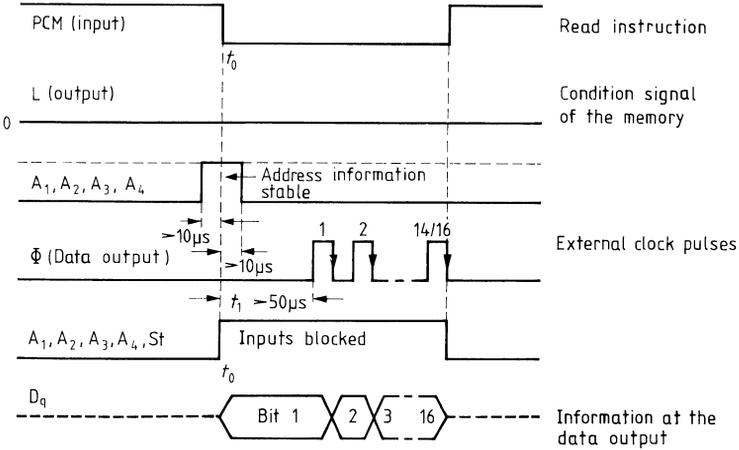
Fig. 2 Erase-write operation
