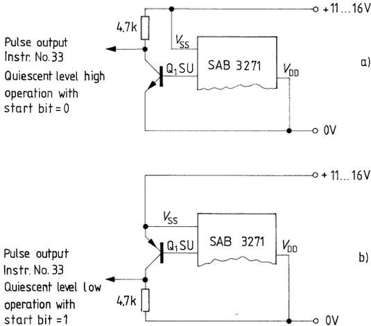
The circuit configured to a) can also be applied without restriction at the RS flip-flop output  $Q_2$ , the T flip-flop output  $Q_3$  and the parallel outputs  $Q_A$  to  $Q_F$  in order to change the outputs individually to the pulse function.
