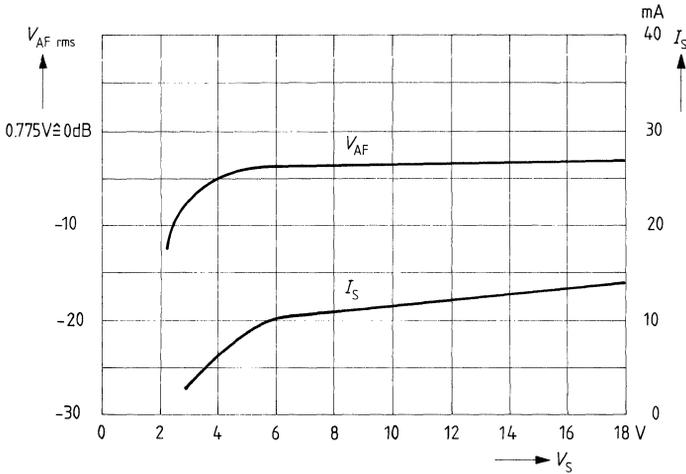
**AF output voltage, indicator voltage, squelch voltage versus input voltage**
