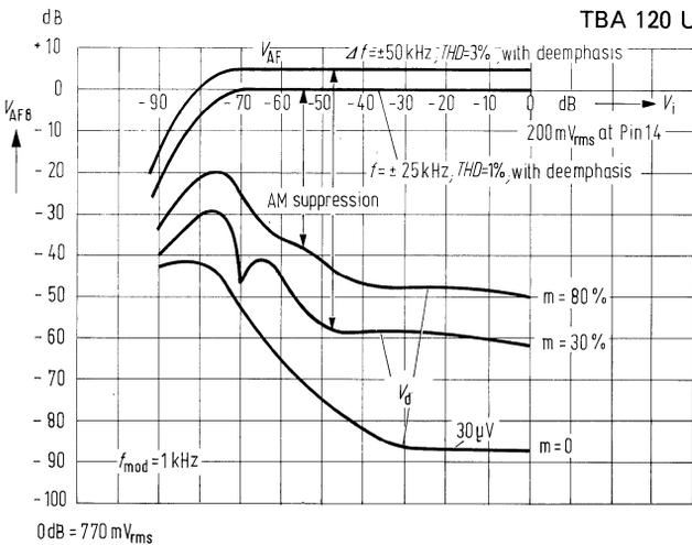
**AF output voltage (pin 8), disturbance voltage, and total harmonic distortion versus input voltage**
