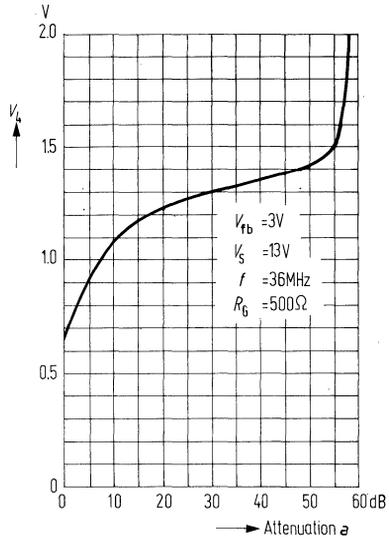
**Tuner control current versus attenuation**
