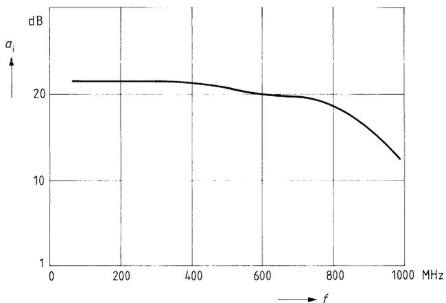
**Input sensitivity versus input frequency**
