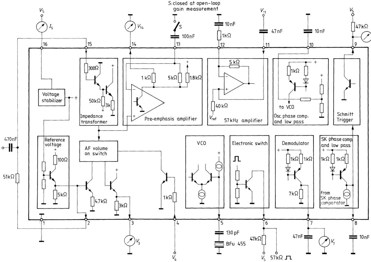
Block diagram and test circuit
