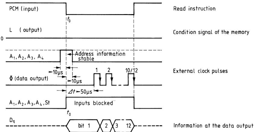
Fig. 2 Erase-write operation
