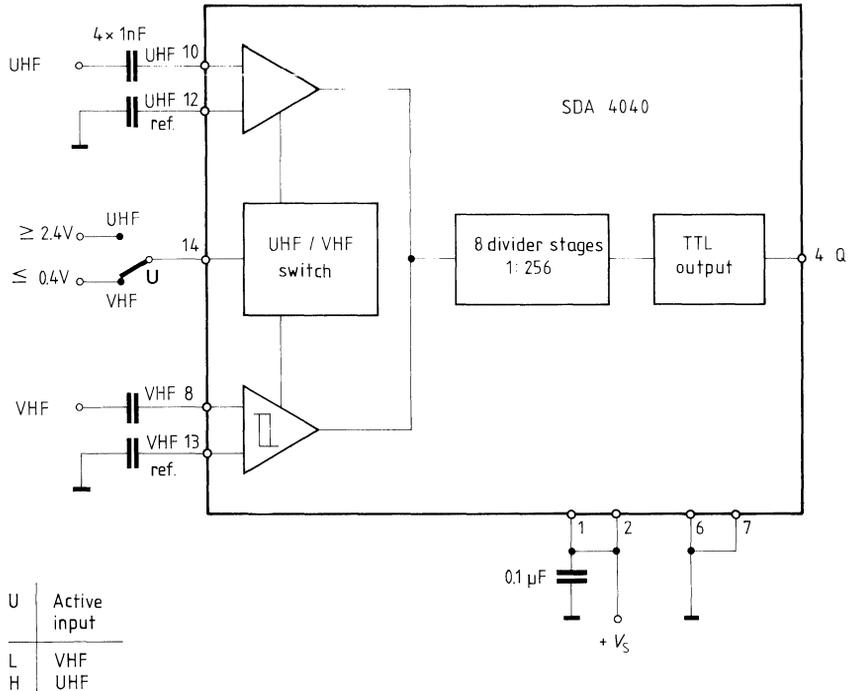
If needed hysteresis can be achieved at the UHF input by connecting a resistor (e. g. 33 k $\Omega$ ) between UHF<sub>ref</sub> (pin 12) and ground (pins 6, 7). At the VHF input the hysteresis can be increased in the same way.
