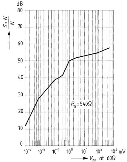
**Signal to noise ratio versus RF input voltage (parameter is generator impedance) (switching position 1)**
