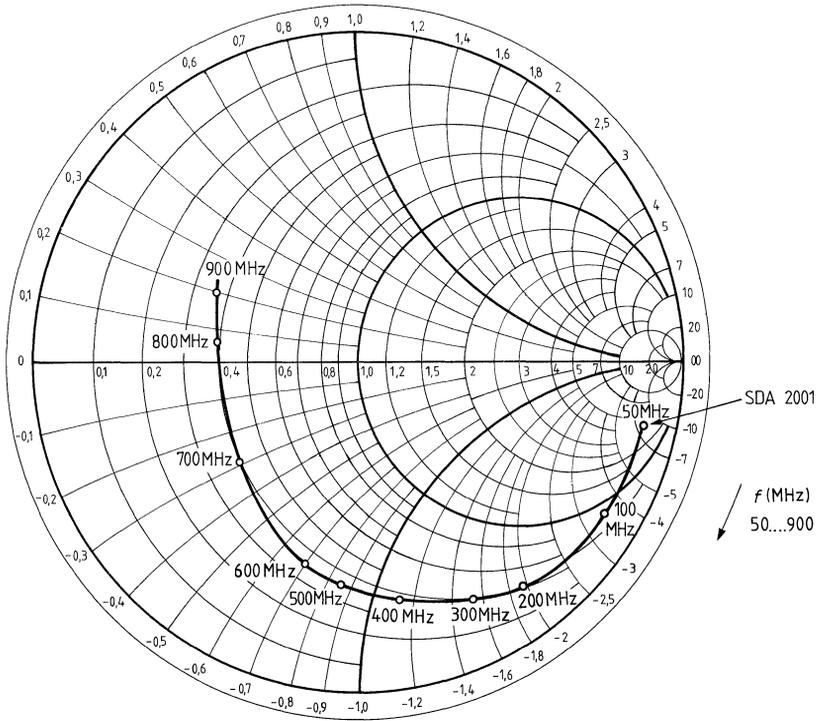
**Decoupling of the VHF and UHF input versus input frequency**
