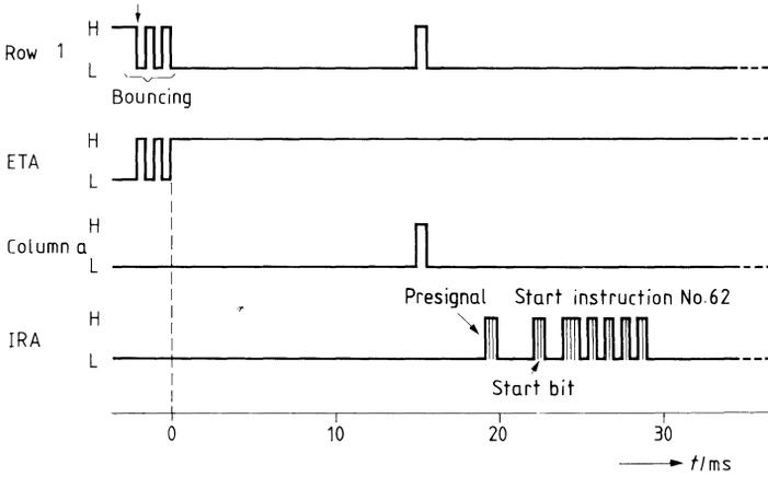
**Releasing a button (1a),  $f_{CLKKI} = 500 \text{ kHz}$**
