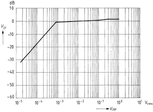
Control characteristic curve  $V_S = 10 \text{ V}$ ;  $V_{\text{IF}} = 225 \text{ mV}_{\text{rms}}$
