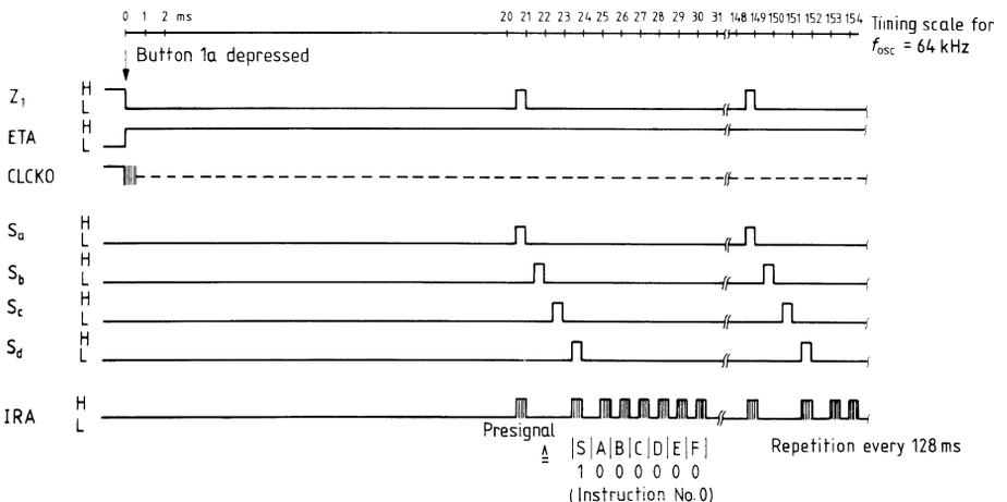
Timing diagram 3 (releasing a button)
