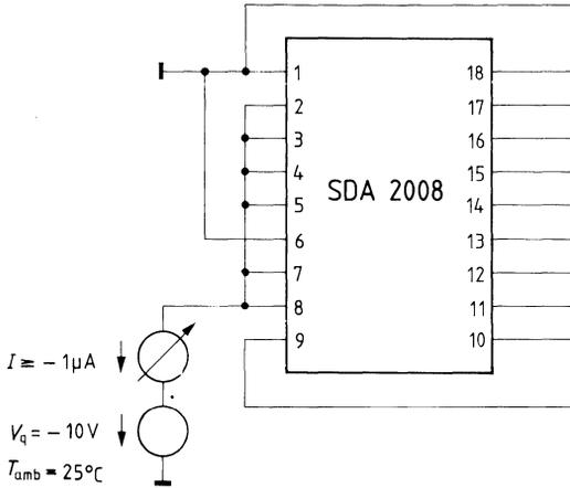
IRA remote control signal output (test circuit)
