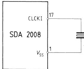
$$C_c \geq 10 \text{ nF} \quad f_{\text{CLCKI}} \approx \frac{1}{2\pi\sqrt{L_0 C_0}}$$
