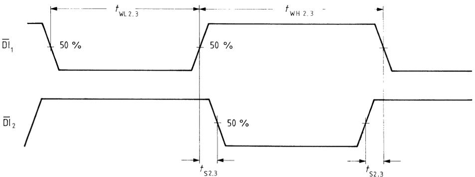
Timing diagram: Set-up and hold times
