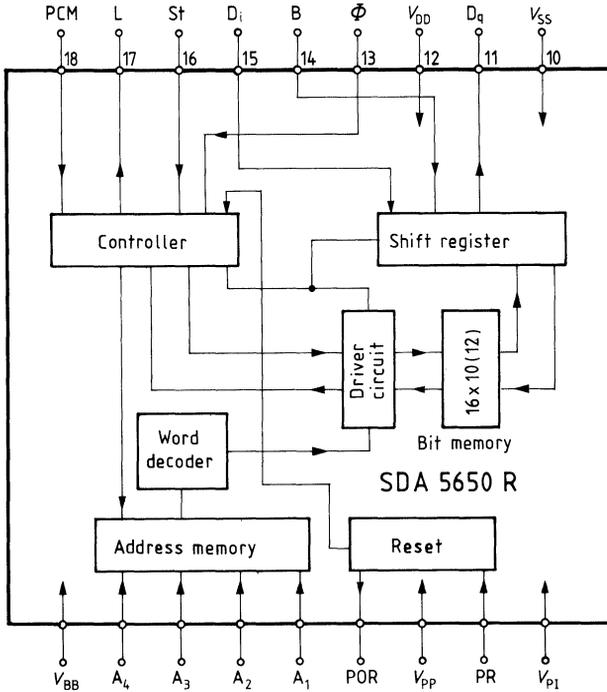
Supply voltage for the tuning memory in radios
