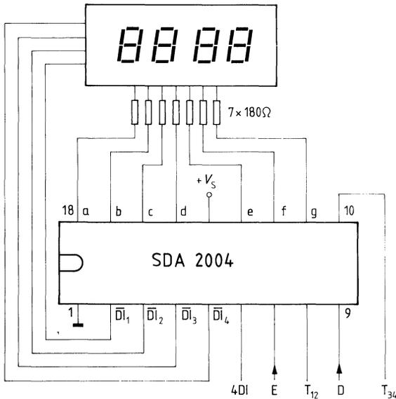
At 2-digit operation ( $\overline{DI}_1$  and  $\overline{DI}_2$ ), 4 DI is grounded
