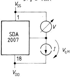
Test circuit 2:  $I = 1\mu\text{A}$
