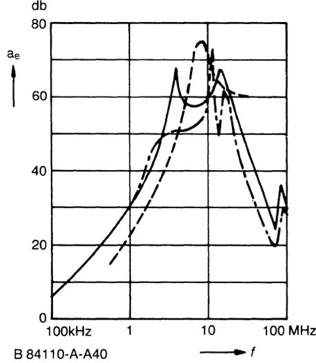
Insertion loss (typical values at  $Z = 50 \Omega$ )
