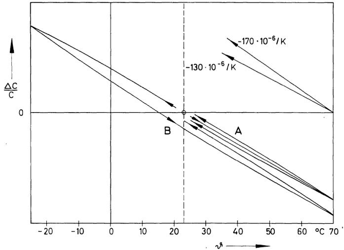
The point of regression of a temperature cycle between room temperature and the maximum limit temperature (curve A) can lie above or below the point of origin.
