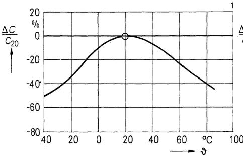
Capacitance change versus temperature for low-loss capacitors (typical values)
