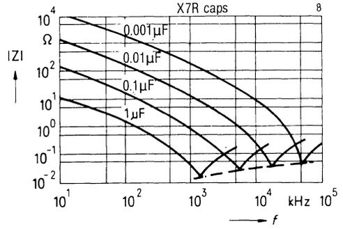
Resonant frequency versus capacitance
