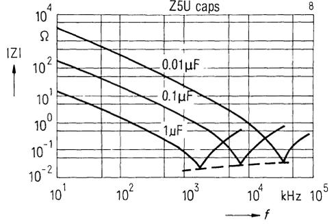
**Resonant frequency versus capacitance**
