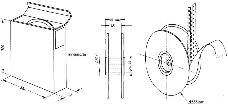
**Taping of chip capacitors with rated voltage 50V–**
