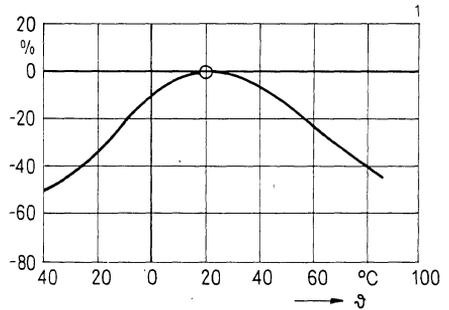
Dissipation factor versus temperature (typical values)
