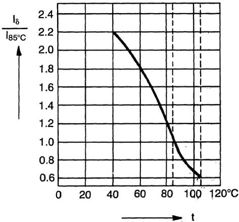
Load duration B versus ambient temperature  $\theta_{amb}$
