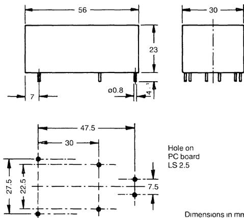
Filter for printed circuits
