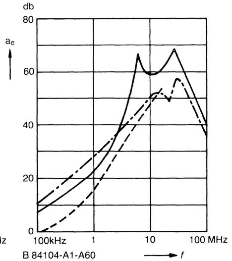
Insertion loss (typical values at  $Z = 50 \Omega$ )
