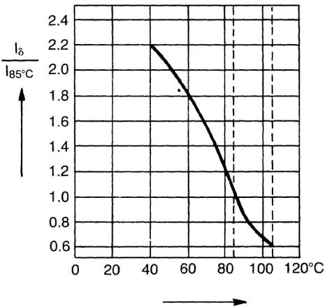
Load duration B versus ambient temperature  $\theta_{amb}$
