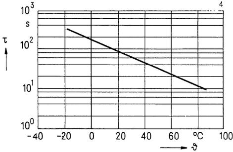
**Insulation resistance versus temperature**
