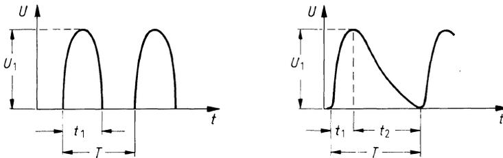
Examples for dividing a non-sinusoidal voltage into approximately sinusoidal parts to calculate the power dissipation for a capacitor.
