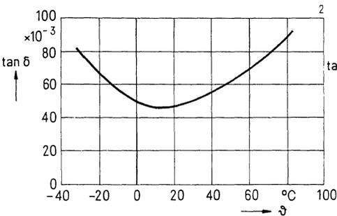
Dissipation factor versus temperature for low-loss capacitors (typical values)
