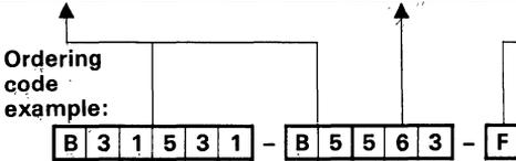
STYROFLEX capacitor B31531 56 000 pF ± 1% 63 V GSE
