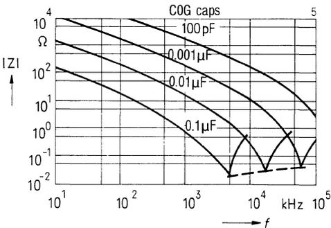
**Resonant frequency versus capacitance**
