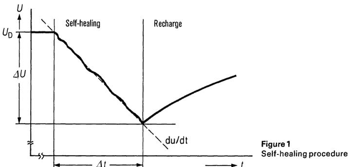
In heavy current supplies, even in mains, voltage peaks up to 3 times the rated supply voltage still frequently occur. These voltage peaks mostly result from switching operations with magnetic parts. Locations of breakdown are weak points, such as included conducting parts, holes in the dielectric, or conductive contaminations, which could not be eliminated at the burnout during the production process.
