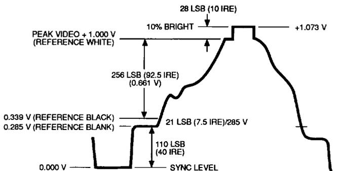
Figure 3. Composite Video Output Signal
