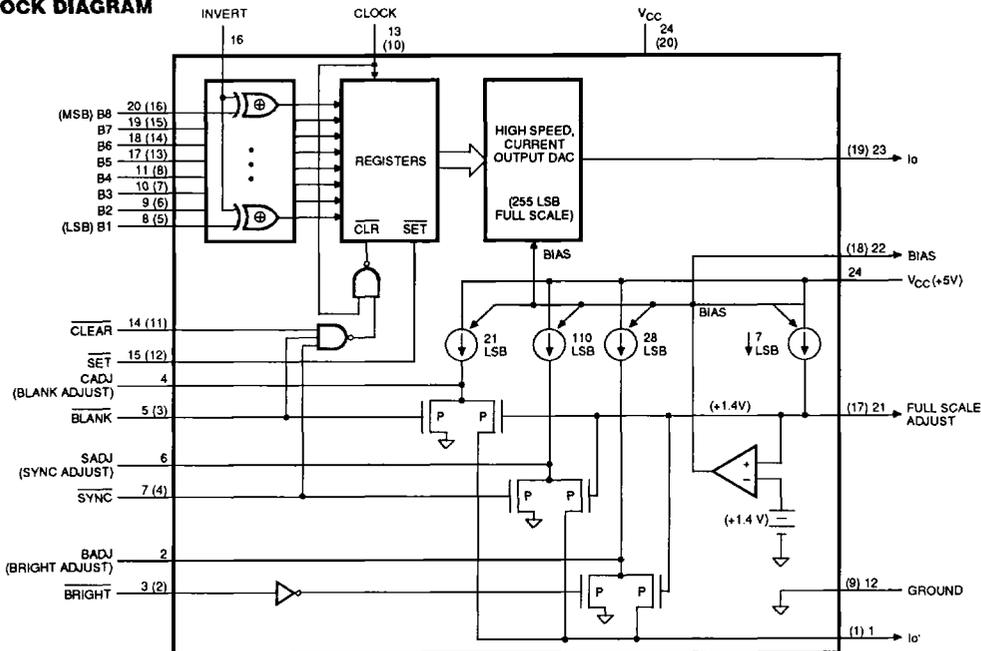
NOTE: NUMBERS NEXT TO SIGNAL NAMES ARE 24-PIN DIP PINS FOR SC11401 AND SC11403. NUMBERS IN ( ) ARE 20-PIN DIP PINS FOR SC11402 AND SC11404.
