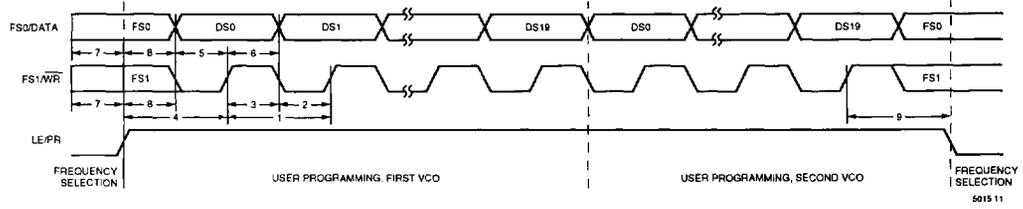
**Timing for Programming Two Clock Generators**
