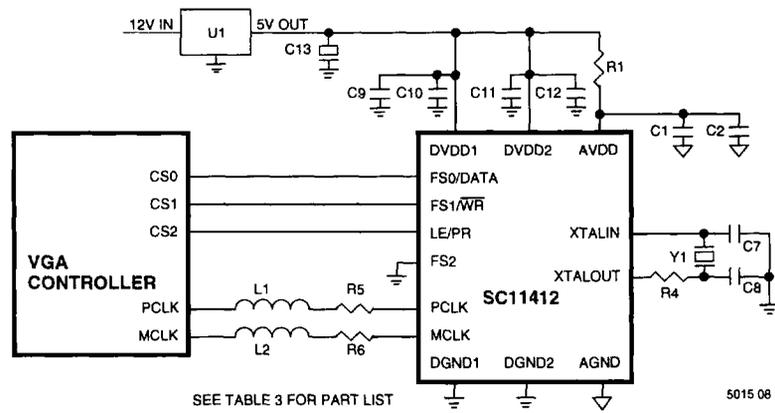
Figure 3. Application Diagram for 5 Pre-Programmed and Two User-Programmable Pixel & Memory Clock Frequencies
