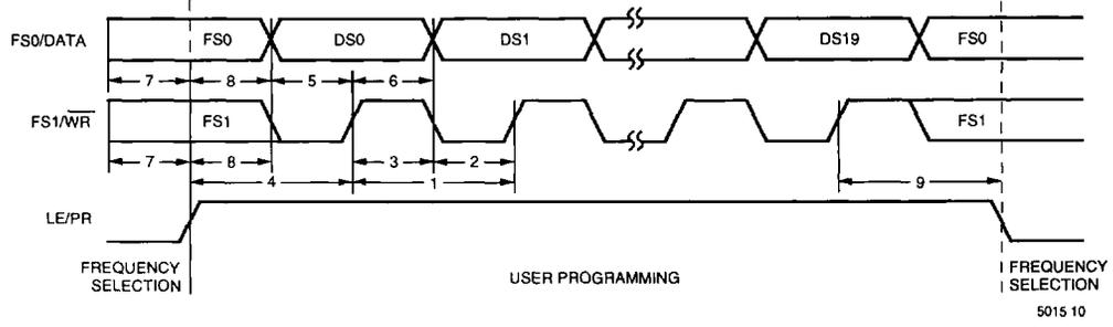
**Timing for Programming One Clock Generator**
