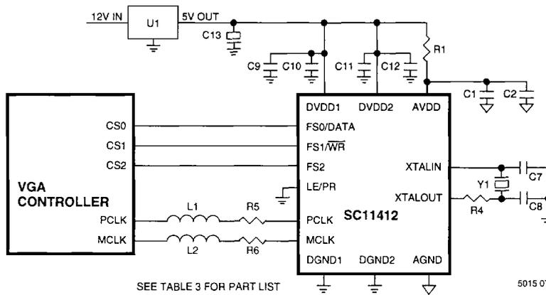
Figure 2. Application Diagram for 9 Pre-Programmed Pixel & Memory Clock Frequencies
