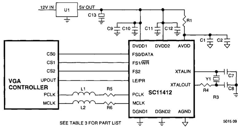
Figure 4. Application Diagram for 9 Pre-Programmed and Two User-Programmable Pixel & Memory Clock Frequencies
