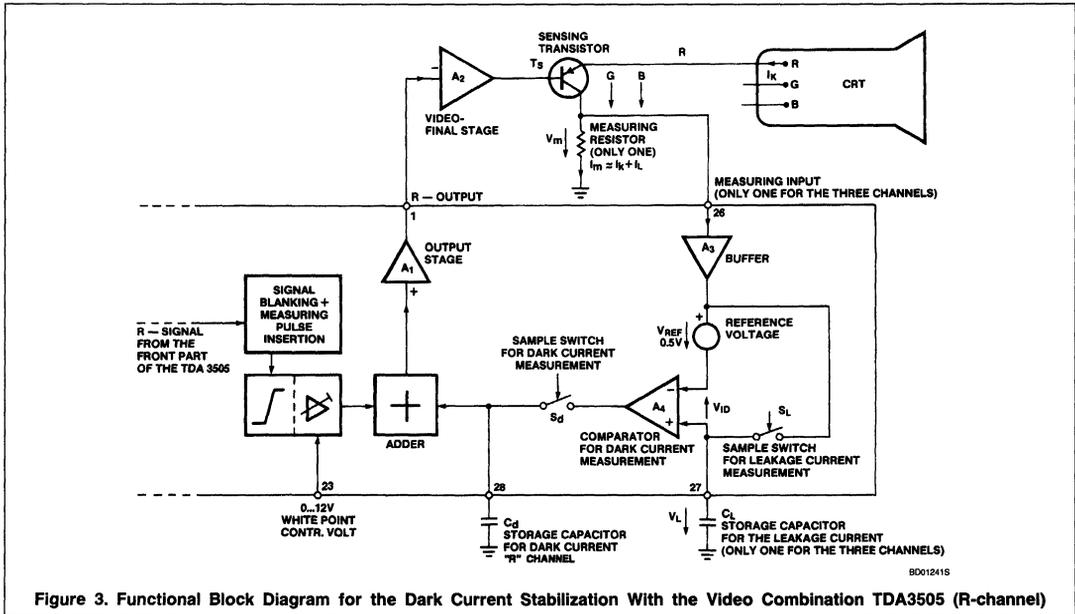
Figure 3. Functional Block Diagram for the Dark Current Stabilization With the Video Combination TDA3505 (R-channel)
