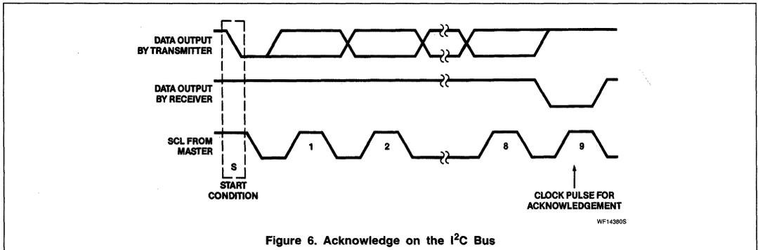
Figure 6. Acknowledge on the I<sup>2</sup>C Bus
