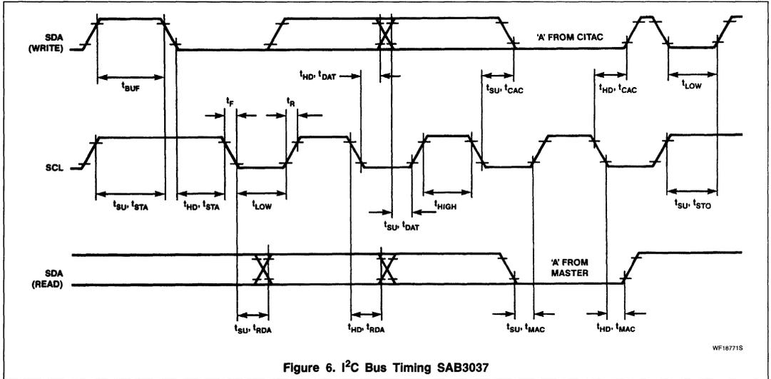
Figure 6. I<sup>2</sup>C Bus Timing SAB3037
