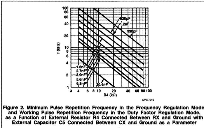
**Figure 2. Minimum Pulse Repetition Frequency in the Frequency Regulation Mode, and Working Pulse Repetition Frequency in the Duty Factor Regulation Mode, as a Function of External Resistor  $R_4$  Connected Between RX and Ground with External Capacitor  $C_5$  Connected Between CX and Ground as a Parameter**
