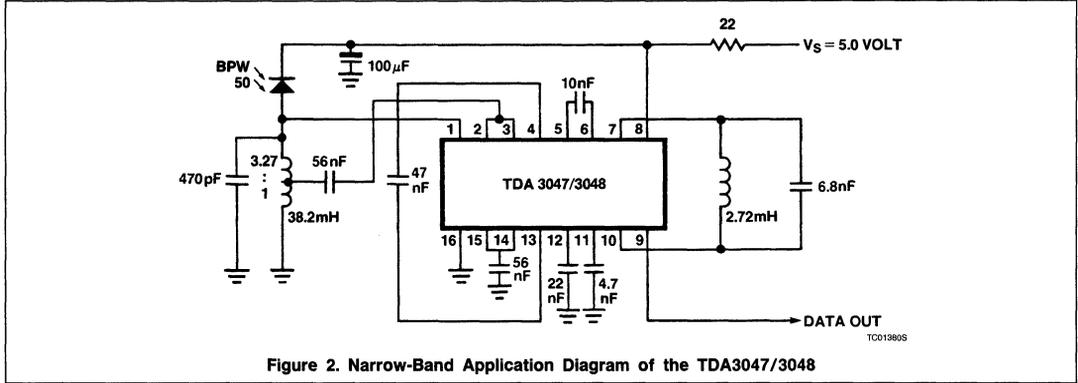
Figure 2. Narrow-Band Application Diagram of the TDA3047/3048
