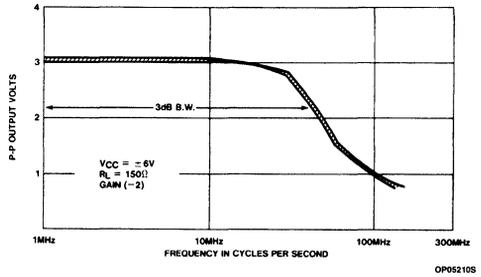
SE5539 Open-Loop Gain vs Frequency
