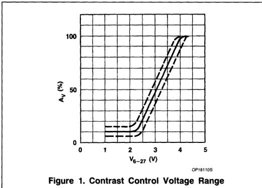
Figure 1. Contrast Control Voltage Range
