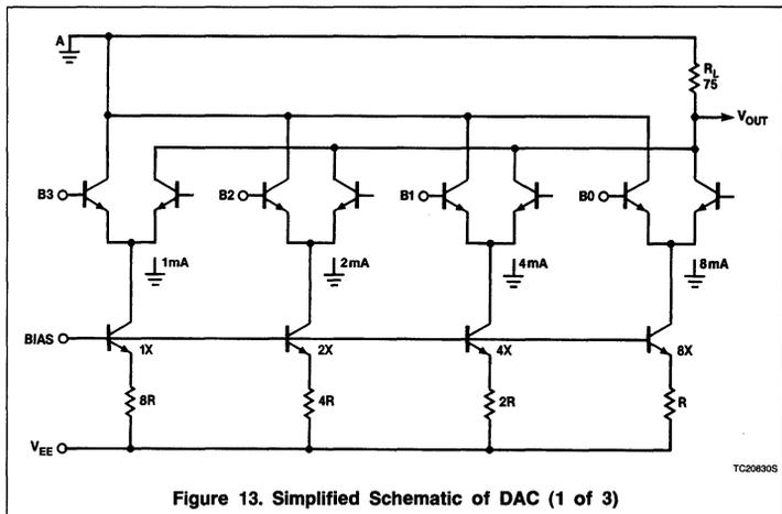
Figure 13. Simplified Schematic of DAC (1 of 3)
