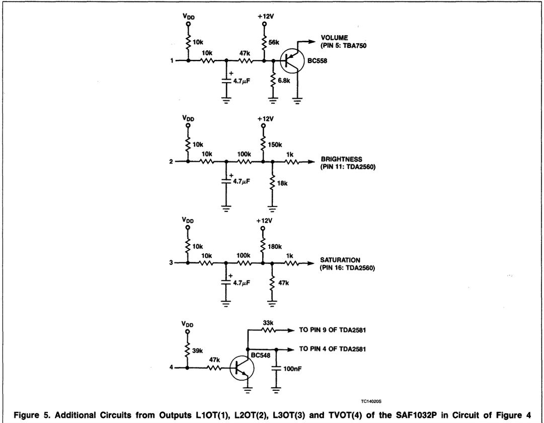
Figure 5. Additional Circuits from Outputs L1OT(1), L2OT(2), L3OT(3) and TVOT(4) of the SAF1032P in Circuit of Figure 4
