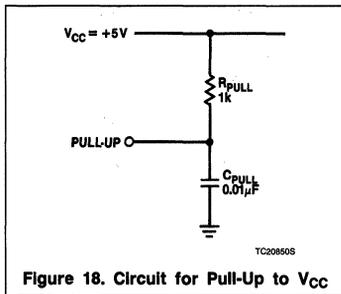
Figure 18. Circuit for Pull-up to V<sub>CC</sub>
