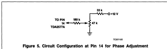
Figure 5. Circuit Configuration at Pin 14 for Phase Adjustment
