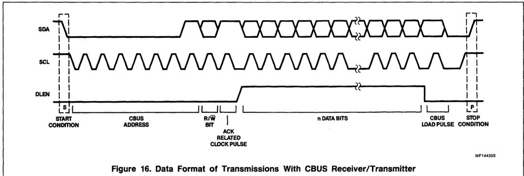
Figure 16. Data Format of Transmissions With CBUS Receiver/Transmitter
