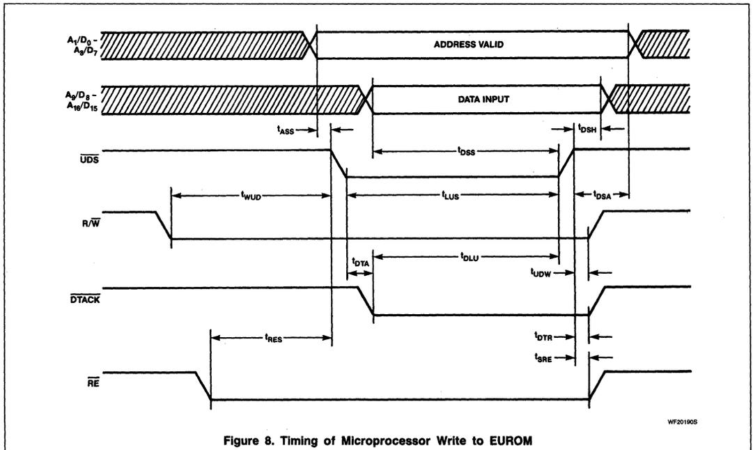
Figure 8. Timing of Microprocessor Write to EUROM
