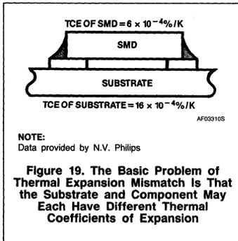
To address this problem, three basic solutions are emerging. First, the use of leadless ceramic chip carriers can sometimes be avoided by using leaded devices; the leads can flex and absorb the stress. Second, when this solution is not feasible, the stresses can be taken up by inserting a compliant elastomeric layer between the ceramic package and the epoxy glass substrate. Third, TCE values of component and substrate can be matched.
