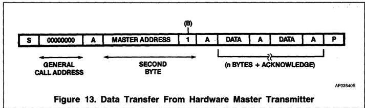
Figure 13. Data Transfer From Hardware Master Transmitter
