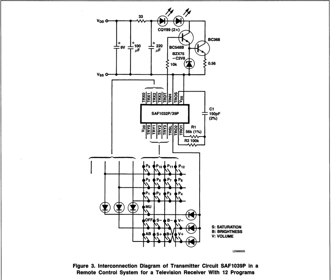
Figure 3. Interconnection Diagram of Transmitter Circuit SAF1039P in a Remote Control System for a Television Receiver With 12 Programs
