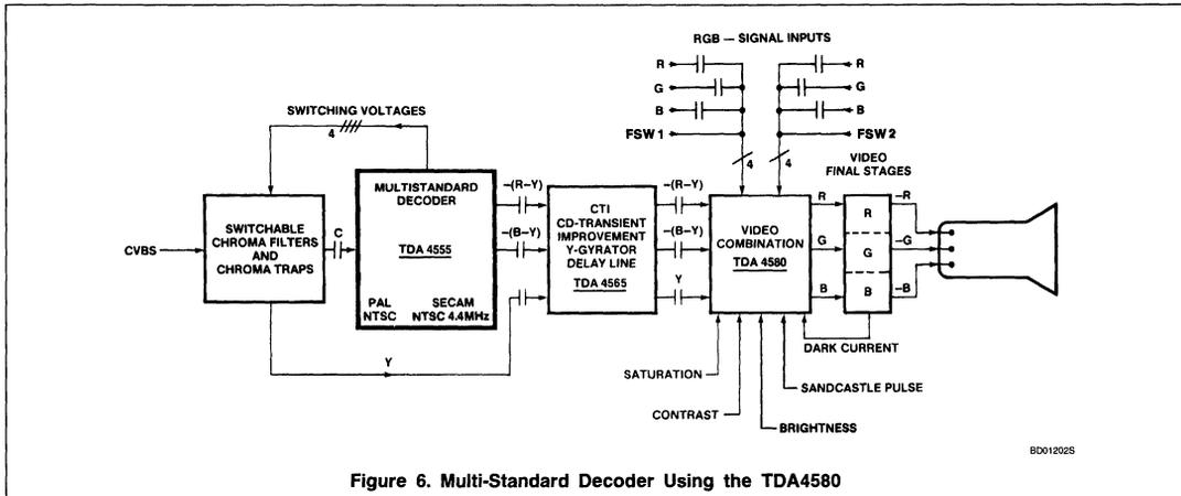
Figure 6. Multi-Standard Color Decoder Using the TDA4580
