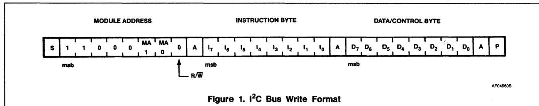
Figure 1. I<sup>2</sup>C Bus Write Format
