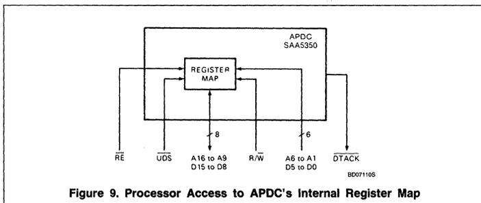
Figure 9. Processor Access to APDC's Internal Register Map
