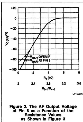
Figure 2. The AF Output Voltage at Pin 8 as a Function of the Resistance Values as Shown in Figure 3
