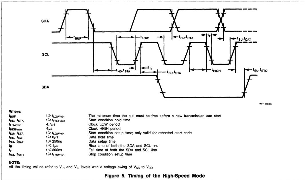
Figure 5. Timing of the High-Speed Mode
