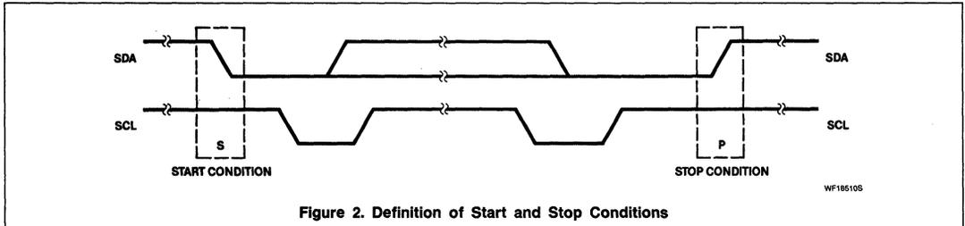
Figure 2. Definition of Start and Stop Conditions
