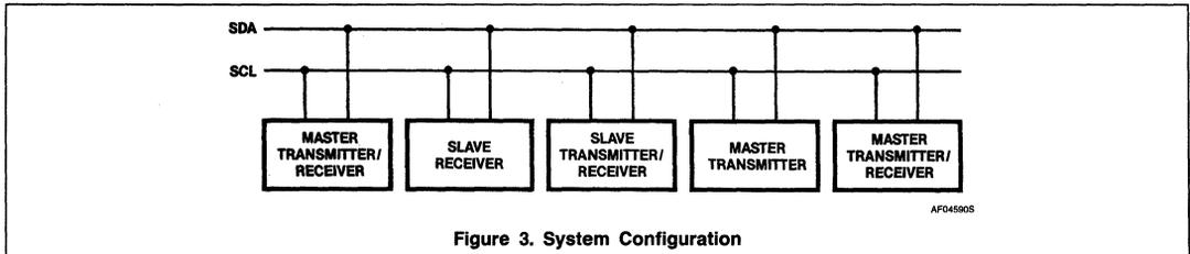
Figure 3. System Configuration
