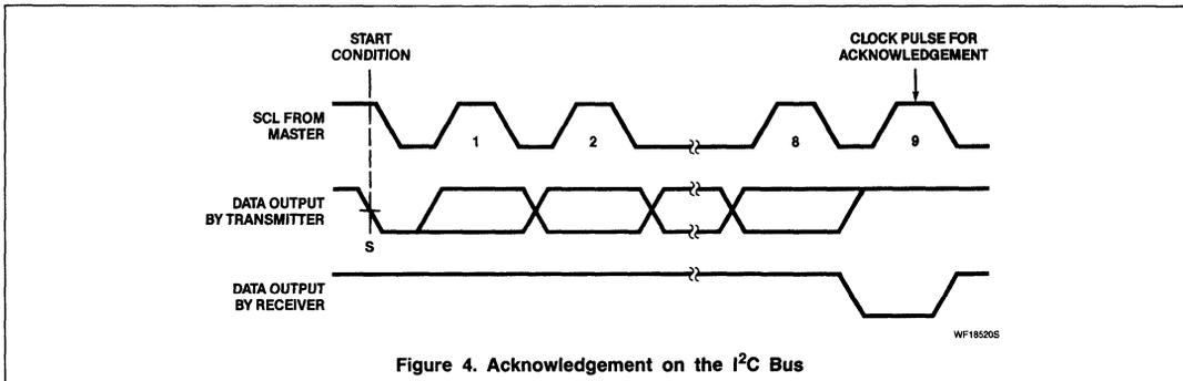
Figure 4. Acknowledgement on the I<sup>2</sup>C Bus
