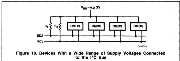
Figure 18. Devices With a Wide Range of Supply Voltages Connected to the I<sup>2</sup>C Bus
