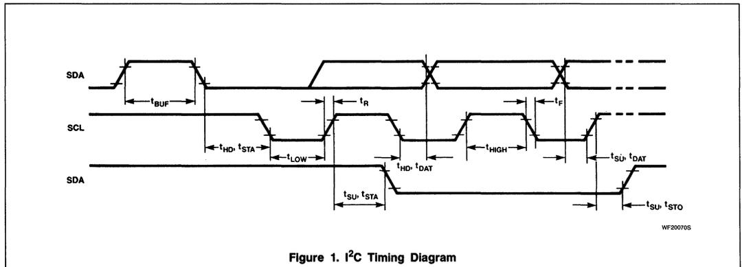
Figure 1. I<sup>2</sup>C Timing Diagram
