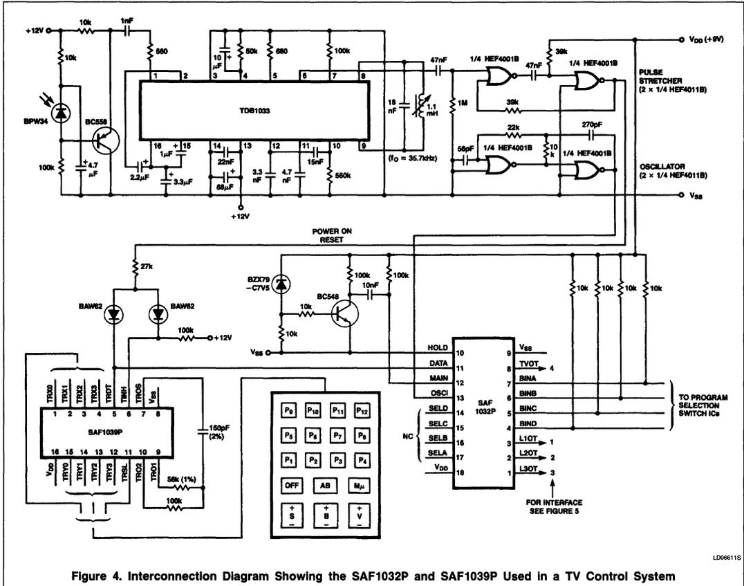
Figure 4. Interconnection Diagram Showing the SAF1032P and SAF1039P Used in a TV Control System
