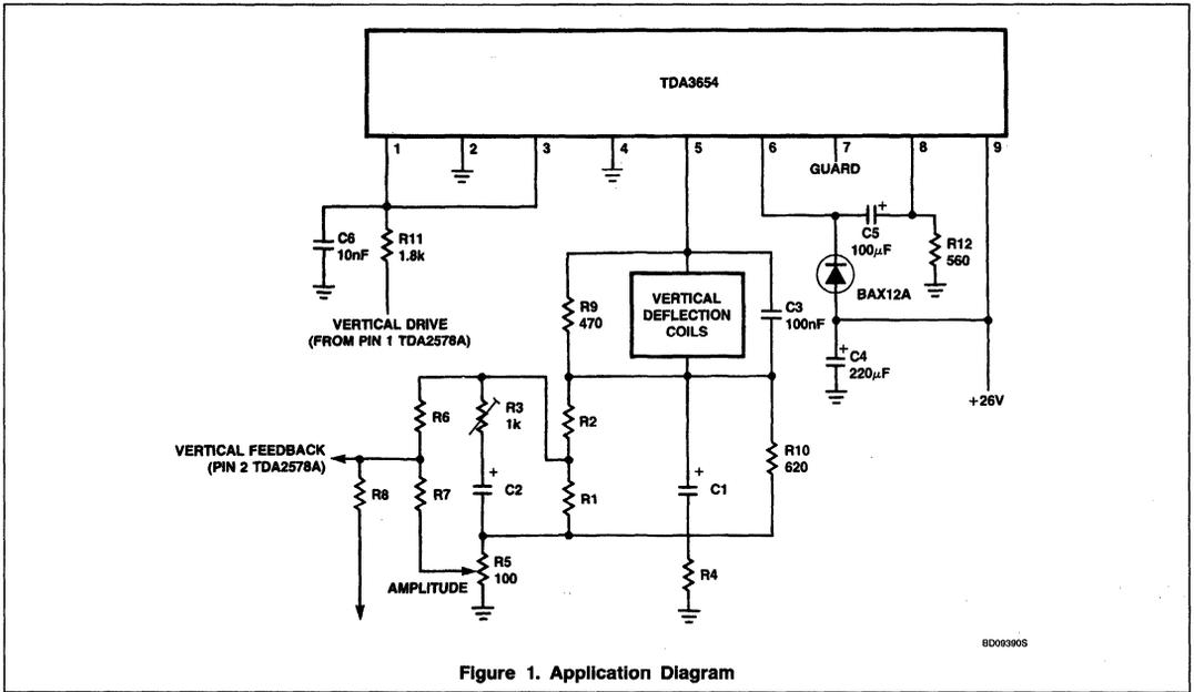
Figure 1. Application Diagram
