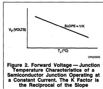
**Figure 2. Forward Voltage — Junction Temperature Characteristics of a Semiconductor Junction Operating at a Constant Current. The K Factor is the Reciprocal of the Slope**
