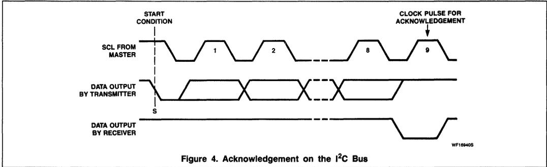
Figure 4. Acknowledgement on the I<sup>2</sup>C Bus
