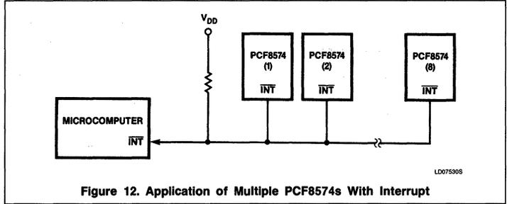
Figure 12. Application of Multiple PCF8574s With Interrupt
