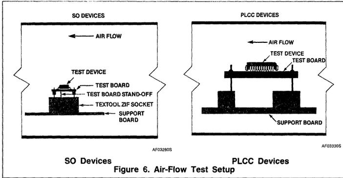
Figure 6. Air-Flow Test Setup
