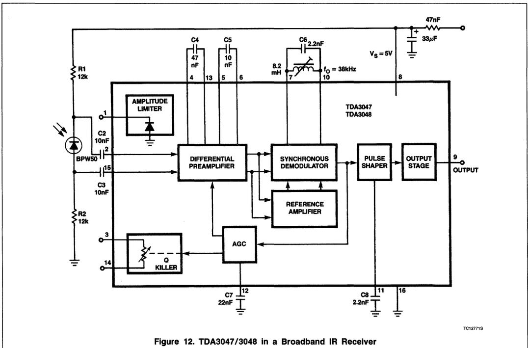
Figure 12. TDA3047/3048 in a Broadband IR Receiver
