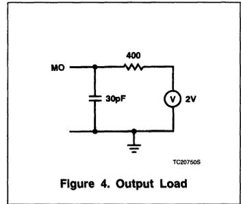
Figure 4. Output Load
