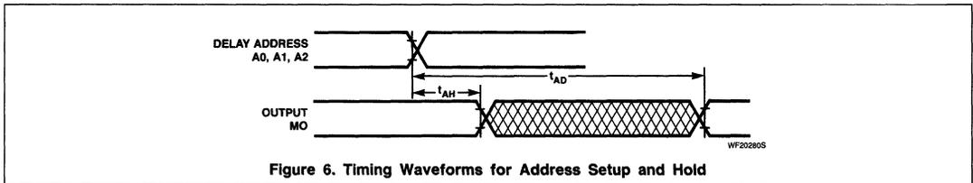
Figure 6. Timing Waveforms for Address Setup and Hold
