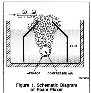
Figure 1. Schematic Diagram of Foam Fluxer
