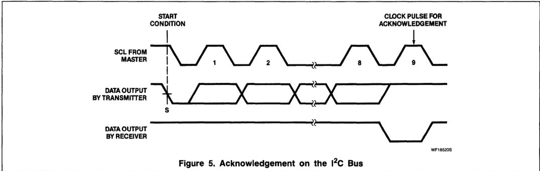
Figure 5. Acknowledgement on the I<sup>2</sup>C Bus
