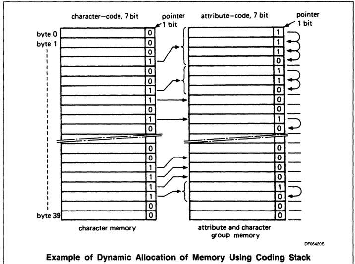
Stack coding used in APDC
