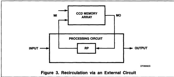
Figure 3. Recirculation via an External Circuit
