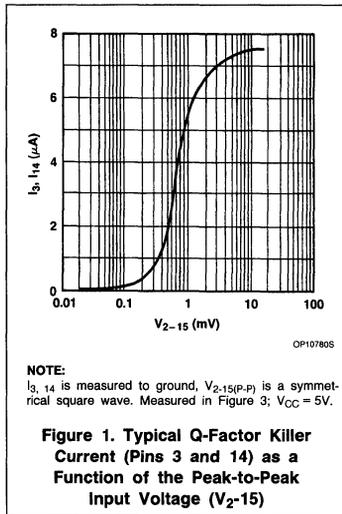
**Figure 1. Typical Q-Factor Killer Current (Pins 3 and 14) as a Function of the Peak-to-Peak Input Voltage ( $V_{2-15}$ )**
