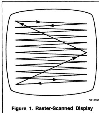
Figure 1. Raster-Scanned Display
