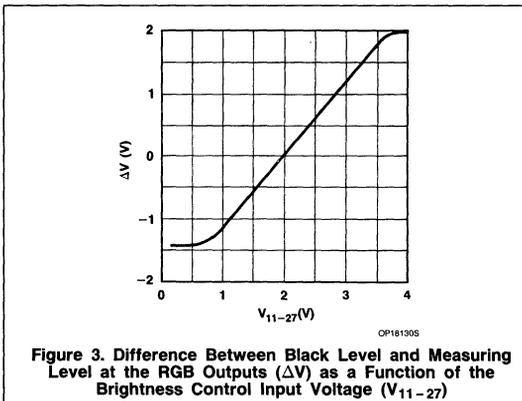
Figure 3. Difference Between Black Level and Measuring Level at the RGB Outputs ( $\Delta V$ ) as a Function of the Brightness Control Input Voltage ( $V_{11-27}$ )
