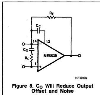
Figure 8.  $C_C$  Will Reduce Output Offset and Noise
