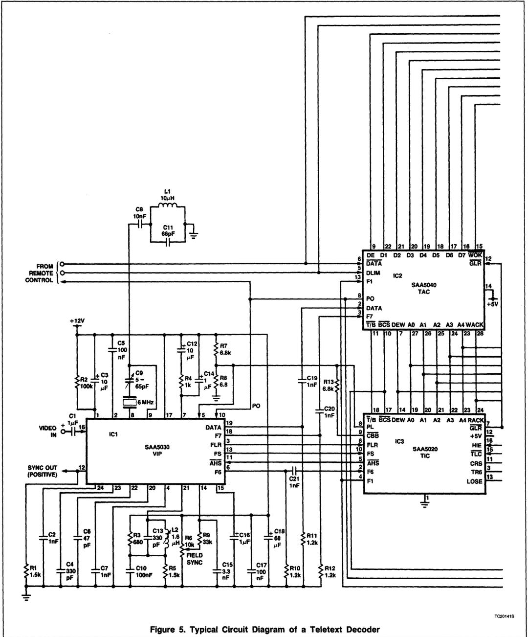
Figure 5. Typical Circuit Diagram of a Teletext Decoder
