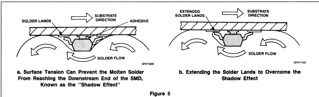
**a. Surface Tension Can Prevent the Molten Solder From Reaching the Downstream End of the SMD, Known as the "Shadow Effect"**
