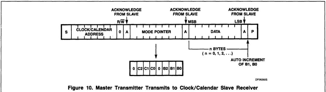
Figure 10. Master Transmitter Transmits to Clock/Calendar Slave Receiver
