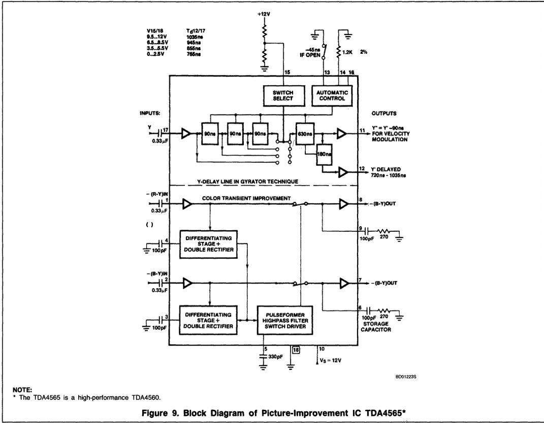
Figure 9. Block Diagram of Picture-Improvement IC TDA4565\*
