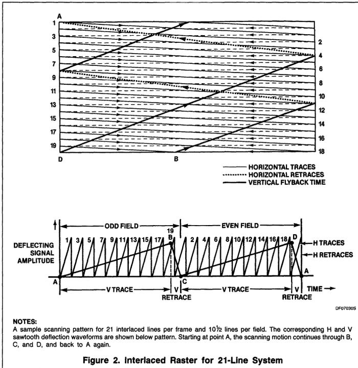
Figure 2. Interlaced Raster for 21-Line System
