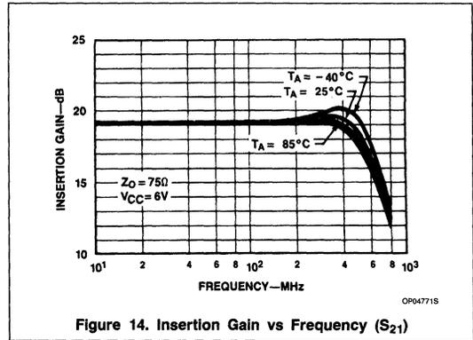
Figure 14. Insertion Gain vs Frequency ( $S_{21}$ )
