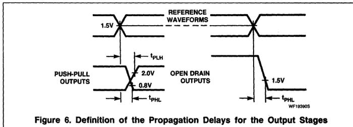
Figure 6. Definition of the Propagation Delays for the Output Stages
