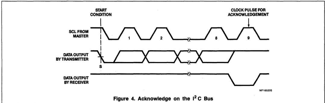
Figure 4. Acknowledge on the I<sup>2</sup>C Bus
