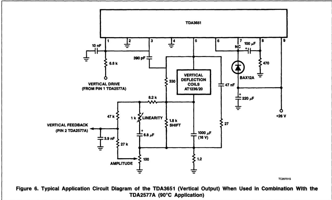
Figure 6. Typical Application Circuit Diagram of the TDA3651 (Vertical Output) When Used in Combination With the TDA2577A (90°C Application)
