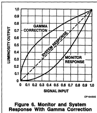
Figure 6. Monitor and System Response With Gamma Correction
