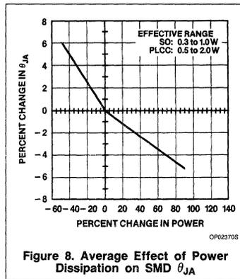
Figure 8. Average Effect of Power Dissipation on SMD  $\theta_{JA}$
