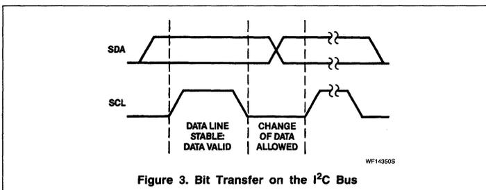
Figure 3. Bit Transfer on the I<sup>2</sup>C Bus
