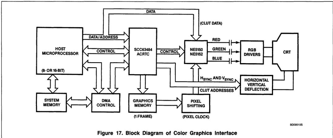
Figure 17. Block Diagram of Color Graphics Interface
