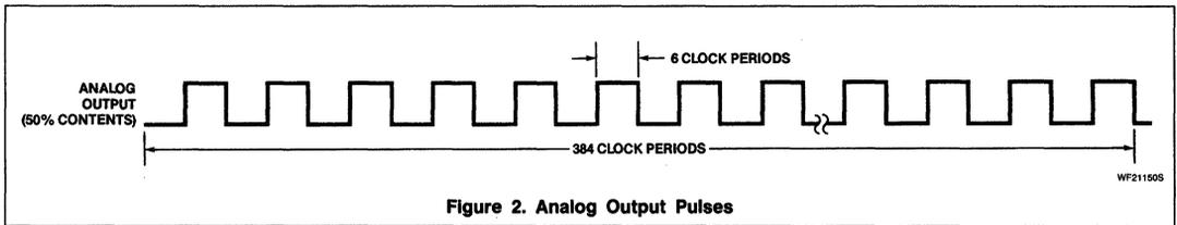
Figure 2. Analog Output Pulses
