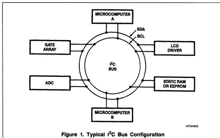
Figure 1. Typical I<sup>2</sup>C Bus Configuration
