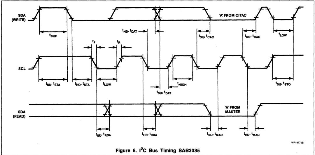
Figure 6. I<sup>2</sup>C Bus Timing SAB3035
