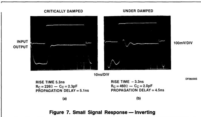
Figure 7. Small Signal Response — Inverting
