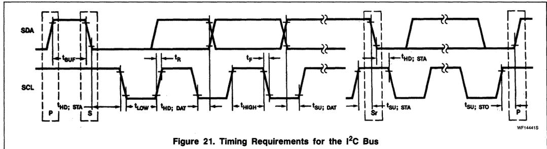
Figure 21. Timing Requirements for the I<sup>2</sup>C Bus
