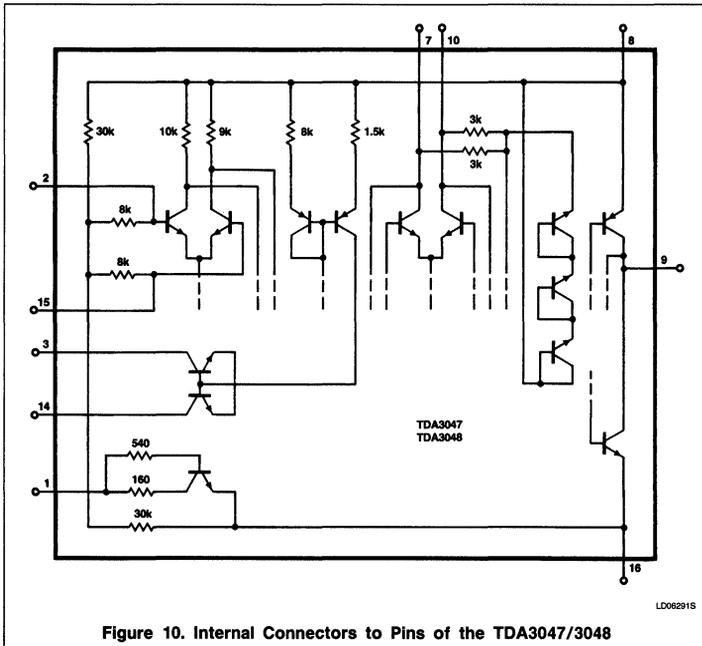
Figure 10. Internal Connectors to Pins of the TDA3047/3048
