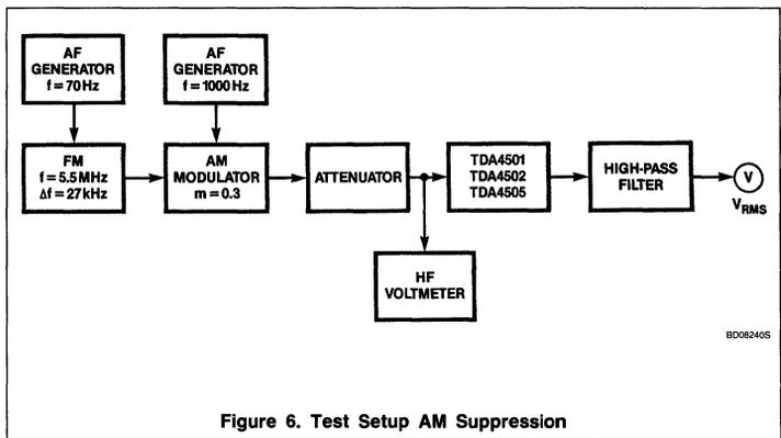
Figure 6. Test Setup AM Suppression
