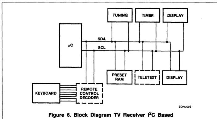
Figure 6. Block Diagram TV Receiver I<sup>2</sup>C Based
