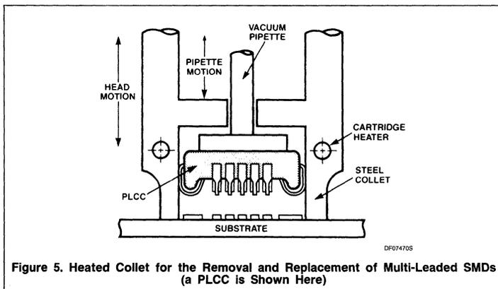
Figure 5. Heated Collet for the Removal and Replacement of Multi-Leaded SMDs (a PLCC is Shown Here)
