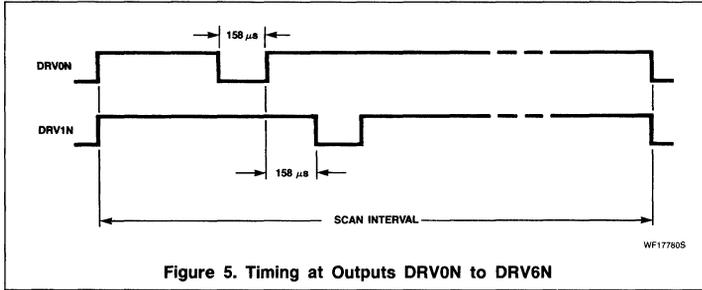
Figure 5. Timing at Outputs DRV0N to DRV6N
