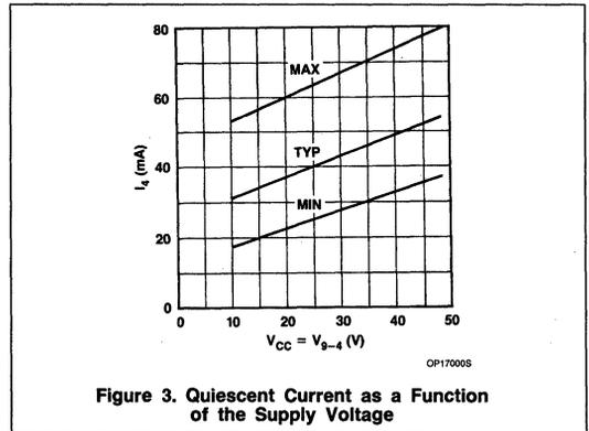
Figure 3. Quiescent Current as a Function of the Supply Voltage
