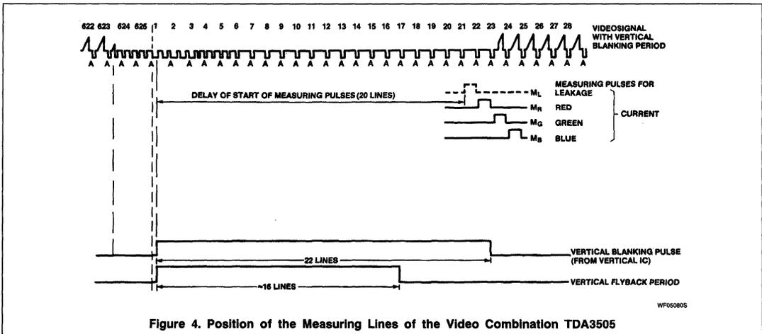
Figure 4. Position of the Measuring Lines of the Video Combination TDA3505
