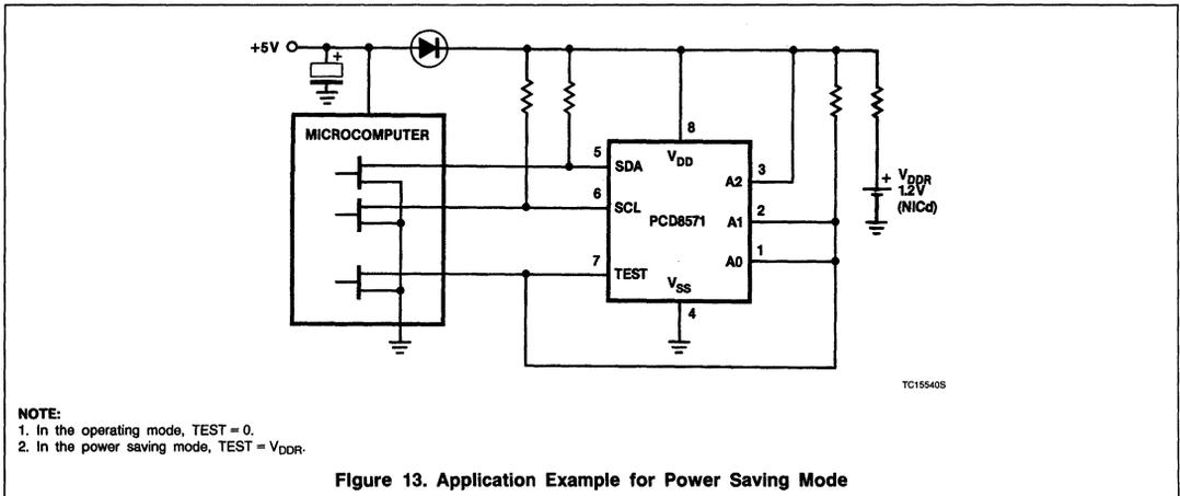
Figure 13. Application Example for Power Saving Mode
