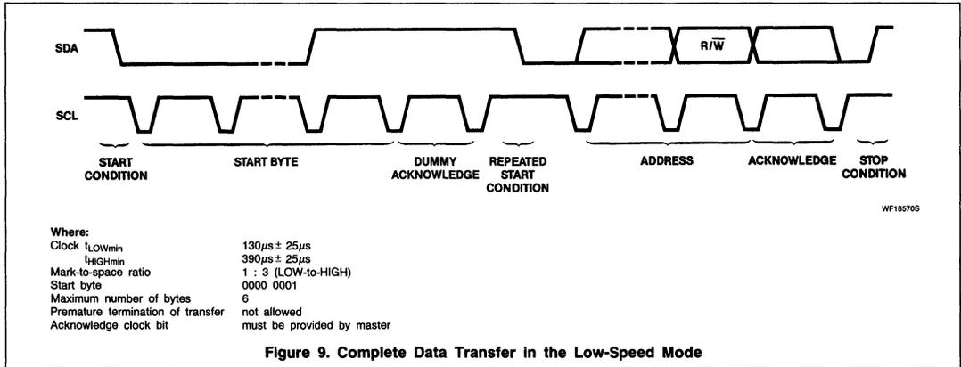
Figure 9. Complete Data Transfer in the Low-Speed Mode
