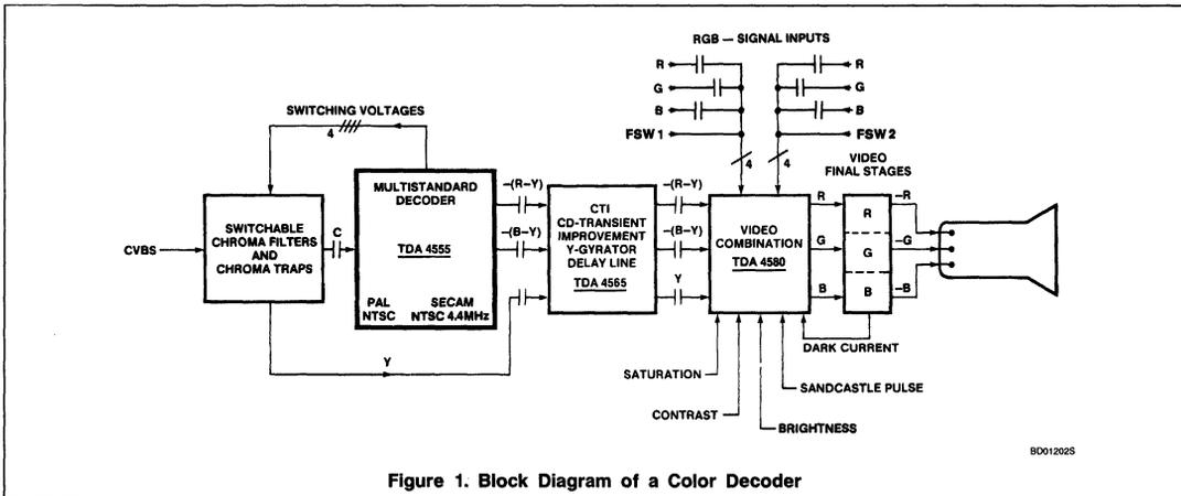
Figure 1. Block Diagram of a Color Decoder
