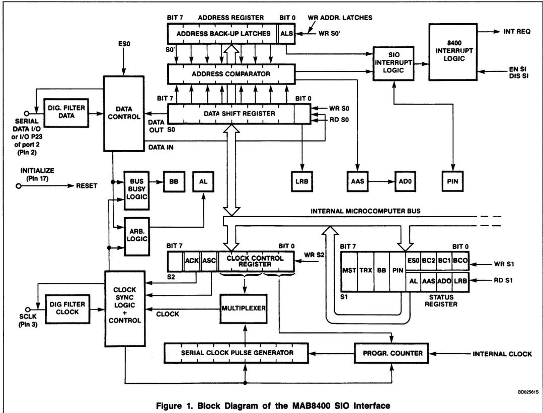
Figure 1. Block Diagram of the MAB8400 SIO Interface
