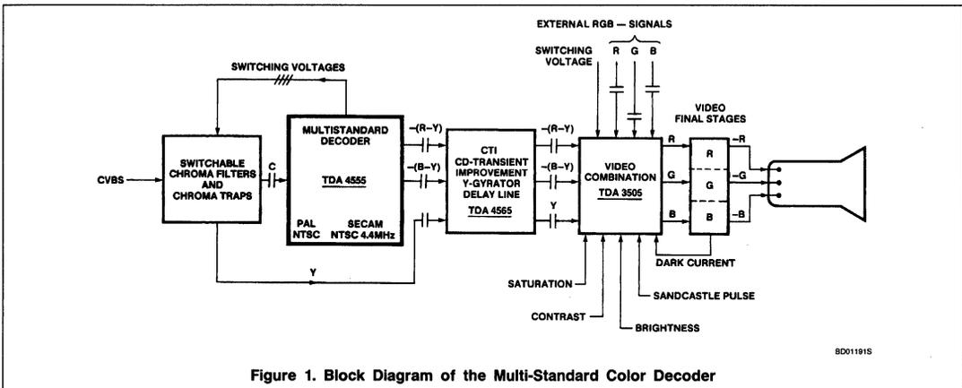
Figure 1. Block Diagram of the Multi-Standard Color Decoder
