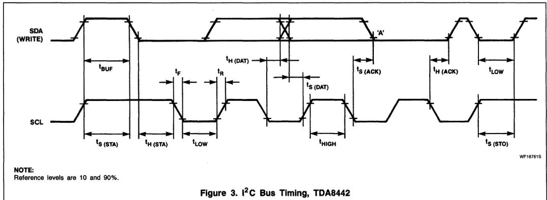
Figure 3. I<sup>2</sup>C Bus Timing, TDA8442
