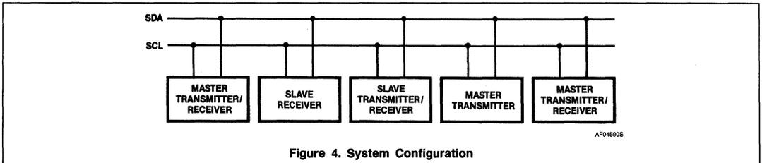
Figure 4. System Configuration
