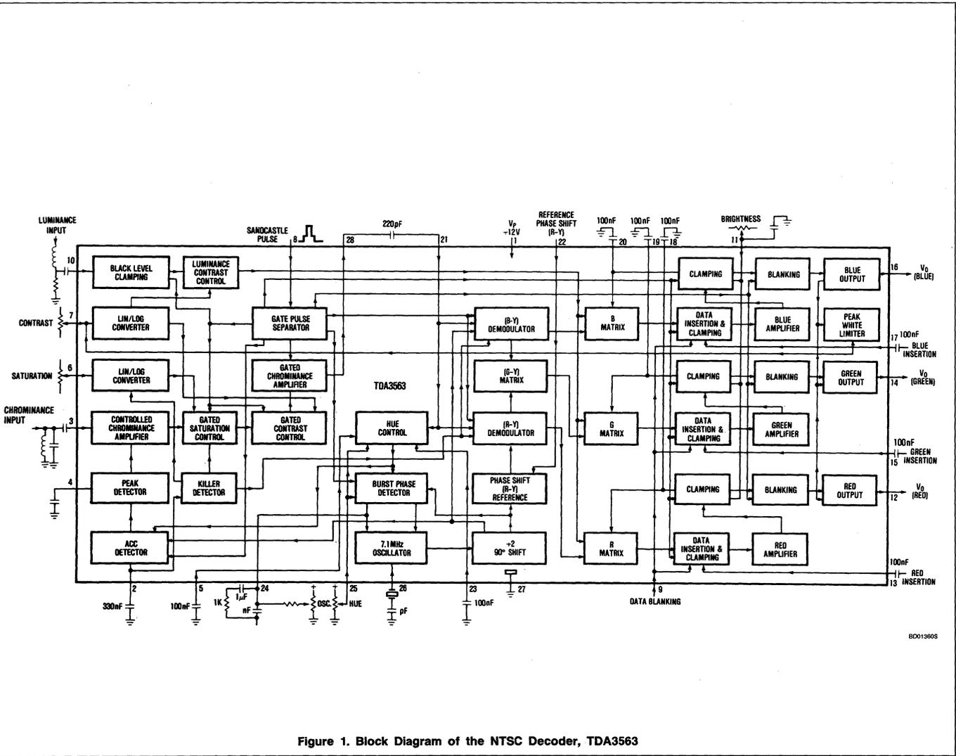
Figure 1. Block Diagram of the NTSC Decoder, TDA3563
