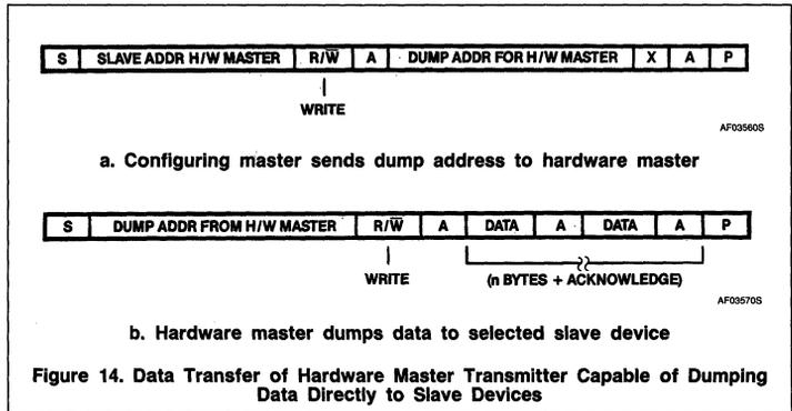
Figure 14. Data Transfer of Hardware Master Transmitter Capable of Dumping Data Directly to Slave Devices
