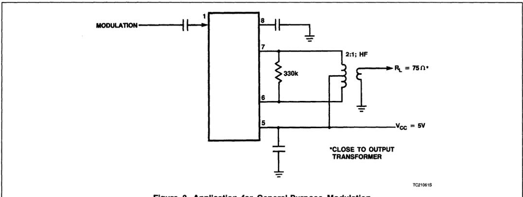
Figure 3. Application for General-Purpose Modulation
