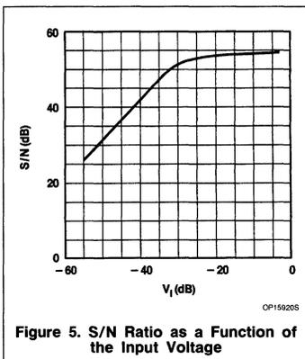
Figure 5. S/N Ratio as a Function of the Input Voltage
