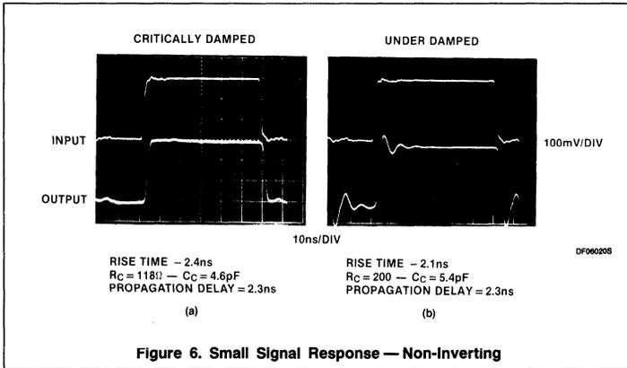
Figure 6. Small Signal Response — Non-Inverting
