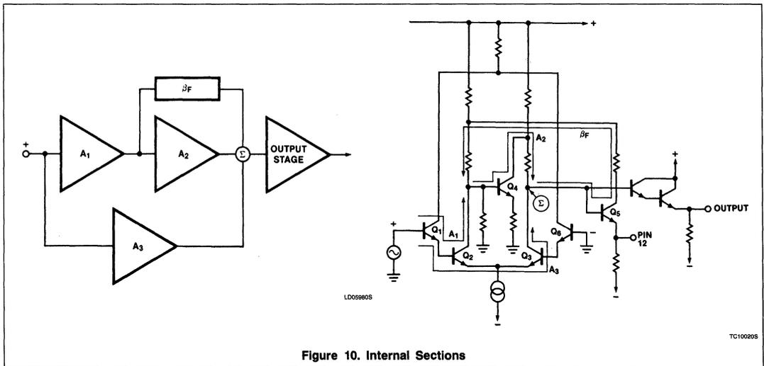
Figure 10. Internal Sections
