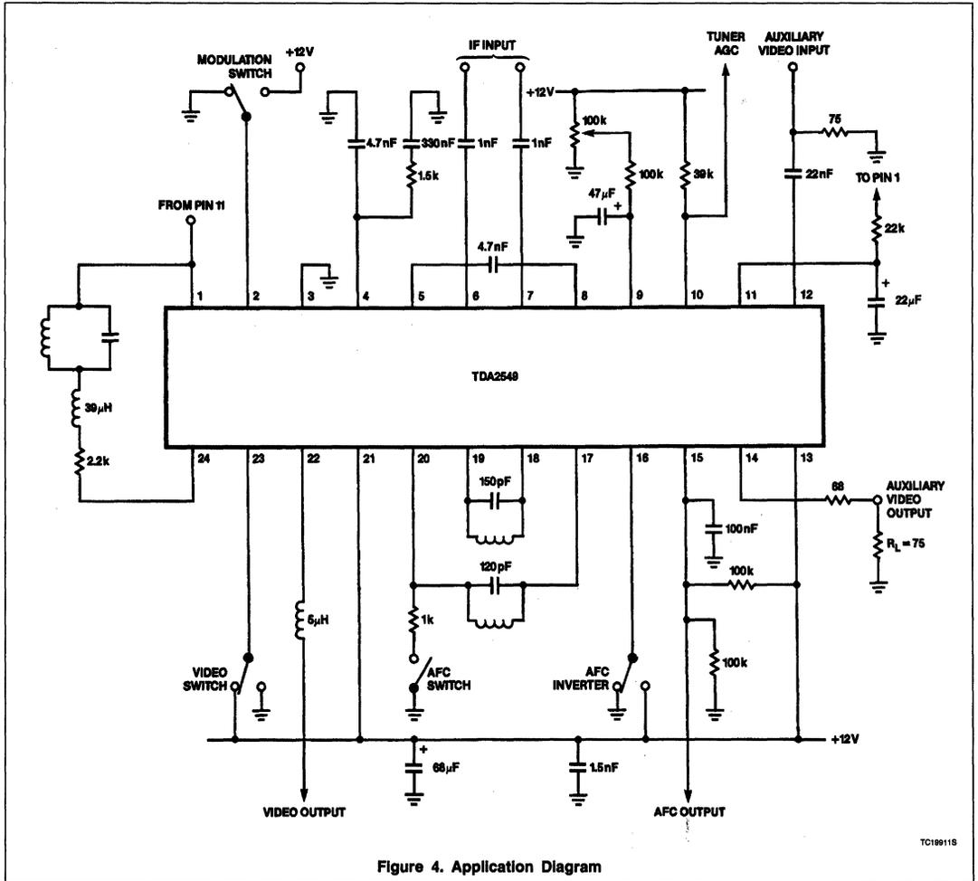
Figure 4. Application Diagram
