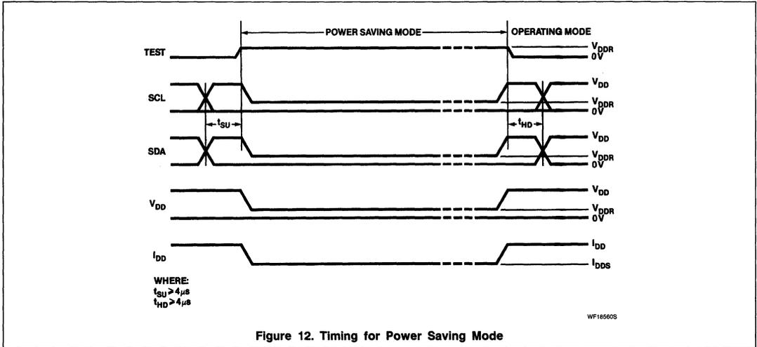
Figure 12. Timing for Power Saving Mode
