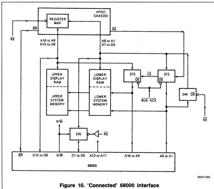
Figure 10. 'Connected' 68000 Interface
