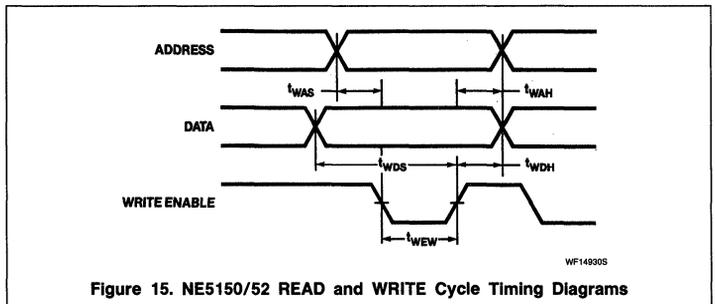
Figure 15. NE5150/52 READ and WRITE Cycle Timing Diagrams
