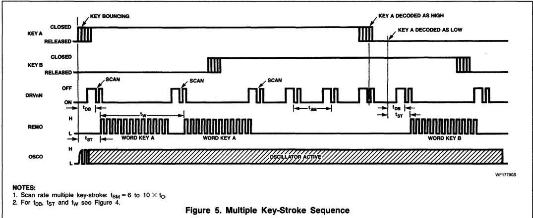
Figure 5. Multiple Key-Stroke Sequence
