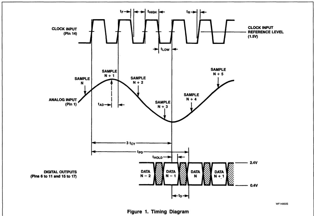
Figure 1. Timing Diagram
