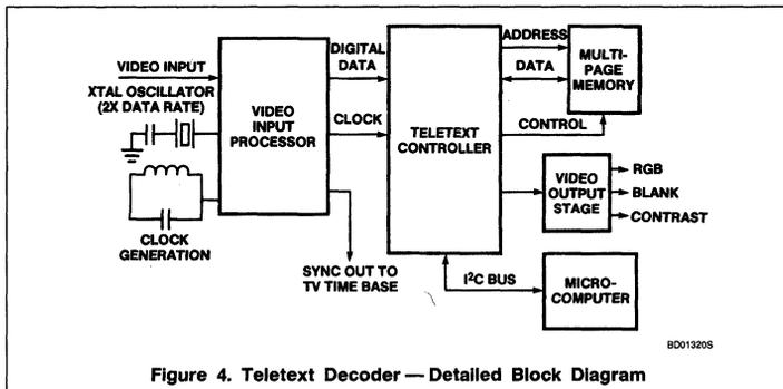
Figure 4. Teletext Decoder — Detailed Block Diagram
