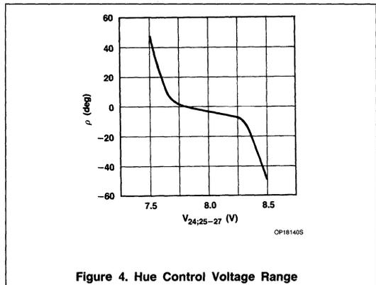
Figure 4. Hue Control Voltage Range
