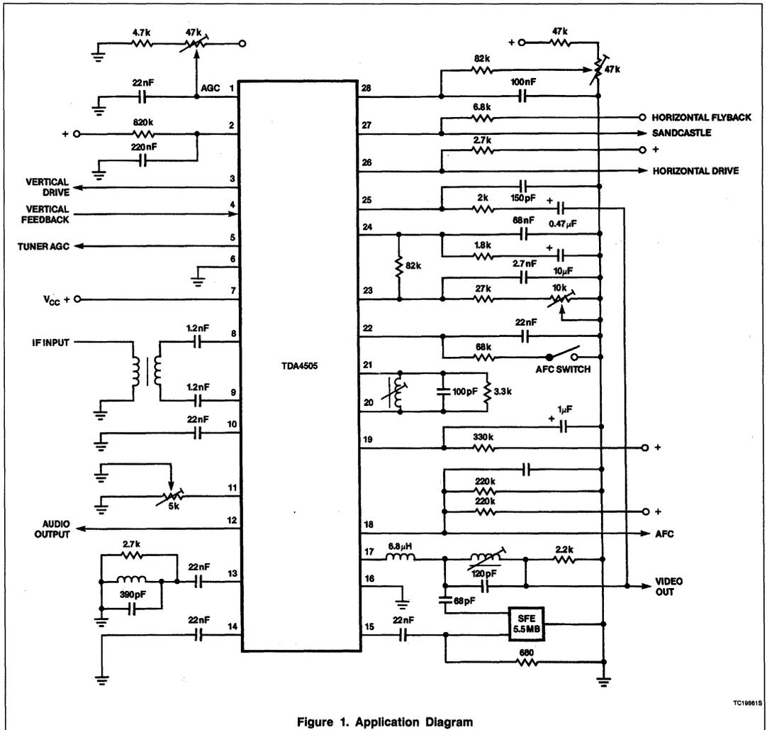
Figure 1. Application Diagram
