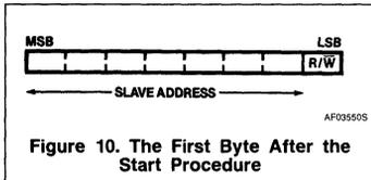
Figure 10. The First Byte After the Start Procedure
