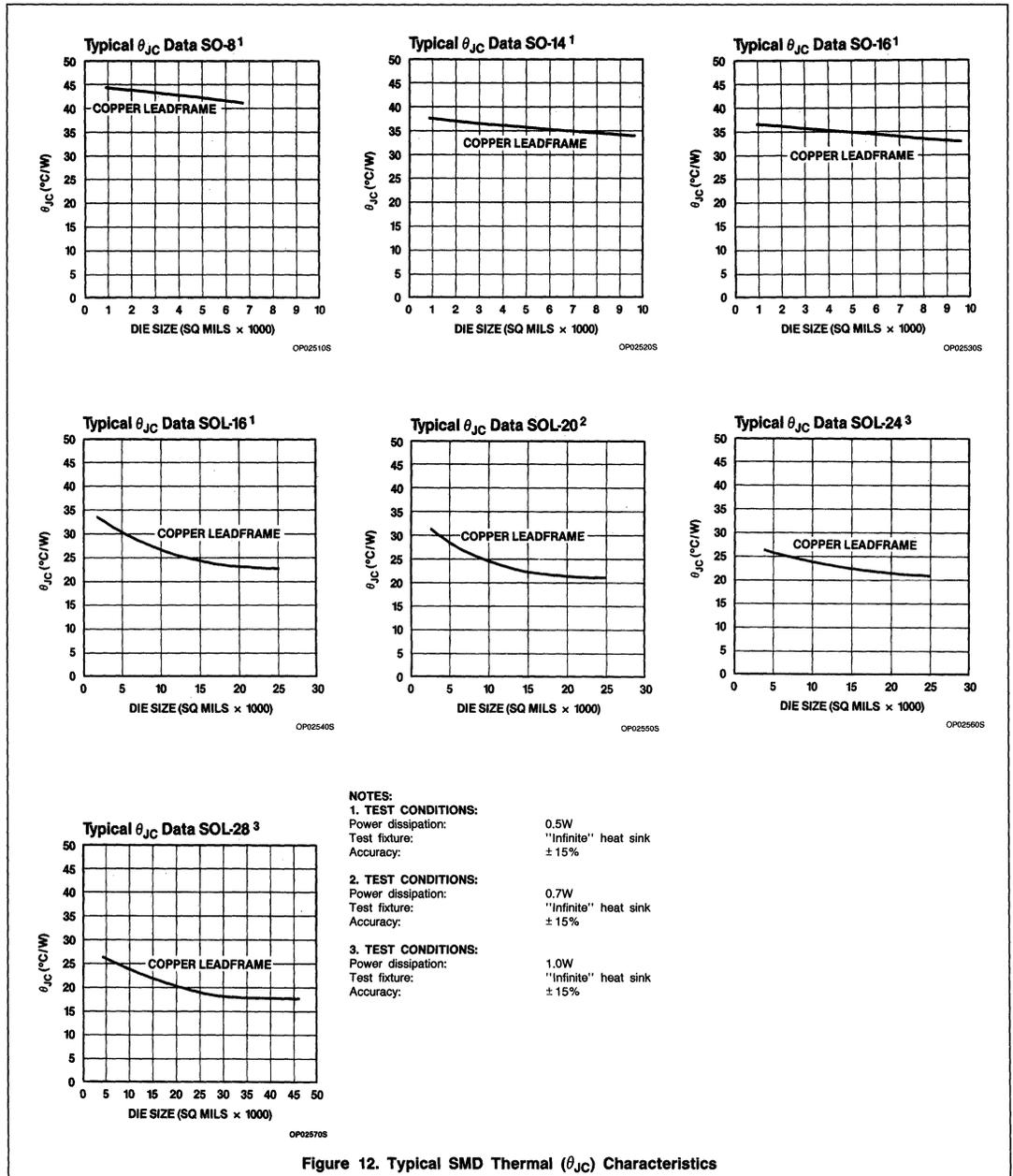
Figure 12. Typical SMD Thermal ( $\theta_{JC}$ ) Characteristics
