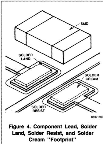
**Figure 4. Component Lead, Solder Land, Solder Resist, and Solder Cream "Footprint"**
