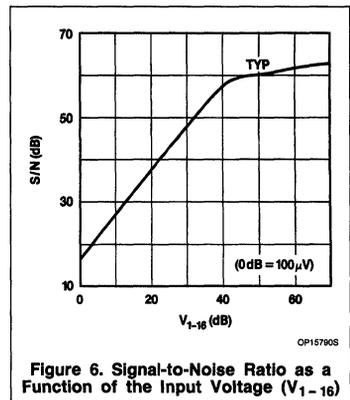
Figure 6. Signal-to-Noise Ratio as a Function of the Input Voltage ( $V_{1-16}$ )
