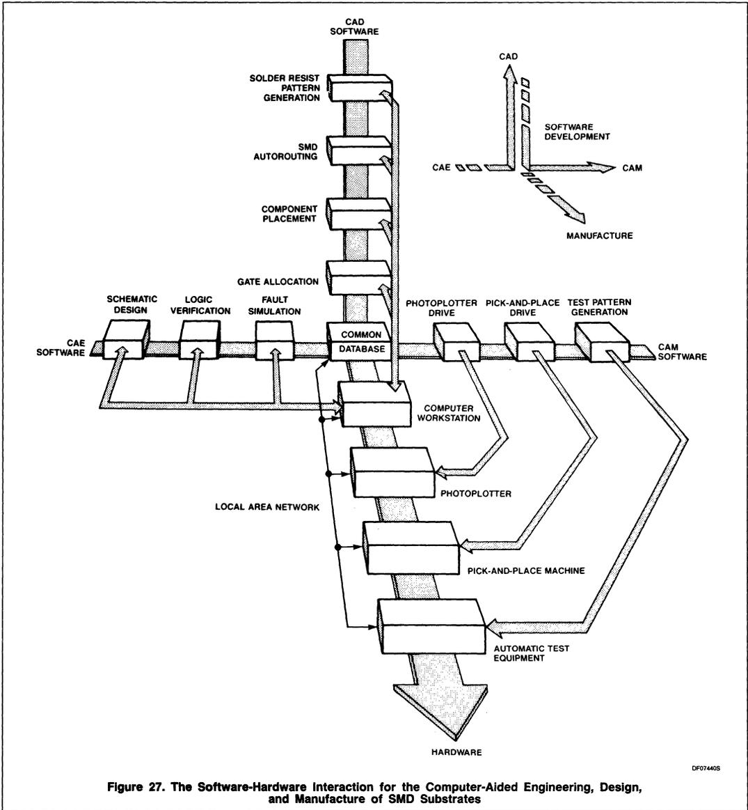
Figure 27. The Software-Hardware Interaction for the Computer-Aided Engineering, Design, and Manufacture of SMD Substrates
