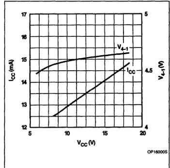
Figure 8. Supply Current and the Reference Voltage at Pin 4 as a Function of Supply Voltage
