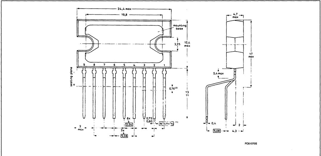
**12-PIN PLASTIC DIP WITH METAL COOLING FIN (SOT-150)**
