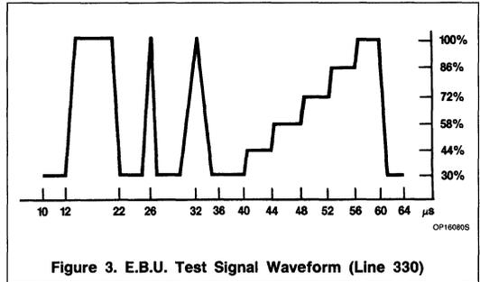
Figure 3. E.B.U. Test Signal Waveform (Line 330)
