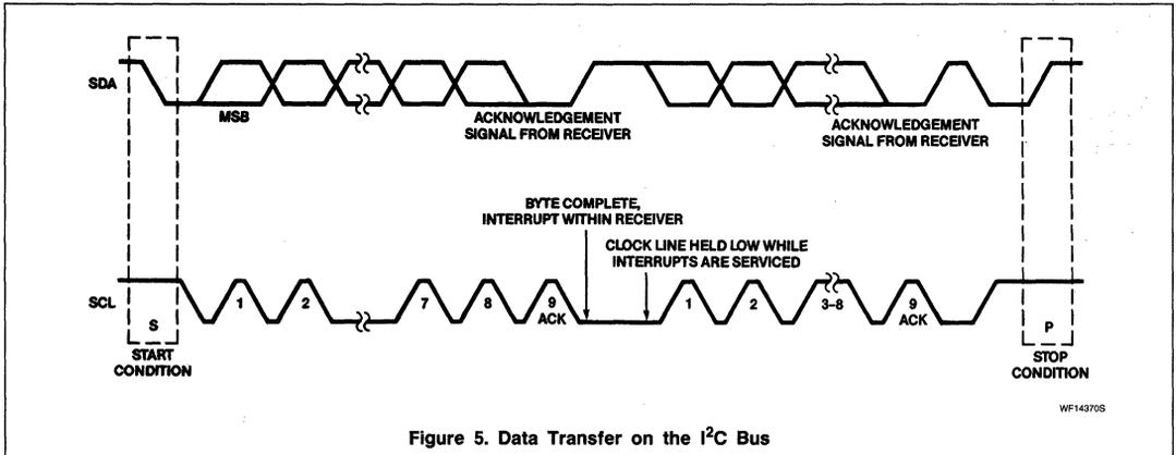
Figure 5. Data Transfer on the I<sup>2</sup>C Bus
