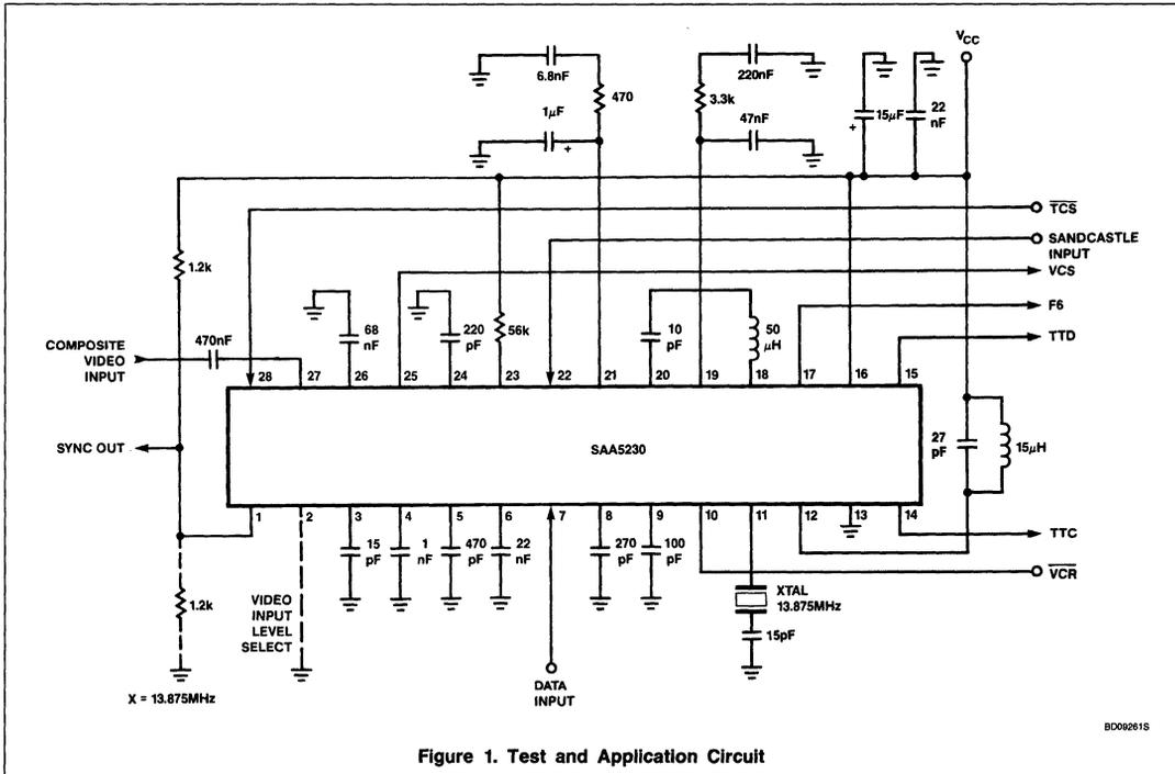
Figure 1. Test and Application Circuit
