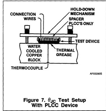
Figure 7.  $\theta_{JC}$  Test Setup With PLCC Device
