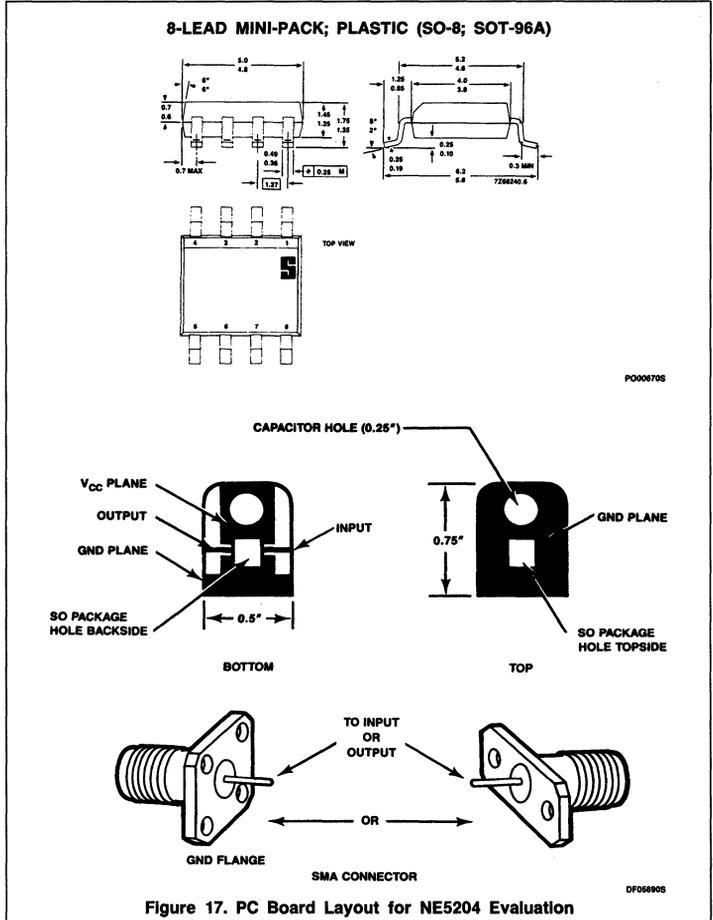
Figure 17. PC Board Layout for NE5204 Evaluation
