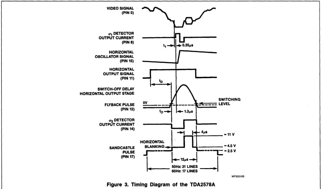
Figure 3. Timing Diagram of the TDA2578A
