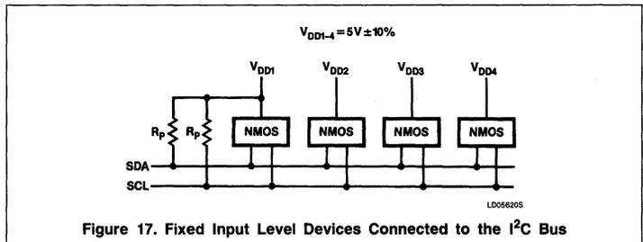
Figure 17. Fixed Input Level Devices Connected to the I<sup>2</sup>C Bus
