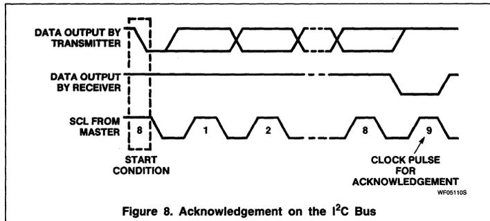
Figure 8. Acknowledgement on the I<sup>2</sup>C Bus
