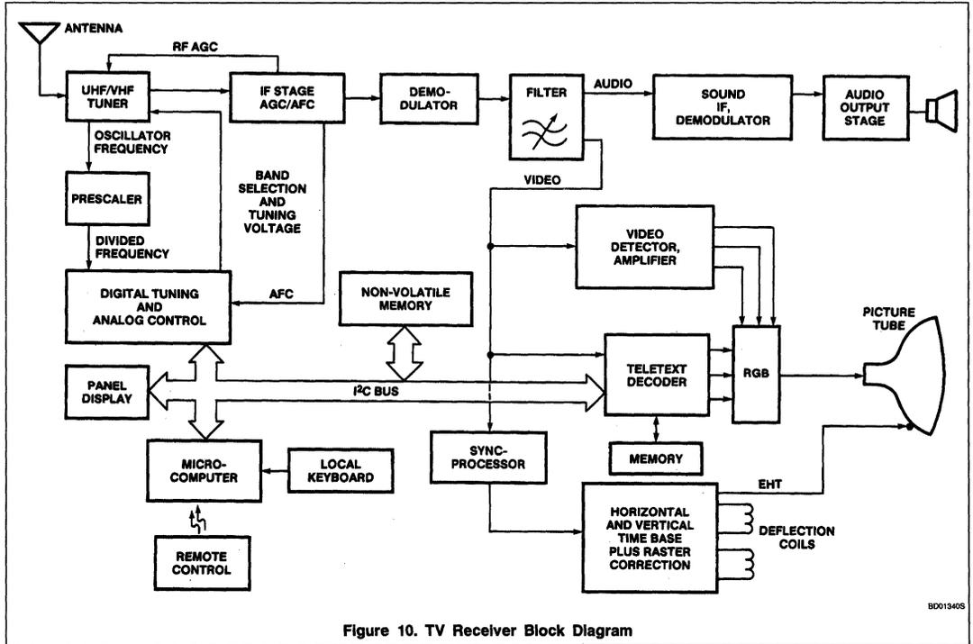
Figure 10. TV Receiver Block Diagram
