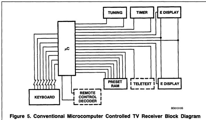
Figure 5. Conventional Microcomputer Controlled TV Receiver Block Diagram
