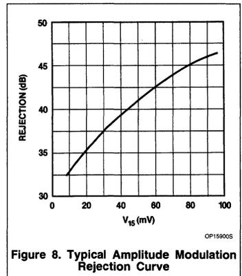
Figure 8. Typical Amplitude Modulation Rejection Curve
