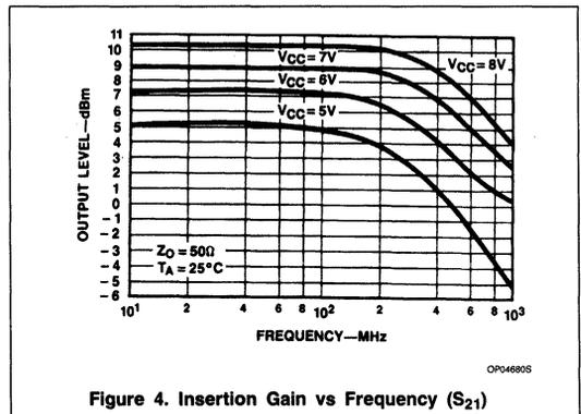
Figure 4. Insertion Gain vs Frequency ( $S_{21}$ )
