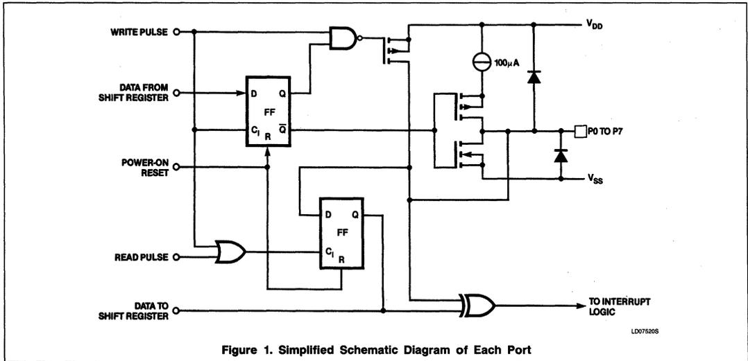
Figure 1. Simplified Schematic Diagram of Each Port
