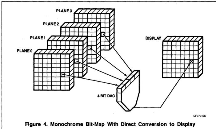
Figure 4. Monochrome Bit-Map With Direct Conversion to Display
