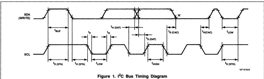
Figure 1. I<sup>2</sup>C Bus Timing Diagram
