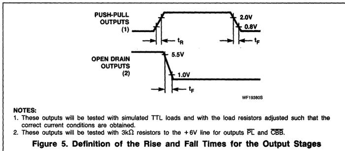
Figure 5. Definition of the Rise and Fall Times for the Output Stages
