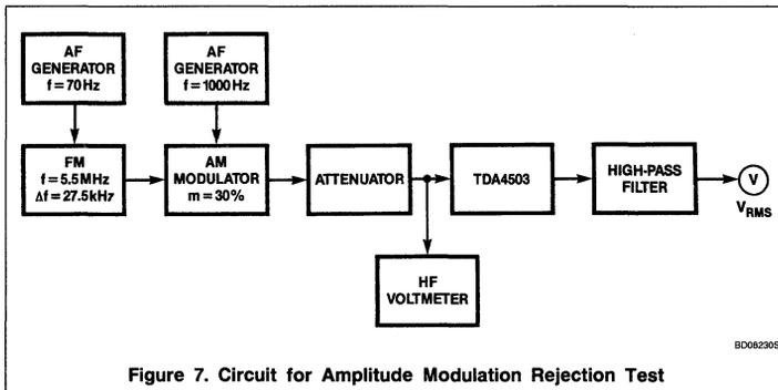
Figure 7. Circuit for Amplitude Modulation Rejection Test
