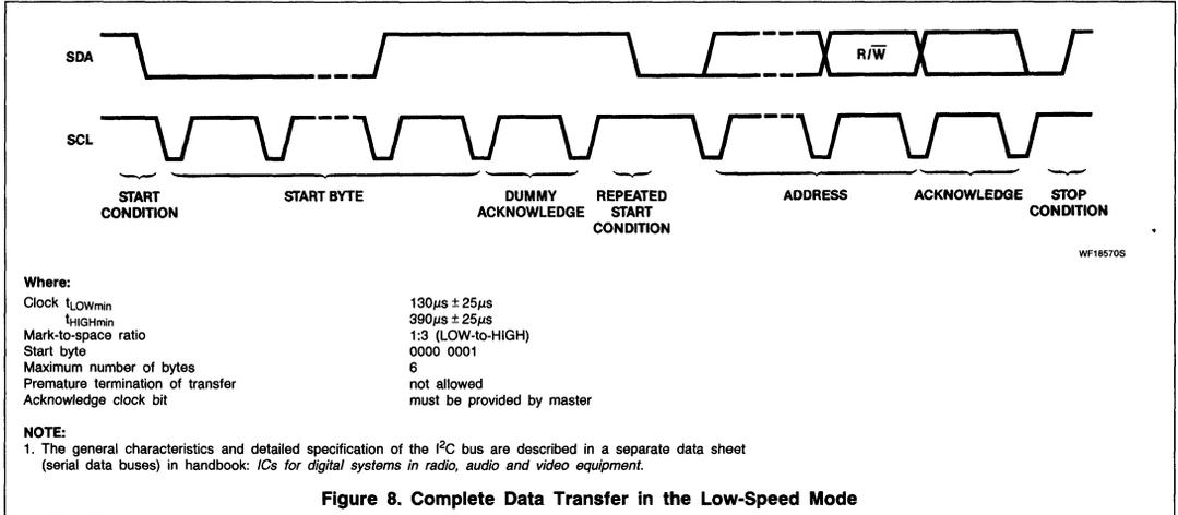
Figure 8. Complete Data Transfer in the Low-Speed Mode
