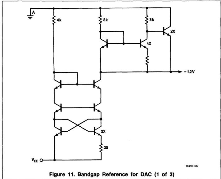
Figure 11. Bandgap Reference for DAC (1 of 3)
