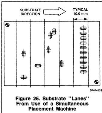
Placement of the 10 components in the lane on the right of the substrate shown will require a machine with 10 placement modules (or ten passes beneath a single placement module), an inefficient process considering that there are no more than three SMDs in any other lane.
