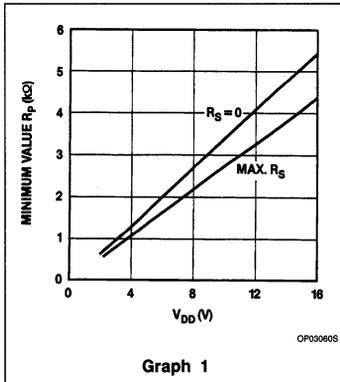
The desired noise margin of 0.1  $V_{DD}$  for the low level limits the maximum value of  $R_S$ .
