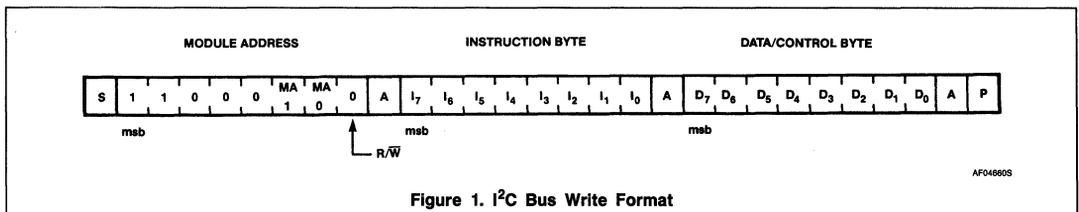
Figure 1. I<sup>2</sup>C Bus Write Format
