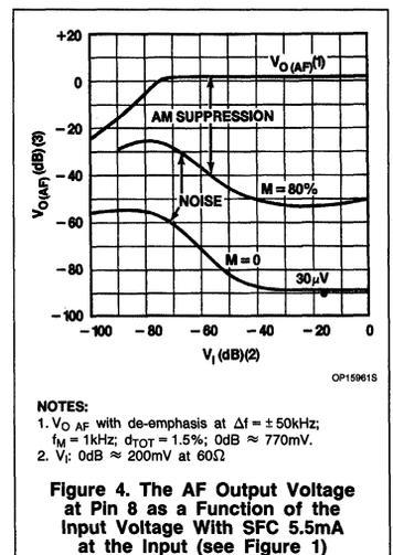
Figure 4. The AF Output Voltage at Pin 8 as a Function of the Input Voltage With SFC 5.5mA at the Input (see Figure 1)
