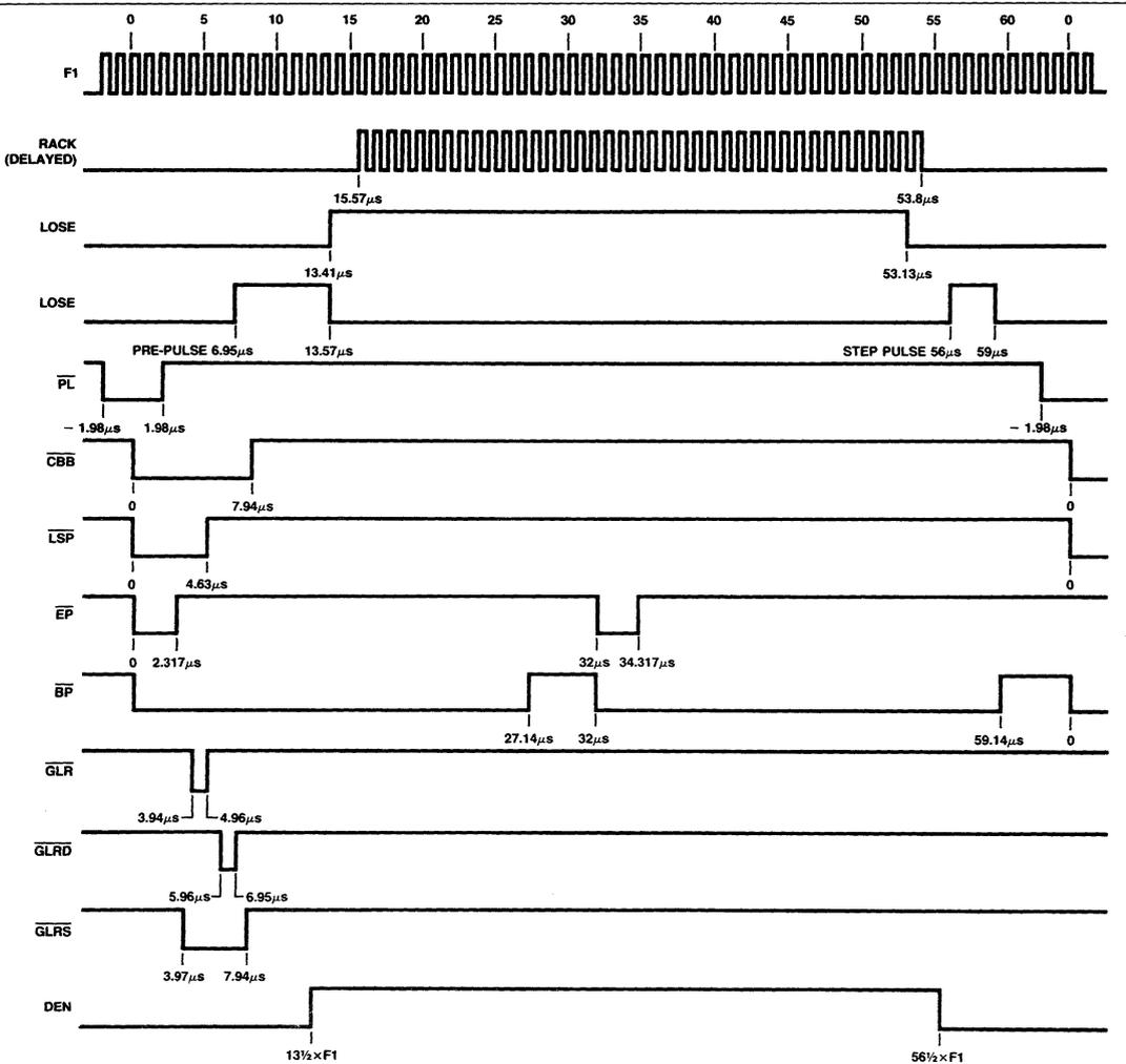
Figure 1. Timing Diagram Showing the Line-Rate Signals
