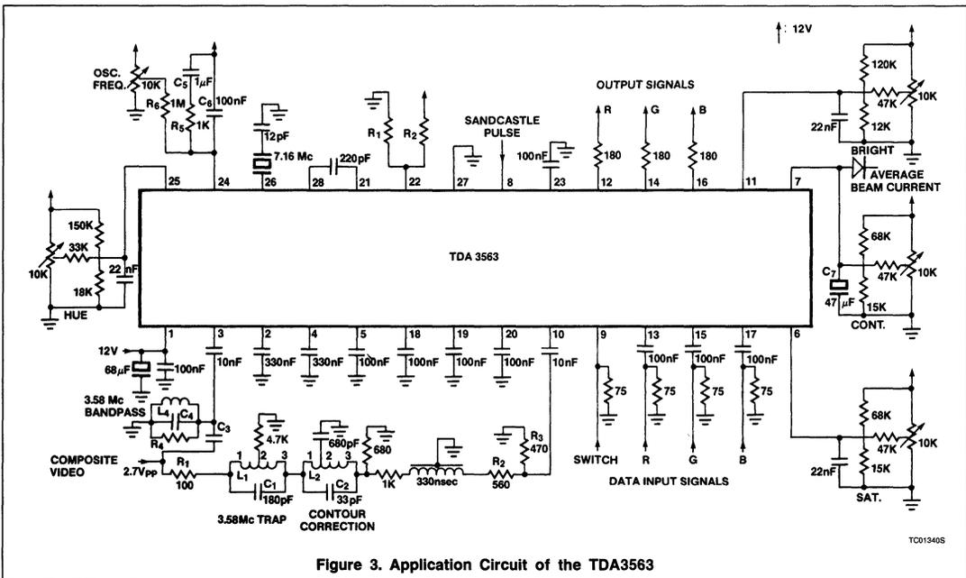
Figure 3. Application Circuit of the TDA3563
