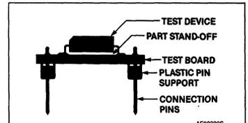
Figure 5. Cross-Section of Test Device Soldered to Test Board
