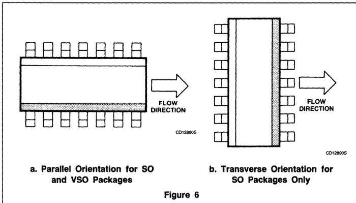
For bonding small outline (SO) ICs to the substrate, two dots of adhesive are sufficient for SO-8, -14, and -16 packages, but the SOL-20, -24, -28, and VSO-40 packages need three dots. The through-tracks (or dummy tracks) must be positioned beneath the IC accordingly to support the adhesive dots.
