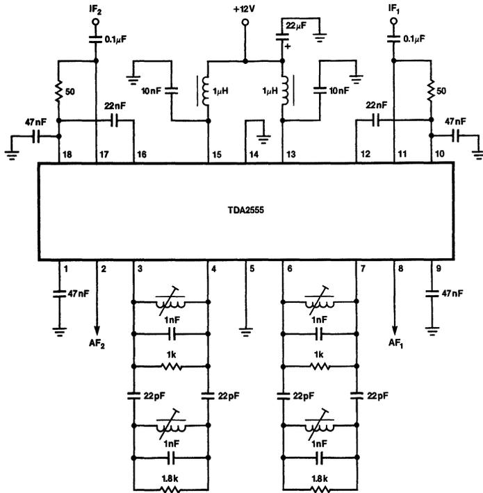
Figure 1. Test Circuit
