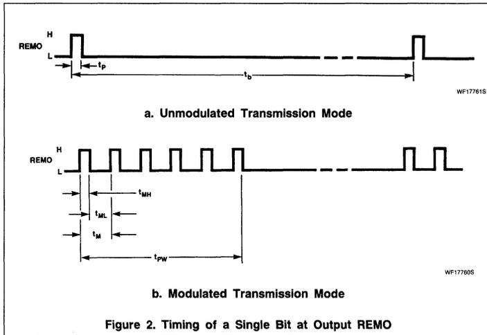
output REMO via the output modulator. After a key is released, the oscillator stops and the circuits return to the standby state to conserve battery power as soon as the output sequence is completed.
