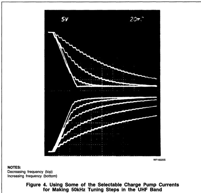
Figure 4. Using Some of the Selectable Charge Pump Currents for Making 50kHz Tuning Steps in the UHF Band
