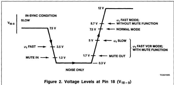
**Figure 2. Voltage Levels at Pin 18 ( $V_{18-9}$ )**
