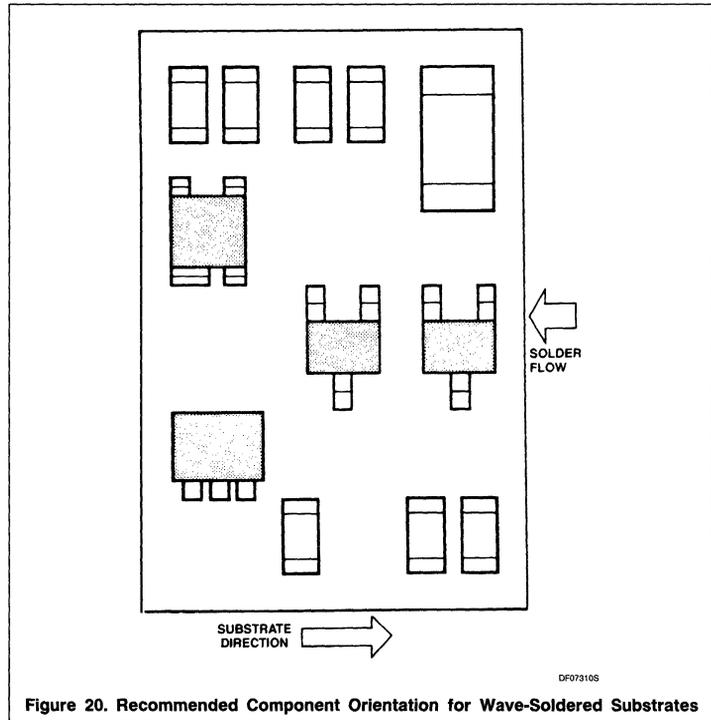
Figure 20. Recommended Component Orientation for Wave-Soldered Substrates
