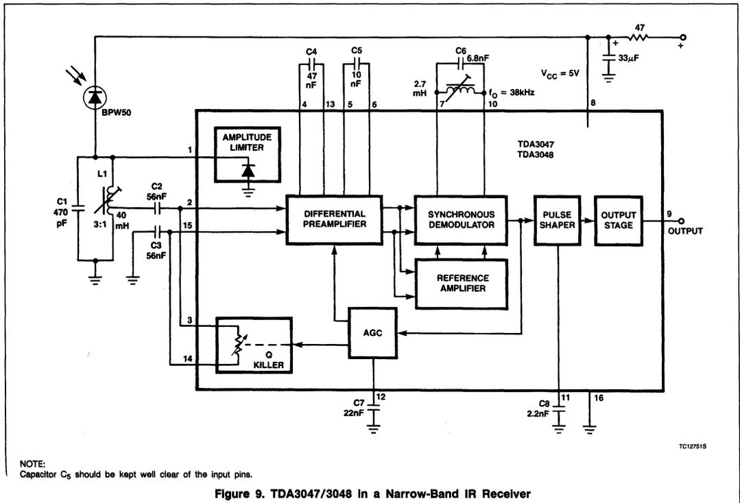
Figure 9. TDA3047/3048 in a Narrow-Band IR Receiver
