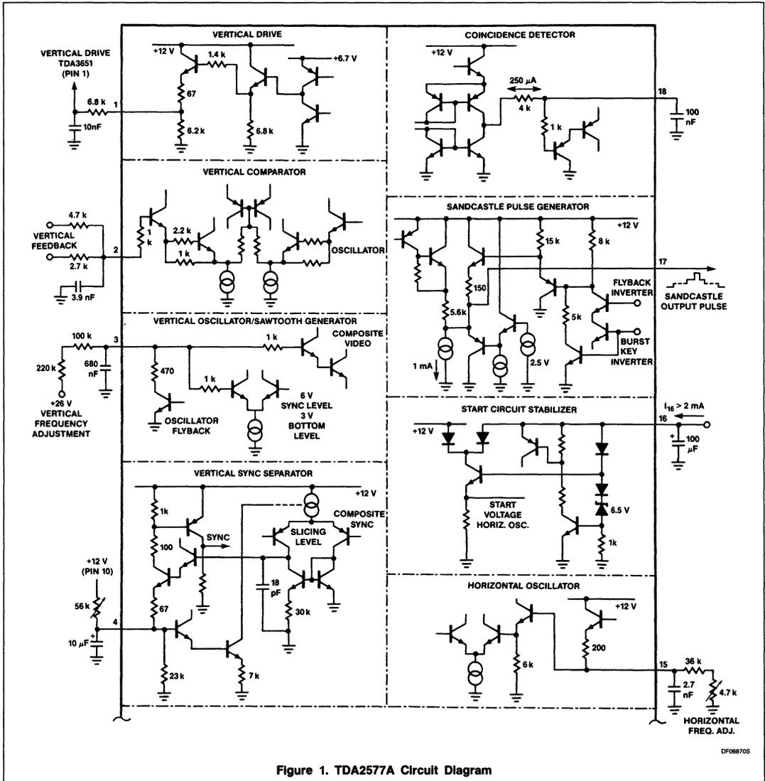
Figure 1. TDA2577A Circuit Diagram
