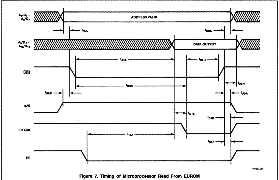
Figure 7. Timing of Microprocessor Read From EUROM
