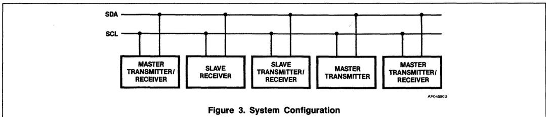
Figure 3. System Configuration
