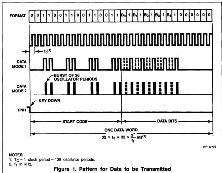
With a tolerance of  $\pm 10\%$  on the oscillator frequency ( $f_T$ ) of the transmitter, the receiver oscillator frequency ( $f_R = 3 \times f_T$ ) must be kept constant with a tolerance of  $\pm 20\%$ .
