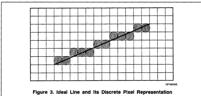
Figure 3. Ideal Line and Its Discrete Pixel Representation
