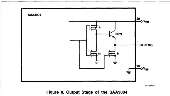
Figure 8. Output Stage of the SAA3004
