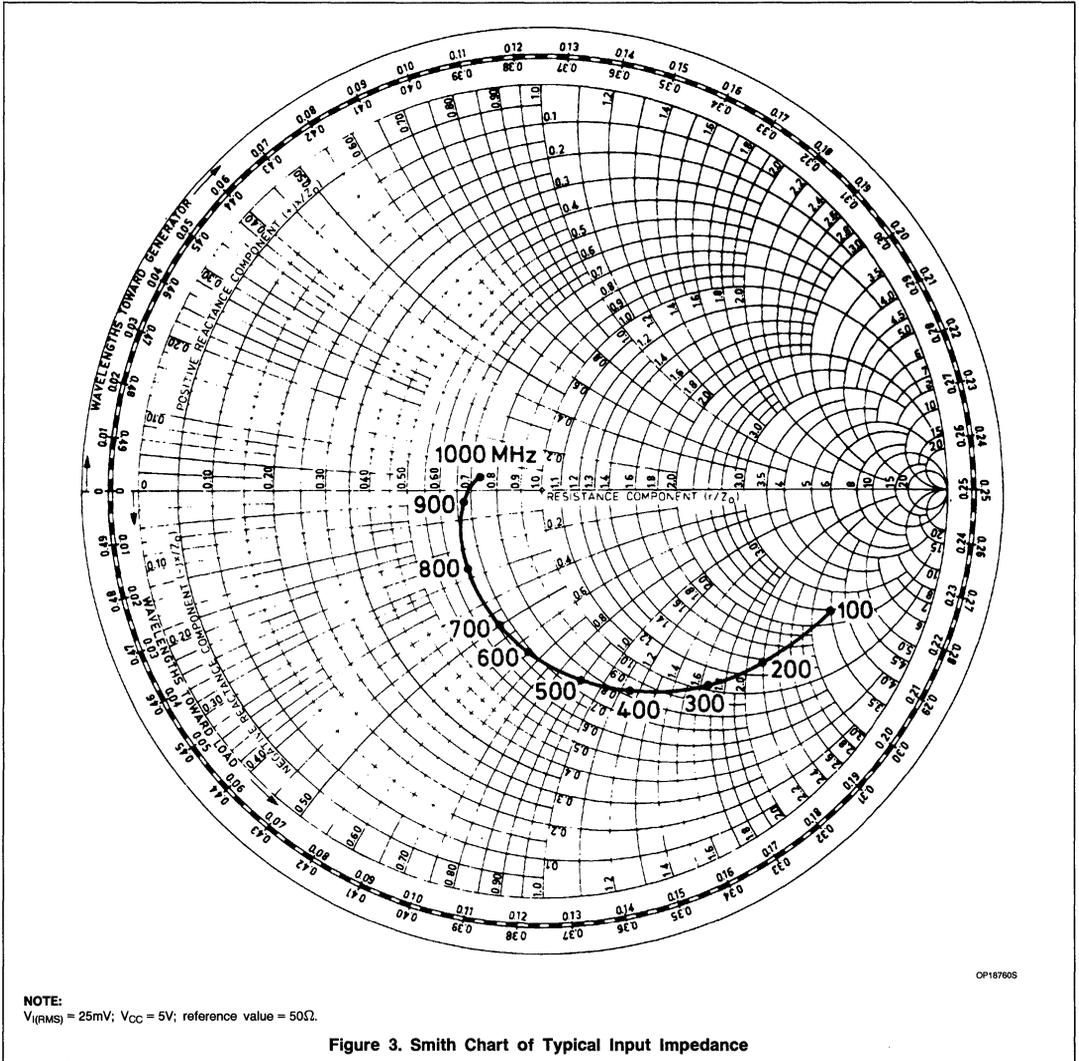
Figure 3. Smith Chart of Typical Input Impedance
