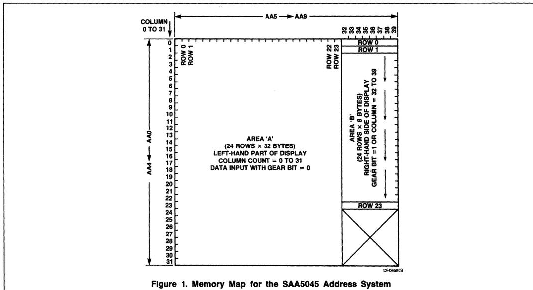
Figure 1. Memory Map for the SAA5045 Address System
