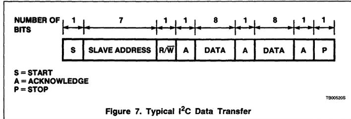
Figure 7. Typical I<sup>2</sup>C Data Transfer
