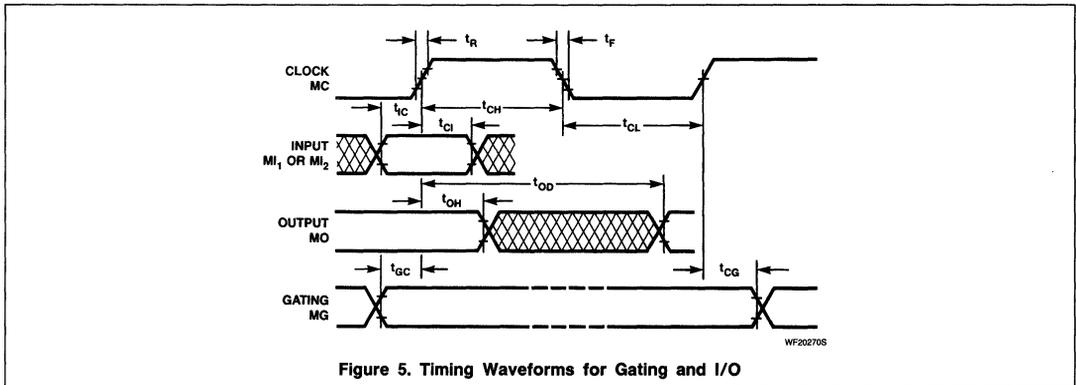
Figure 5. Timing Waveforms for Gating and I/O
