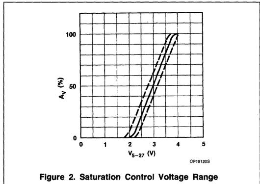
Figure 2. Saturation Control Voltage Range
