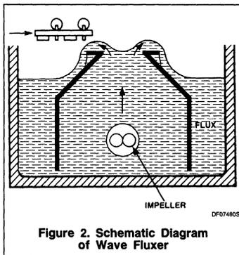
Figure 2. Schematic Diagram of Wave Fluxer
