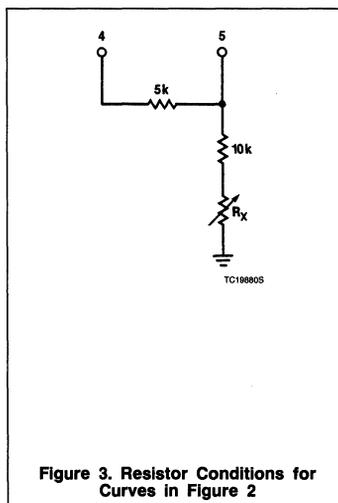
Figure 3. Resistor Conditions for Curves in Figure 2
