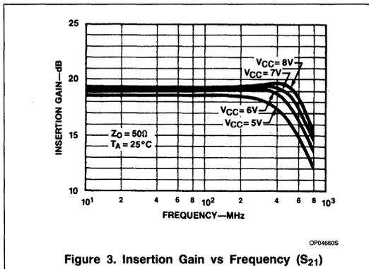
Figure 3. Insertion Gain vs Frequency ( $S_{21}$ )
