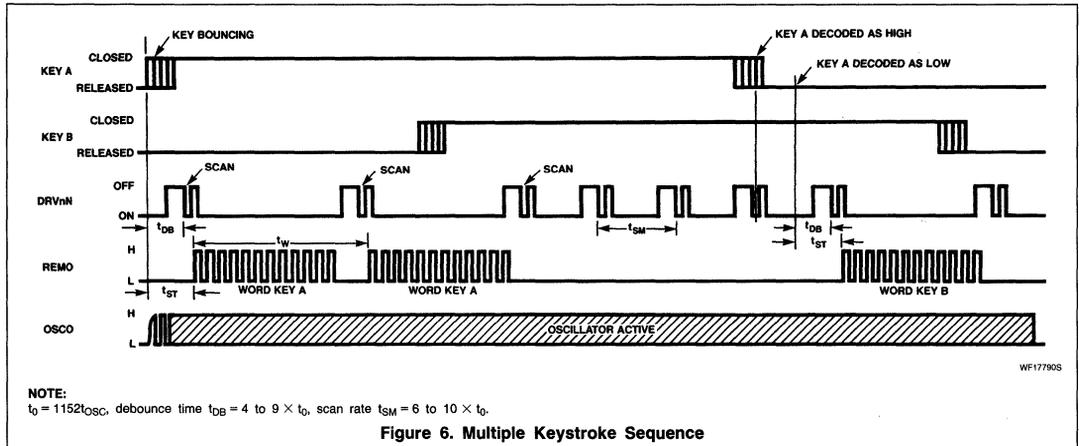
Figure 6. Multiple Keystroke Sequence
