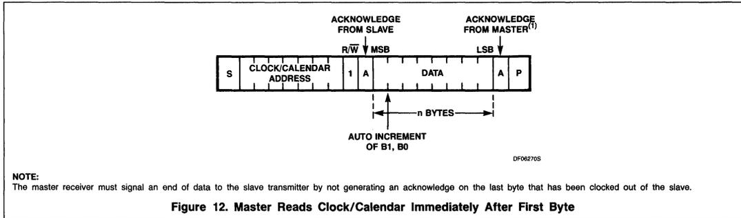
To read the addressed part of the time counter and alarm register, plus information from specified control/status flags, the BCD digits in the DATA byte are organized as shown in Table 7. The status of the MODE-POINTER-WORD concerning the CONTROL-nibble remains unchanged until a write to MODE POINTER condition occurs.
