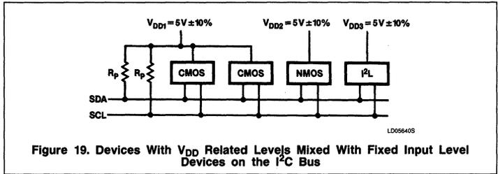
Figure 19. Devices With V<sub>DD</sub> Related Levels Mixed With Fixed Input Level Devices on the I<sup>2</sup>C Bus
