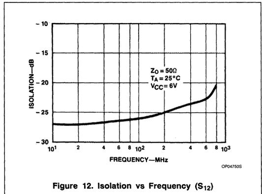
Figure 12. Isolation vs Frequency ( $S_{12}$ )
