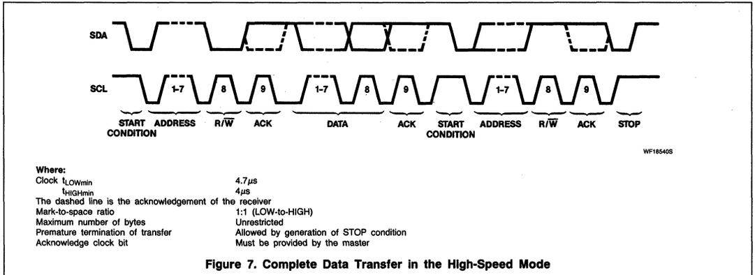
Figure 7. Complete Data Transfer in the High-Speed Mode
