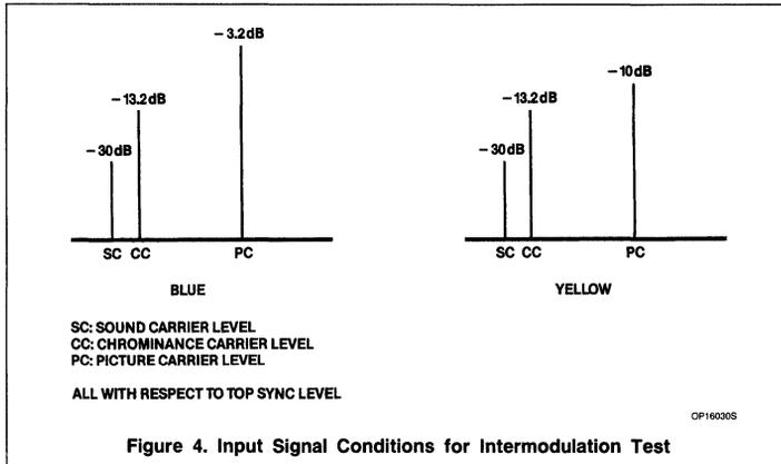
Figure 4. Input Signal Conditions for Intermodulation Test
