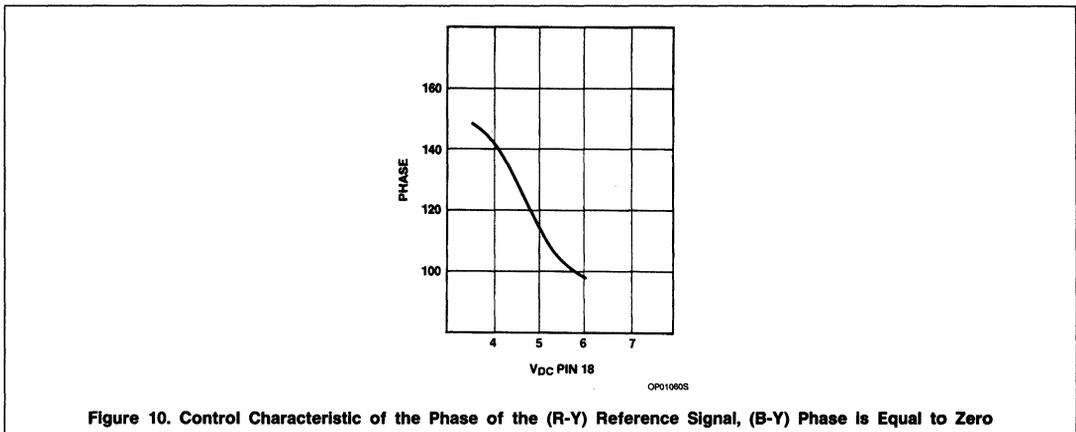
Figure 10. Control Characteristic of the Phase of the (R-Y) Reference Signal, (B-Y) Phase is Equal to Zero
