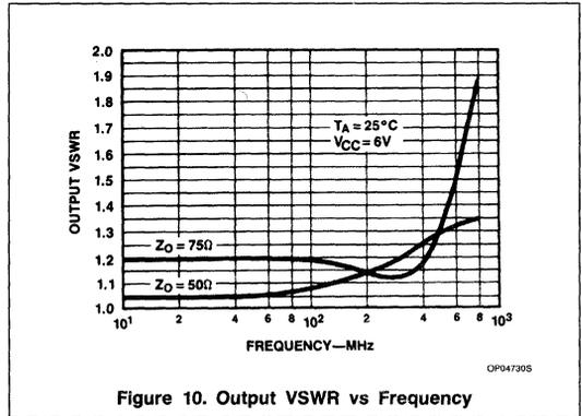
Figure 10. Output VSWR vs Frequency
