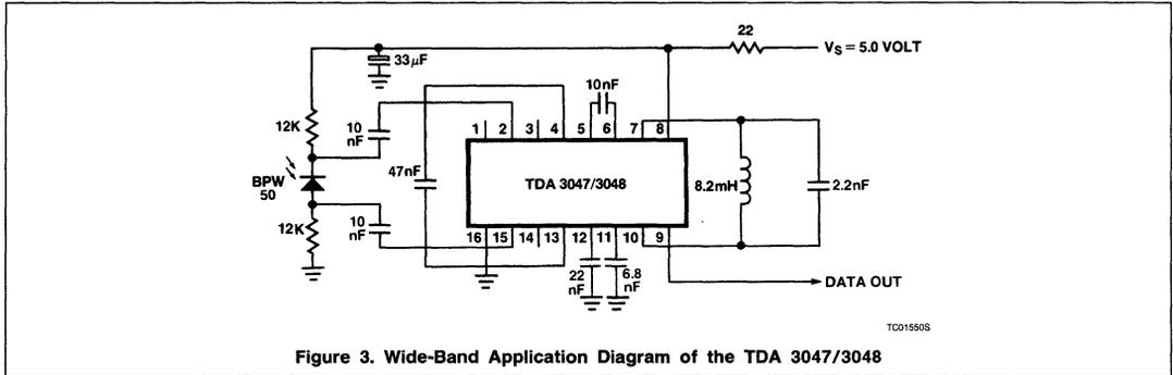
Figure 3. Wide-Band Application Diagram of the TDA 3047/3048
