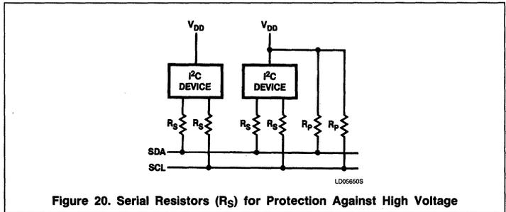
Figure 20. Serial Resistors (R<sub>S</sub>) for Protection Against High Voltage
