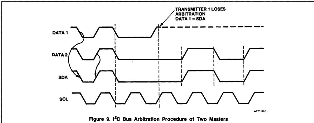
Figure 9. I<sup>2</sup>C Bus Arbitration Procedure of Two Masters
