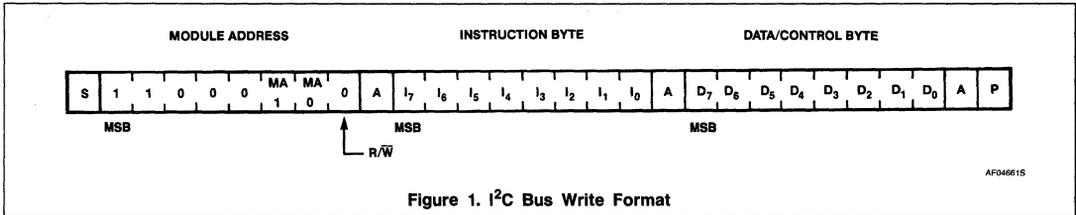
Figure 1. I<sup>2</sup>C Bus Write Format
