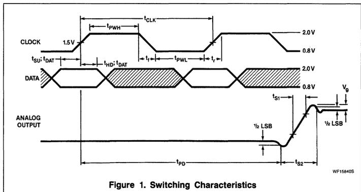
Figure 1. Switching Characteristics
