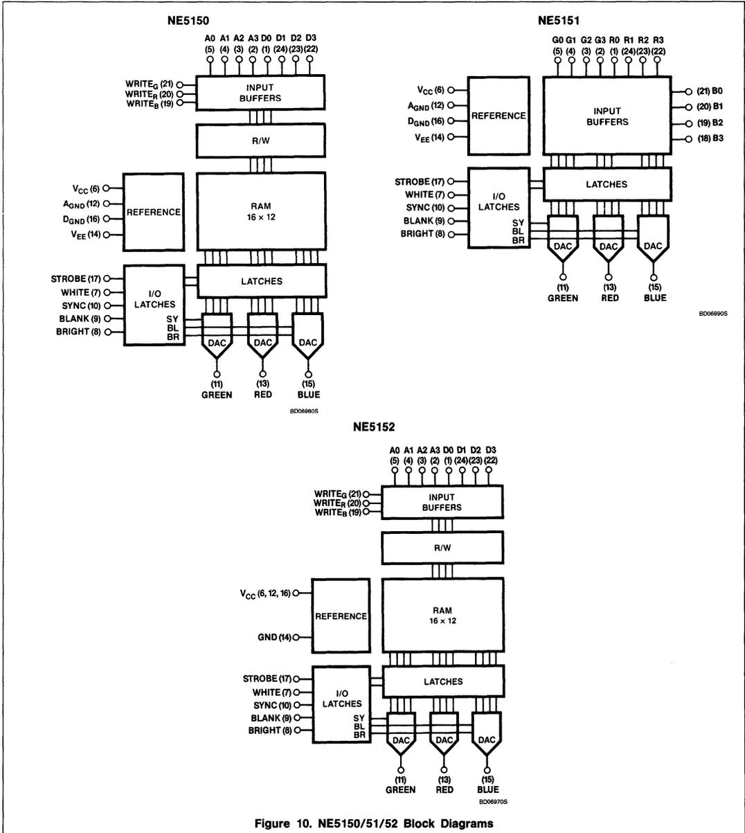
Figure 10. NE5150/51/52 Block Diagrams
