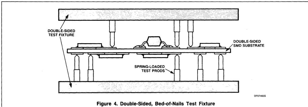
Figure 4. Double-Sided, Bed-of-Nails Test Fixture
