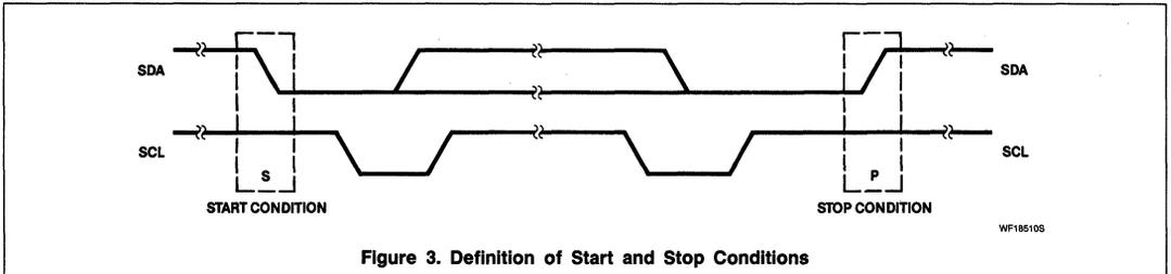
Figure 3. Definition of Start and Stop Conditions
