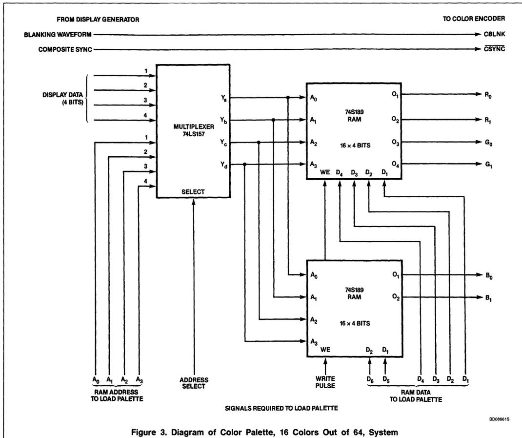
Figure 3. Diagram of Color Palette, 16 Colors Out of 64, System
