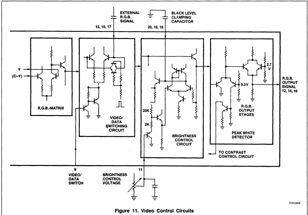
Figure 11. Video Control Circuits
