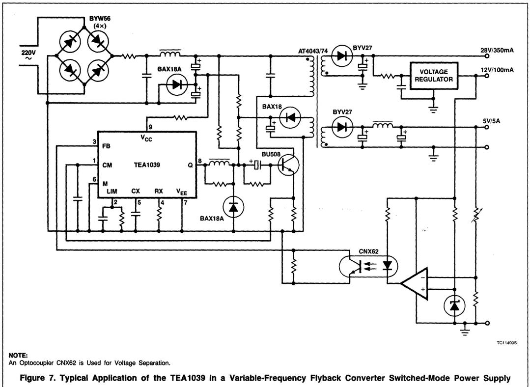
Control Circuit for Switched-Mode Power Supply
