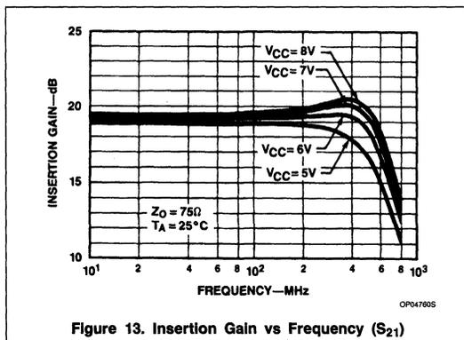
Figure 13. Insertion Gain vs Frequency ( $S_{21}$ )
