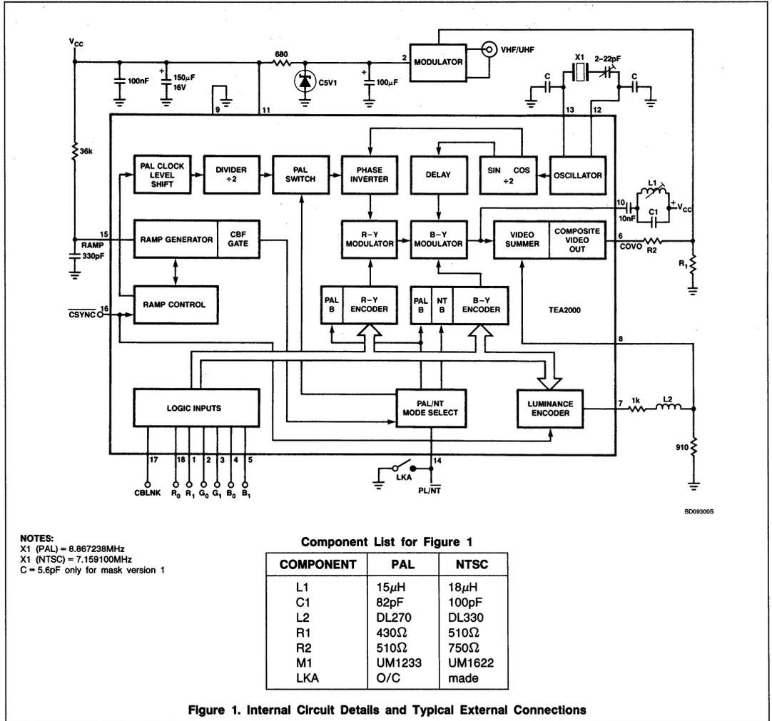
Figure 1. Internal Circuit Details and Typical External Connections
