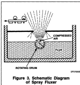
Figure 3. Schematic Diagram of Spray Fluxer
