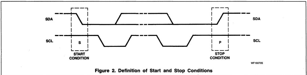
Figure 2. Definition of Start and Stop Conditions
