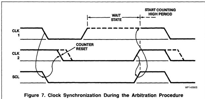
Figure 7. Clock Synchronization During the Arbitration Procedure
