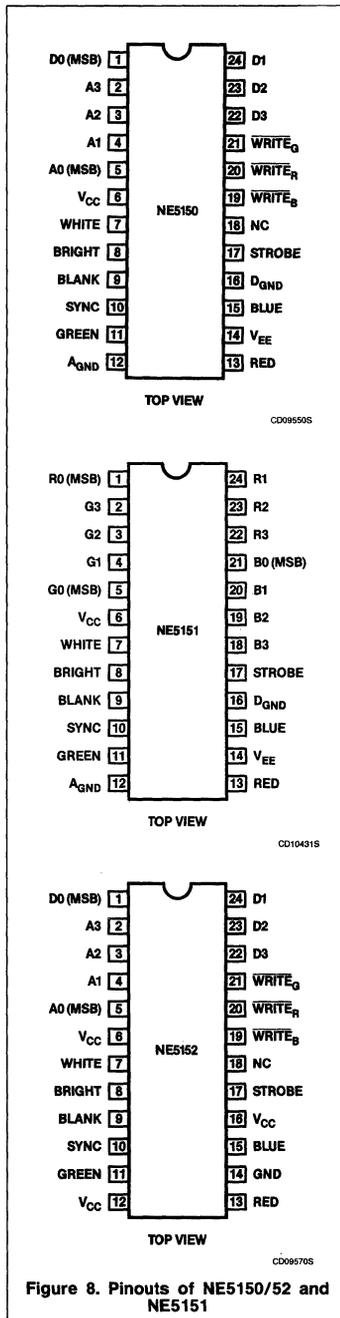
Figure 8. Pinouts of NE5150/52 and NE5151
