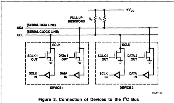
Figure 2. Connection of Devices to the I<sup>2</sup>C Bus
