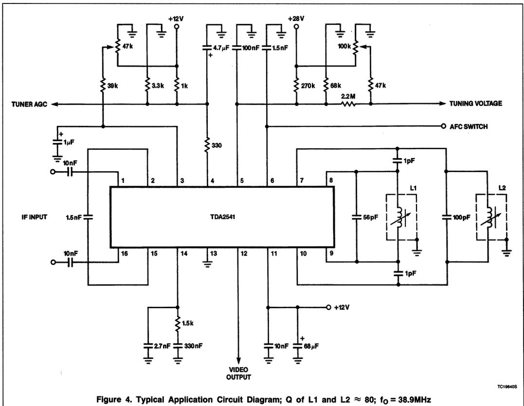
Figure 4. Typical Application Circuit Diagram; Q of L1 and L2  $\approx$  80;  $f_0 = 38.9\text{MHz}$
