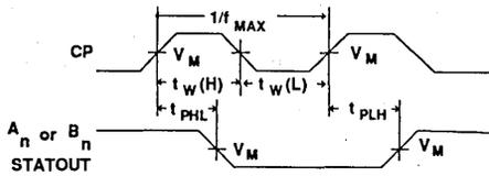
Waveform 1. Propagation Delay, Clock Input To Outputs, Clock Pulse Width, and Maximum Clock Frequency
