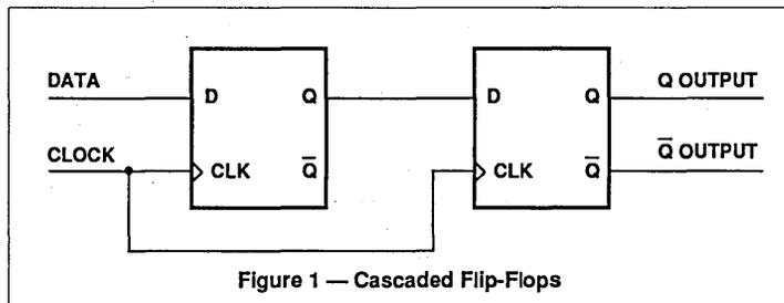
Figure 1 — Cascaded Flip-Flops
