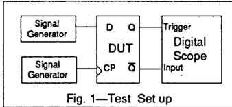
fied on the 74F5074. By running two independent signal generators (see Fig. 1) at nearly the same frequency (in this case 10 MHz clock and 10.02 MHz data) the device-under-test can often be driven into a metastable state. If the Q output is then used to trigger a digital scope set to infinite persistence the  $\bar{Q}$  output will build a waveform. An experiment was run by continuously operating the devices in the region where metastability will occur.
