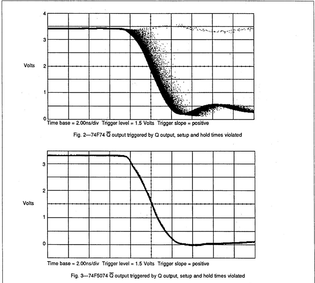
Fig. 2—74F74  $\bar{Q}$  output triggered by Q output, setup and hold times violated
