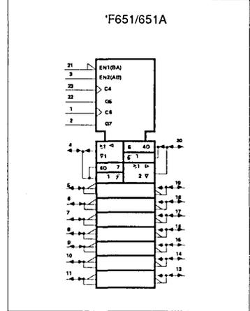
The following examples demonstrate the four fundamental bus-management functions that can be performed with the 'F651/651A and 'F652/652A. The select pins determine whether data is stored or transferred through the device in real time. The Output Enable pins determine the direction of the data flow.
