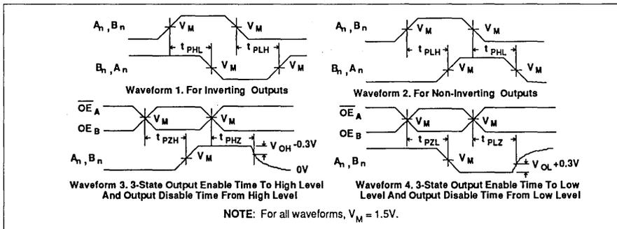
TEST CIRCUIT AND WAVESFORMS
