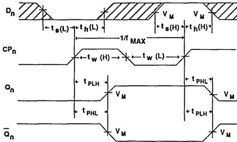
Waveform 1. Propagation Delay For data to output, data setup time and hold times, and clock width
