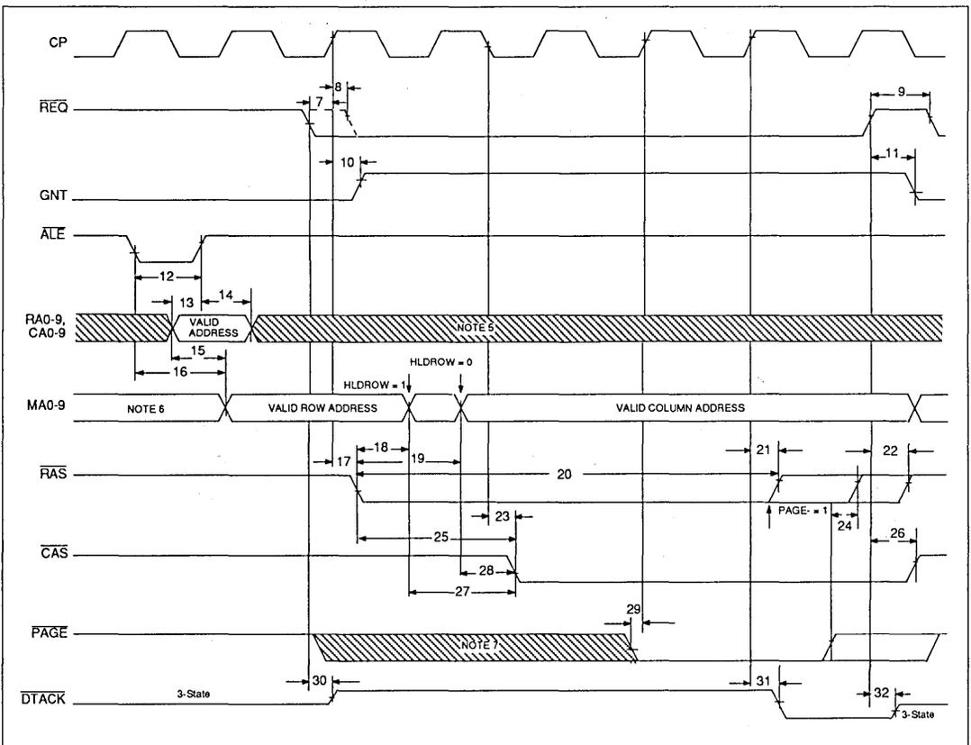
**Note 5:** If the RA0-9 & CA0-9 address inputs are not latched, RA0-9 inputs should remain valid until row address hold time is met and CA0-9 inputs should remain valid until column address hold time is met.
