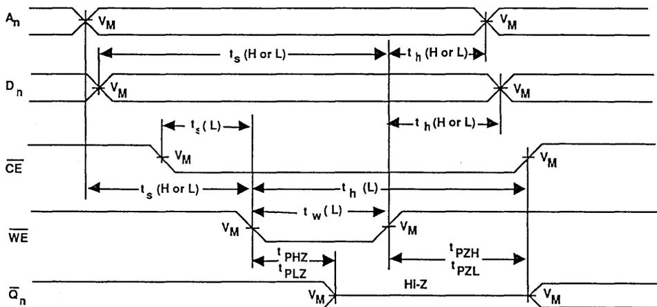
Waveform 4. Write Cycle
