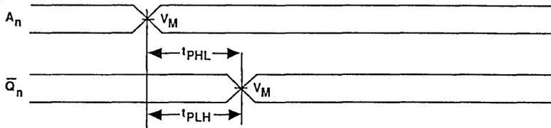
Waveform 1. Read Cycle, Address Access Time
