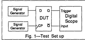
Fig. 1—Test Set up
