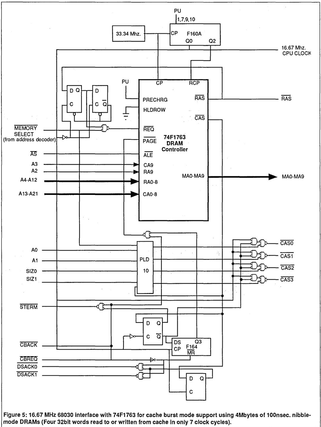
Figure 5: 16.67 MHz 68030 interface with 74F1763 for cache burst mode support using 4Mbytes of 100nsec. nibble-mode DRAMs (Four 32bit words read to or written from cache in only 7 clock cycles).
