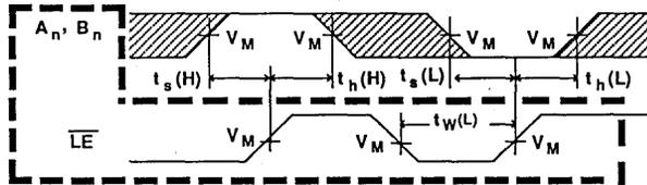
Waveform 3. Data Setup And Hold Times, Latch Enable pulse width
