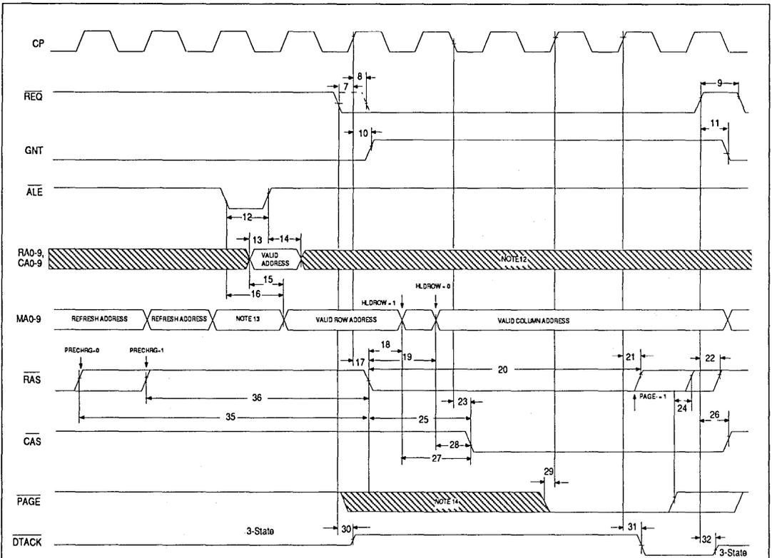
Figure 4: Memory access cycle timing following a refresh cycle
