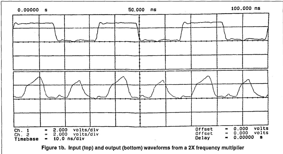
Figure 1b. Input (top) and output (bottom) waveforms from a 2X frequency multiplier
