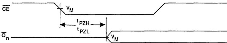
Waveform 2. Read Cycle, Chip Enable Access Time
