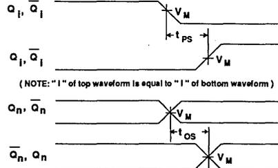
Waveform 4. Propagation delay skew and output to output skew
