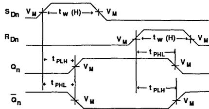
Waveform 2. Propagation Delay for set and reset to output, set and reset pulse width
