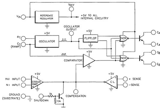
Figure 1. SG1524B Pulse Width Modulator Block Diagram
