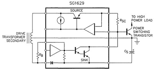
Figure 6. SG1629 Floating Switch Driver Block Diagram
