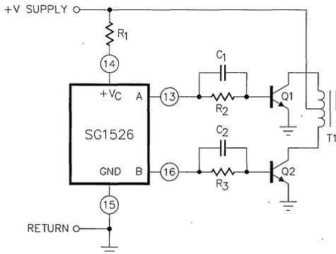
Figure 20. Basic Connections For a Push-Pull Grounded-Emitter Configuration
