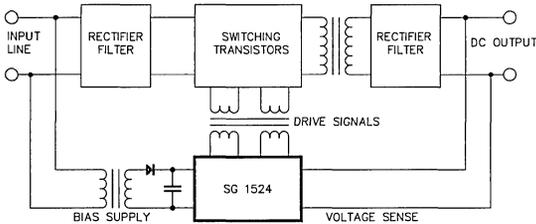
Figure 22. Input/Output Isolation
