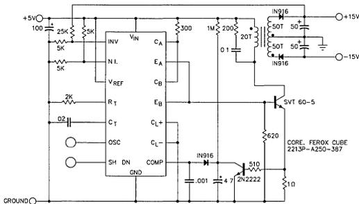
Figure 19. +5 to ±15 Volt, Flyback Converter
