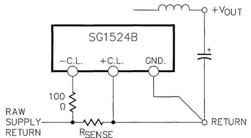
Figure 10. Current Sensing in the Ground Line
