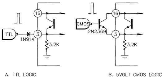
Figure 6. Oscillator Sync to an External Clock
