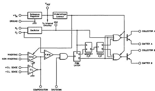
Figure 2. SG1524B Block Diagram
