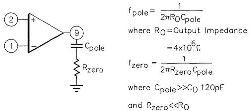
Figure 7. Frequency Compensation of the Error Amplifier
