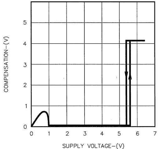
Figure 5 - Undervoltage Lockout At The Error Amp
