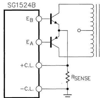
Figure 11. Sensing Primary Current With an Emitter Resistor
