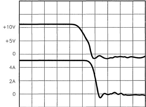
Figure 17. MOSFETS Turn-Off Waveforms.
