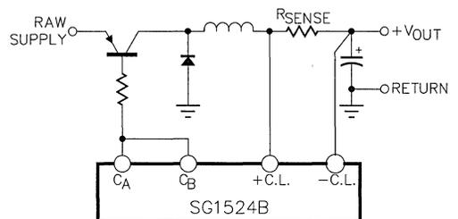
Figure 12. Current Sensing in the Output Line
