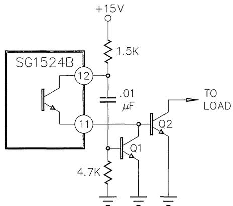
Figure 14. Driving Power Bi-Polar Transistors with the SG1524B
