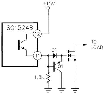
Figure 16. Driving Power MOSFETS With the SG1524B
