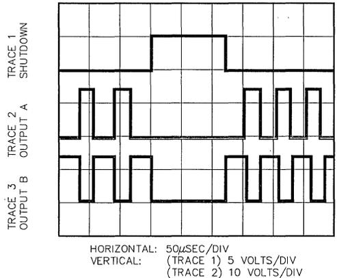
Figure 6. Output Sequence Without Double Pulse Suppression
