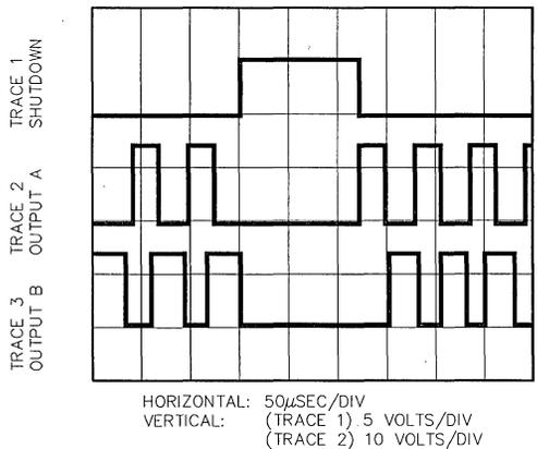
Figure 7. Output Sequence With Double Pulse Suppression
