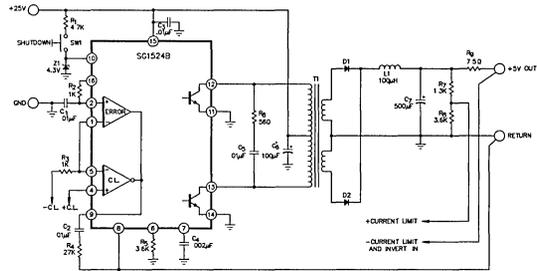
Figure 8. A Single IC 50 kHz Push-Pull Converter
