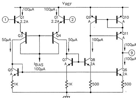
Figure 2. Schematic Diagram of the SG1524B Error Amplifier
