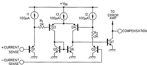
Figure 3. High-Gain Current Limit Amplifier
