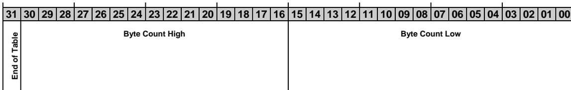
This register defines the byte count register in the PCI bus master logic for IDE Channel #0 in the Sil 0680A. The register bits are defined below.
