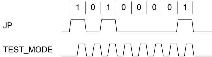
Figure 10-2: Test Mode Register Programming (A1<sub>H</sub>)
