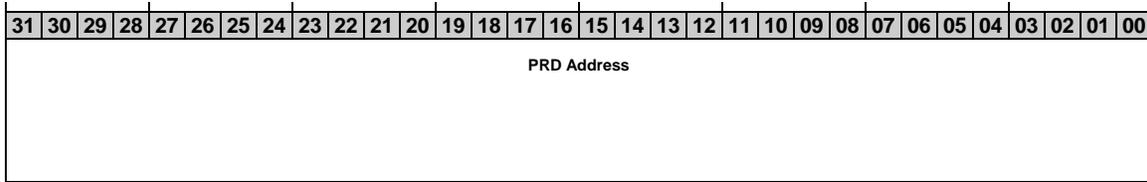
This register reflects the current DMA address and uses for diagnostic purposes only.
