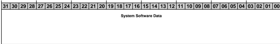
This register is used by the software for non-resettable data storage. The contents are unknown on power-up and are never cleared by any type of reset. The register bits are also mapped to Base Address 5, Offset 4C<sub>H</sub>. See Section 9.7.14 for bit definitions.
