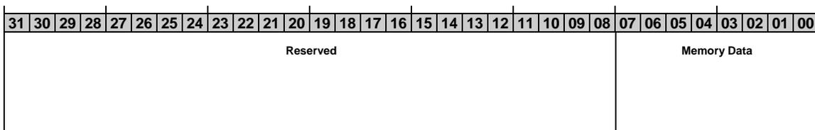
This register defines the data register for FLASH memory interface in the Sil 0680A. The register bits are also mapped to Base Address 5, Offset 54<sub>H</sub>. See Section 9.7.16 for bit definitions.
