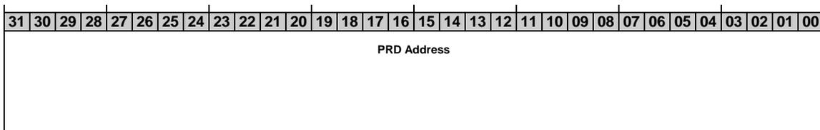
This register reflects the current DMA1 Address and uses for diagnostic purposes only.
