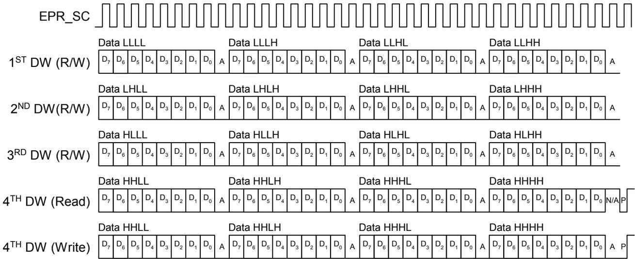
Figure 5: I<sup>2</sup>C Block Transfer
