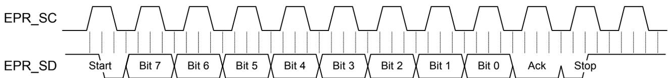
Figure 3: I<sup>2</sup>C Transfer Timing
