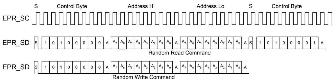
**Figure 4: I<sup>2</sup>C Random Read and Write Timing**
