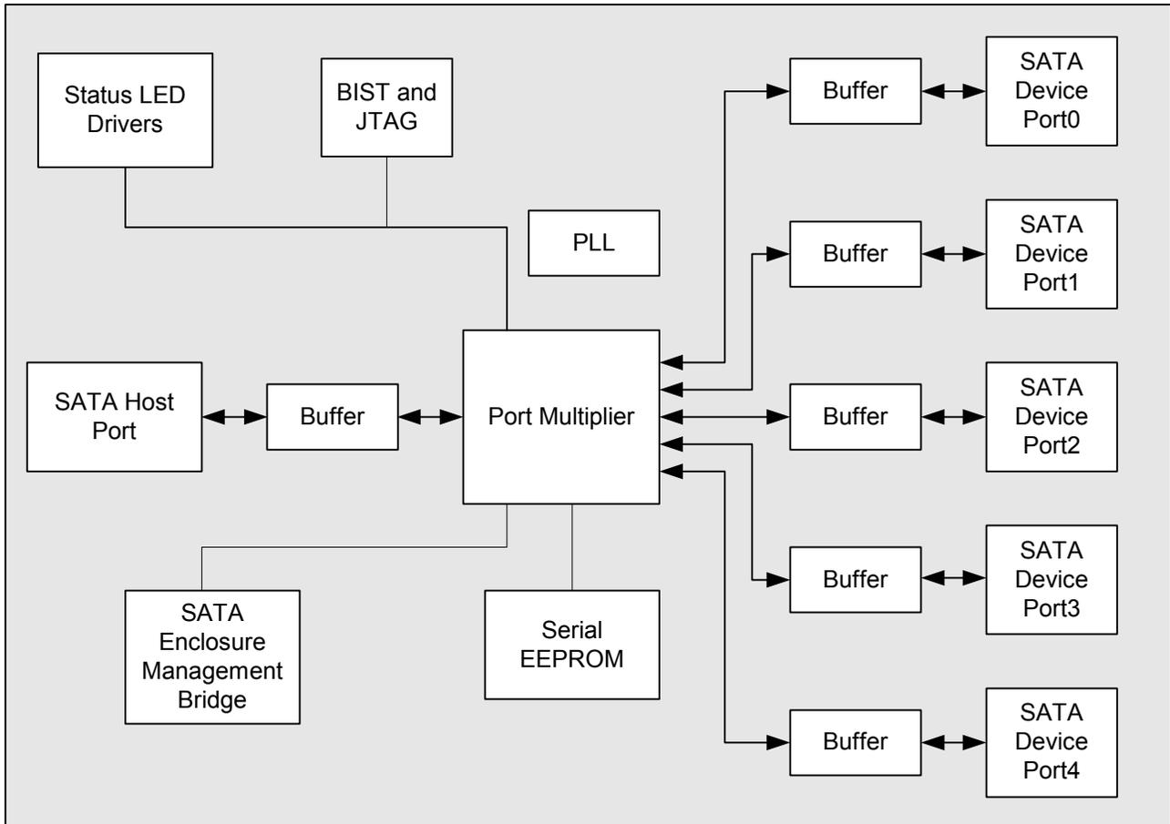
Figure 1: Sil 3726 SATA Port Multiplier Block Diagram
