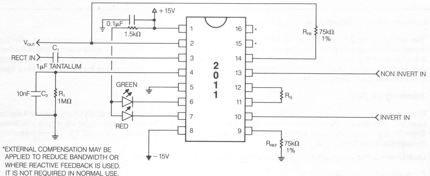
FIGURE 2. STANDARD CONFIGURATION.  $R_G = \frac{150k\Omega}{\text{REQUIRED GAIN}}$
