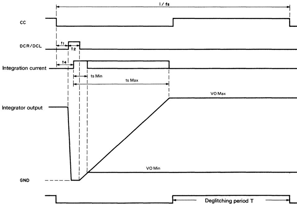
The maximum and minimum values of the integration voltage output,  $V_O \text{ Max}$  and  $V_O \text{ Min}$ , are expressed as follows:
