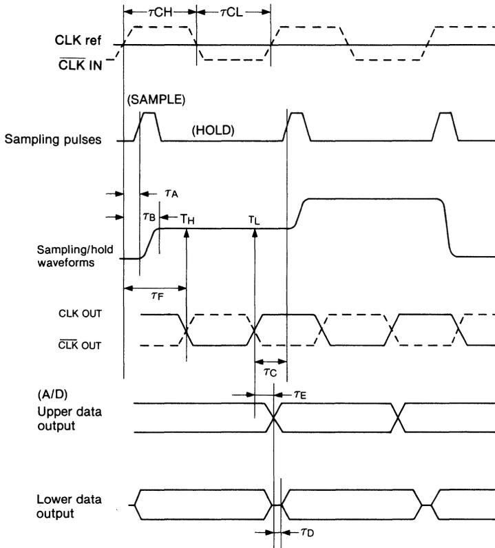
$T_H$  shows a timing when the A/D latches upper 4 bits.
