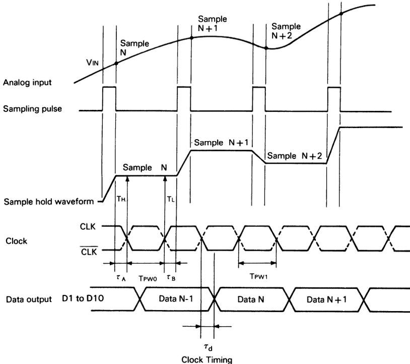
$$\tau_A \geq \tau_A \text{ (Aperture time + setting time of sample and hold circuit)}$$
