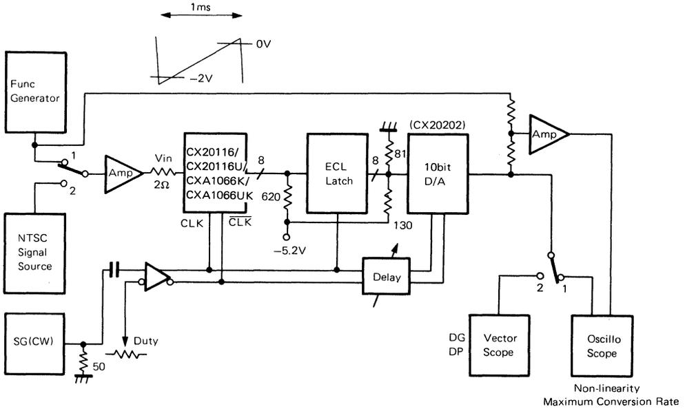
**Differential Non-linearity Measuring Circuit**
