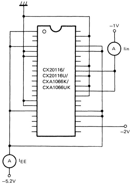
**Aperture Jitter Measuring Circuit**
