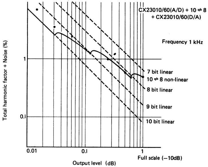
**Total harmonic distortion factor + Noise vs. Input frequency
