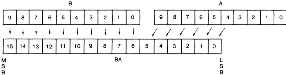
Fig. 6 "BA" Pin Configuration
