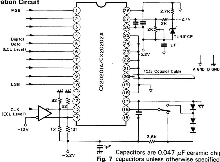
Capacitors are 0.047  $\mu$ F ceramic chip capacitors unless otherwise specified.
