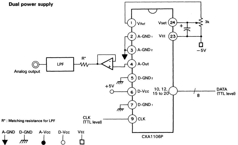
**8 bit 20 MHz A/D Converter Module**
