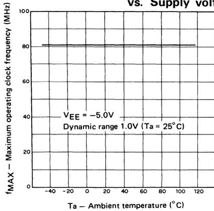
**Maximum operating clock frequency vs. Ambient temperature**
