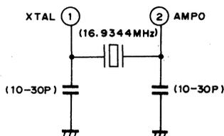
Fig. 1 Oscillation circuit
