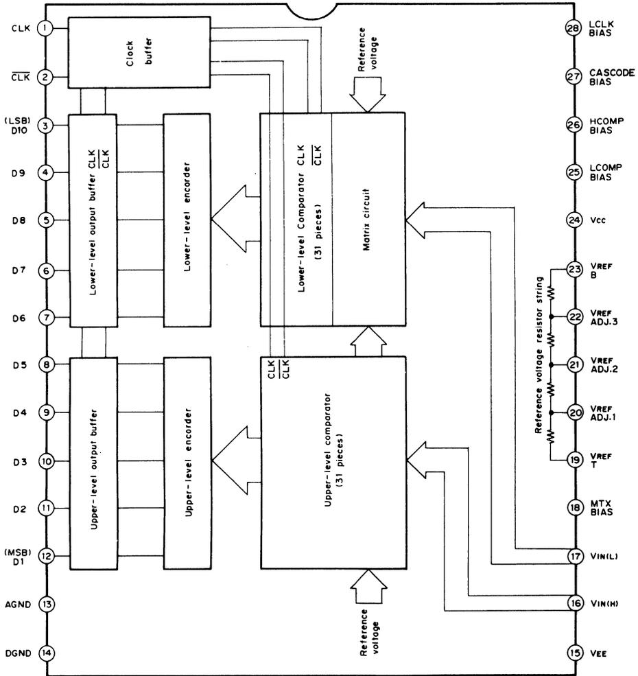
**Pin Description and Equivalent Circuit**
