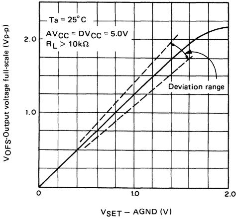
**Output zero offset voltage vs. V<sub>SET</sub>-AGND**
