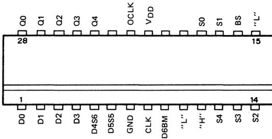
The data is input from D0, D1, D2, D3 and D4S6 and output from Q0, Q1, Q2, Q3 and Q4 respectively, after passing through the stages which is specified by the stage selecting signal. The S0 to S4 and D5S5 are the input pins of the stage selecting signal. Now, assuming that
