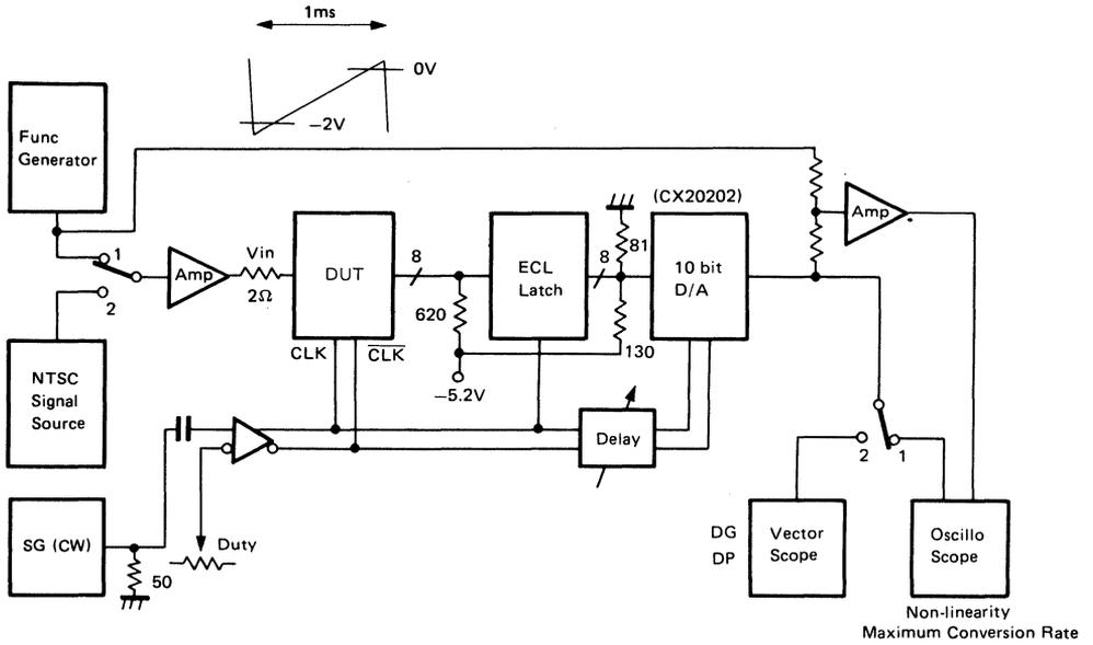
**Differential Non-linearity Measuring Circuit**
