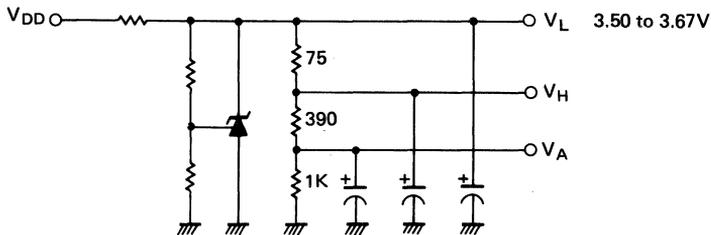
Resistance tolerance of 5% is recommended.
