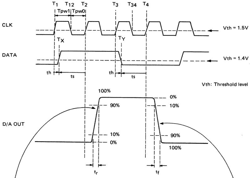
At the time  $t = T_X$ , the data of individual bits are switched and thereafter when the CLK becomes L → H at  $t = T_2$ , the D/A OUT is varied synchronous with it. That is, the D/A OUT is synchronous with the rise of the CLK.
