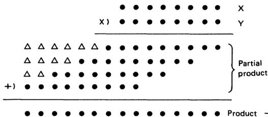
△ ... Sign extend bit for aligning partial product sign bits together
