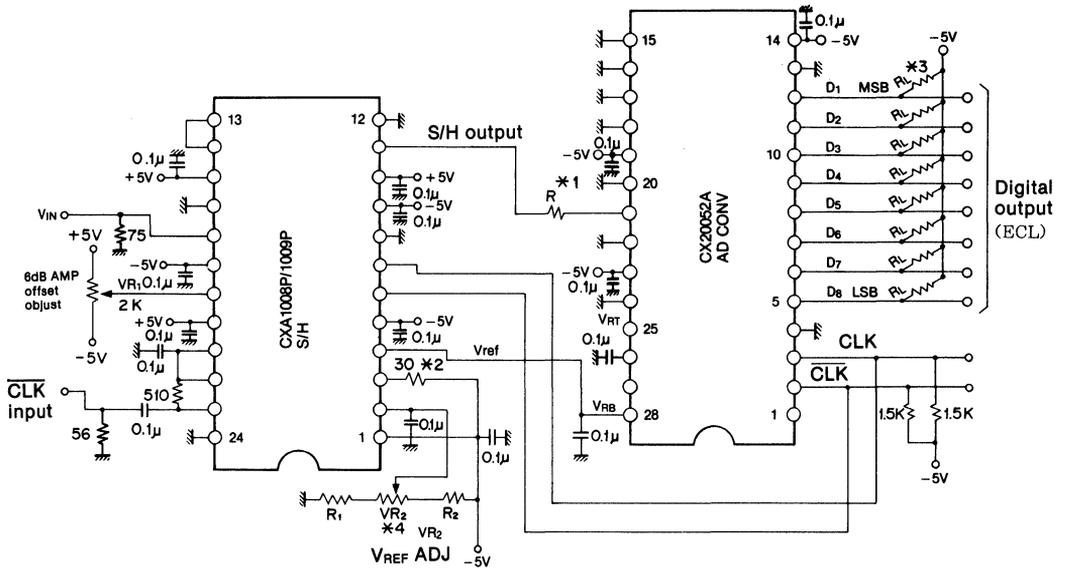
Fig. 5 Connection of CXA 1008P/1009P with CX20052A (1)
