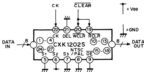
Fig. 3 Circuit of 123 bits delay
