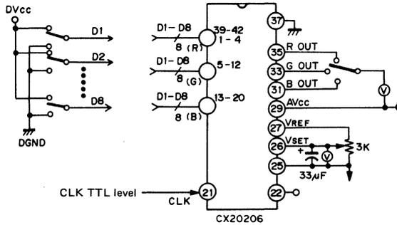
Maximum conversion speed measuring circuit
