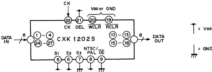
Fig. 1 Circuit of 908 bits delay
