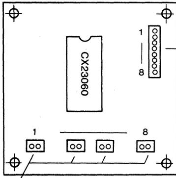
8 pin connector for the input/output of control clock
