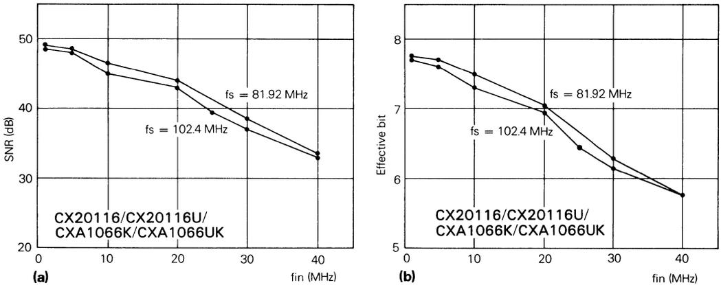
**Fig. 8 SNR and effective bit of CX20116/CX20116U/CXA1066K/CXA1066UK**
