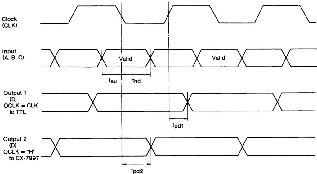
The above timing chart defines t<sub>pd</sub>, t<sub>su</sub> and t<sub>hd</sub> for the clock (CLK). The actual input/output operations are performed with a throughput delay having the number of clocks as shown in the operation mode throughput delay (Fig. 7).
