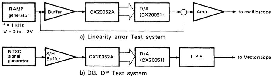
Electrical Characteristics Test Circuit
