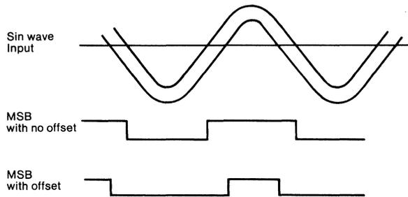
In Fig. 11, integration OP amplifier output. Stays  $\phi$  level when there is no DC offset.
