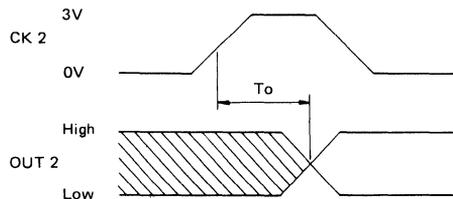
$T_p$ : Time required for I/O to become high impedance from OE input
