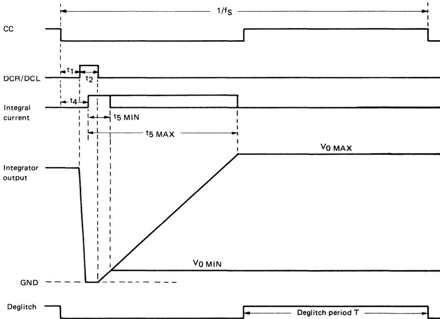
By denoting the clock frequency  $f_{\text{CLK}}$  cycle as  $\tau_0$ , the maximum value  $V_{0\text{MAX}}$  and minimum value  $V_{0\text{MIN}}$  of the integral voltage output can be given as the following equations.
