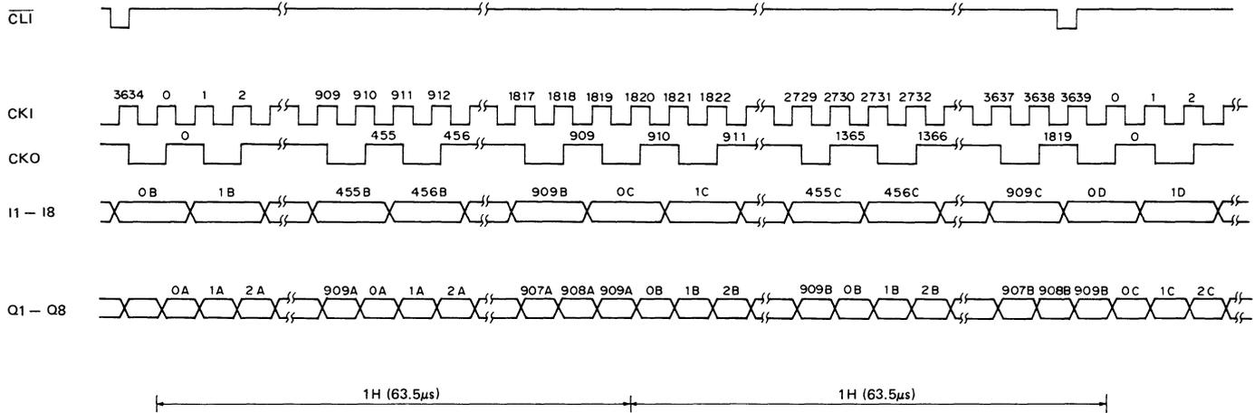
Fig. 2 Double speed conversion timing chart
