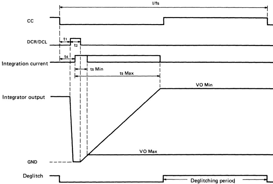
The maximum and minimum values of the integration voltage output,  $VO \text{ Max}$  and  $VO \text{ Min}$ , are expressed as follows.
