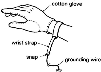
When using a copper wire for grounding, connect a 1M resistance in series near the hand for safety.
