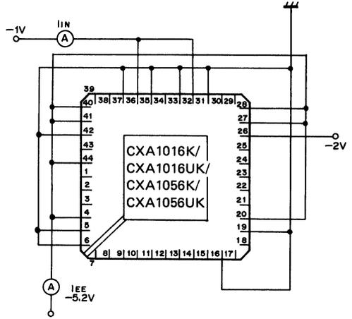
**Aperture Jitter Measuring Circuit**
