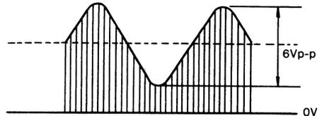
Fig. 3 The Waveform at Point A
