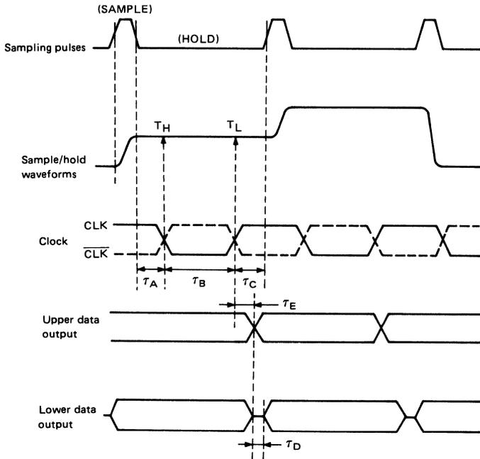
$\tau_A \geq T_A$  (aperture time of S/H circuit + settling time)
