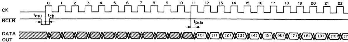
Fig. 7 The data read OUT timing
