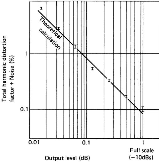
**Total harmonic distortion factor + Noise vs. In frequency (D/A conversion mode)**
