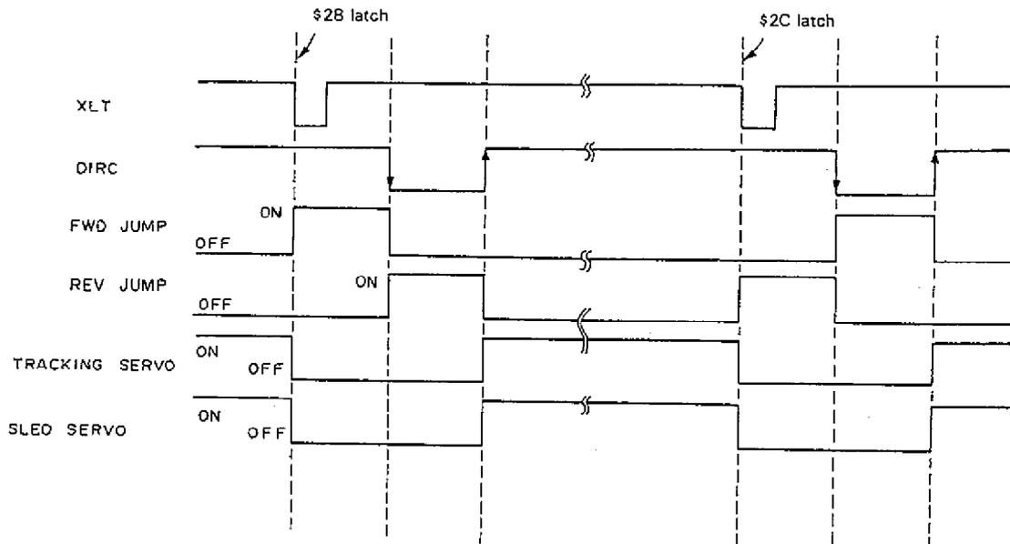
2. LOCK (Sled runaway prevention circuit)
