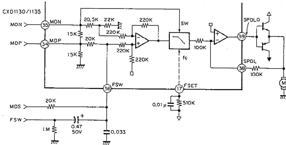
The 200 Hz LPF is formed with 0.033  $\mu$ F and 20 k $\Omega$  connected to pin 36. The secondary LPF is formed with the built-in LPF ( $f_c$  up to 200 Hz with 510 k $\Omega$  for pin 17), and the carrier component of the CLV servo error signals MDS and MDP is eliminated.
