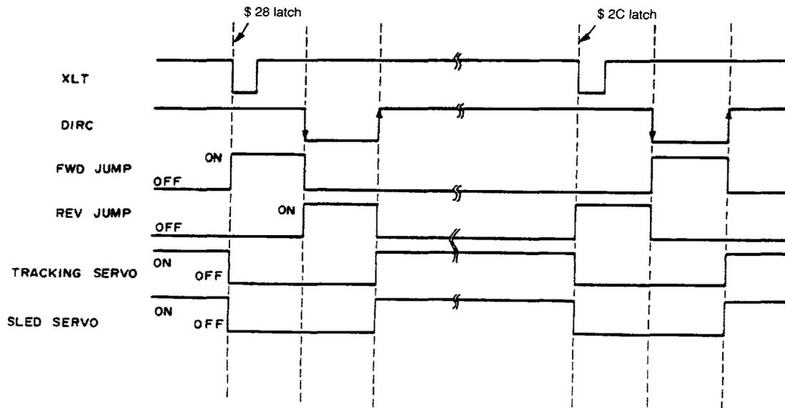
2. LOCK (Sled runaway prevention circuit)
