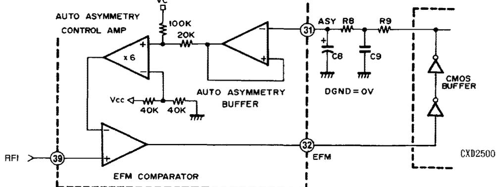
As this comparator is a current SW type, each of the H and L levels is not equal to the power supply voltage. A feedback has to be composed through the CMOS buffer.
