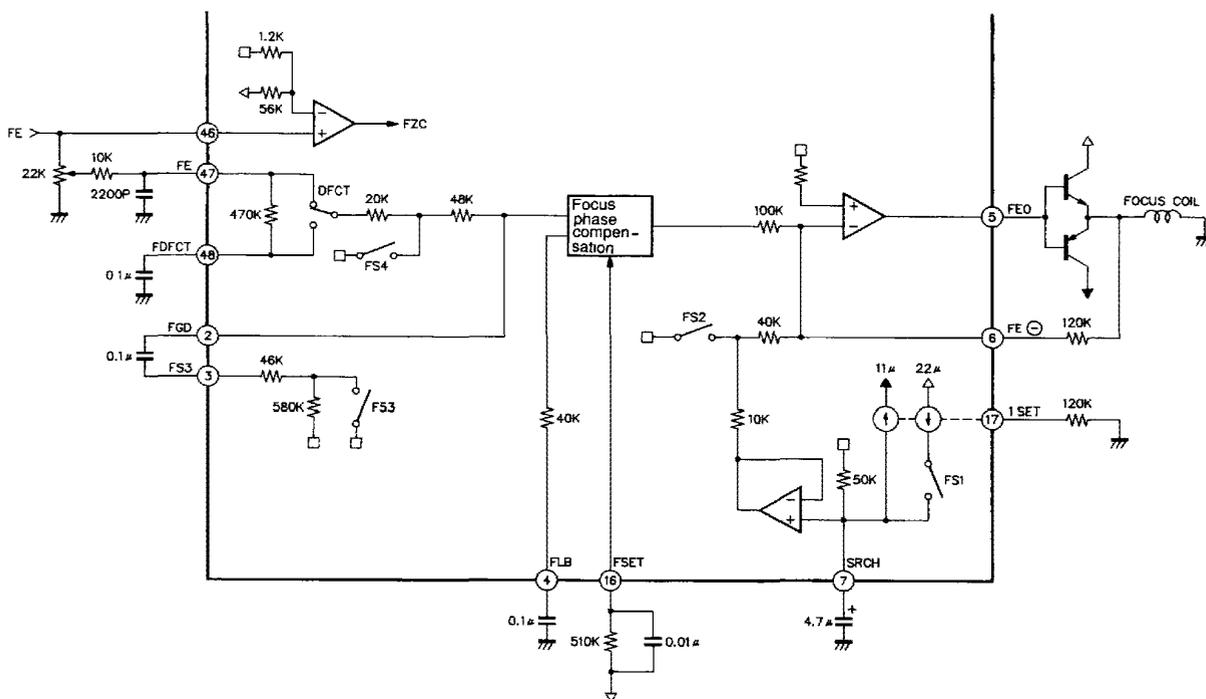
Above is a block diagram of the focus servo system.
