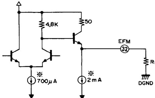
\*The power supply current is given as 5V from Vcc to DGND. Then we have EFM comparator output as follows,
