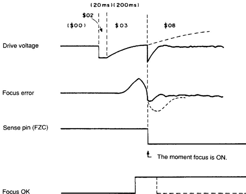
Dotted lines in the diagram after a case where a focus cannot be applied.
