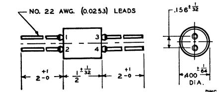
FIGURE 1—2-winding construction
