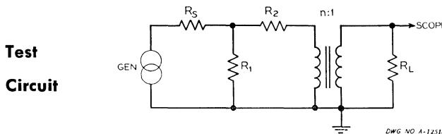
$R_S$  = Pulse Generator Impedance
