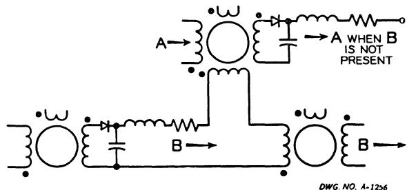
*The outputs of two cores may be mixed into one core.*
