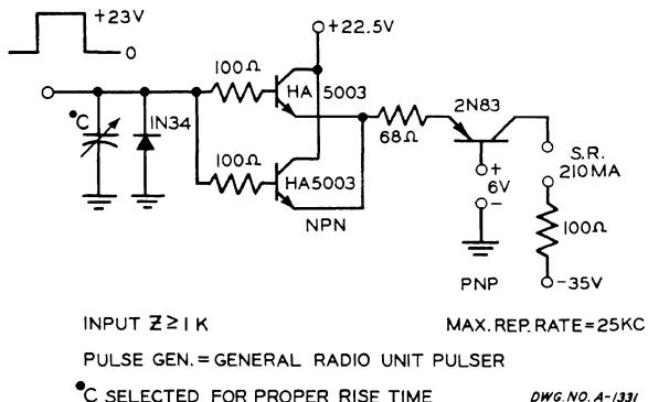
Blocking oscillators may be used as drivers up to repetition rates of 100 kc. These circuits have the advantage of developing the required wave form as well as acting as a current switch. A standard circuit is shown in the following figure with a table of component values and electrical performance.
