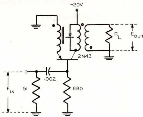
E<sub>IN</sub> - 4 VOLTS, 0.2 μSEC. DWG. NO. A-1774A
