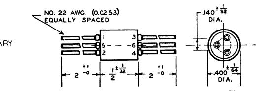
FIGURE 2—3-winding construction
