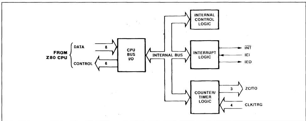
Figure 4 : Counter/ Timer Block Diagram.
