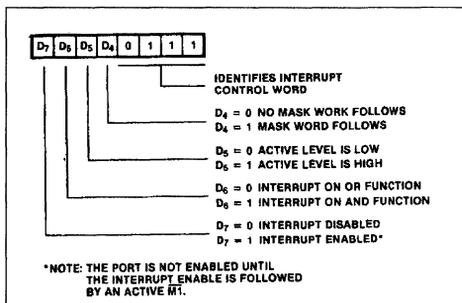
MASK CONTROL WORD. This word sets the mask control register, allowing any unused bits to be masked off. If any bits are to be masked, then D<sub>4</sub> must be set. When D<sub>4</sub> is set, the next word written to the port must be a mask control word (figure 9).
