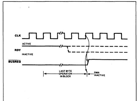
**Figure 18 : Bus Release When Not Ready (Burst Mode).**
