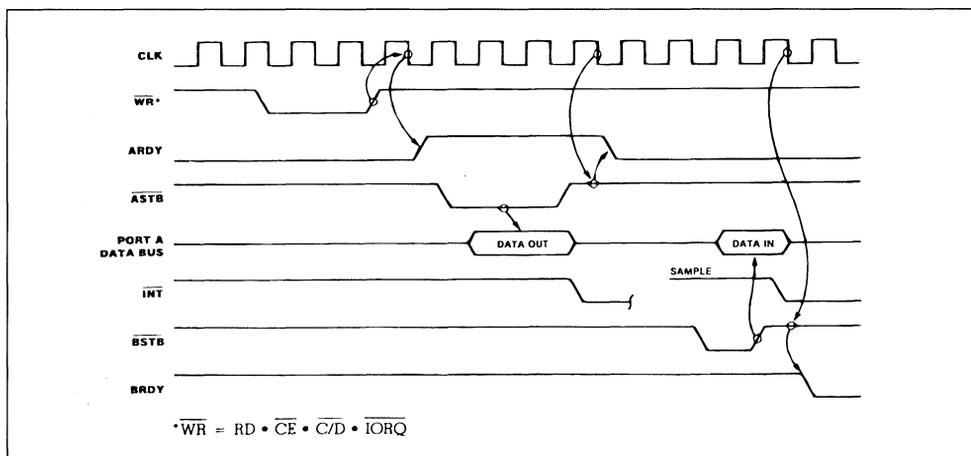
Figure 16 : Mode 3 Bit Mode Timing.
