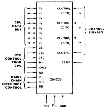
Interrupt processing is simplified because only one vector need be specified ; the CTC internally generates a unique vector for each channel.
