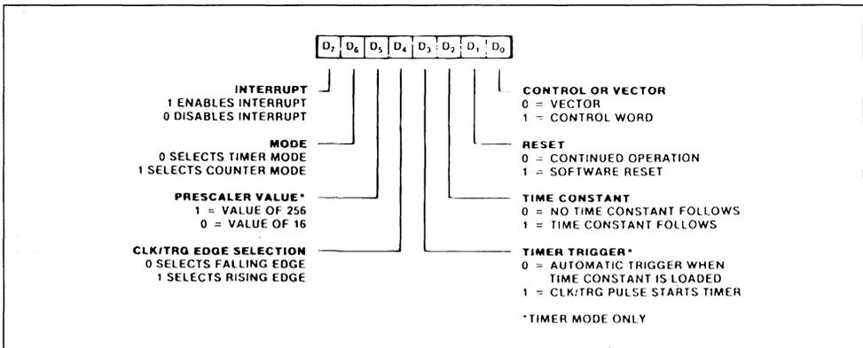
is an update. A channel will not operate without a time constant value. The only way to write a time constant value is to write a control word with D<sub>2</sub> set.
