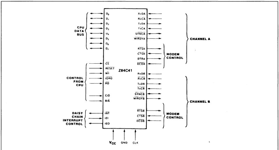
**DTRA, DTRB.** *Data Terminal Ready* (Outputs, Active Low). These outputs follow the state programmed into Z80C SIO. They can also be programmed as general-purpose outputs.
