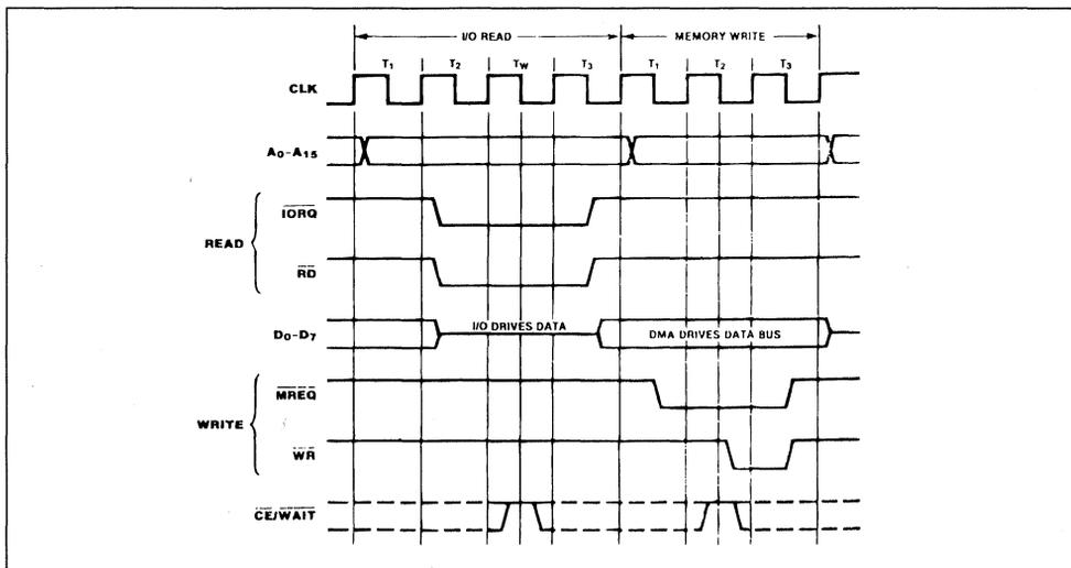
(figure 18). The action on  $\overline{\text{BUSREQ}}$  is thus somewhat delayed from action on the RDY line. The DMA always completes its current byte operation in an orderly fashion before releasing the bus.
