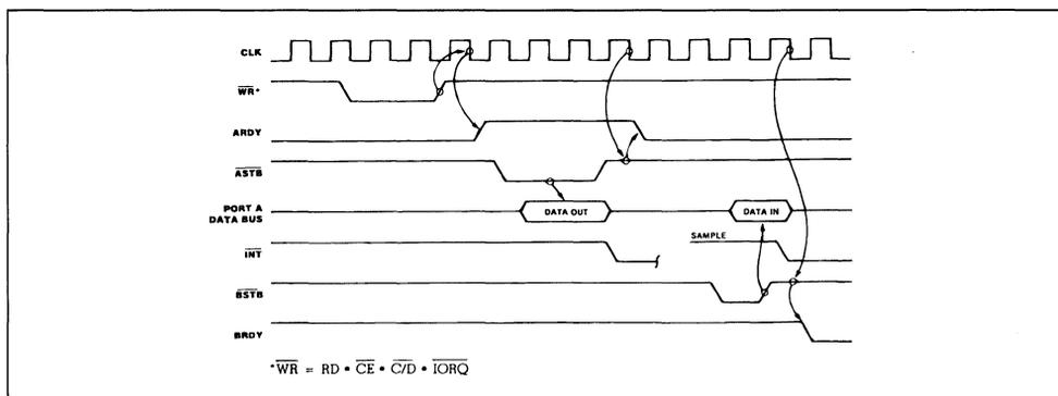
Figure 16 : Mode 3 Bit Mode Timing.
