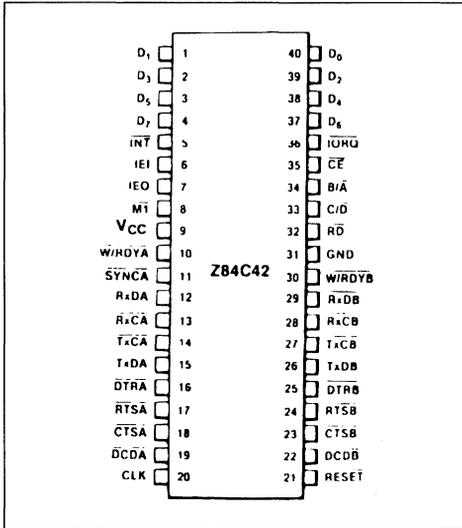
Both pins are Schmitt-trigger buffered to accommodate slow-risetime signals. The SIO detects pulses on these pins and interrupts the CPU on both logic level transitions. Schmitt-trigger buffering does not guarantee a specific noise-level margin.
