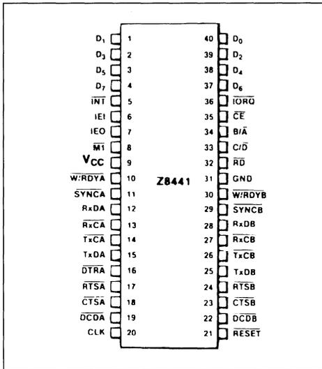
IORQ are all active, the channel selected by B/A transfers data to the CPU (a read operation). When CE and IORQ are active but RD is inactive, the channel selected by B/A is written to by the CPU with either data or control information as specified by C/D. If IORQ and M1 are active simultaneously, the
