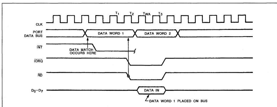
Figure 17 : Interrupt Acknowledge Timing.
