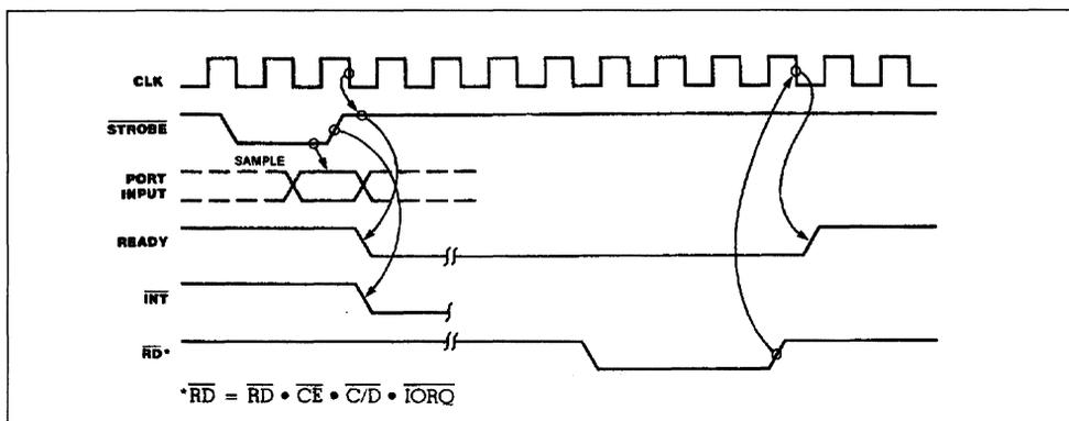
Figure 15 : Mode 2 Bidirectional Timing.
