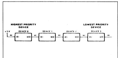
The CTC interrupt logic determines the highest priority channel requesting an interrupt. If the CTC interrupt enable input (IEI) is High, the highest priority interrupting channel within the CTC places its interrupt vector on the data bus when IORQ goes Low. Two wait states ( $T_{WA}$ ) are automatically inserted at this time to allow the daisy chain to stabilize. Additional wait states may be added.
