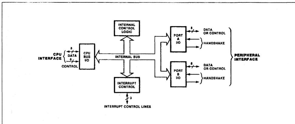
Figure 4 : Typical Port I/O Block Diagram.
