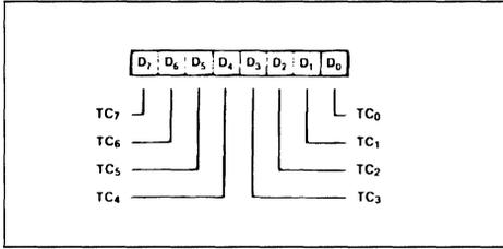
Consequently, the time interval is the product of  $\phi \times P \times T$ . The minimum timer resolution is  $16 \times \phi$  (4  $\mu$ s with a 4 MHz clock). The maximum timer interval is  $256 \times \phi \times 256$  (16.4 ms with a 4 MHz clock). For longer intervals timers may be cascaded.
