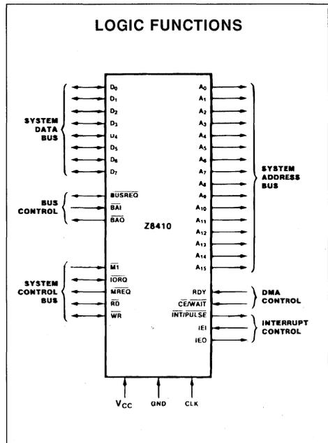
isticated bus and interrupt controls. Many programmable features, including variable cycle timing and auto-restart, minimize CPU software overhead. They are especially useful in adapting this special-purpose transfer processor to a broad variety of memory, I/O and CPU environments.
