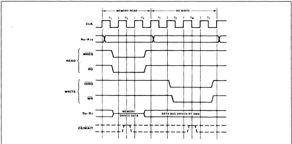
**Figure 10 : CPU-to-DMA Write Cycle**
