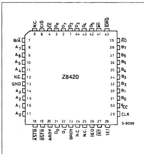
A and Port B. Each port has eight data bits and two handshake signals, Ready and Strobe, which control data transfer. The Ready output indicates to the peripheral that the port is ready for a data transfer. Strobe is an input from the peripheral that indicates when a data transfer has occurred.
