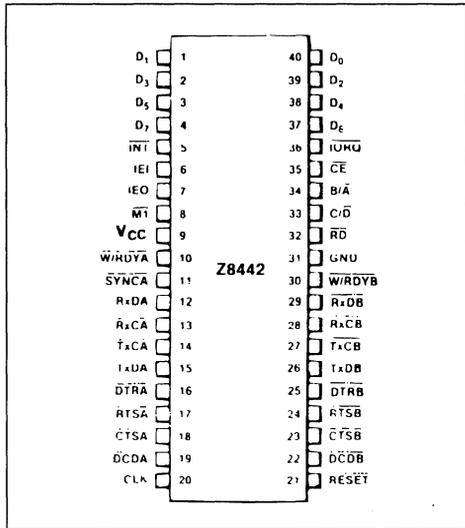
SIO is programmed for Auto Enables ; otherwise they may be used as general-purpose input pins. Both pins are Schmitt-trigger buffered to accommodate slow-risetime signals. The SIO detects pulses
