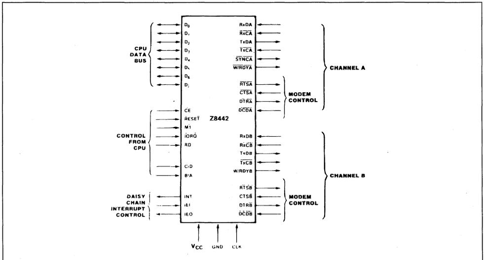
**Figure 2 :** Z80 SIO-2 Dual in Line Pin Configuration.
