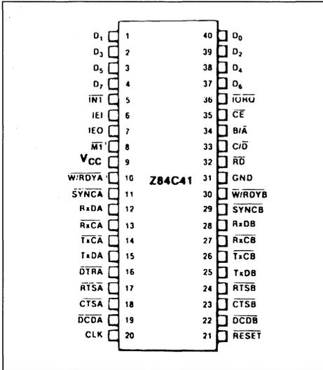
control information as specified by C/D. If IORQ and M1 are active simultaneously, the CPU is acknowledging an interrupt and the SIO automatically places its interrupt vector on the CPU data bus if it
