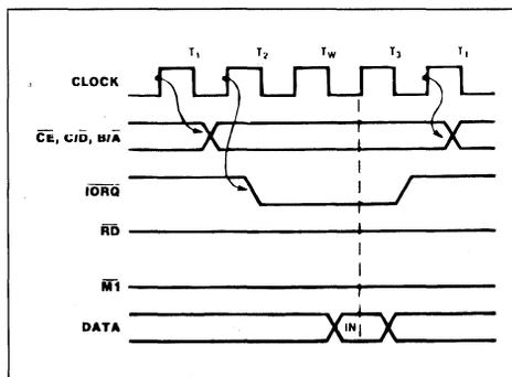
Figure 19 : Interrupt Acknowledge Cycle.
