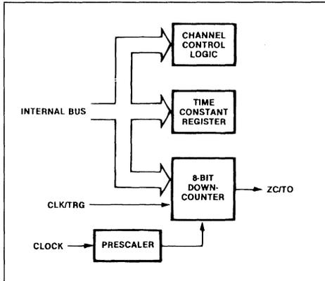
loaded into the down-counter when the counter/time channel is initialized, and subsequently after each zero count.
