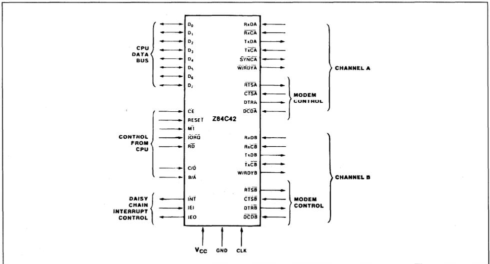
**Figure 2 :** Z80C SIO-2 Dual in Line Pin Configuration.
