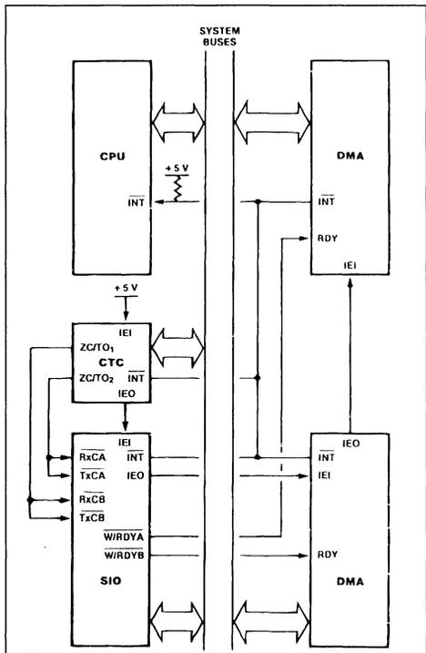
Figure 4 : Function of the Z80 DMA.
