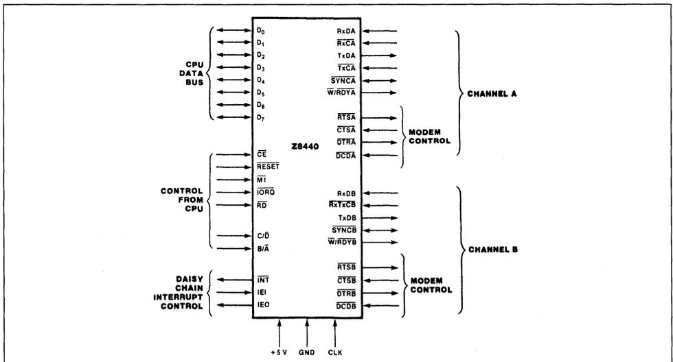
Figure 6 : Z80 SIO-0 Dual in Line Pin Configuration.
