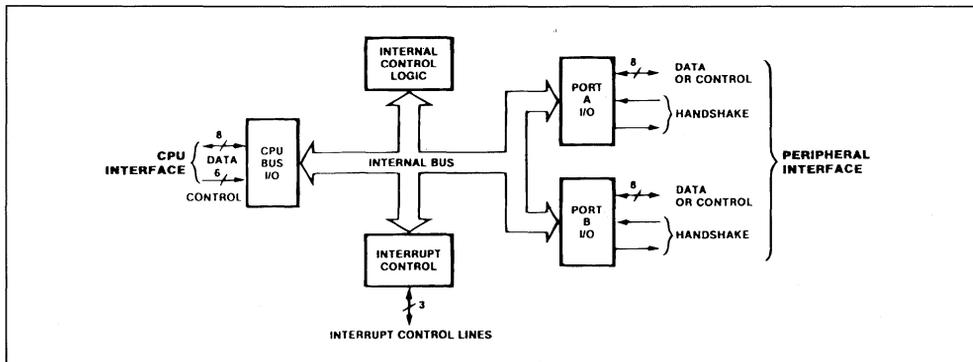
Figure 4 : Typical Port I/O Block Diagram.
