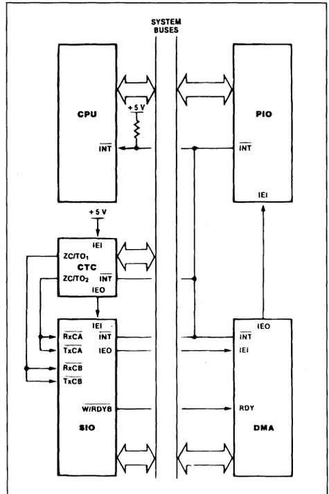
ving an interrupt from any Z80 CTC channel. IEO blocks lower priority devices from interrupting while a higher priority interrupting device is being serviced.
