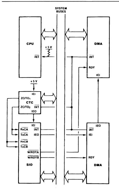
In all modes, once a byte of data is read into the DMA, the operation on the byte will be completed in an orderly fashion, regardless of the state of other signals (including a port's Ready line).
