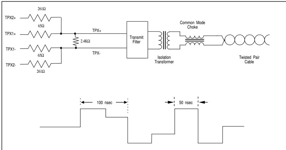
**FIGURE 2-6. TWISTED-PAIR TRANSMIT PATH AND TIMING**
