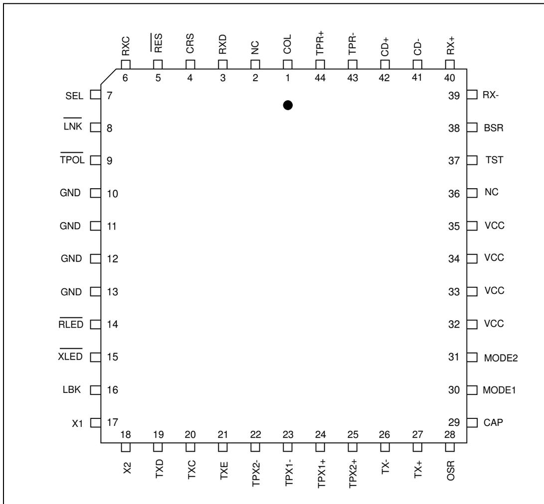
FIGURE 3-1. 83C694C 44-PIN PLCC PACKAGE DRAWING
