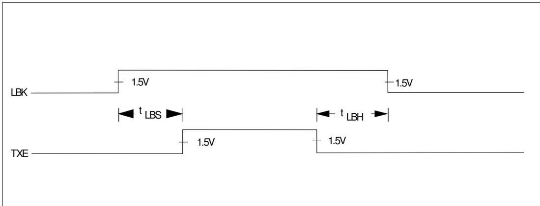
FIGURE 5-11. LOOPBACK TIMING
