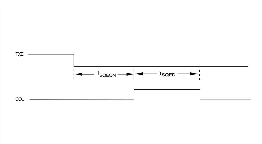
FIGURE 5-10. SQE TEST TIMING
