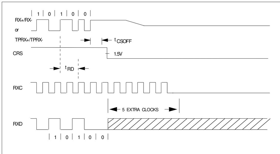
FIGURE 5-6. RECEIVE TIMING - END OF PACKET (LAST BIT = 0)
