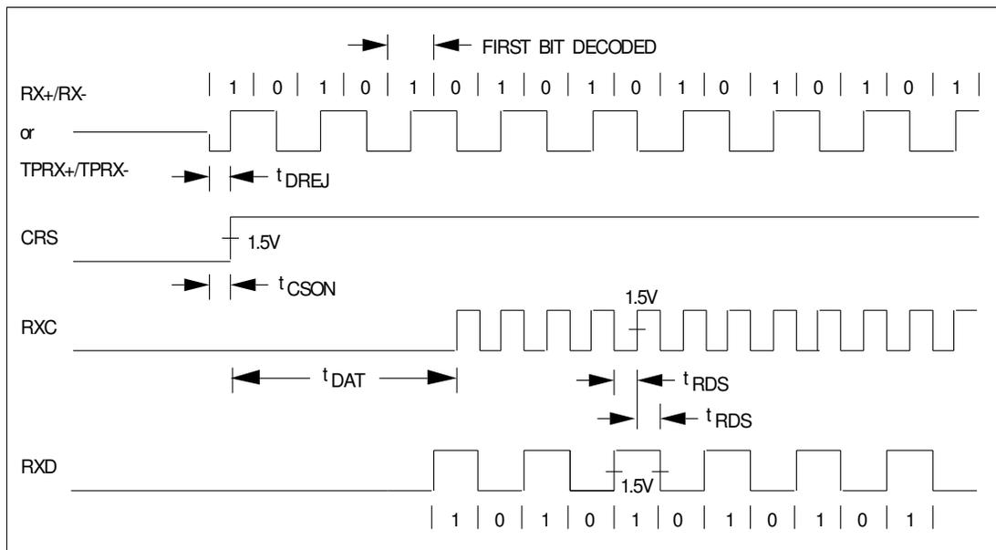
FIGURE 5-5. RECEIVE TIMING - START OF PACKET
