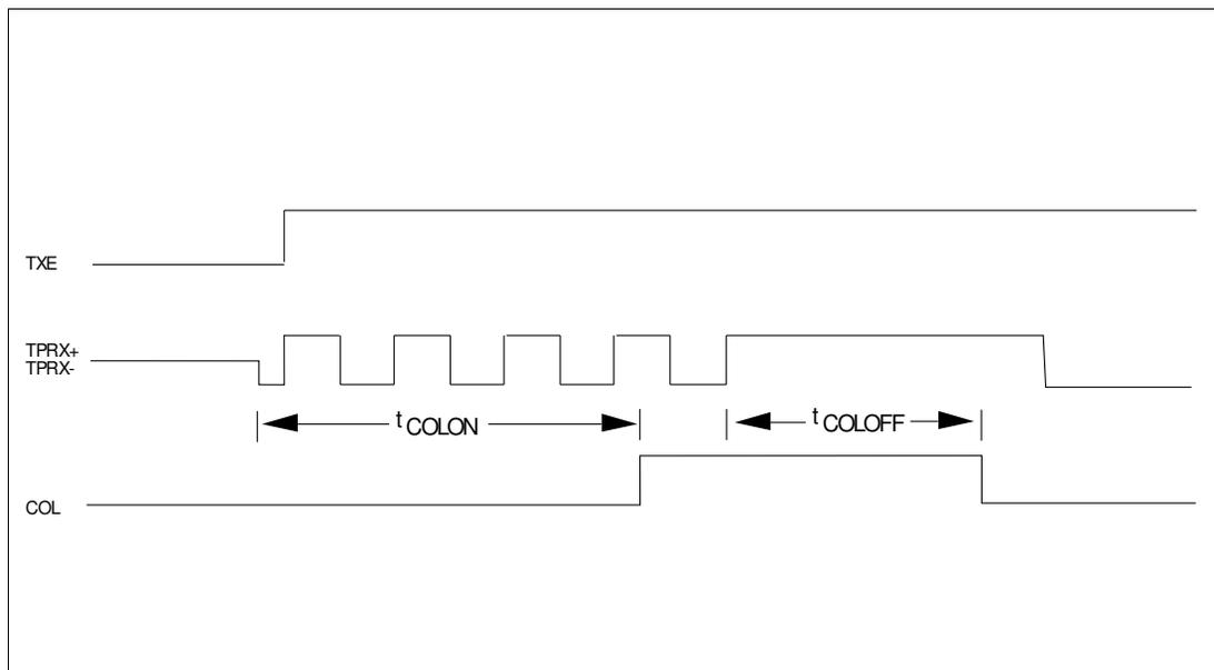
FIGURE 5-9. COLLISION TIMING (TP)
