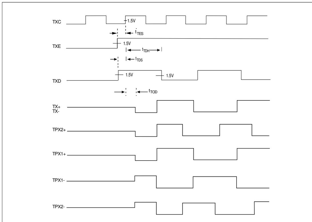
FIGURE 5-1. TX TIMING - START OF TRANSMISSION
