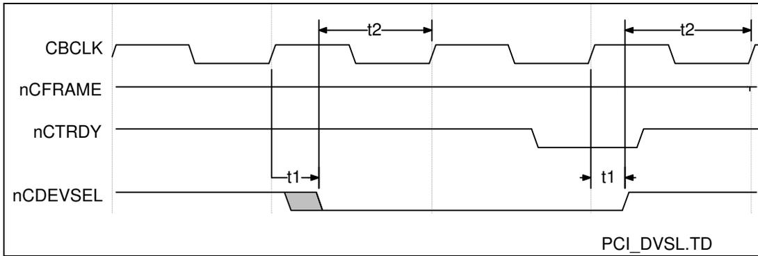
**FIGURE 7 - CardBus/nCDEVSEL TIMING**
