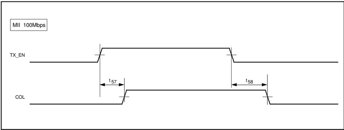
**FIGURE 28 - COLLISION TEST TIMING**
