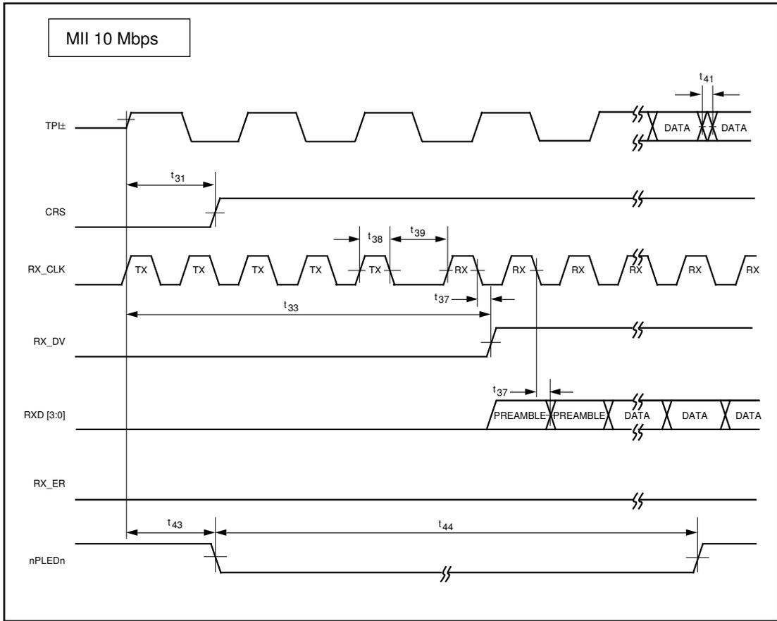
FIGURE 23 - RECEIVE TIMING, START OF PACKET - 10 Mbps
