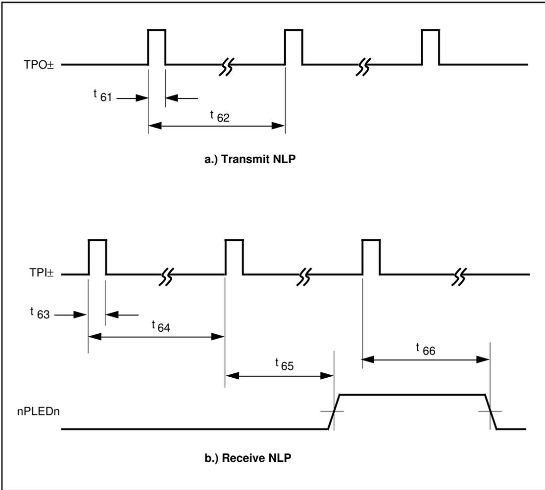
**FIGURE 30 - NLP LINK PULSE TIMING**
