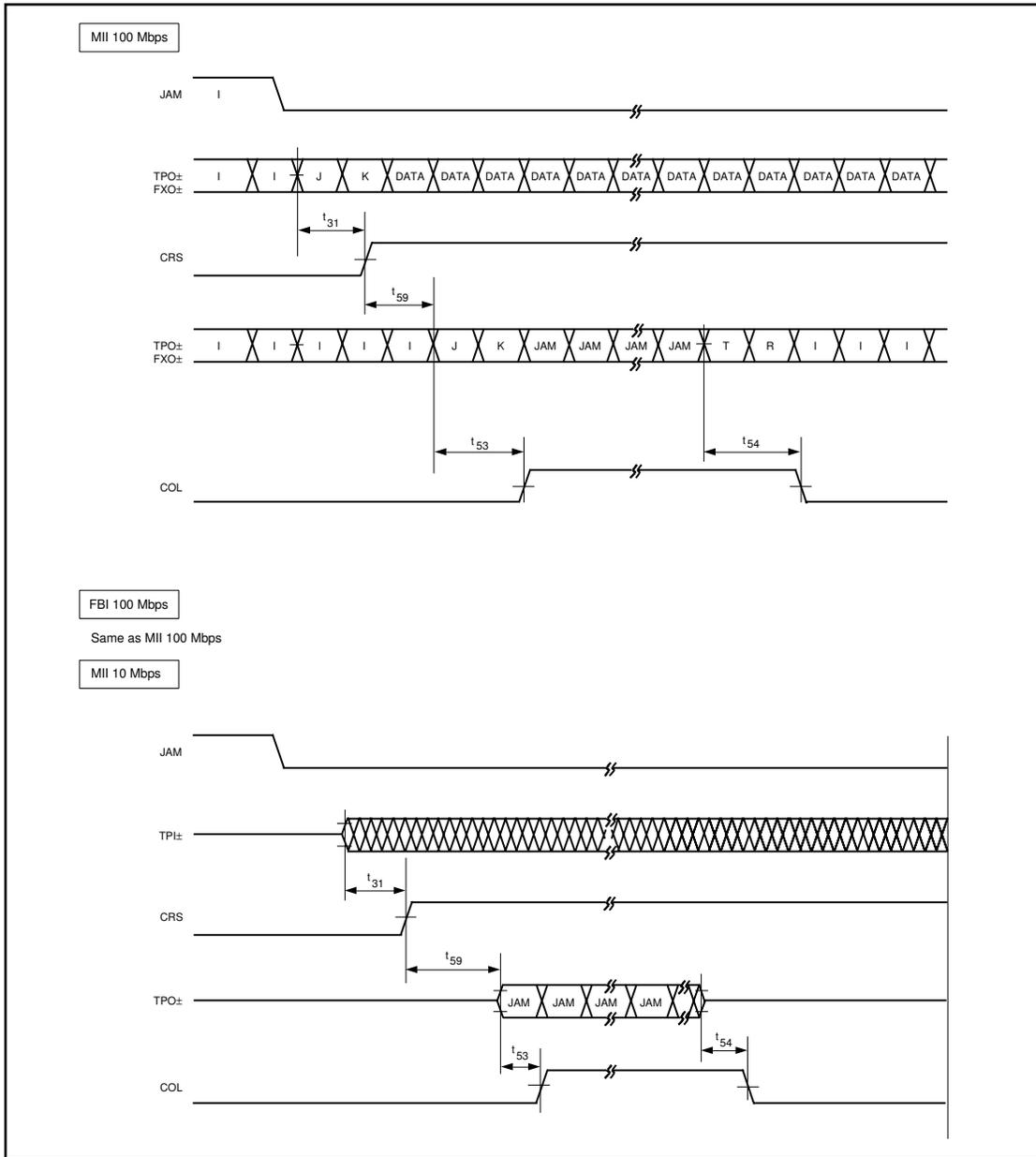
**FIGURE 29 - JAM TIMING**
