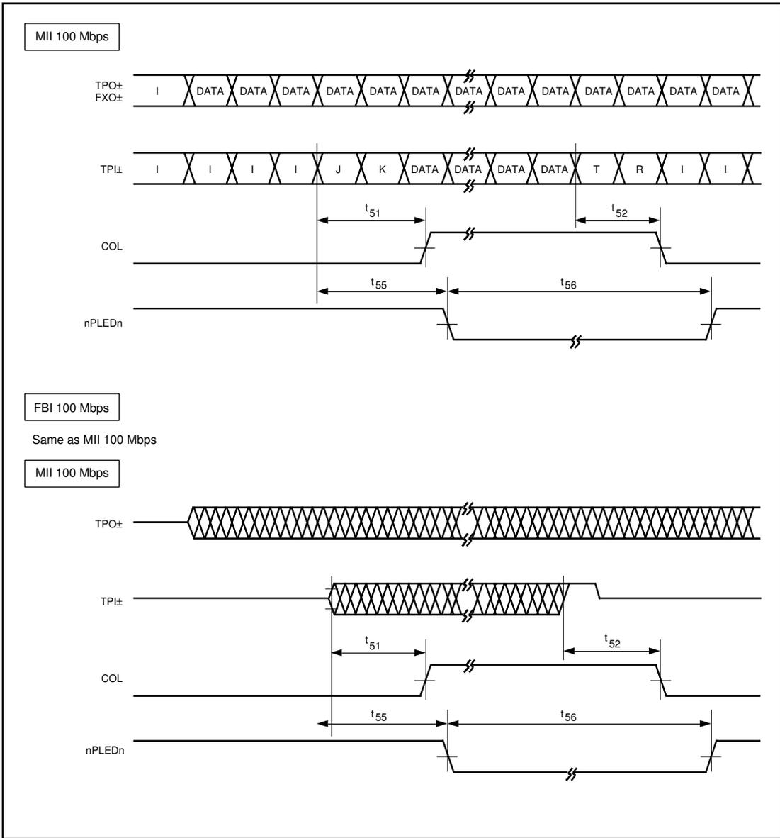
FIGURE 26 - COLLISION TIMING, RECEIVE
