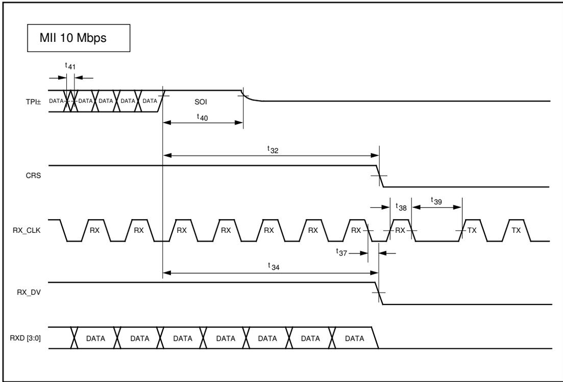
**FIGURE 24 - RECEIVE TIMING, END OF PACKET - 10 Mbps**
