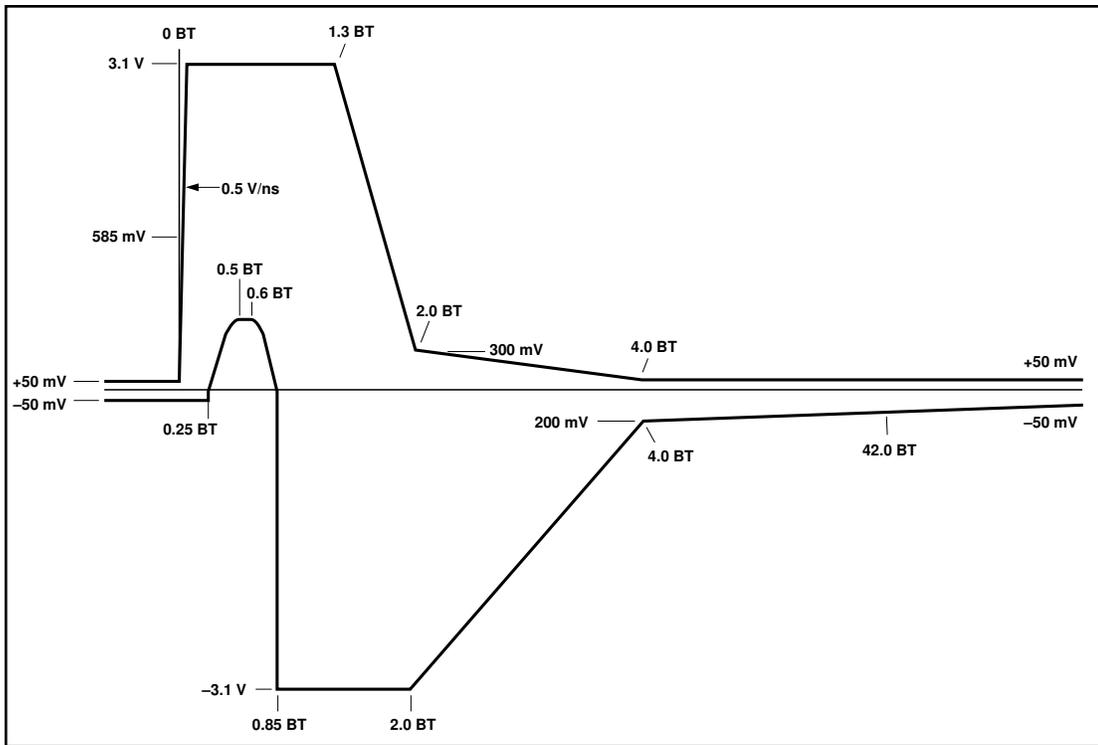
FIGURE 7 - LINK PULSE OUTPUT VOLTAGE TEMPLATE \_ NLP, FLP
