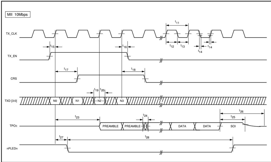
**FIGURE 20 - TRANSMIT TIMING - 10 Mbps**
