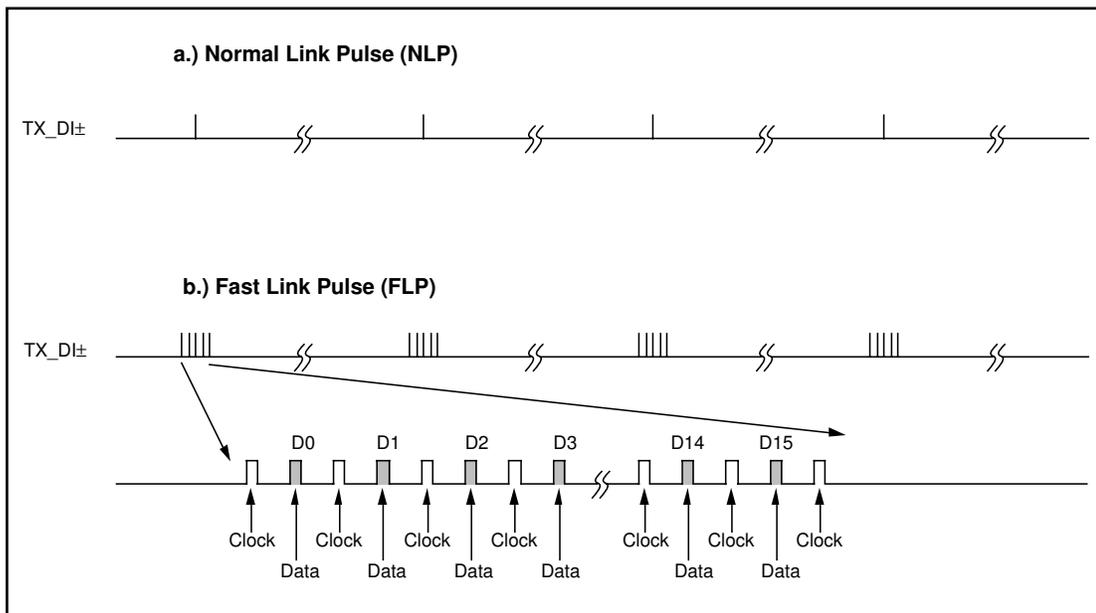
FIGURE 8 - NLP VS. FLP LINK PULSE
