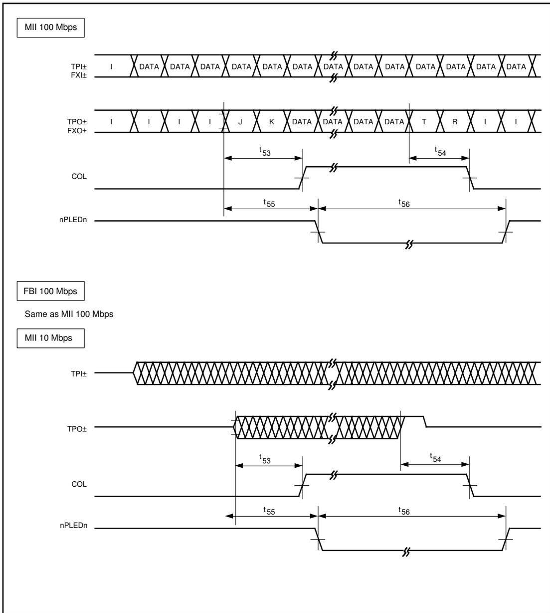
FIGURE 27 - COLLISION TIMING, TRANSMIT
