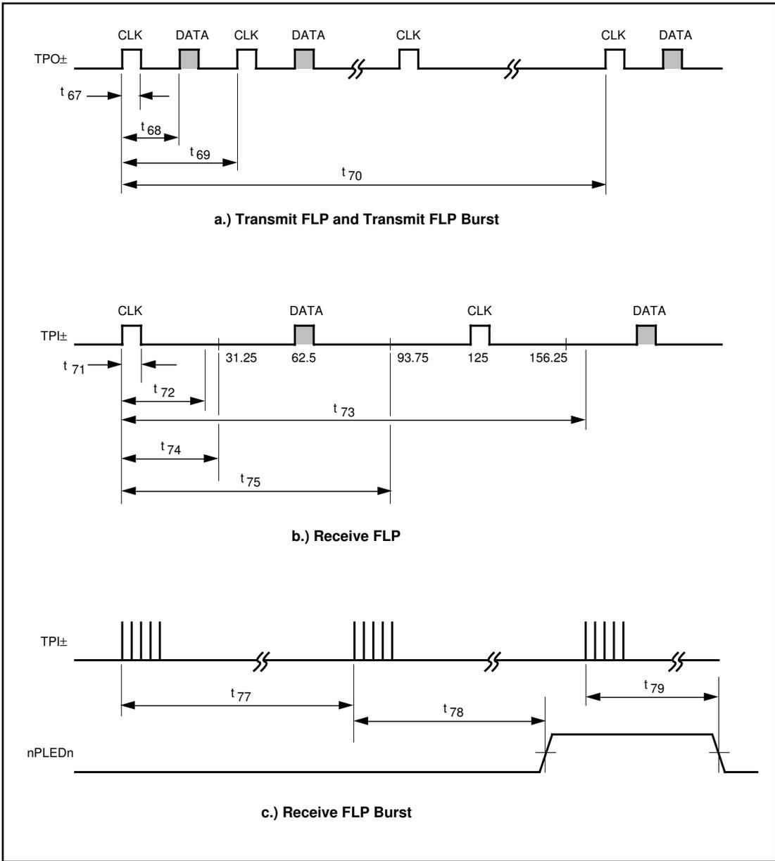
**FIGURE 31 - FLP LINK PULSE TIMING**
