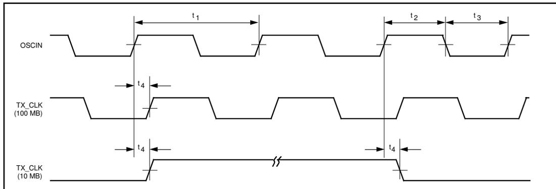
FIGURE 18 - 25 MHz OUTPUT TIMING
