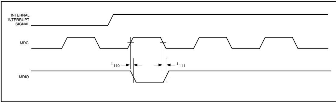
**Figure 35 - MDIO Interrupt Pulse Timing**
