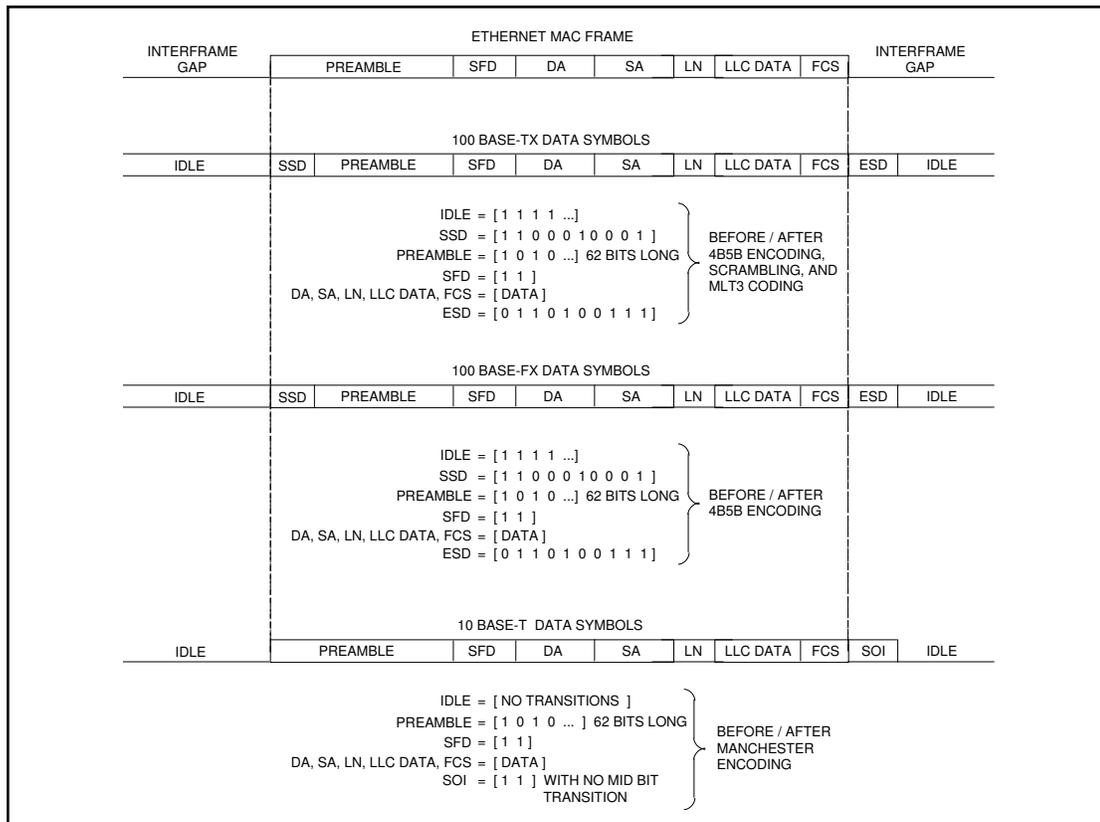
**FIGURE 2 - TX/FX/10BT FRAME FORMAT**
