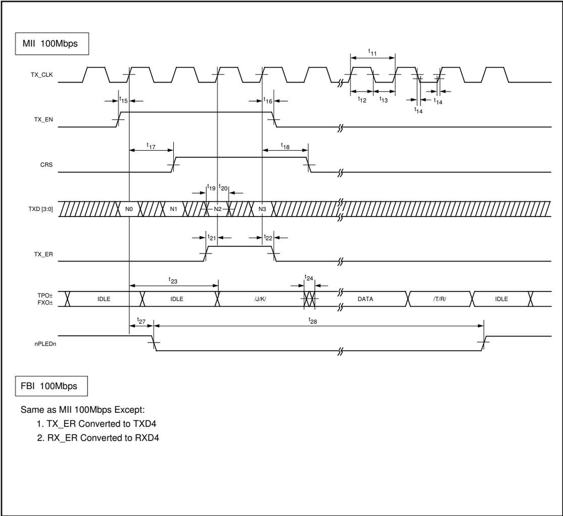
**FIGURE 19 - TRANSMIT TIMING - 100 Mbps**
