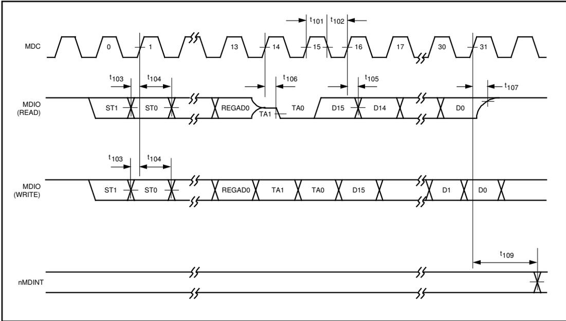
**FIGURE 34 - MI SERIAL PORT TIMING**
