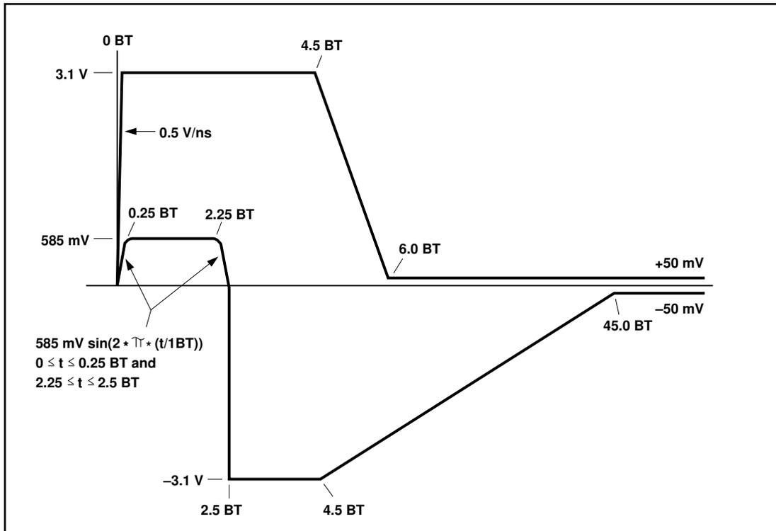
FIGURE 6 - SOI OUTPUT VOLTAGE TEMPLATE - 10 MBPS
