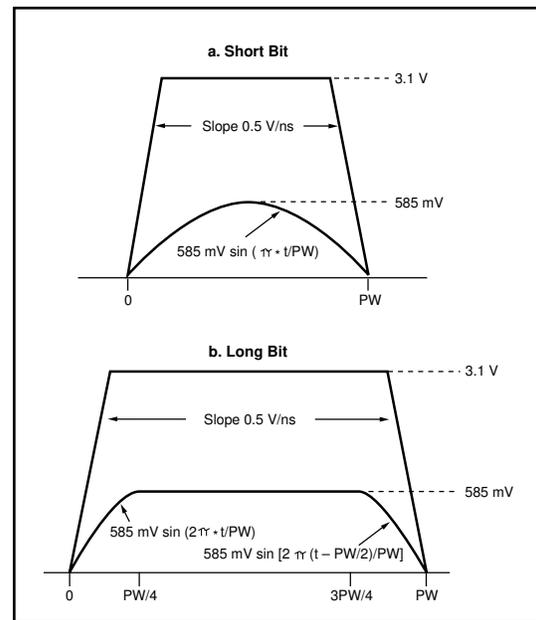
FIGURE 5 - TP INPUT VOLTAGE TEMPLATE-10MBPS
