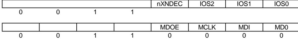
nXNDEC - Read only bit reflecting the status of the nXENDEC pin.
