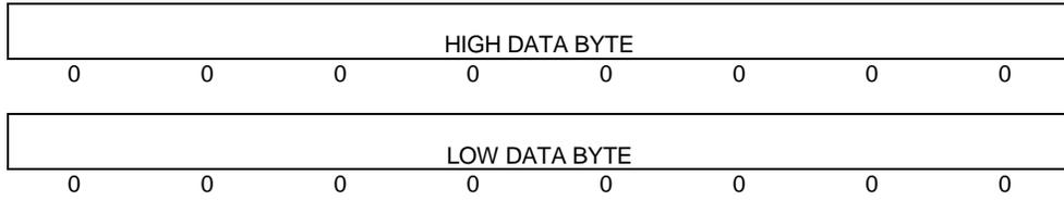
This register can be used as a way of storing and retrieving non-volatile information in the EEPROM to be used by the software driver. The storage is word oriented, and the EEPROM word address to be read or written is specified using the six lowest bits of the Pointer Register.
