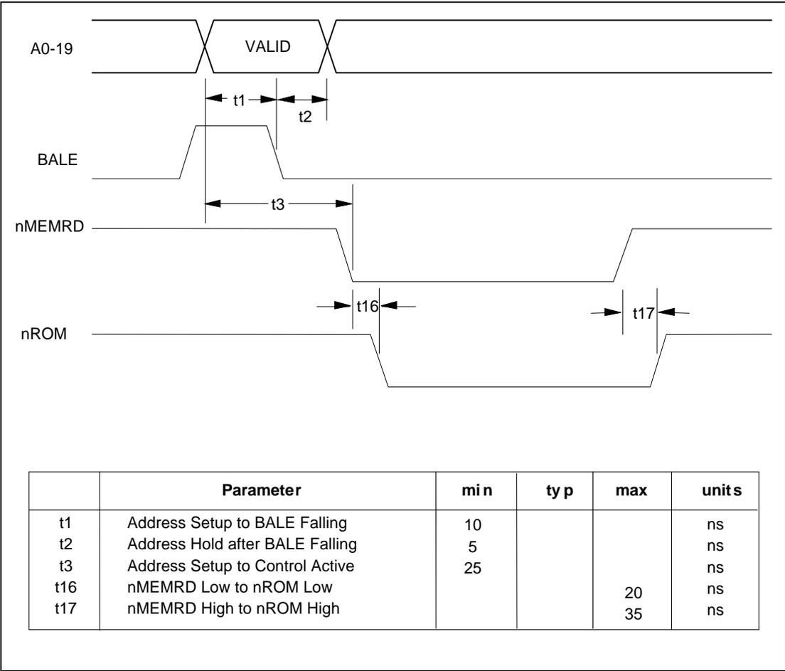
FIGURE 33 - EXTERNAL ROM READ ACCESS USING BALE
