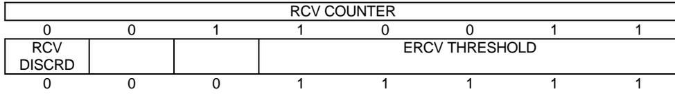
RCV DISCRD - Set to discard a packet being received.
