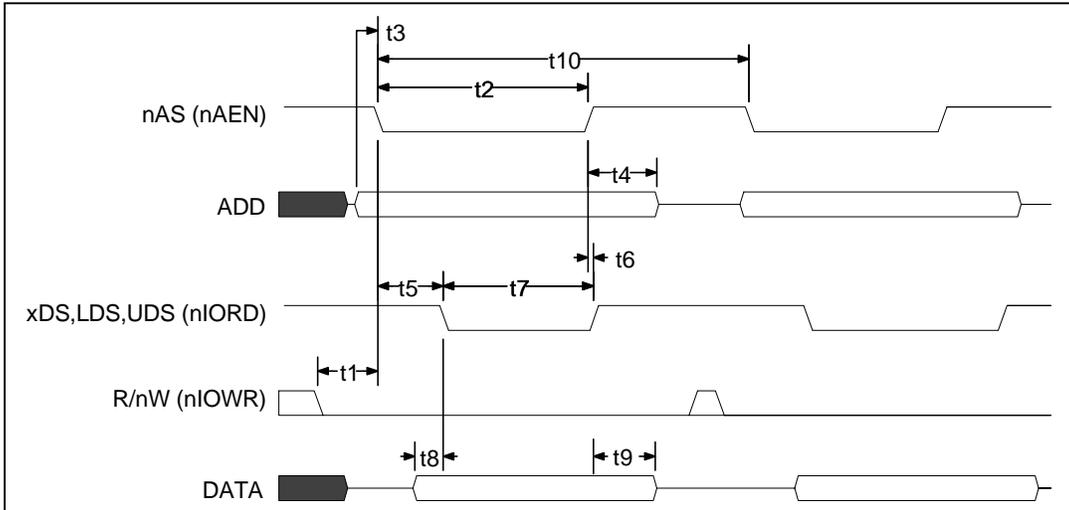
**FIGURE 30 - 68000 WRITE TIMING**
