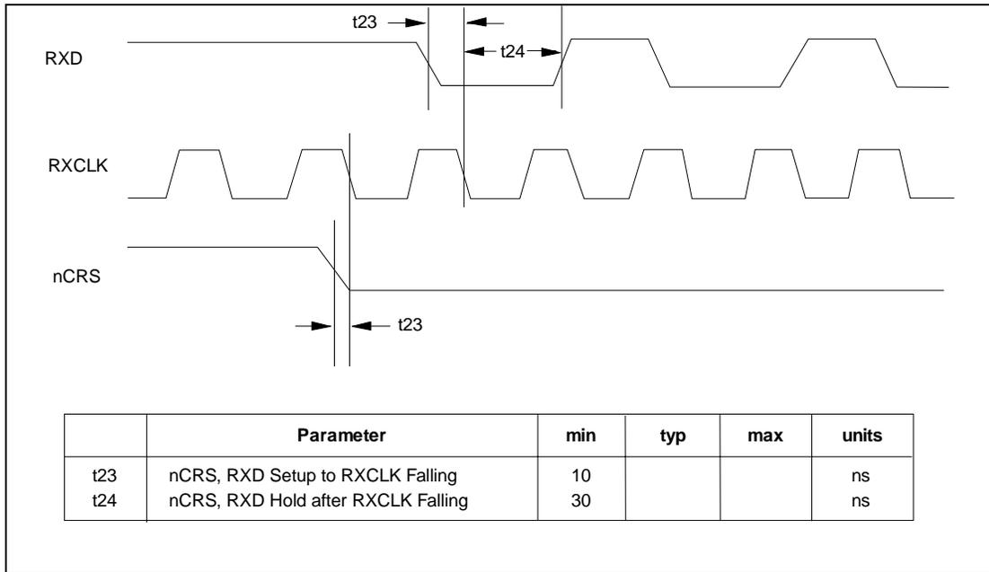
**FIGURE 38 - EXTERNAL ENDEC INTERFACE - RECEIVE DATA
