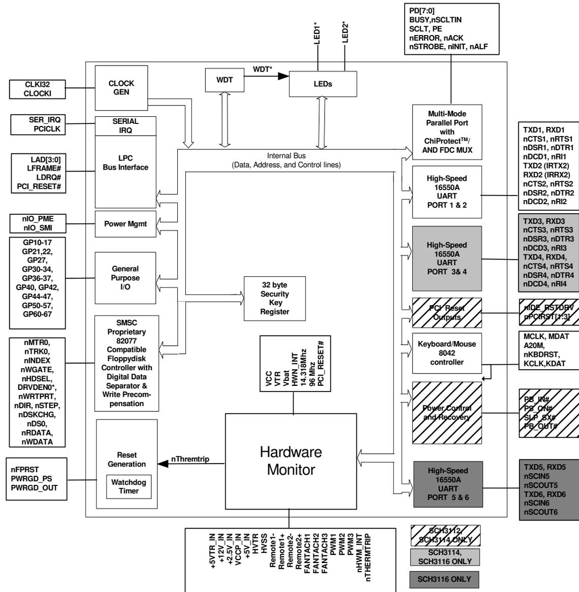
Figure 1 SCH311X Block Diagram
