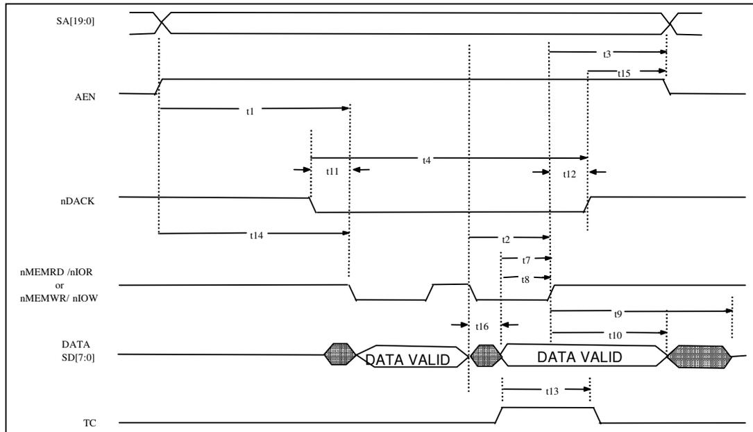
**FIGURE 19 - DMA TIMING (BURST TRANSFER MODE)**
