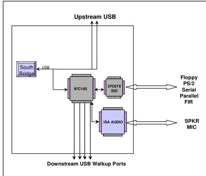
FIGURE 2 – USB97C102 CONFIGURED IN A PC MOTHERBOARD
