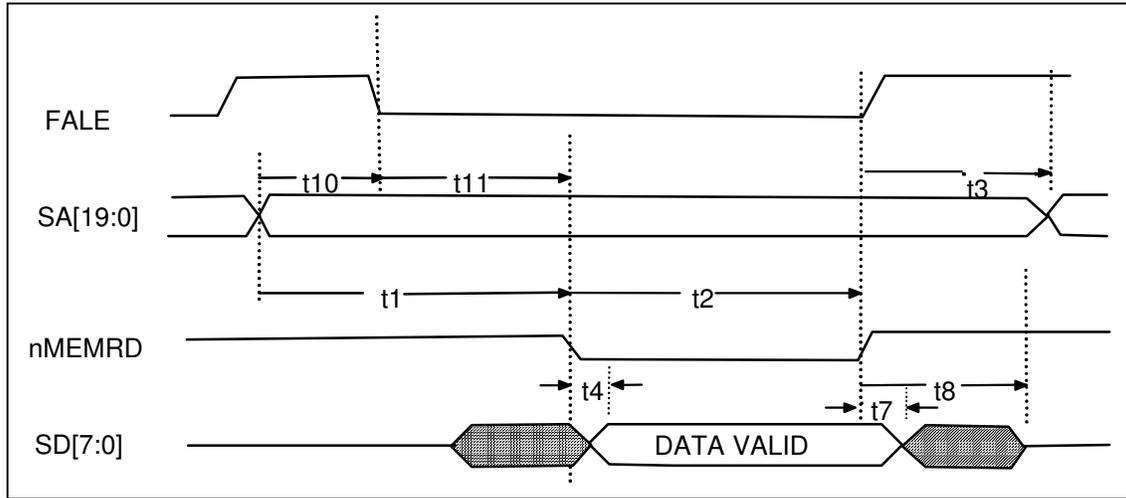
FIGURE 21 - 8051 FLASH MEMORY READ TIMING
