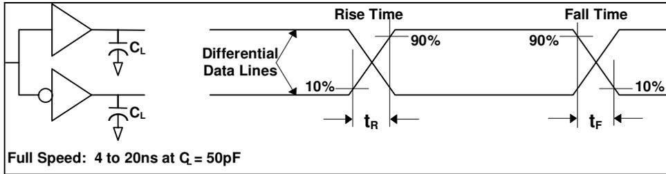
FIGURE 10 - DATA SIGNAL RISE AND FALL TIME
