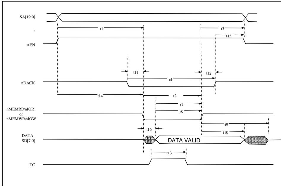
**FIGURE 18 - DMA TIMING (SINGLE TRANSFER MODE)**
