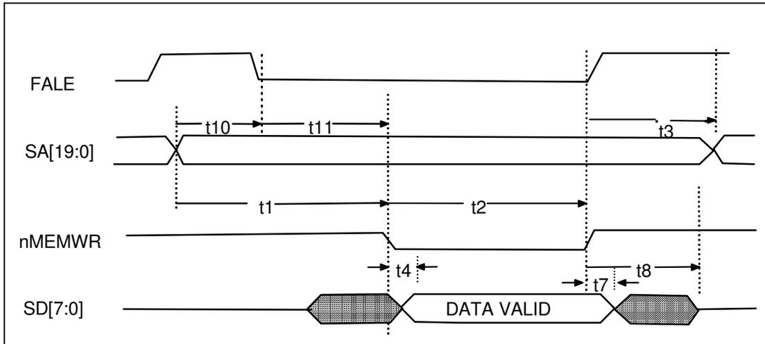
**FIGURE 22 - 8051 FLASH MEMORY WRITE TIMING**
