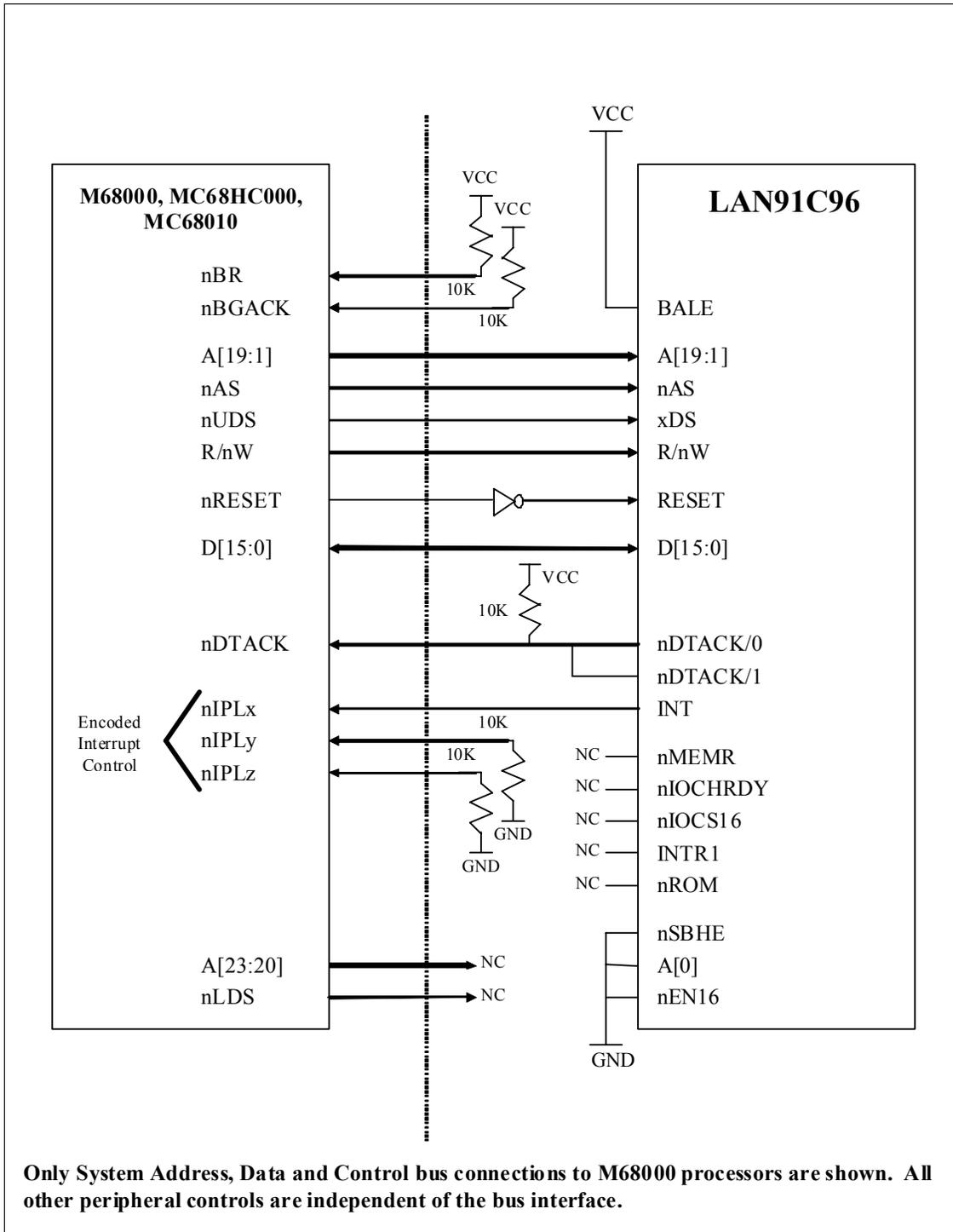
Figure 2.2 – MC68000, MC68HC000, AND MC68010 (16-BIT PROCESSORS)
