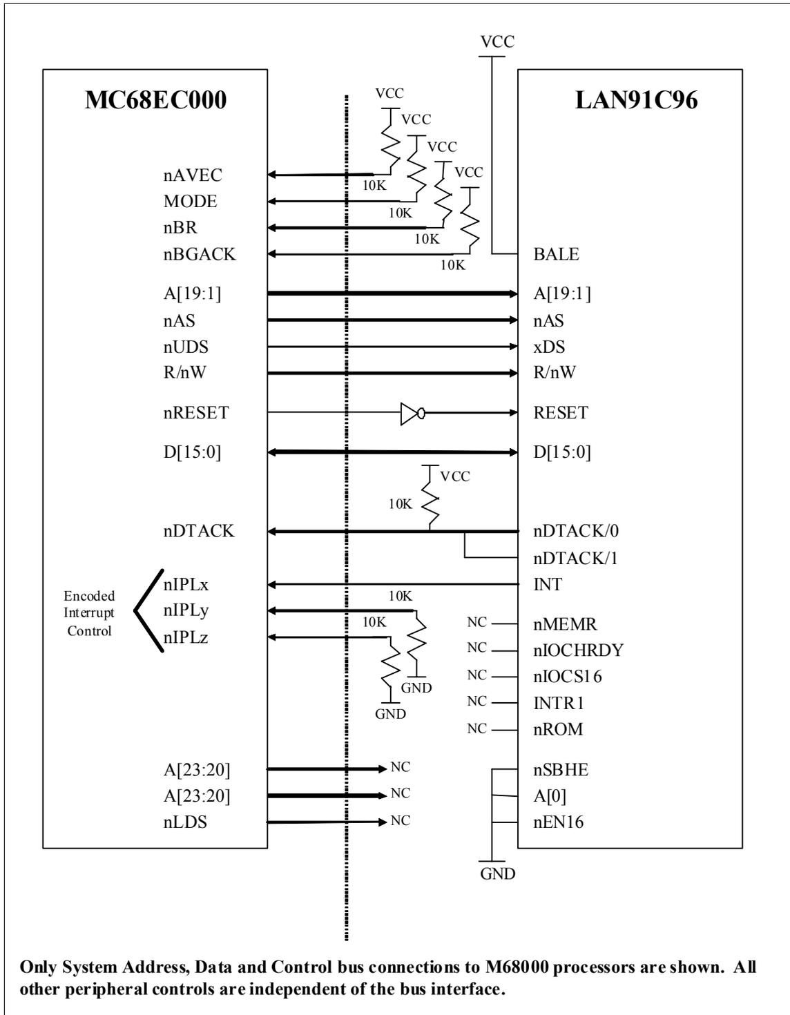
Figure 2.4 - MC68EC000 (8-/16-BIT PROCESSOR)
