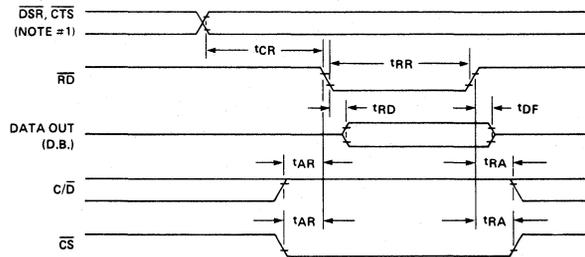
NOTE #1:  $t_{CR}$  INCLUDES THE EFFECT OF  $\overline{CTS}$  ON THE TxENBL CIRCUITRY.
