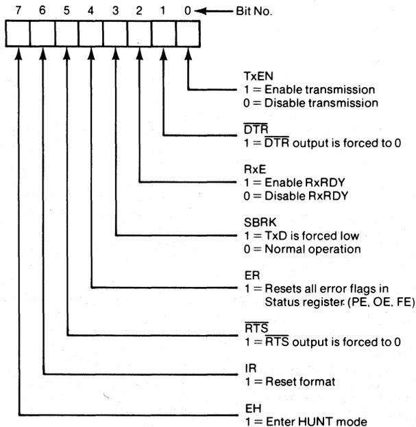
**Figure 2. Synchronous Mode Control Code.**
