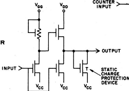
NOTE: Output driver capable of driving one TTL load with no external resistor. Capable of driving two TTL loads using an external 6.8KΩ resistor to V<sub>GG</sub>
