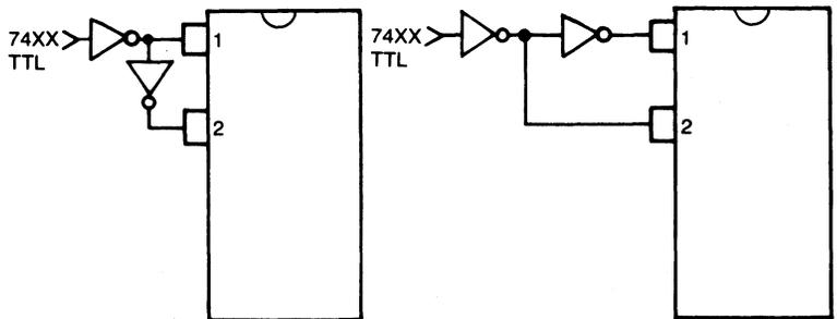
74XX—totem pole or open collector output (external pull-up resistor required)
