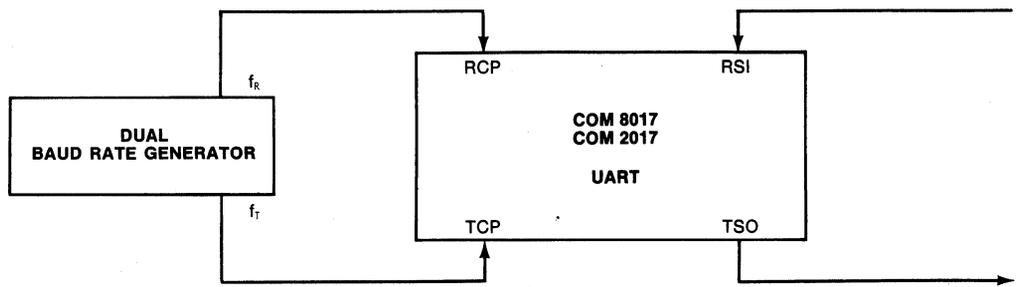
**Typical UART—Dual Baud Rate Generator Configuration
