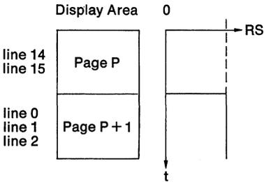
To properly maintain the memory address when displaying more than two pages, EOP pulses low at the point in time when page P is scrolled completely off the screen. At this time, RS will remain low for the entire frame since page P + 1 is now the only displayed page. The circuit at the right will allow scrolling through 4 pages of memory.
