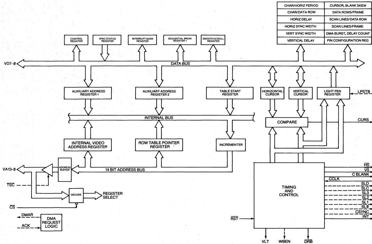
Figure 1. CRT9007 Block Diagram
