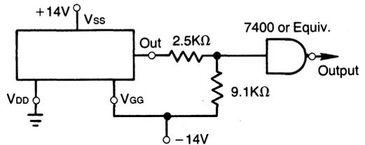
$t_r = t_f < 50$  ns for all timing diagram forcing functions.
