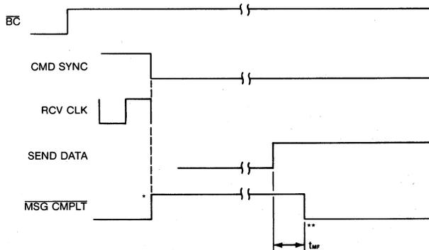
\*WORD COUNTER PRESET TO TRANSMIT COMMAND WORD FIELD PLUS 1. THIS ALLOWS FOR THE STATUS WORD.
