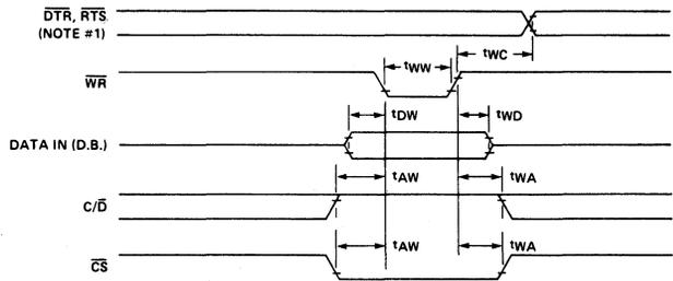
NOTE #1:  $T_{WC}$  INCLUDES THE RESPONSE TIMING OF A CONTROL BYTE.
