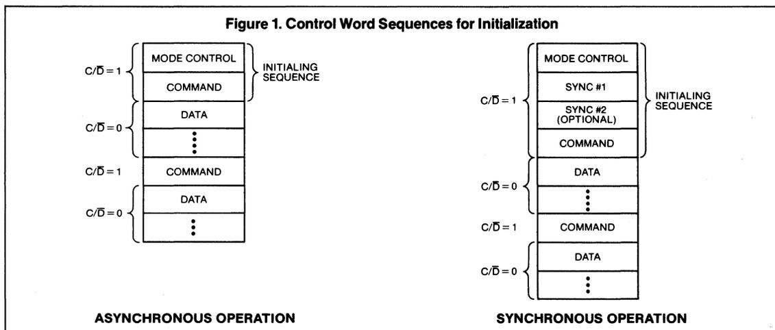
The COM 8251A may be initialized following a system RESET or prior to starting a new serial I/O sequence. The USART must be RESET (external or internal) following power up and subsequently may be reset at any time following completion of one activity and preceding a new set of operations. Following a reset, the COM 8251A enters an idle state in which it can neither transmit nor receive data.
