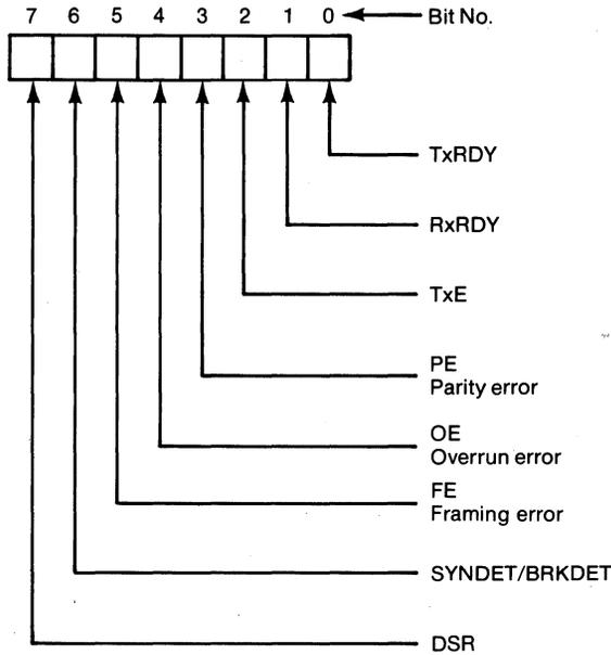
TxE signals the processor that the Transmit Register is empty.
