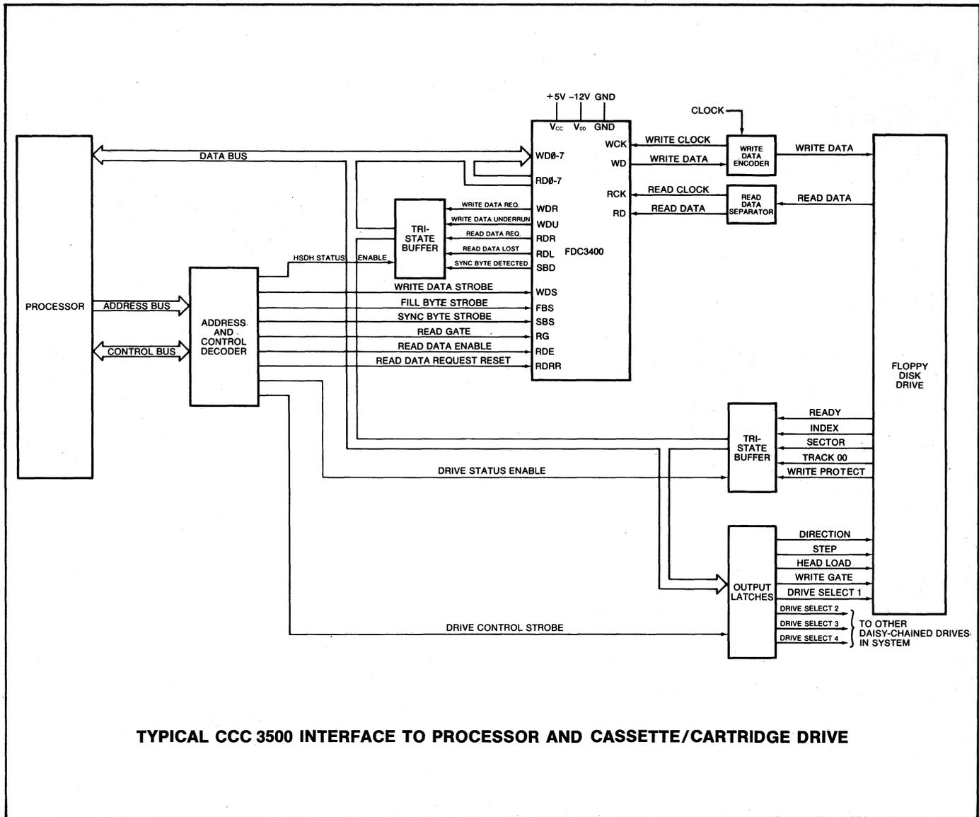
**TYPICAL CCC 3500 INTERFACE TO PROCESSOR AND CASSETTE/CARTRIDGE DRIVE**
