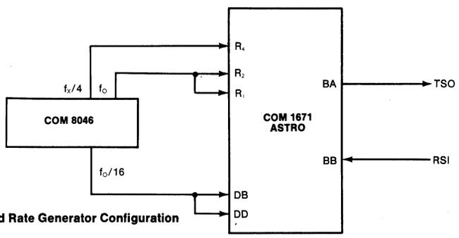
**Typical ASTRO—Baud Rate Generator Configuration**
