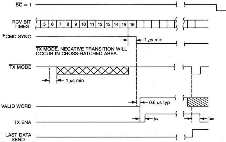
\*THIS IS A CMD WORD BEING RECEIVED. IT IS ADDRESSED TO THIS BUFFER AND THE T/R BIT = 1. TX ENA IS RESET BY 2ND TX MODE NEGATIVE TRANSITION OR BY LAST SEND DATA (MESSAGE COMPLETE FUNCTION).
