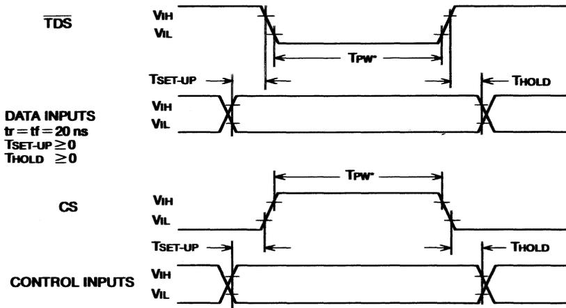
\*Input information (Data/Control) need only be valid during the last  $T_{pw}$ , min time of the input strobes (TDS, CS).
