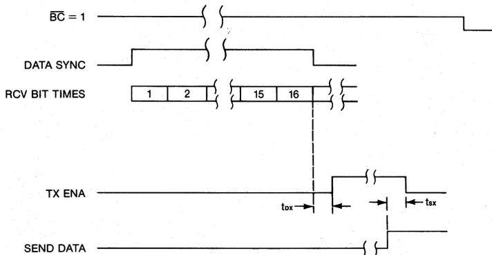
\*\*THIS IS THE LAST DATA WORD BRING RECEIVED. THIS TERMINAL PREVIOUSLY HAD RECEIVED A REC CMD WORD WITH OUR ADDRESS AND A REC/XMIT BIT = 0 DURING THIS MESSAGE SEQUENCE. TX ENABLE IS SET BY MSG CMLPT FUNCTION AND RESET BY RECEIPT OF SEND DATA.
