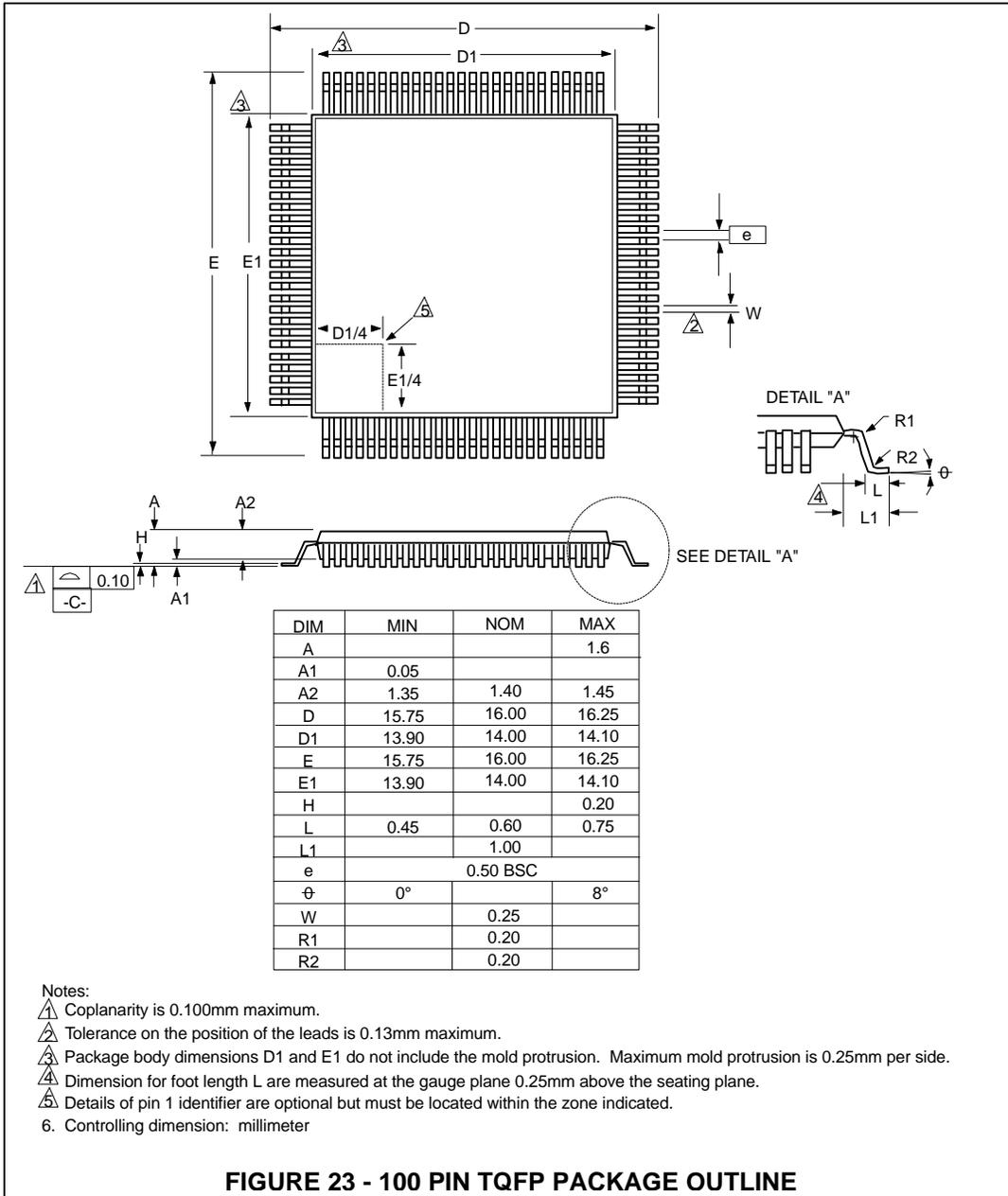
**FIGURE 23 - 100 PIN TQFP PACKAGE OUTLINE**
