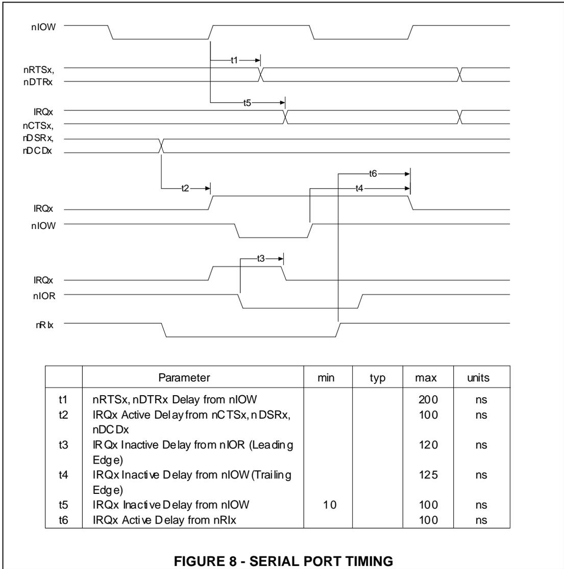
**FIGURE 8 - SERIAL PORT TIMING**
