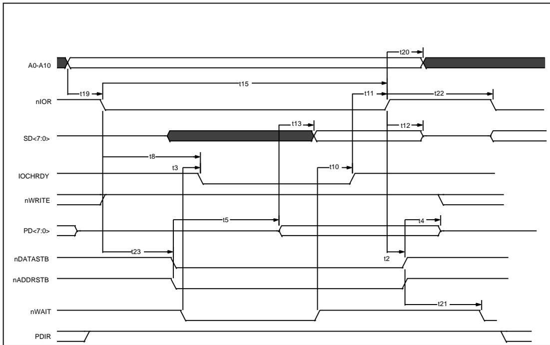
**FIGURE 16A - EPP 1.7 DATA OR ADDRESS READ CYCLE**
