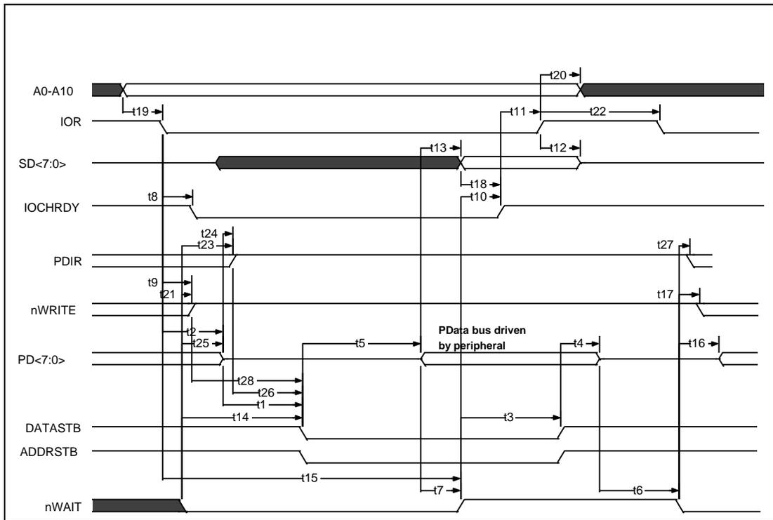
**FIGURE 14A - EPP 1.9 DATA OR ADDRESS READ CYCLE**
