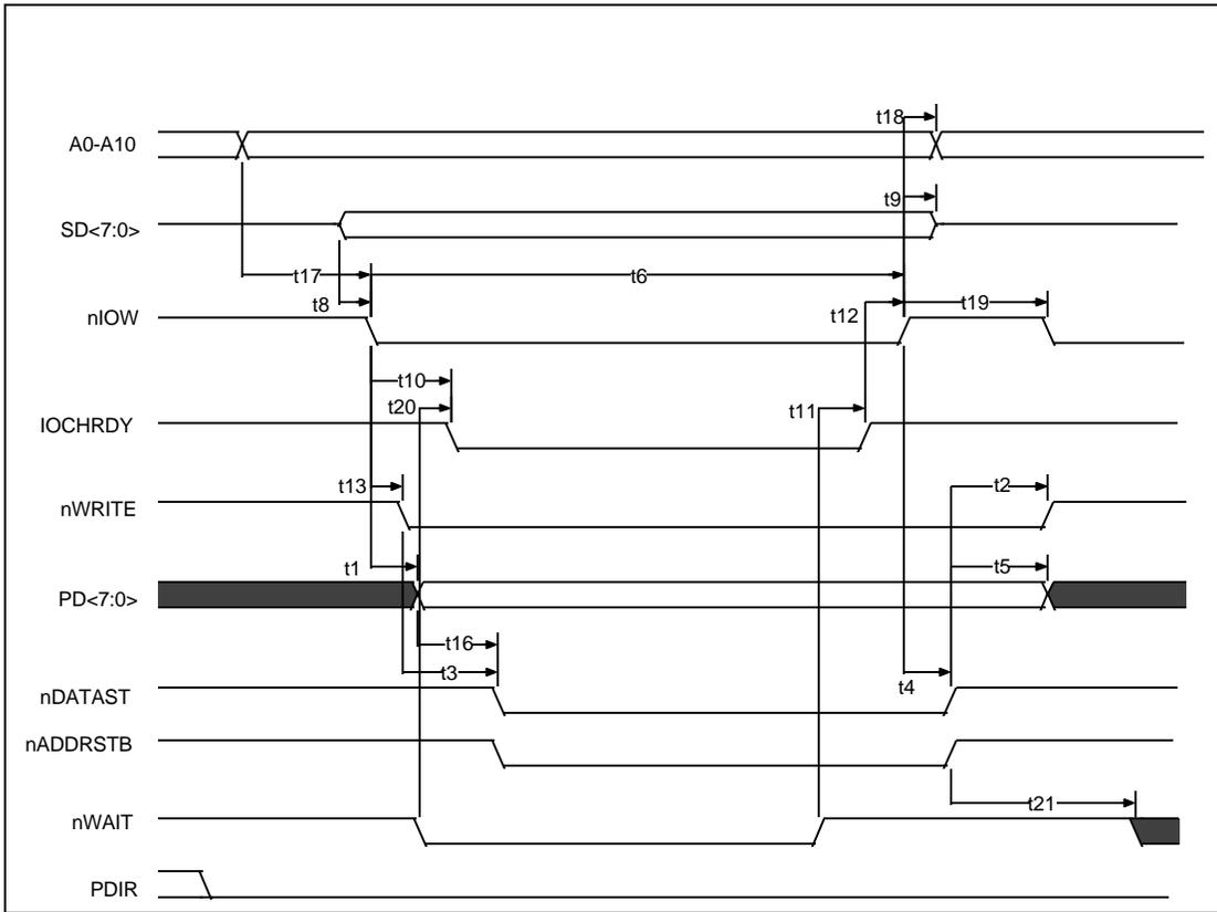
**FIGURE 15A - EPP 1.7 DATA OR ADDRESS WRITE CYCLE**
