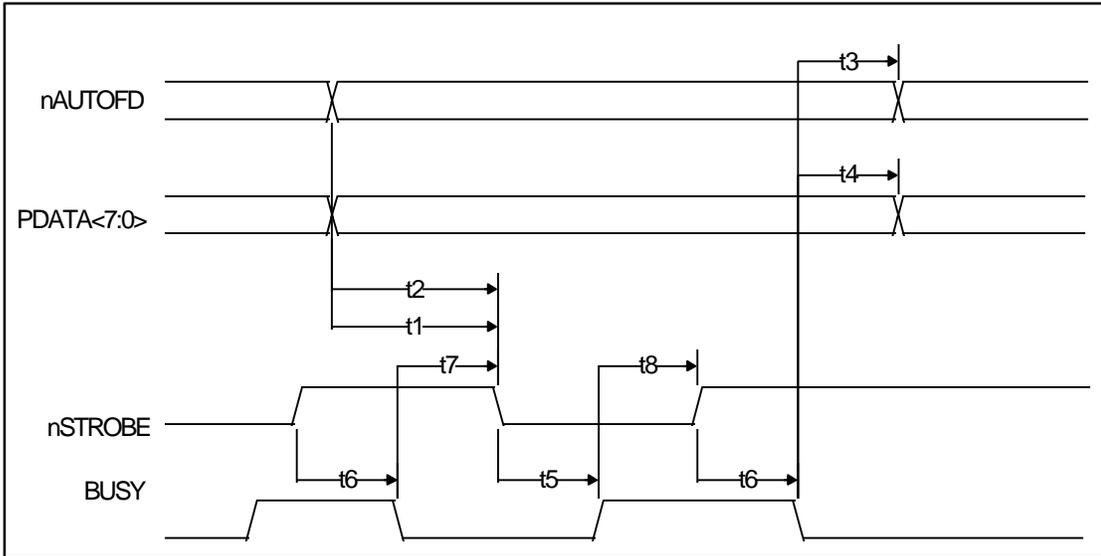
**FIGURE 18 - ECP PARALLEL PORT FORWARD TIMING**
