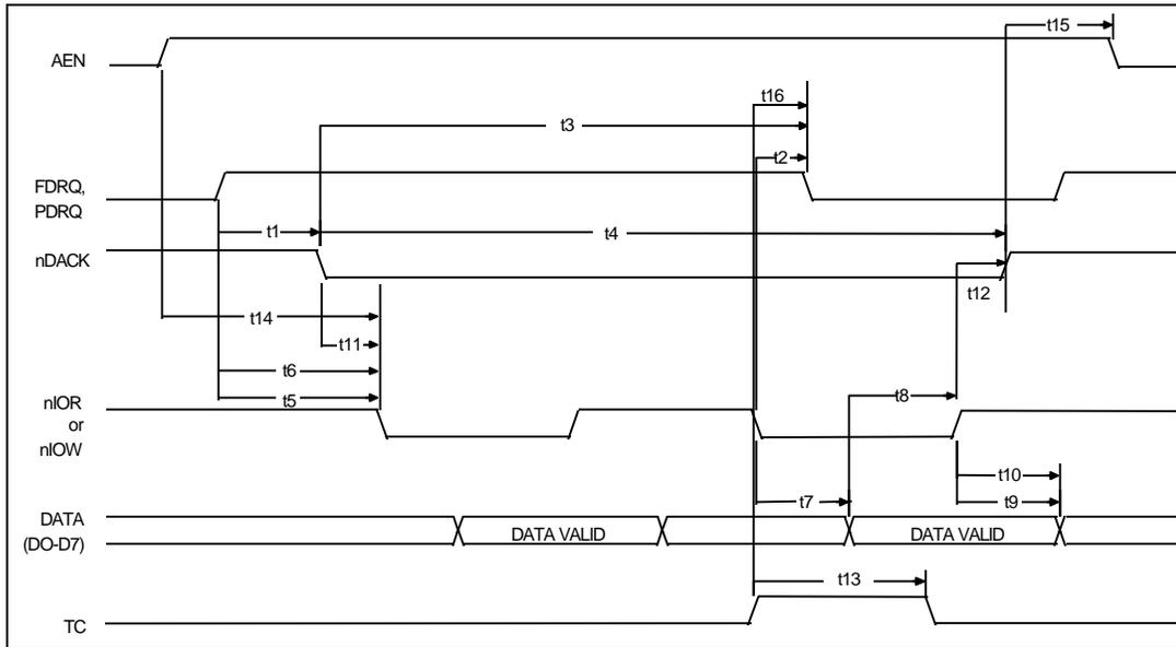
**FIGURE 9B - DMA TIMING (BURST TRANSFER MODE)**
