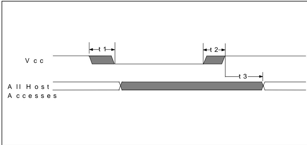
**FIGURE 4 - POWER-UP TIMING**
