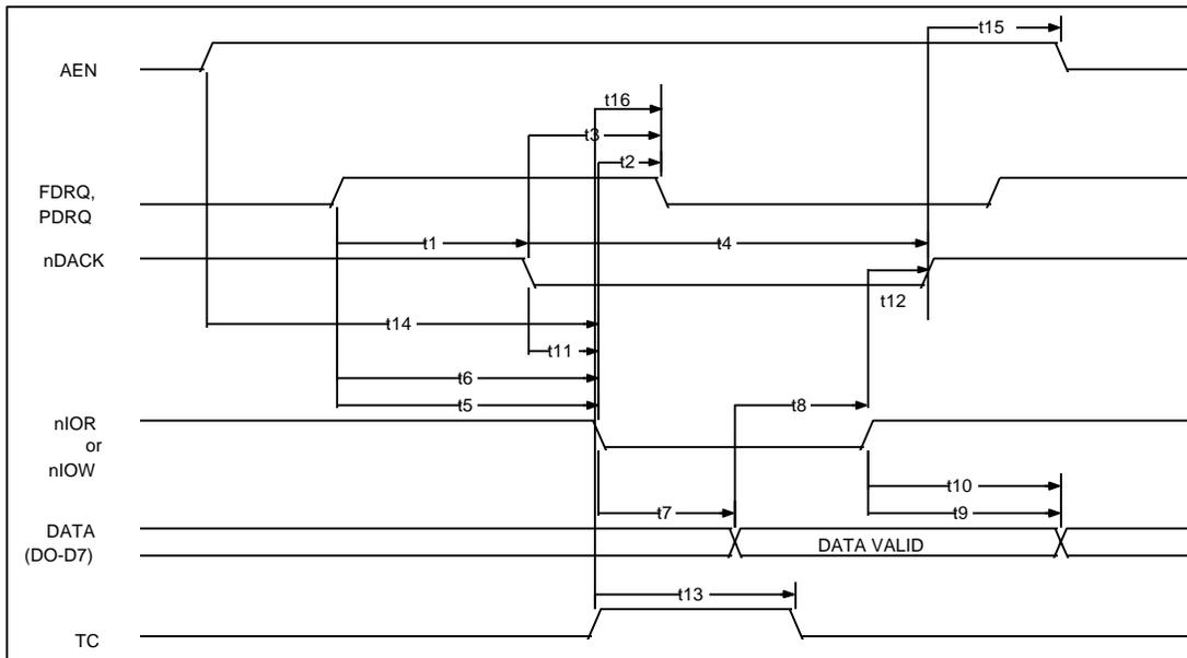
**FIGURE 9A - DMA TIMING (SINGLE TRANSFER MODE)**
