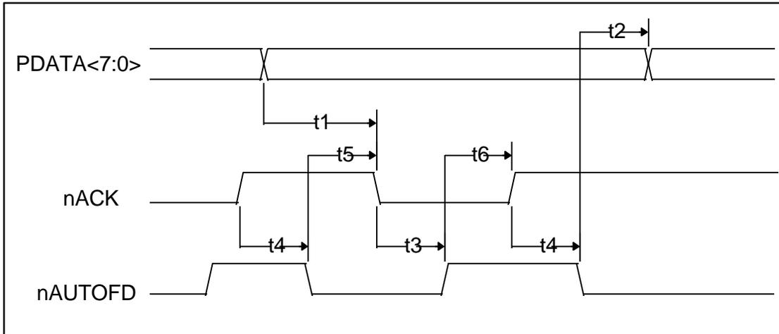
**FIGURE 19 - ECP PARALLEL PORT REVERSE TIMING**
