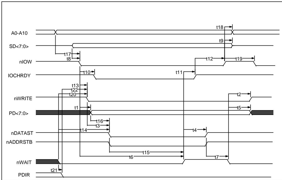
**FIGURE 13A - EPP 1.9 DATA OR ADDRESS WRITE CYCLE**
