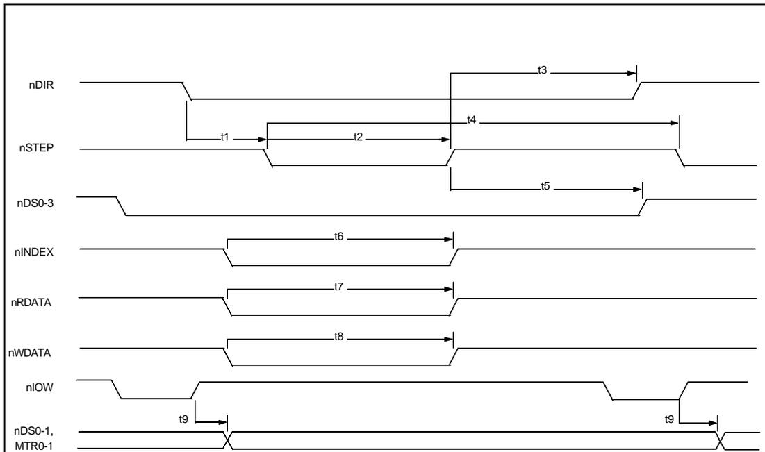
**FIGURE 10 - DISK DRIVE TIMING (AT MODE ONLY)**
