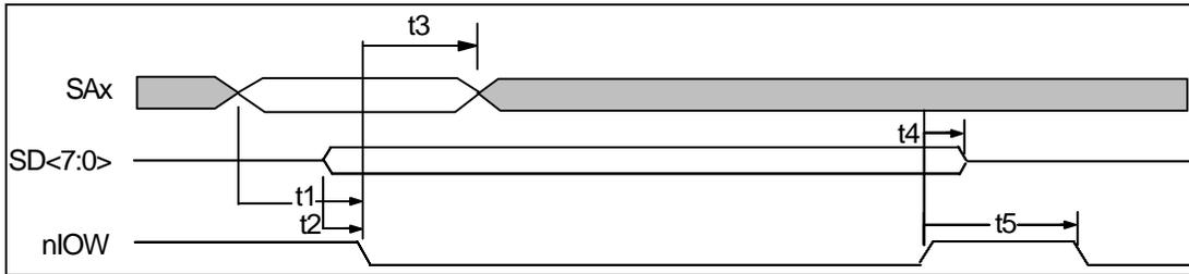
**FIGURE 3 - IOW TIMING FOR PORT 92**
