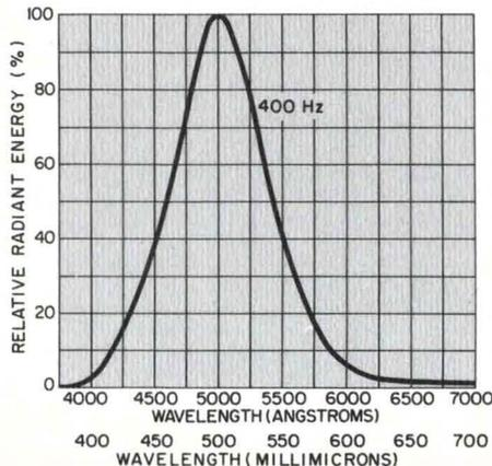
Fig. 4. Spectral emission characteristics, metal-glass and all-glass EL readout panels. Light output very closely matches the response of the human eye, permitting easy prolonged viewing.
