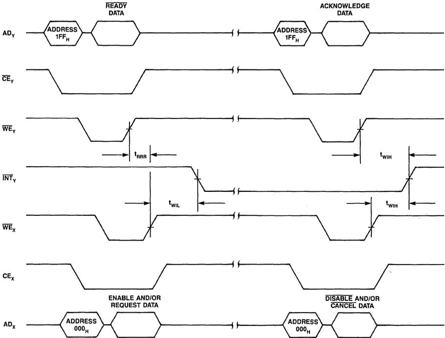
Figure 6. Interrupt Request Timing
