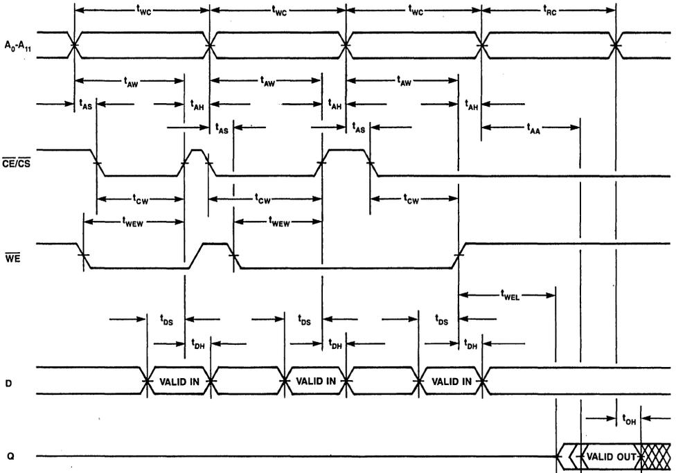
**Figure 3. Write-Write-Write-Read Timing**
