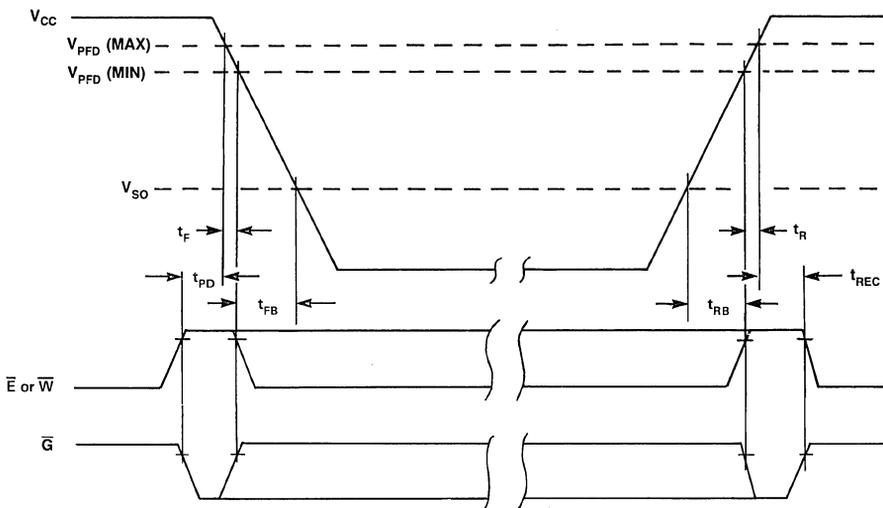
Figure 6. Power-Down/Power-Up Timing
