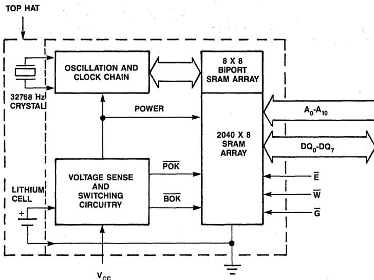
Figure 2. Block Diagram
