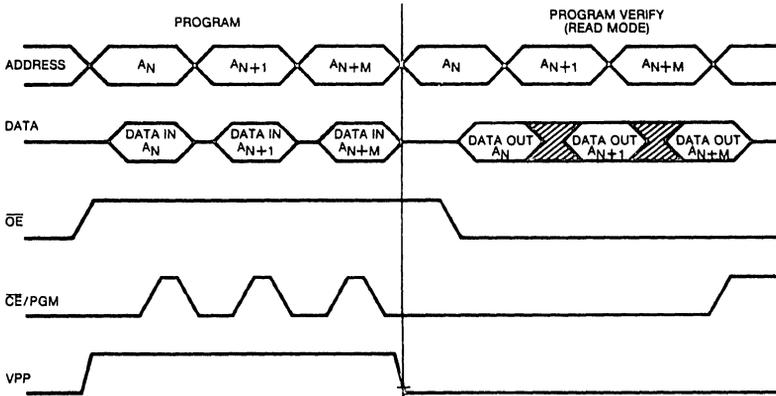
\* All timings are the same as the single address programming mode. A dummy read is required only if the last programmed byte is the first byte to be verified.
