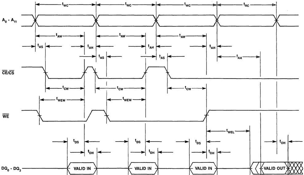
Figure 3. Write-Write-Write-Read Timing
