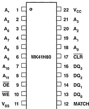
Figure 1. Pin Connections
