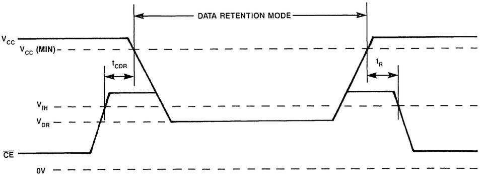
Figure 4. Data Retention Timing
