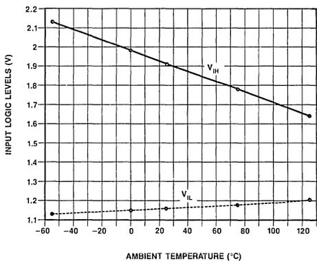
LOGIC THRESHOLD VOLTAGE VS.
