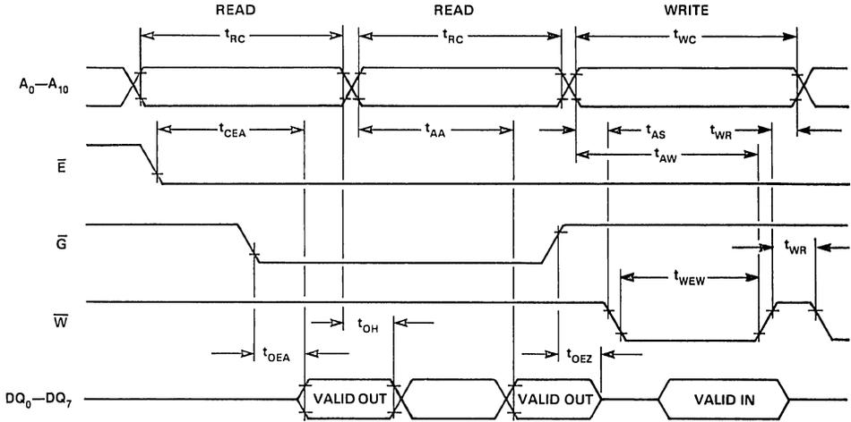
Figure 3. Read-Read-Write Timing
