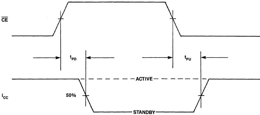
Figure 5. Standby Mode Timing
