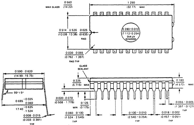
**UV Window Cavity Dual-In-Line Package (Q)**
