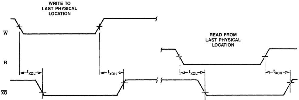
Figure 11. Expansion Out Timing
