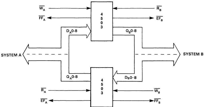
Figure 14. Bidirectional FIFO Application
