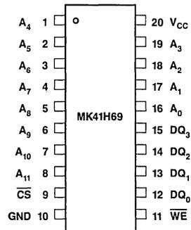
Figure 1. Pin Connections
