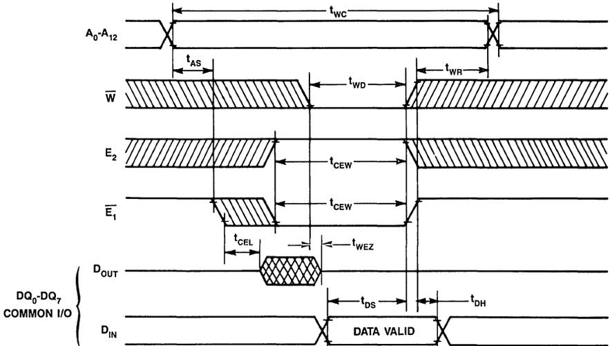
Figure 5. Write Cycle 2 ( $\overline{E}_1$  Controlled Write)
