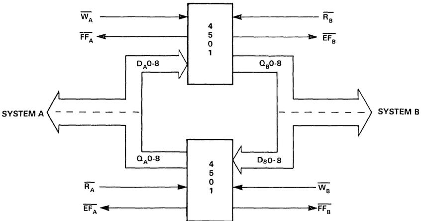
Figure 13. Bidirectional FIFO Application
