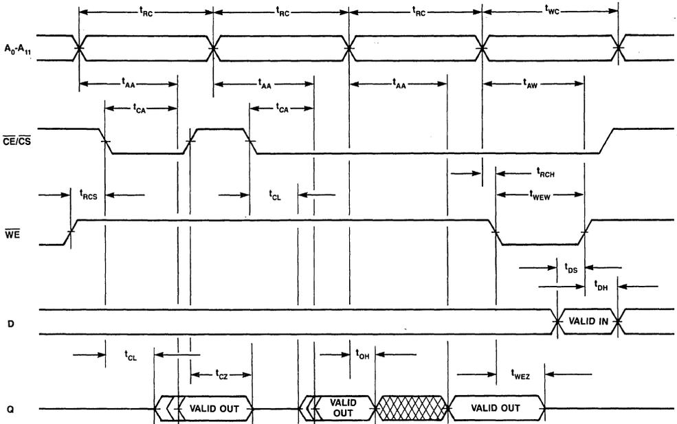
Figure 2. Read-Read-Read-Write Timing
