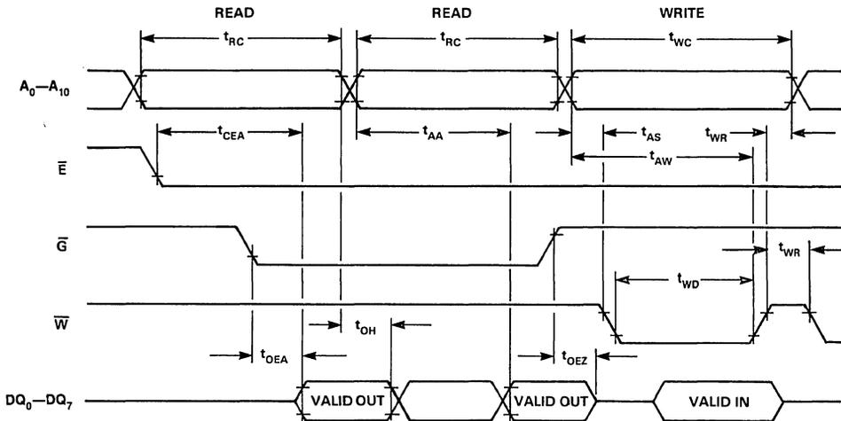
Figure 3. Read-Read-Write Timing
