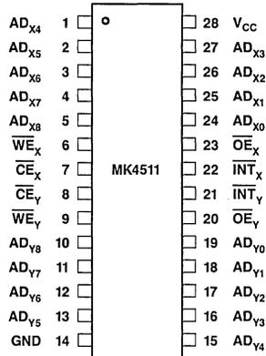
Figure 1. Pin Connections
