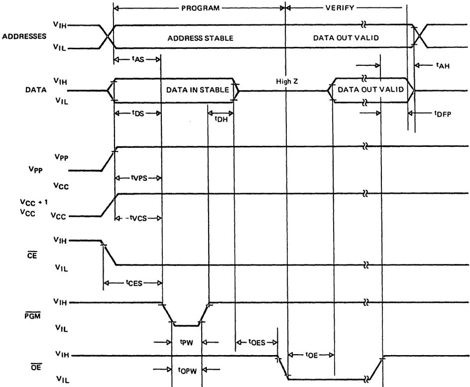
1. The input timing reference level is 0.8V for  $V_{IL}$  and 2.0V for  $V_{IH}$ .
