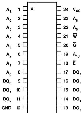
**Figure 1. Pin Connections**
