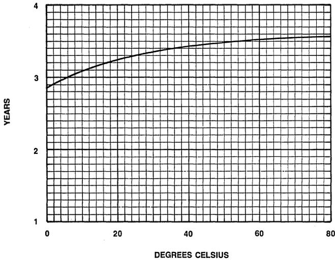
Figure 12. Current Consumption Life Over Temperature with 0%  $V_{CC}$  Duty Cycle
