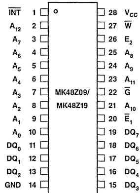
**Figure 1. Pin Connections**
