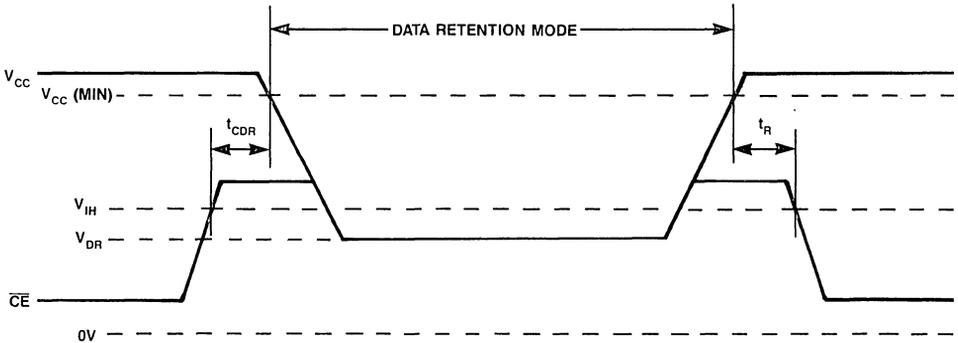
Figure 4. Data Retention Timing
