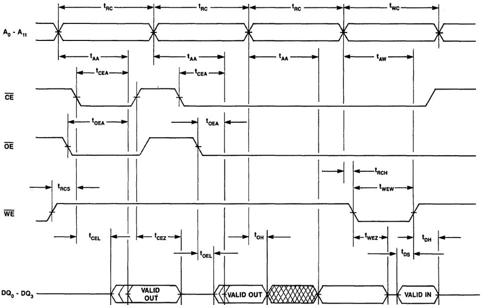
Figure 2. Read-Read-Read-Write Timing
