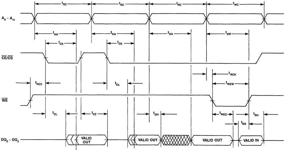
**Figure 2. Read-Read-Read-Write Timing**
