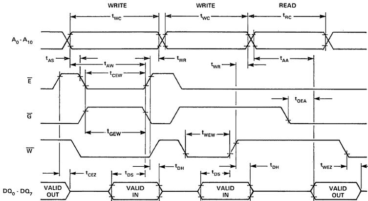
Figure 4. Write-Write-Read Timing
