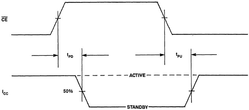
Figure 5. Standby Mode Timing
