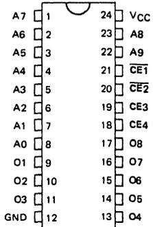
VCC : Power supply voltage (DC + 5 V)
