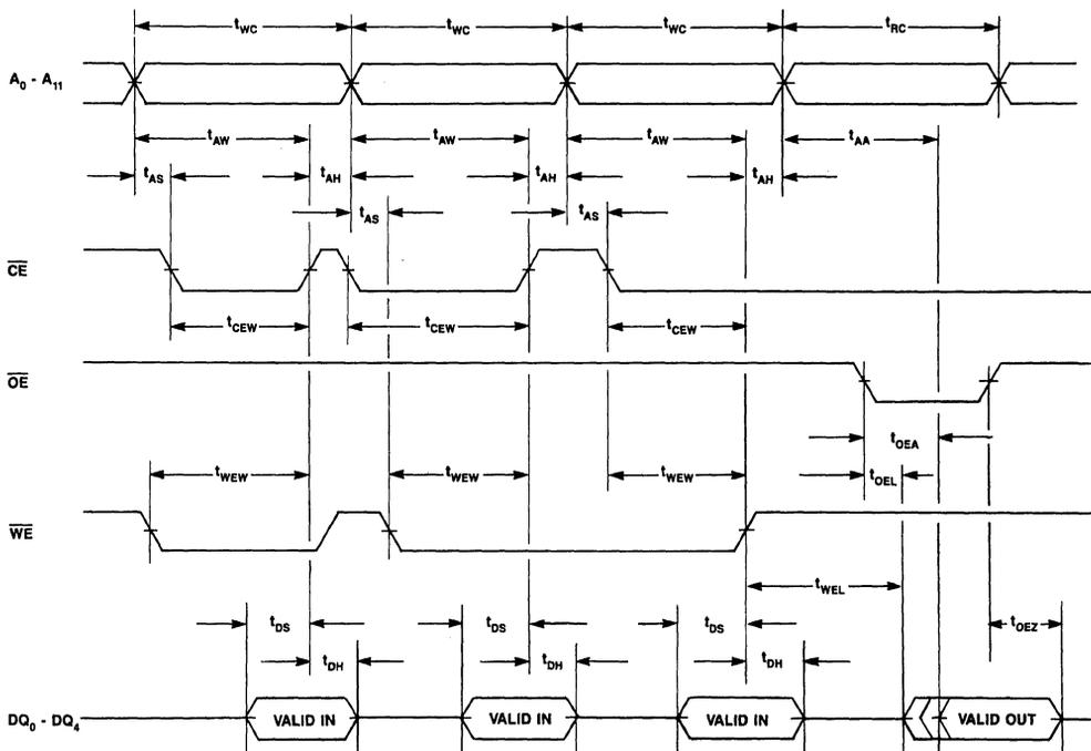
Figure 3. Write-Write-Write-Read Timing
