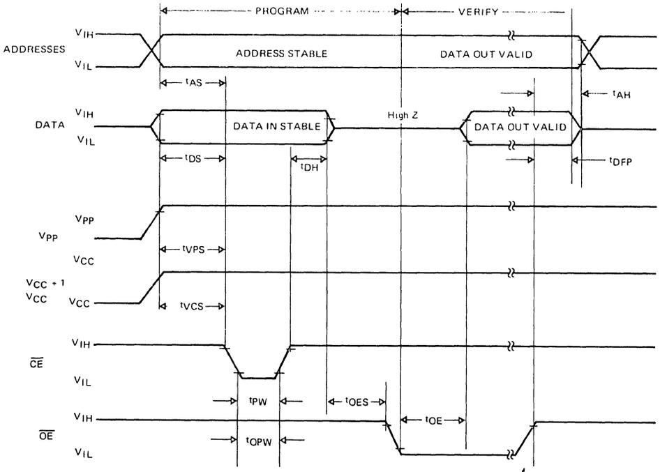
1. The input timing reference level is 0.8V for  $V_{IL}$  and 2.0V for  $V_{IH}$ .
