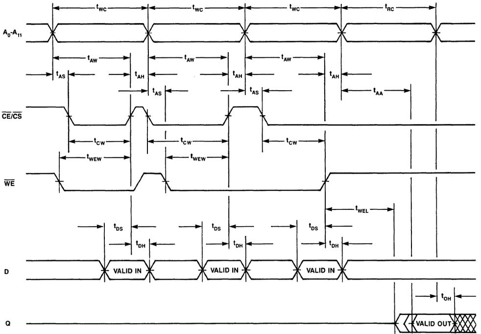
Figure 3. Write-Write-Write-Read Timing
