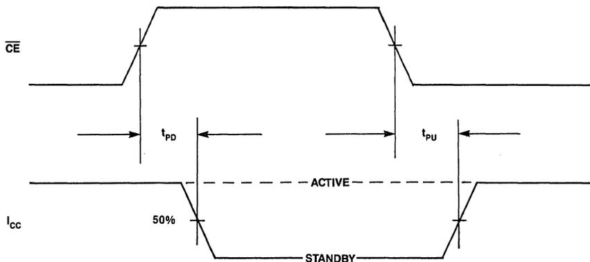
Figure 5. Standby Mode Timing
