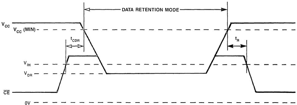
Figure 4. Data Retention Timing
