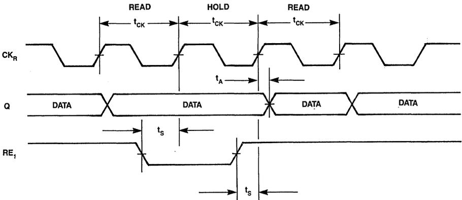
Figure 5. Hold Cycle Timing
