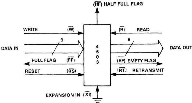
Figure 7. A Single 2048 x 9 FIFO Configuration
