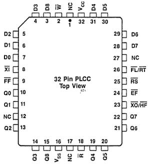
Figure 1. Pin Connections
