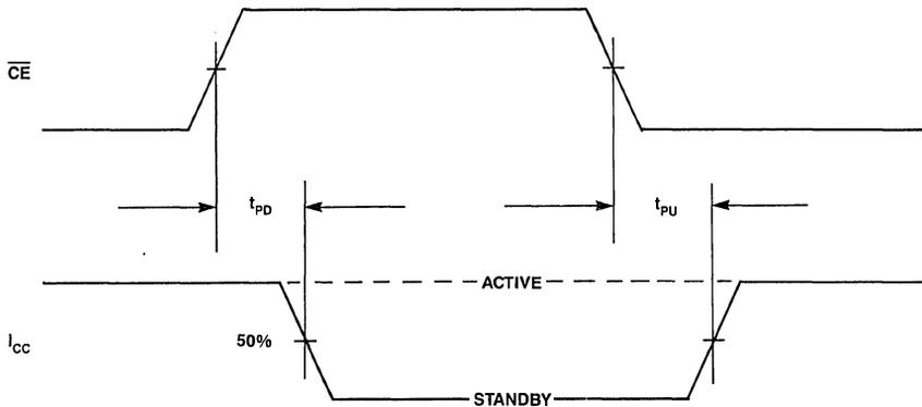
Figure 5. Standby Mode Timing
