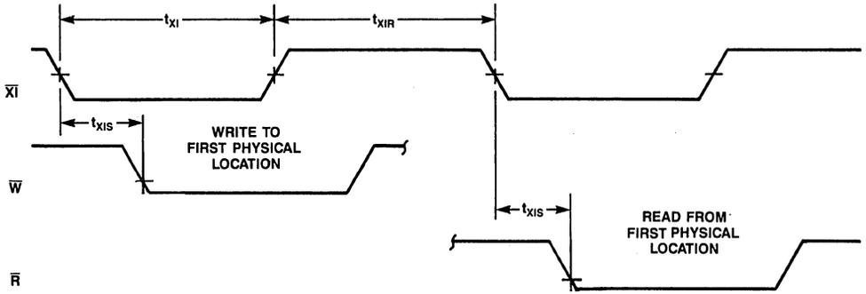
Figure 11. Expansion In Timing
