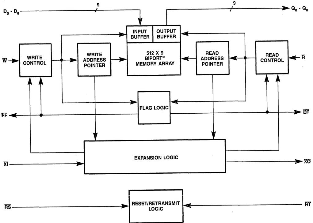
Figure 2. MK4501 Block Diagram
