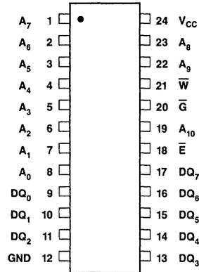
Figure 1. Pin Connections
