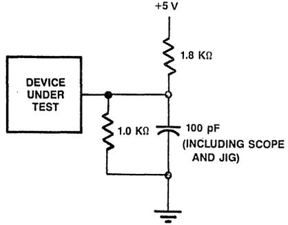
Figure 10. Output Load Diagram
