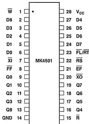
Figure 1. Pin Connections
