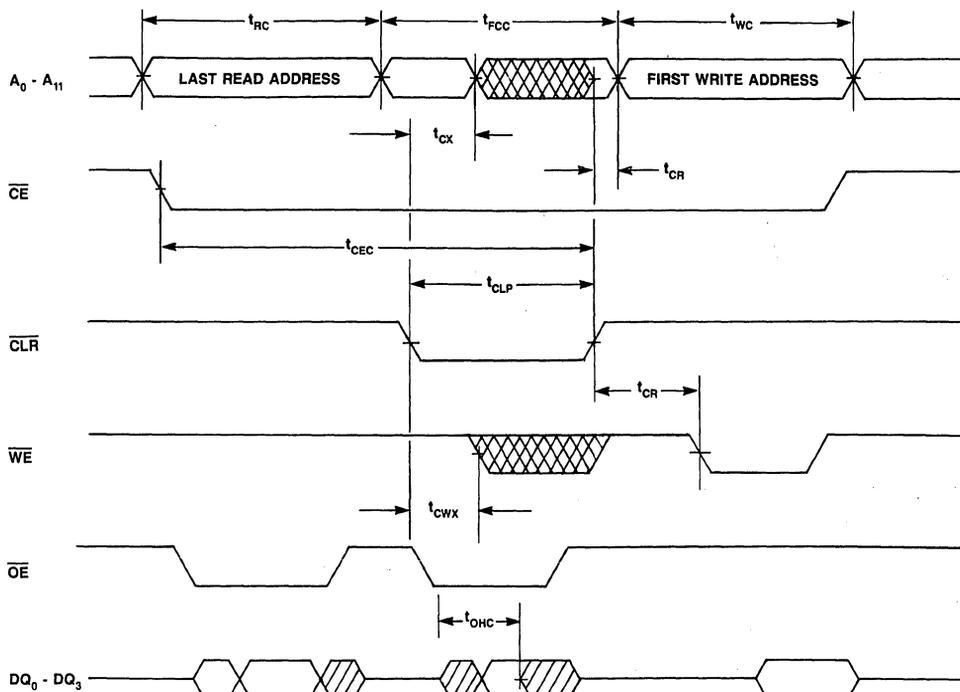
Figure 5. Last Read-Flash Clear-First Write
