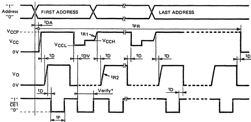
\* Programming verification at both max and min V<sub>CC</sub> is optional (V<sub>CCH</sub>, V<sub>CCL</sub>).
