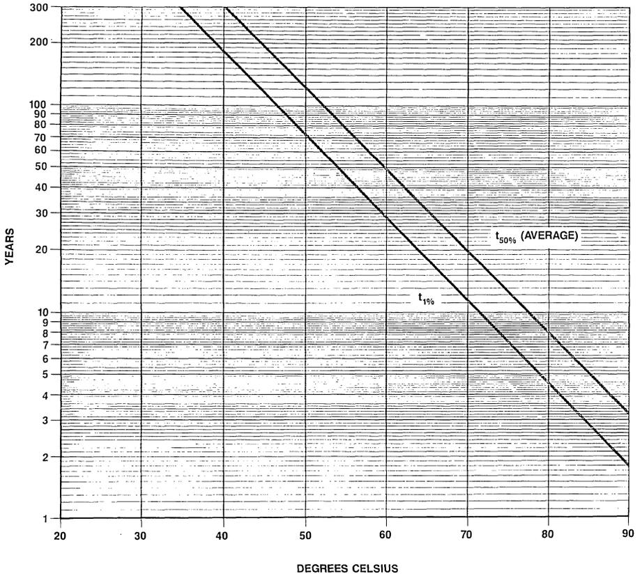
Figure 9. MK48Z08/18/09/19 Predicted Battery Life vs Temperature
