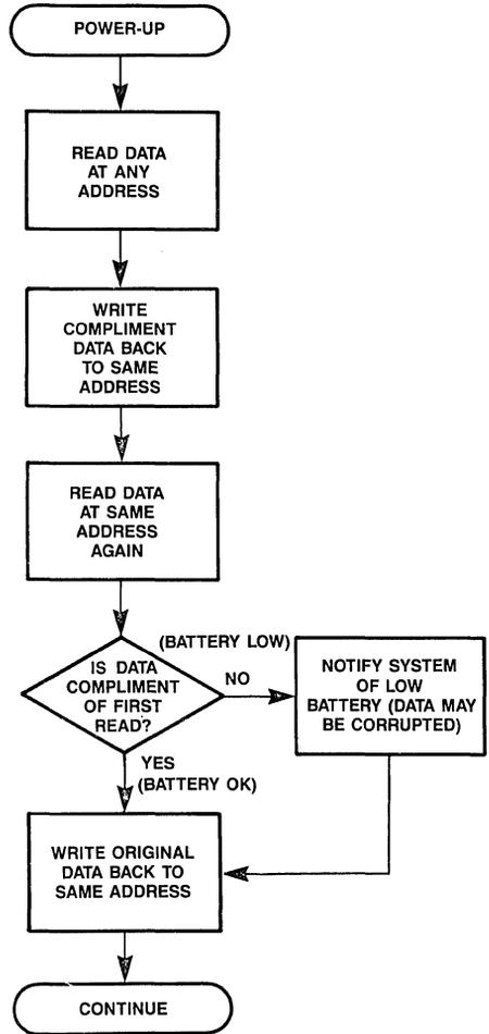
Figure 8. Checking the  $\overline{BOK}$  Flag Status
