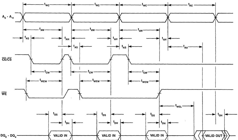
Figure 3. Write-Write-Write-Read Timing
