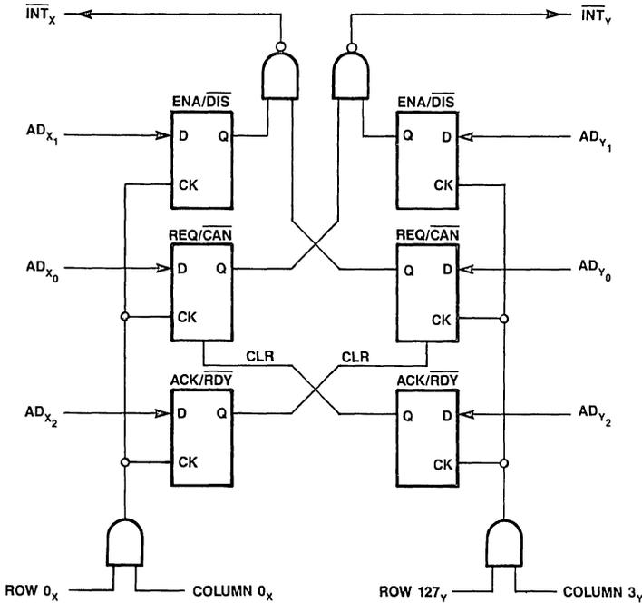
Figure 5. MK4511 Interrupt Control Registers and Interrupt Logic
