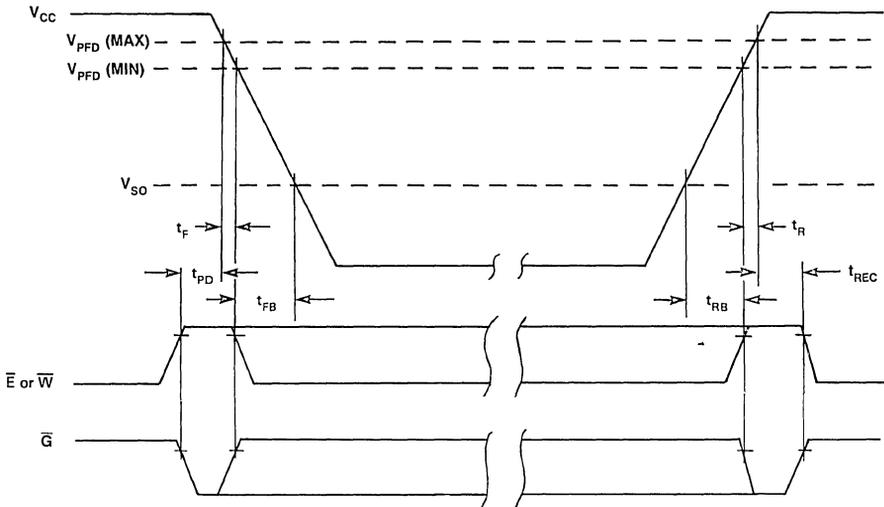
Figure 9. Power-Down/Power-Up Timing
