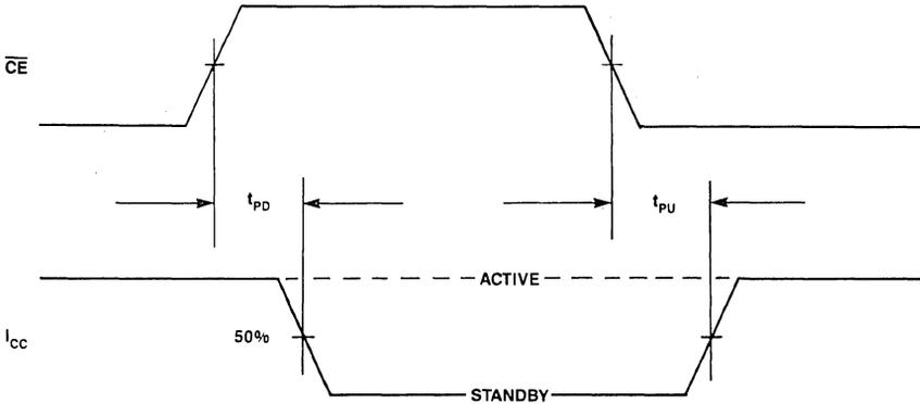
Figure 5. Standby Mode Timing
