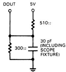
Fig. 1 – Output Load
