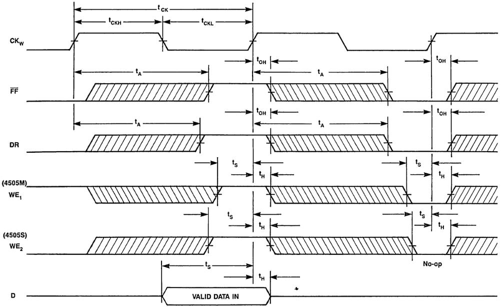
Figure 3. Write Cycle Timing
