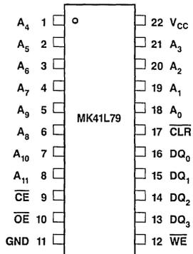
Figure 1. Pin Connections
