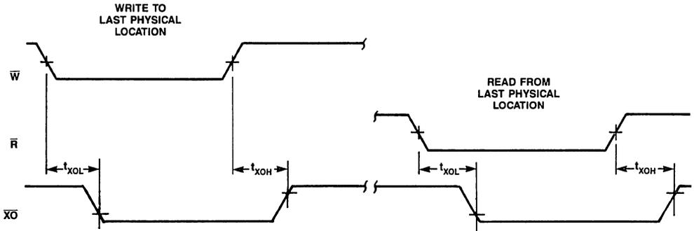
Figure 10. Expansion Out Timing
