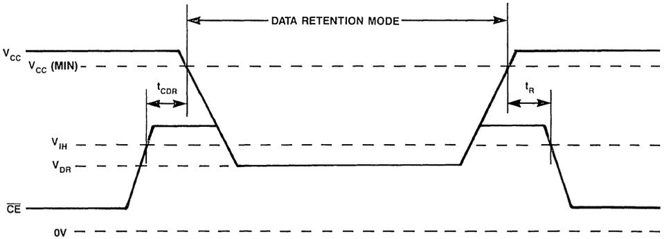
**Figure 4. Data Retention Timing**
