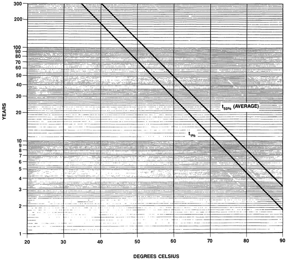
Figure 10. MK48T02/12/03/13 Predicted Battery Storage Life vs. Temperature
