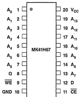
Figure 1. Pin Connections
