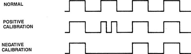
Figure 7. Adjusting the Divide by 256 Pulse Train
