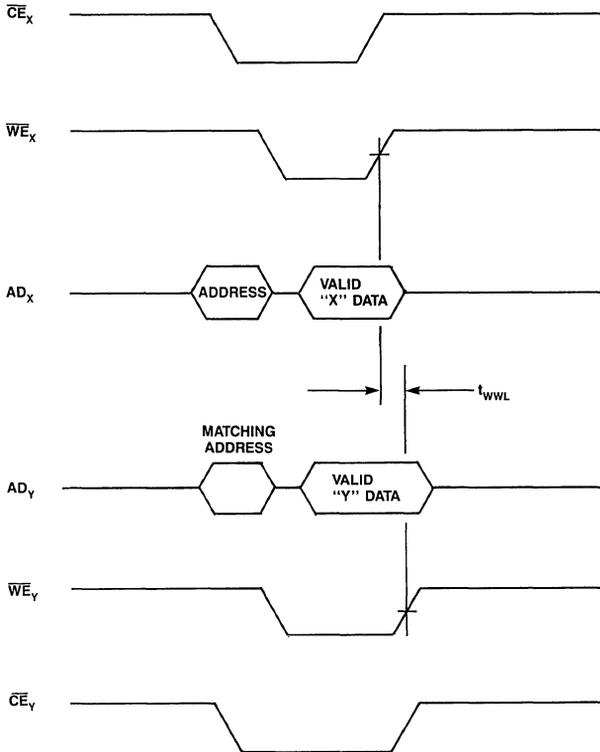
Figure 7. Minimum Write To Write Latency For Valid Data Storage
