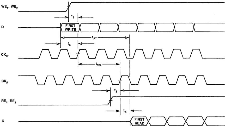
Figure 11. Simultaneous Write/Read Timing (4505S)
