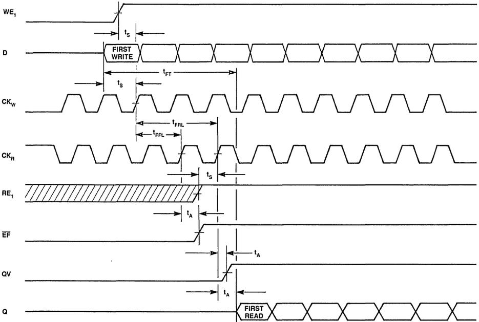
Figure 10. Simultaneous Write/Read Timing (4505M)
