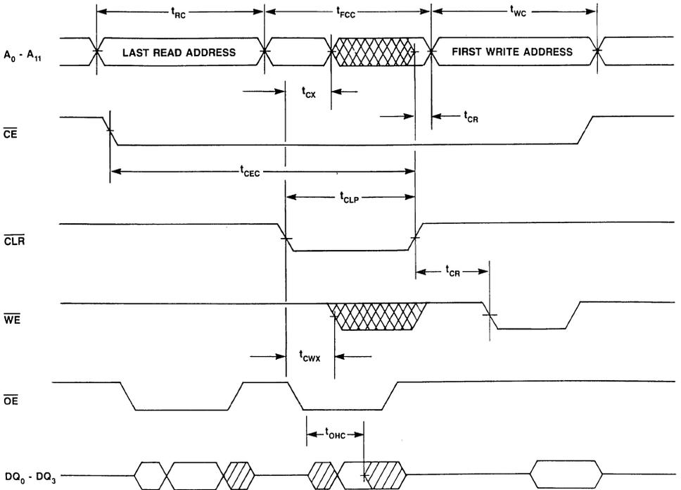
Figure 5. Last Read-Flash Clear-First Write
