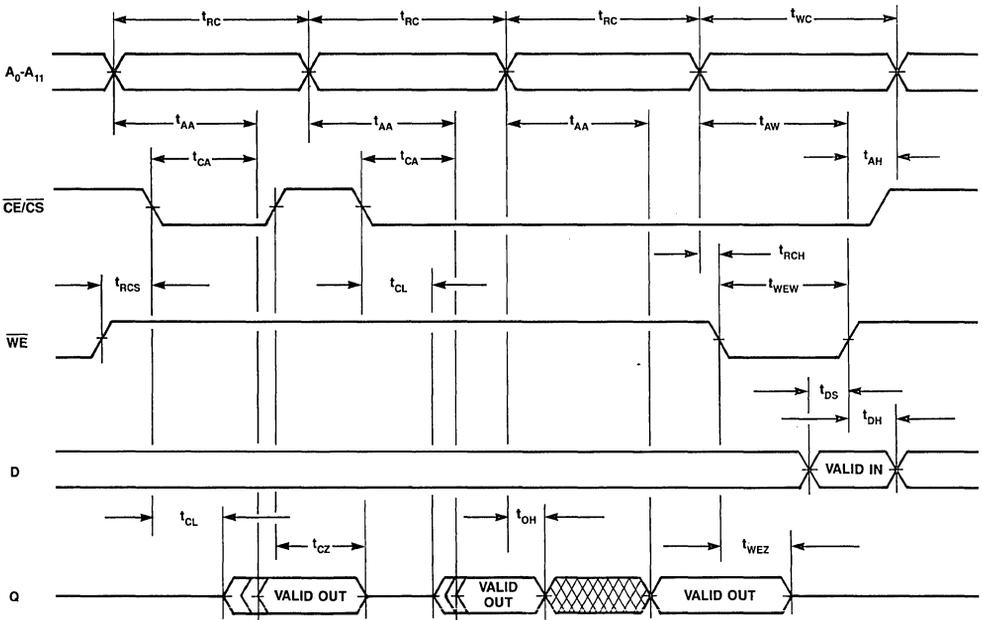
Figure 2. Read-Read-Read-Write Timing
