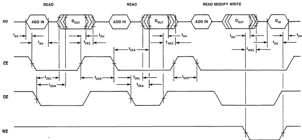
Figure 3. Read-Read-Read Modify Write
