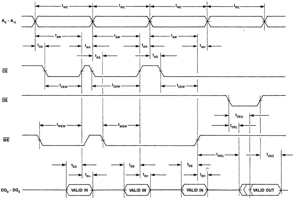
**Figure 3. Write-Write-Write-Read Timing**
