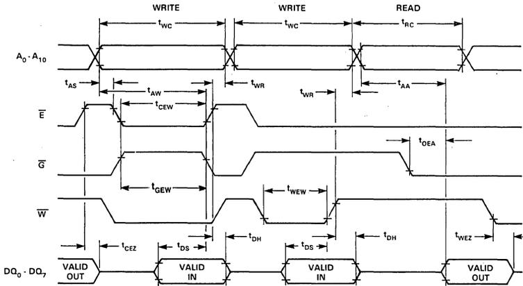
Figure 4. Write-Write-Read Timing
