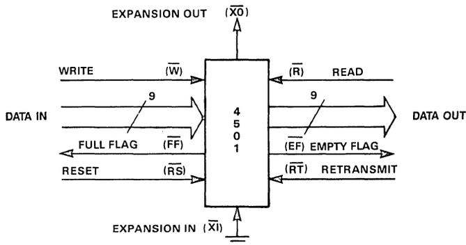
Figure 7. A Single 512 x 9 FIFO Configuration
