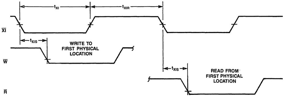
Figure 12. Expansion In Timing
