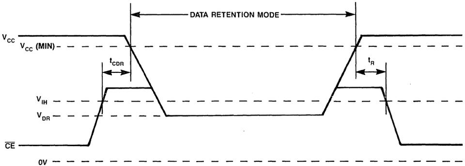
Figure 4. Data Retention Timing
