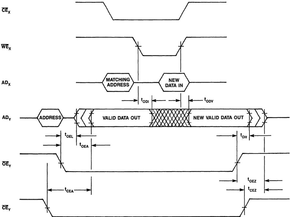
Figure 8. Simultaneous Read Write Timing
