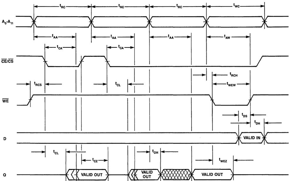
Figure 2. Read-Read-Read-Write Timing
