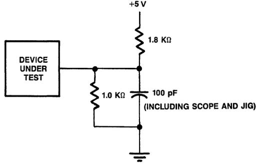
Figure 8. Output Load Diagram
