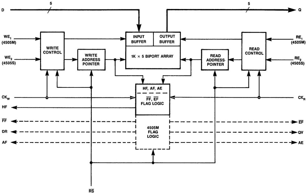
Figure 2. Block Diagram MK4505M/4505S
