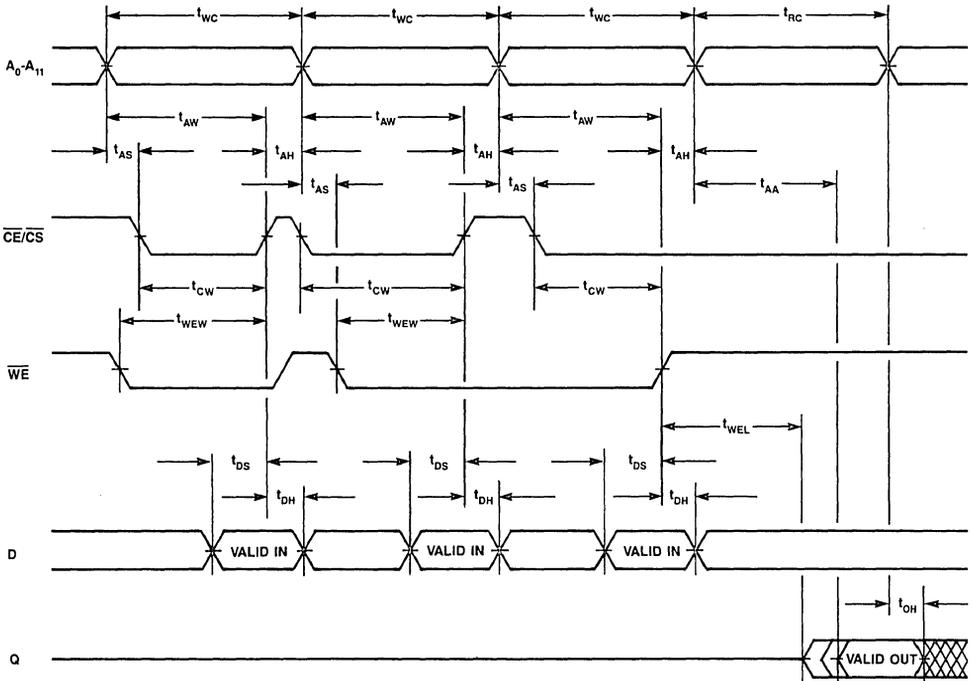
Figure 3. Write-Write-Write-Read Timing
