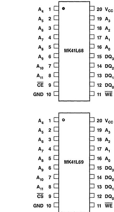
Figure 1. Pin Connections
