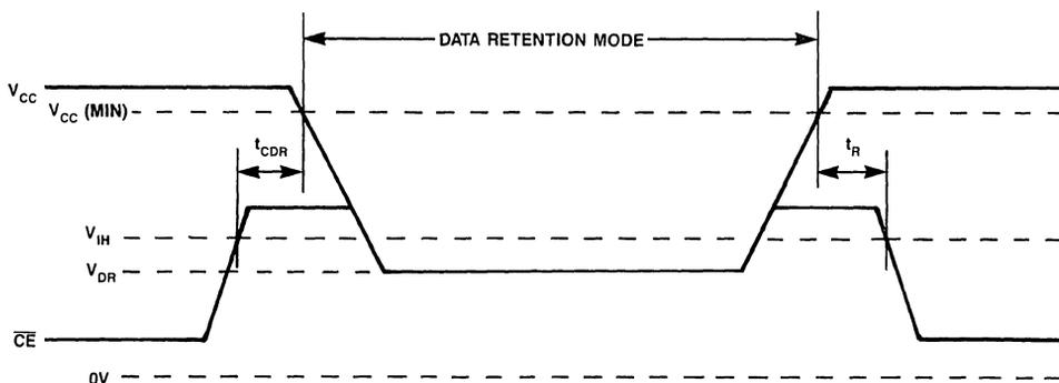
Figure 4. Data Retention Timing
