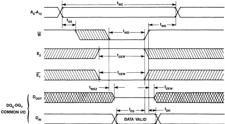
Figure 4. Write Cycle 1 ( $\overline{W}$  Controlled Write)
