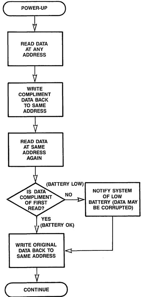
Figure 5. Checking the  $\overline{BOK}$  Flag Status
