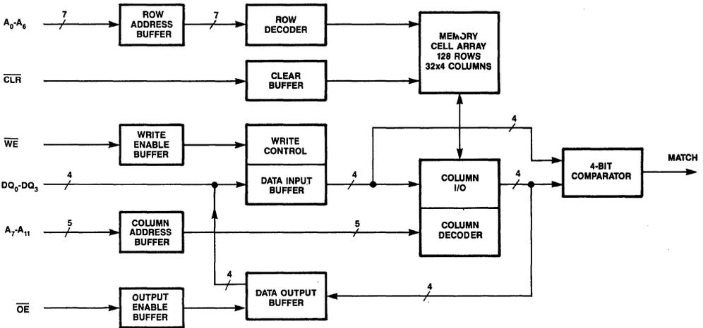
Figure 4. Block Diagram
