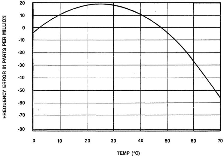
Figure 6. The MK48T02/12/03/13 Oscillator Frequency vs. Temperature
