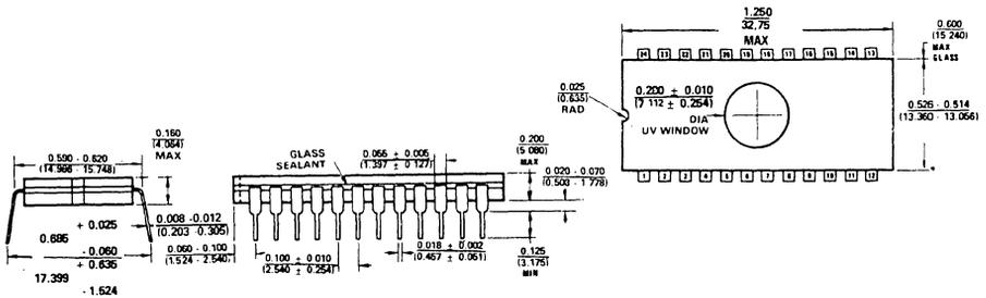
**UV window Cavity Dual-In-Line Package (JQ)**
