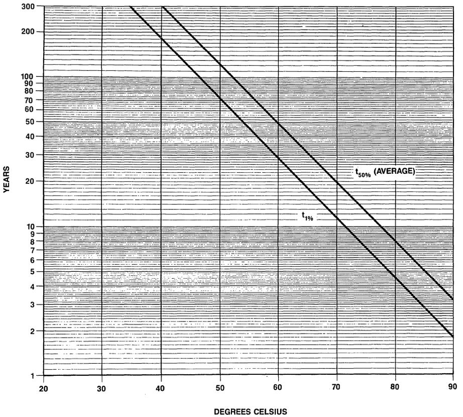
Figure 7. MK48Z02/03/12/13 Predicted Battery Storage Life vs Temperature
