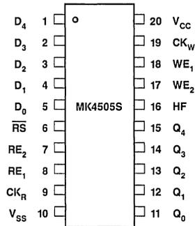
Figure 1. Pin Configuration, 300 mil DIP
