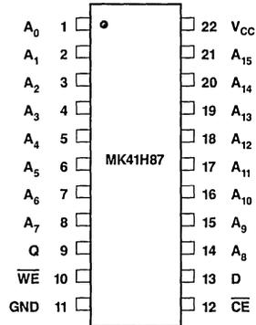
Figure 1. Pin Connections
