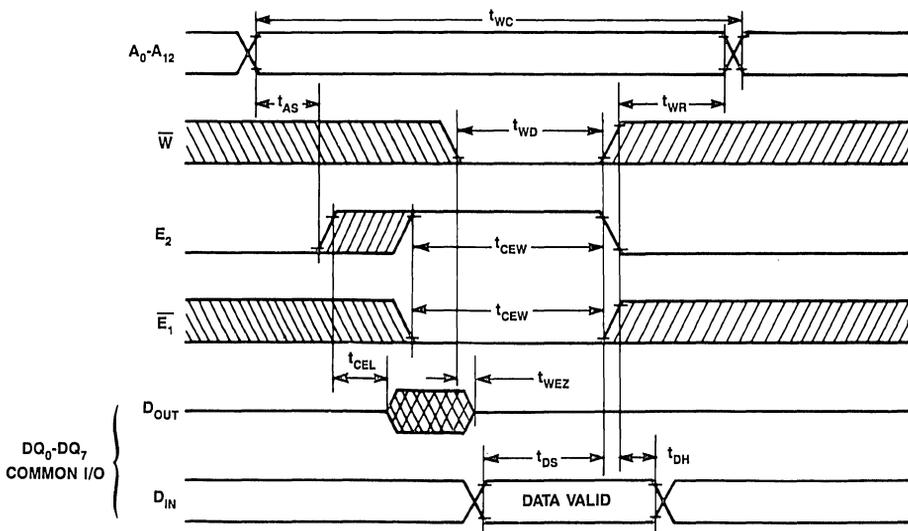
Figure 6. Write Cycle 3 ( $E_2$  Controlled Write)
