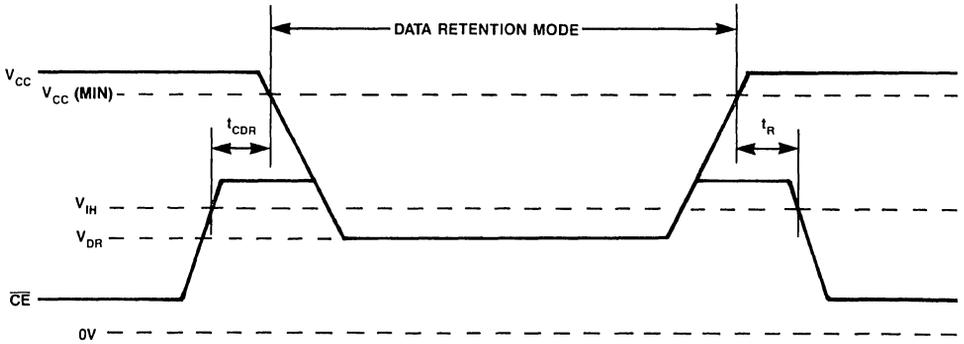
**Figure 4. Data Retention Timing**
