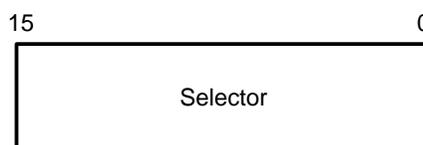
When the TR is loaded, the TR selector field indexes a TSS descriptor that must reside in the global-descriptor table (GDT). The contents of the selected descriptor are cached on-chip in the hidden portion of the TR.
