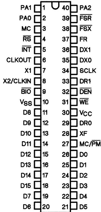
Figure 2-1. TMS32011 Pin Assignments
