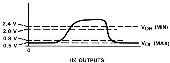
FIGURE 3. VOLTAGE REFERENCE LEVELS
