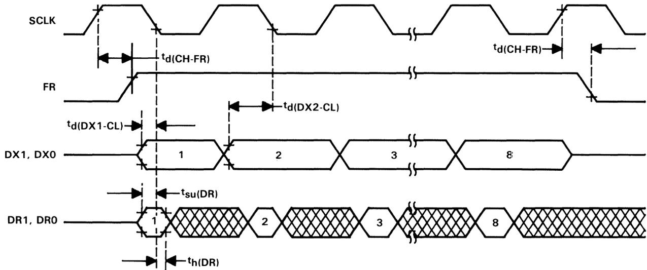
internal framing: fixed-data rate
