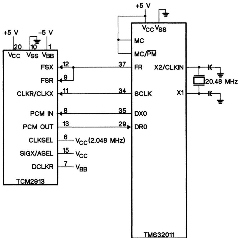
Figure 5-1. Codec Interface for Standalone Serial Operation
