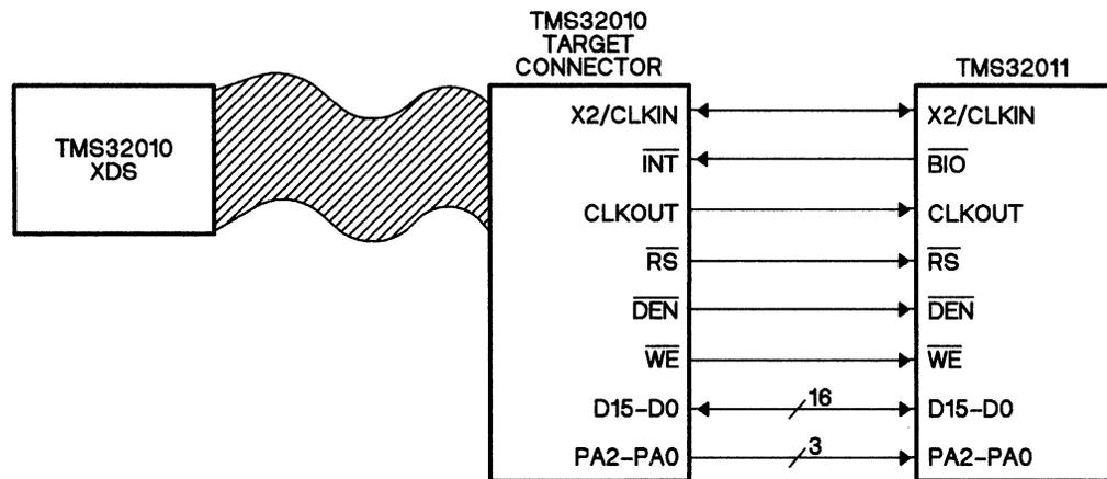
Figure 6-2. XDS/TMS32011 Peripheral Mode Interface
