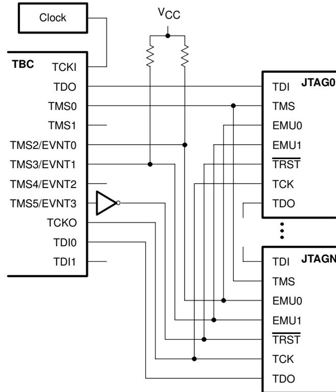
In the system design shown in Figure E–15, the TBC emulation signals TCKI, TDO, TMS0, TMS2/EVNT0, TMS3/EVNT1, TMS5/EVNT3, TCKO, and TDI0 are used, and TMS1, TMS4/EVNT2, and TDI1 are not connected. The target devices' EMU0 and EMU1 signals are connected to  $V_{CC}$  through pullup resistors and tied to the TBC's TMS2/EVNT0 and TMS3/EVNT1 pins, respectively. The TBC's TCKI pin is connected to a clock generator. The TCK signal for the main JTAG pin is driven by the TBC's TCKO pin.
