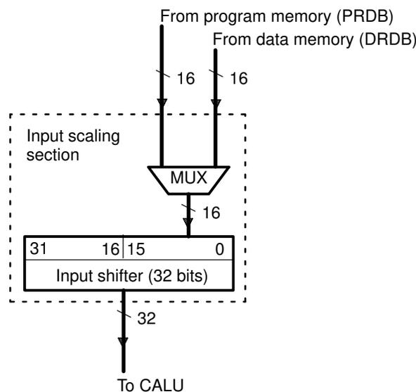
**Input.** Bits 15 through 0 of the input shifter accept a 16-bit input from either of two sources (see Figure 3–2):
