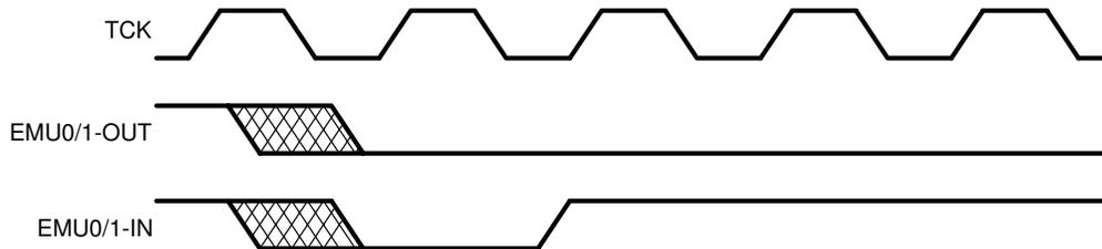
Figure E–13. EMU0/1 Configuration With Additional AND Gate to Meet Timing Requirements of Greater Than 25 ns
