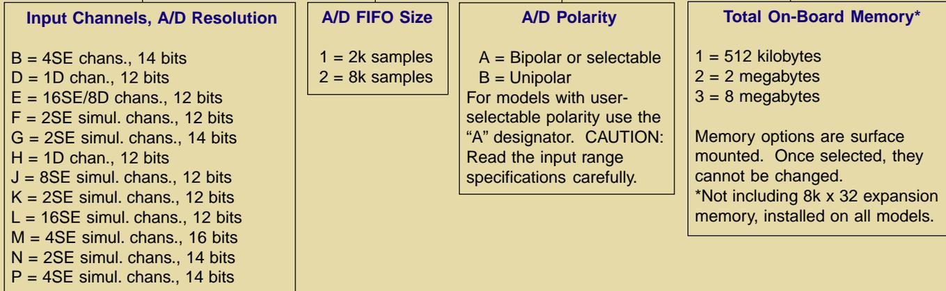
Example: PC-430G2A 14 bits, 8k FIFO, bipolar input, 512 kB memory.
