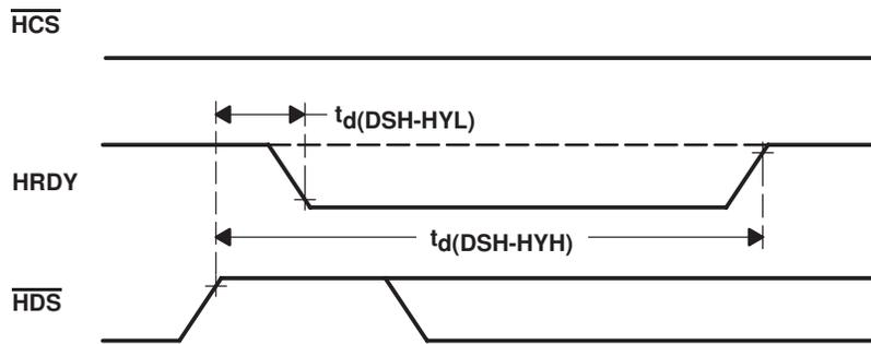
Figure 33. HRDY Signal When  $\overline{\text{HCS}}$  Is Always Low
