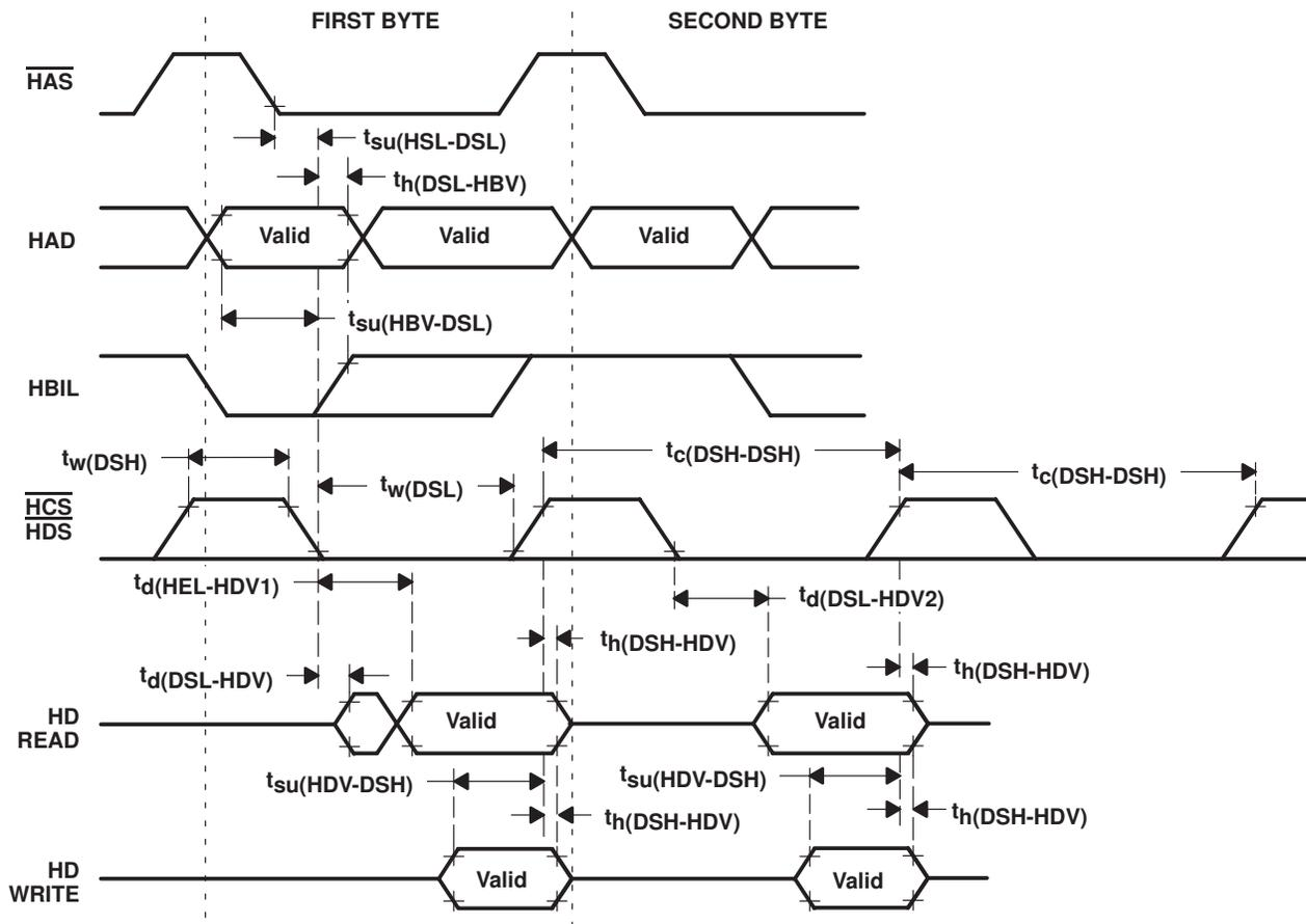
Figure 31. Read/Write Access Timings Using  $\overline{\text{HAS}}$  Without  $\overline{\text{HRDY}}$
