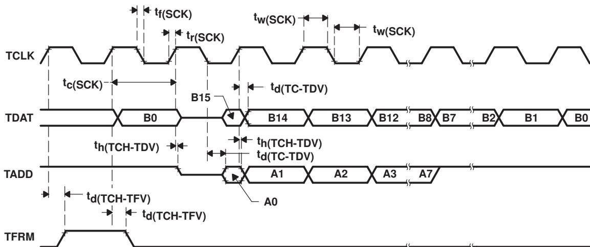
Figure 26. Serial-Port Transmit Timing in TDM Mode
