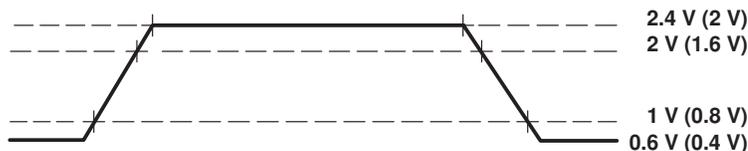
Figure 10. TTL-Level Outputs
