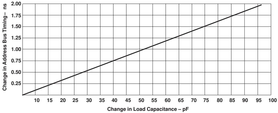
Figure 16. Address Bus Timing Variation With Load Capacitance
