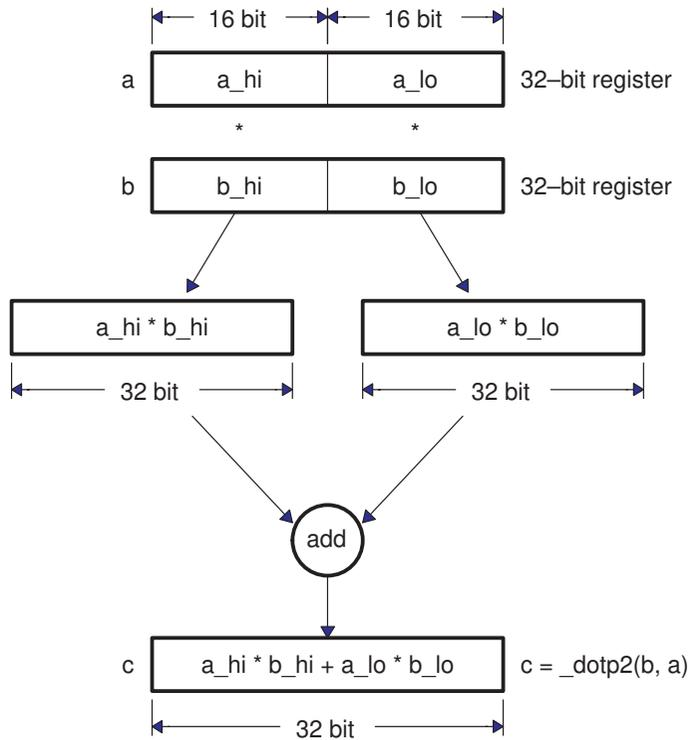
This operation exactly maps to the operation the dot product kernel performs. The modified version of the kernel absorbs two of the four ADDs into `_dotp` intrinsics. The result is shown as Example 6–11. Notice that the variable `c` has been eliminated by summing the results of the `_dotp` intrinsic directly.
