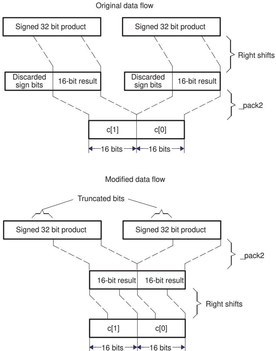
Whether or not the 16-bit shift version is used, consider the vector multiply to be fully optimized from a packed data processing standpoint. It can be further optimized using the more general techniques such as loop-unrolling and software pipelining that are discussed in Chapter 6.
