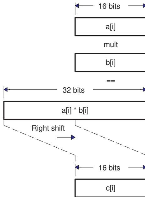
Notice that the values are still loaded and stored as 16-bit quantities. Therefore, you should use the same basic flow as the vector sum. Example 6–7 shows this starting point. Figure 6–11 and Figure 6–12 also apply to this example to illustrate how data is being accessed.
