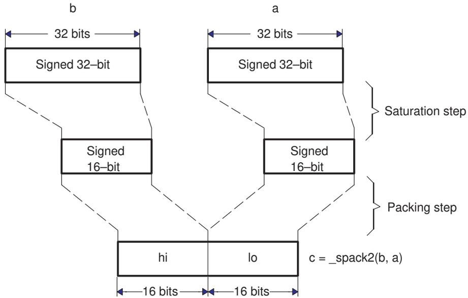
Notice that there are no special unpack operations for 16-bit data. Instead, the normal 32-bit right-shifts and extract operations can be used to unpack 16-bit elements into 32-bit quantities. Table 6–4 describes how to unpack signed and unsigned 16-bit quantities.
