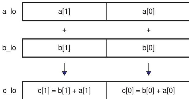
So, putting in `_add2()` to perform the additions provides the complete code shown in Example 6–6.
