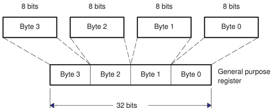
Figure 6–2. Two Half–Words Packed Into a Single General Purpose Register.
