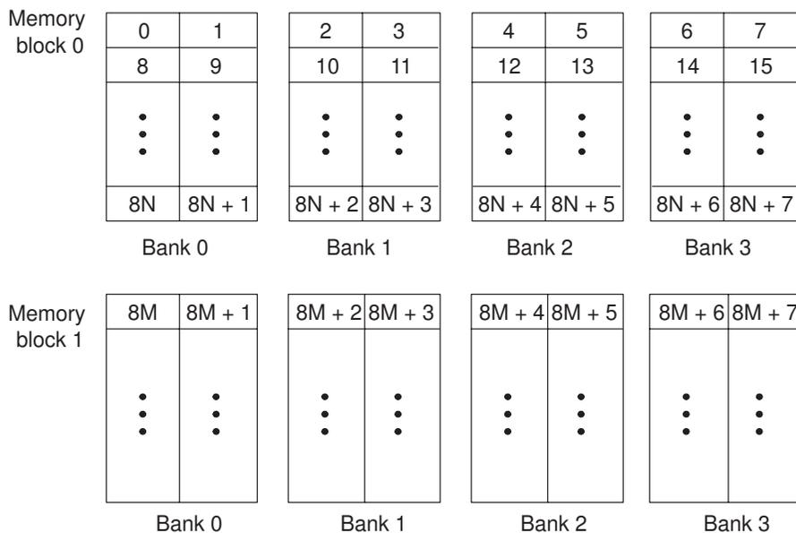
If each array in a loop resides in a separate memory block, the 2-cycle loop in Example 5–61 on page 5-111 is sufficient. This section describes a solution when two arrays must reside in the same memory block.
