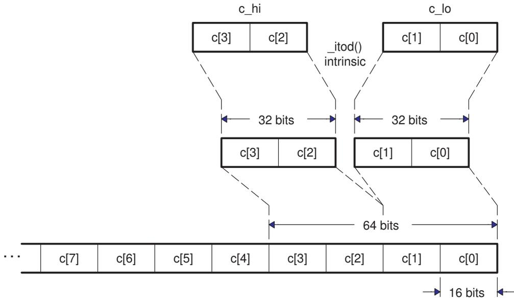
This code now efficiently reads and writes large amounts of data. The next step is to find a method to quickly add them. The `_add2()` intrinsic provides just that: It adds corresponding packed elements in two different words, producing two packed sums. It provides exactly what is needed, a vector addition. Figure 6–13 illustrates.
