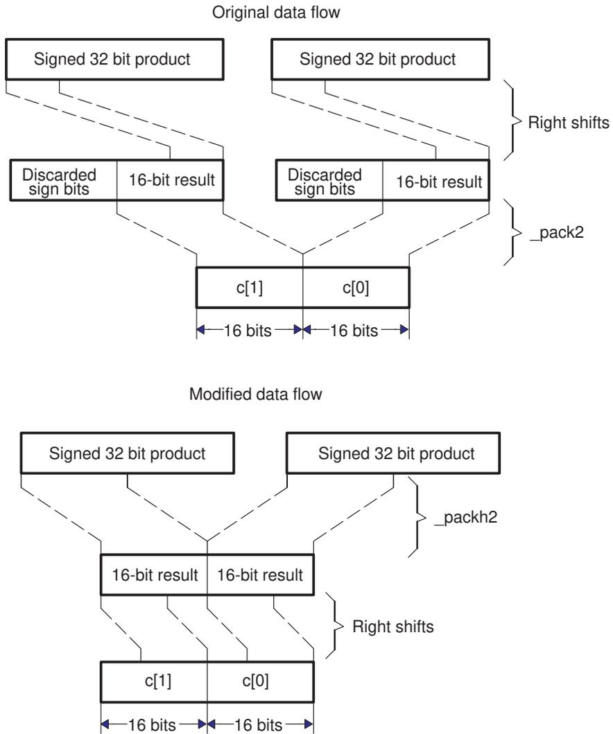
Figure 6–17. Fine Tuning Vector Multiply (shift < 16)
