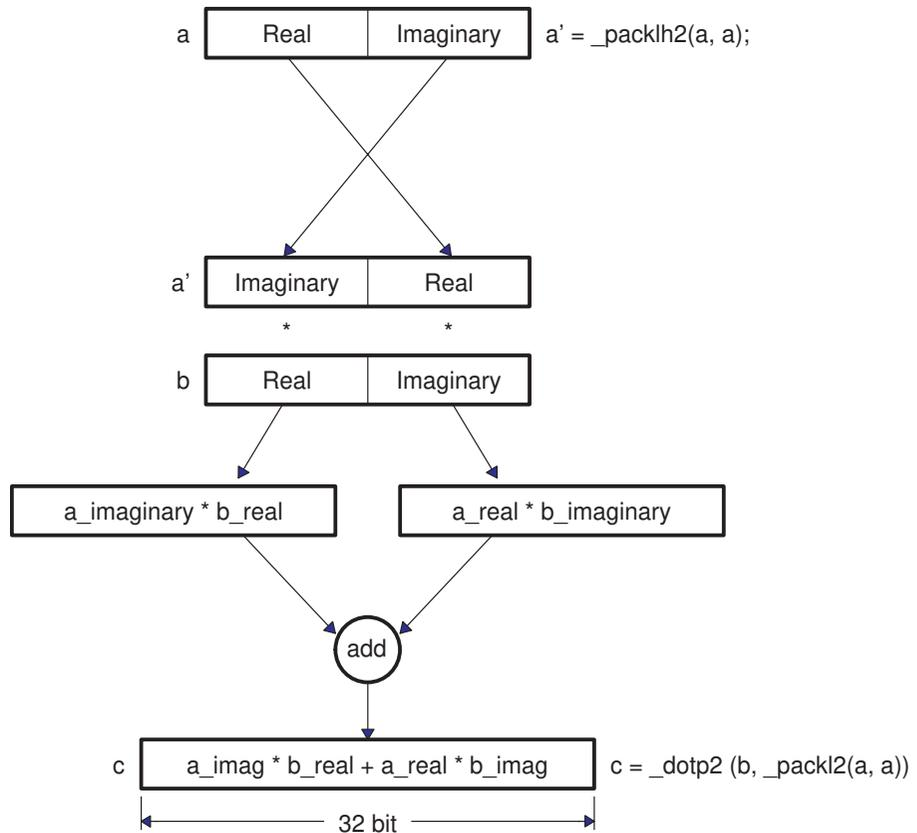
Once both the real and imaginary components of the result are calculated, it is necessary to convert the 32-bit results to 16-bit results and store them. In the original code, the 32-bit results were shifted right by 16 to convert them to 16-bit results. These results were then packed together with `_pack2` for storing. Our final optimization replaces this shift and pack with a single `_packh2`. Example 6–13 shows the result of these optimizations.
