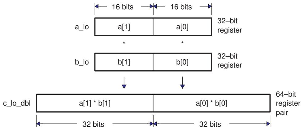
Once the 32-bit products are obtained, use standard 32-bit shifts to shift these to their final precision. However, this will leave the results in two separate 32-bit registers.
