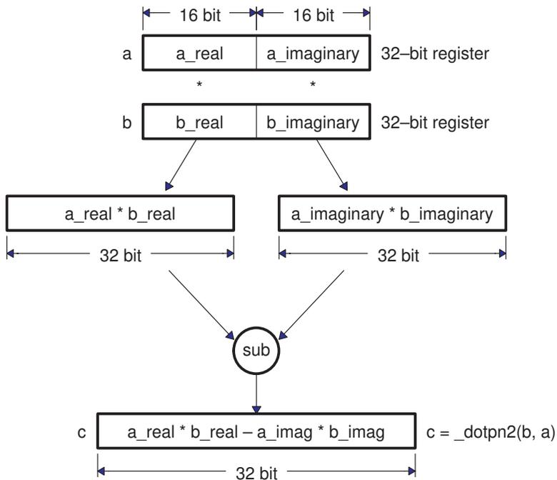
The calculation for the result’s imaginary component provides a different problem. As with the real component, the result is calculated from two products that are added together. A problem arises, though, because it is necessary to multiply the real component of one input with the imaginary component of the other input, and vice versa. None of the 'C64x intrinsics provide that operation directly given the way the data is currently packed.
