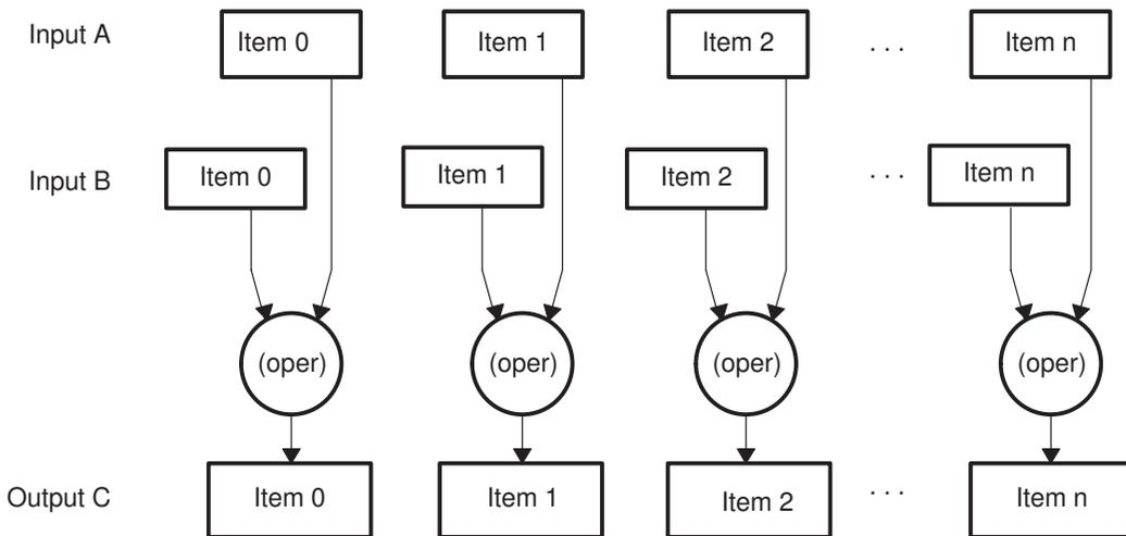
Although pure vector algorithms exist, most applications do not consist purely of vector operations as simple as the one shown above. More commonly, an algorithm will have portions, which behave as a vector algorithm, and portions which do not. These portions of the code are addressed by other packed-data processing techniques.
