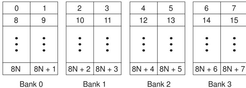
For devices that have more than one memory block (see Figure 5–23), an access to bank 0 in one block does not interfere with an access to bank 0 in another memory block, and no pipeline stall occurs.
