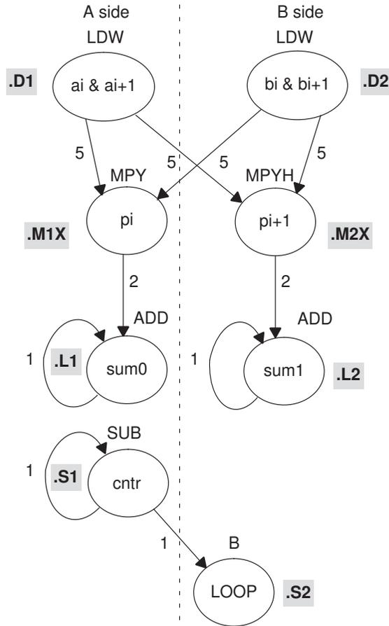
Example 5–21. Linear Assembly for Fixed-Point Dot Product Inner Loop (With Conditional SUB Instruction)
