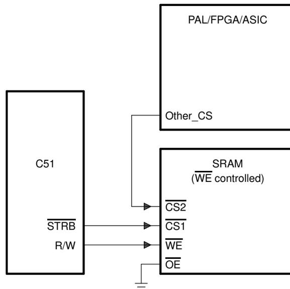
Figure 8. 'C5x No Decode SRAM Interface
