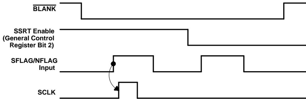
**Figure 11. Relationship Between SFLAG/NFLAG,  $\overline{\text{BLANK}}$ , and SCLK**
