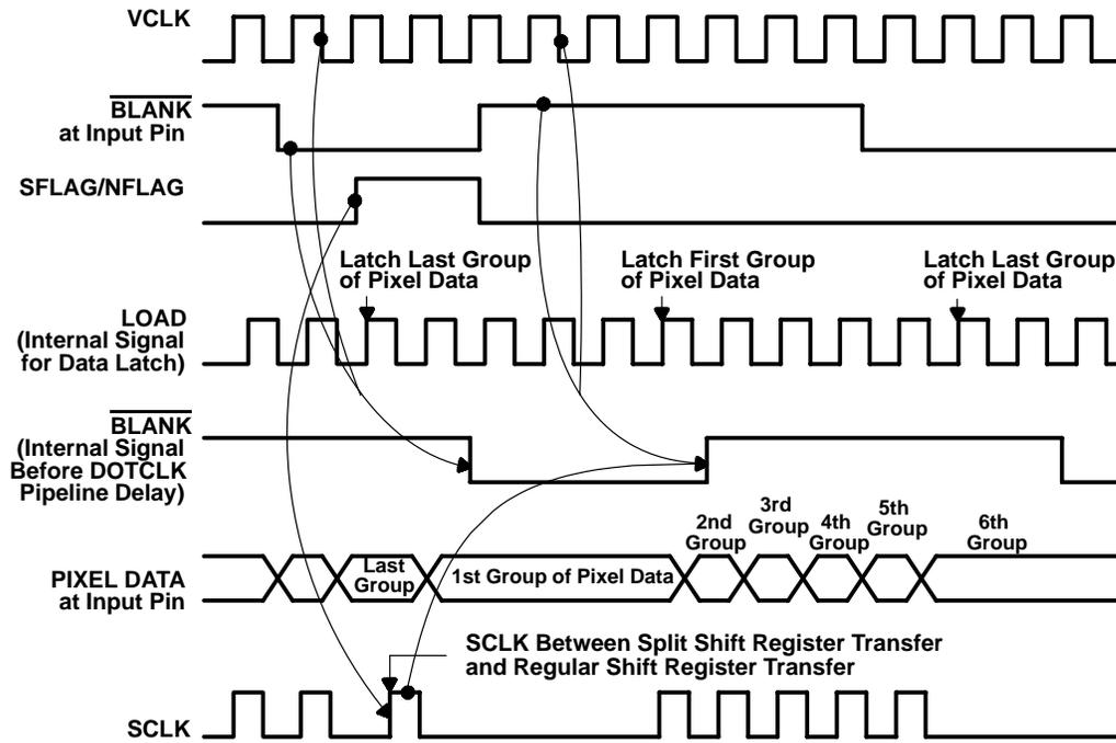
NOTE: The SSRT function is enabled (general control register bit 2 = 1).
