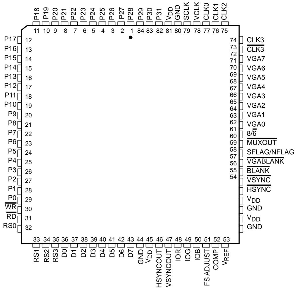
Figure 2. Terminal Assignments
