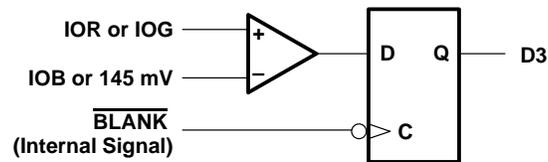
**Figure 14. Internal Comparator Circuitry for Analog Test**
