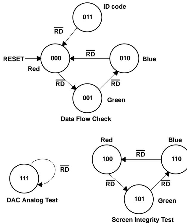
**Figure 13. Test Register Control Word State Diagrams**
