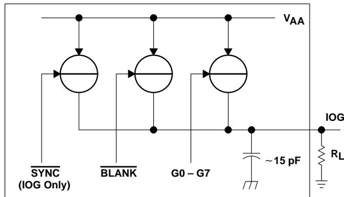
**Figure 2–6. Equivalent Circuit of the IOG Current Output**
