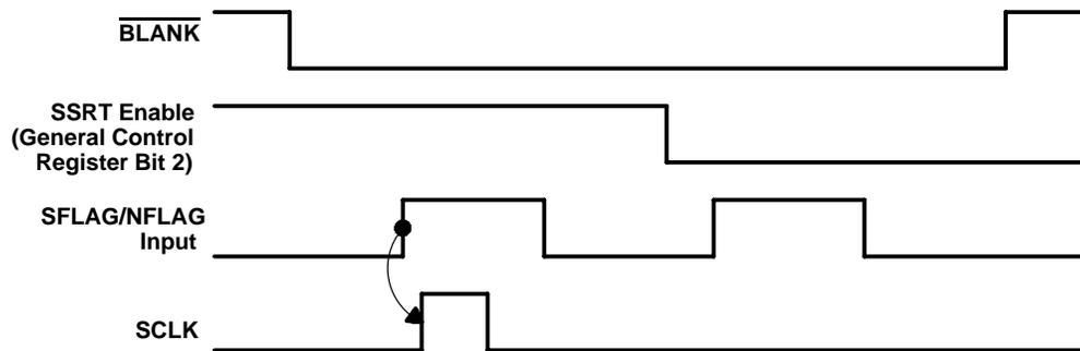
Figure 2–9. Relationship Between SFLAG/NFLAG,  $\overline{\text{BLANK}}$ , and SCLK
