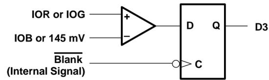
**Figure 2–12. Internal Comparator Circuitry for Analog Test**
