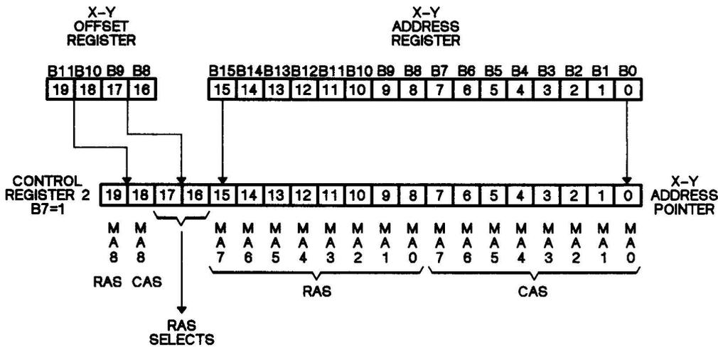
Figure 4-8. X-Y Address Pointer RAS Selects as MSBs
