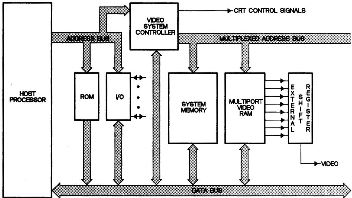
Figure 1-1. Block Diagram of Typical TMS34061 VSC System
