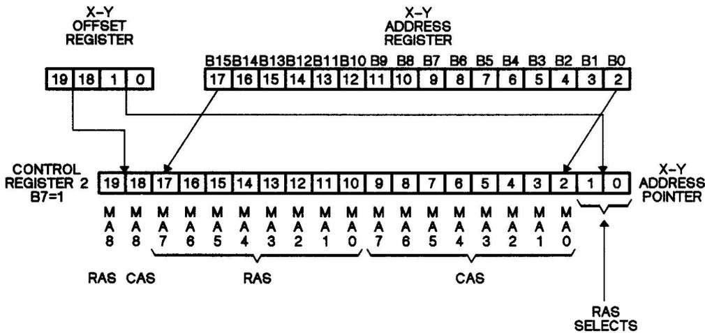
Figure 4-9. X-Y Address Pointer RAS Selects as LSBs
