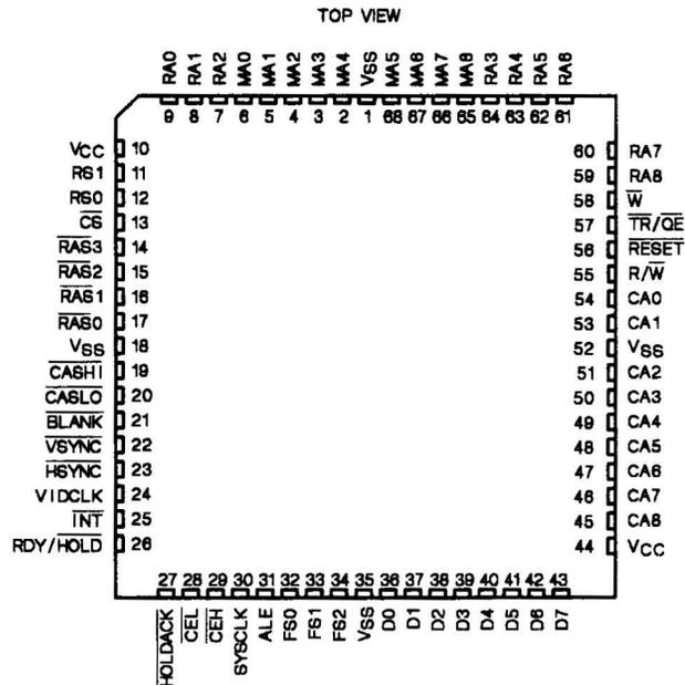
Figure 2-1. TMS34061 Pin Assignments and Signal Names
