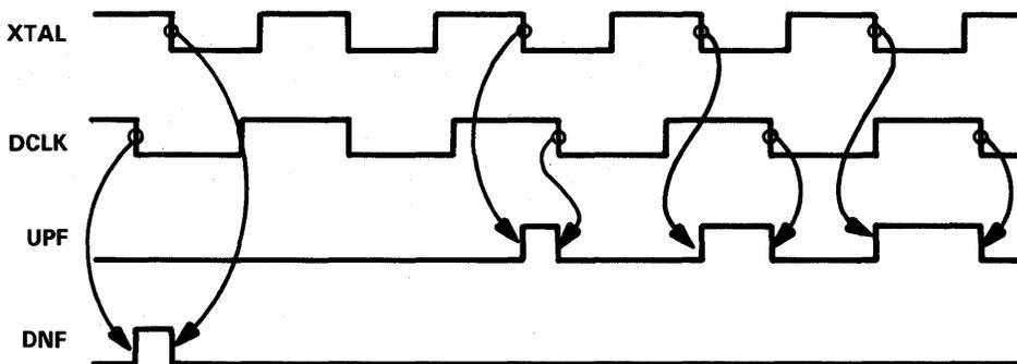
FIGURE 4-75. FREQUENCY DETECTOR TIMING CHARACTERISTICS
