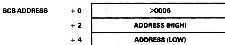
FIGURE 4-53. RECEIVE COMMAND SCB
