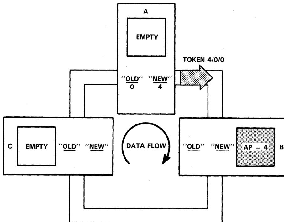
FIGURE 3-32. STATION A PERFORMS A REPLACE AND TRANSMITS THE TOKEN
