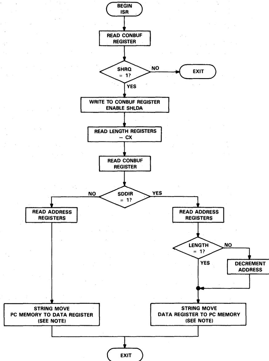
NOTE: The string move instruction automatically increments the source and destination addresses for each byte until the CX register is decremented to zero.
