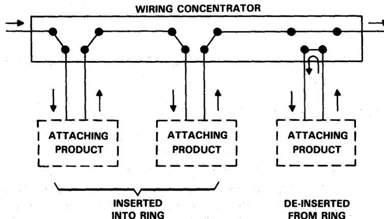
FIGURE 1-5. TOKEN RING WIRING CONCENTRATOR
