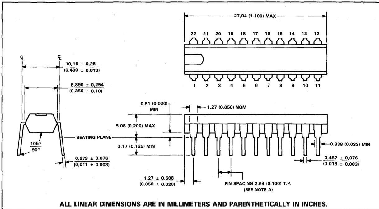
NOTE A: Each pin centerline is located within 0,25(0.010) of its true longitudinal position.
