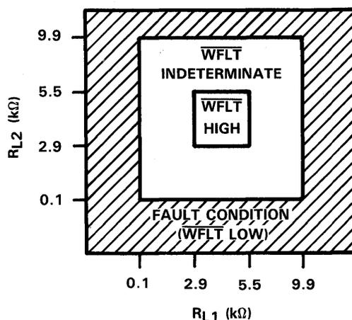
FIGURE 4. WIRE-FAULT PIN TEST
