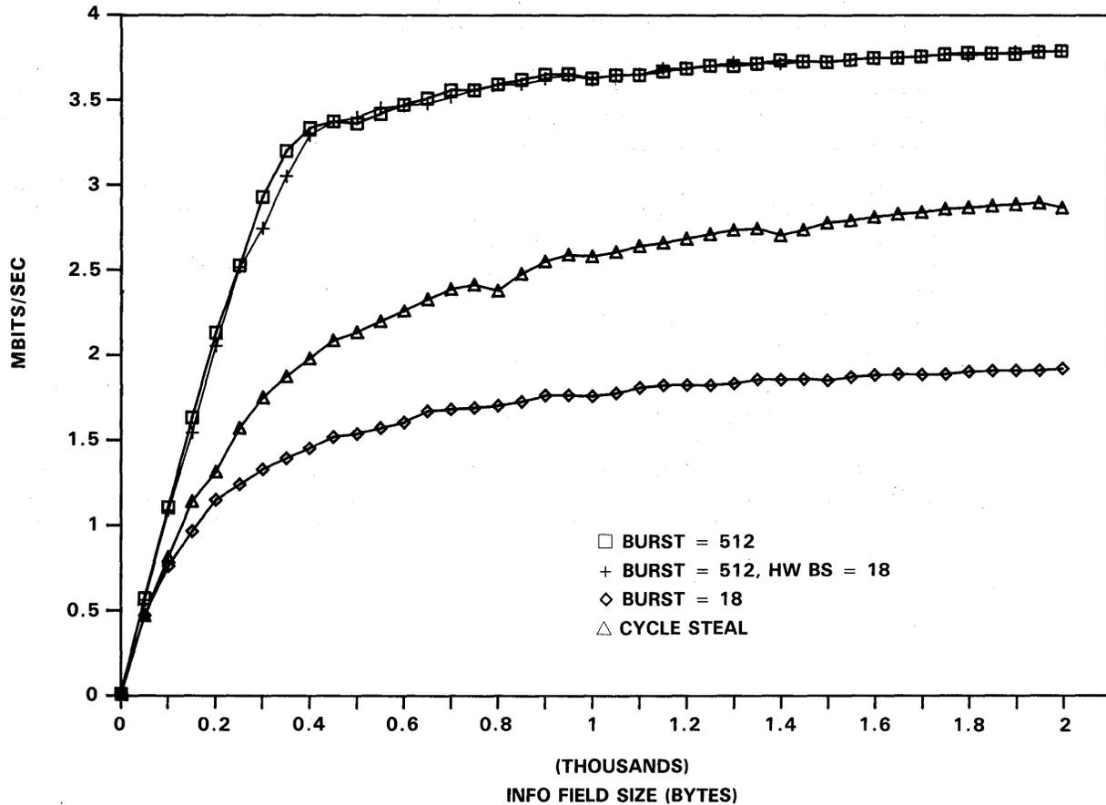
FIGURE 2-10. TRANSMIT THROUGHPUT — PC AT ADAPTER:
