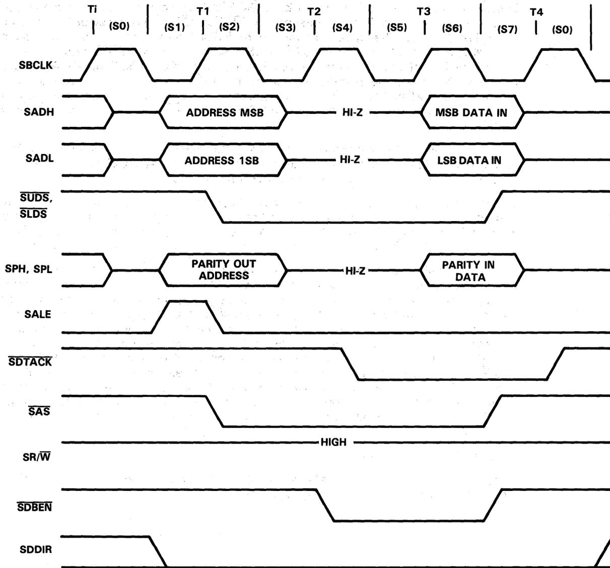
**FIGURE 4-24. 680XX MODE DMA READ TIMING**
