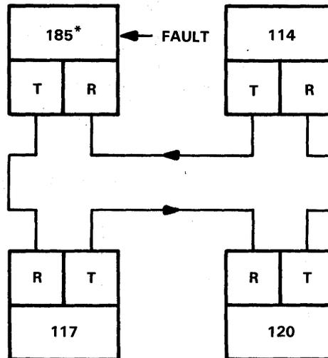
**FIGURE 3-43. TRANSMITTER STREAMING FAULT IN ADAPTER 185**
