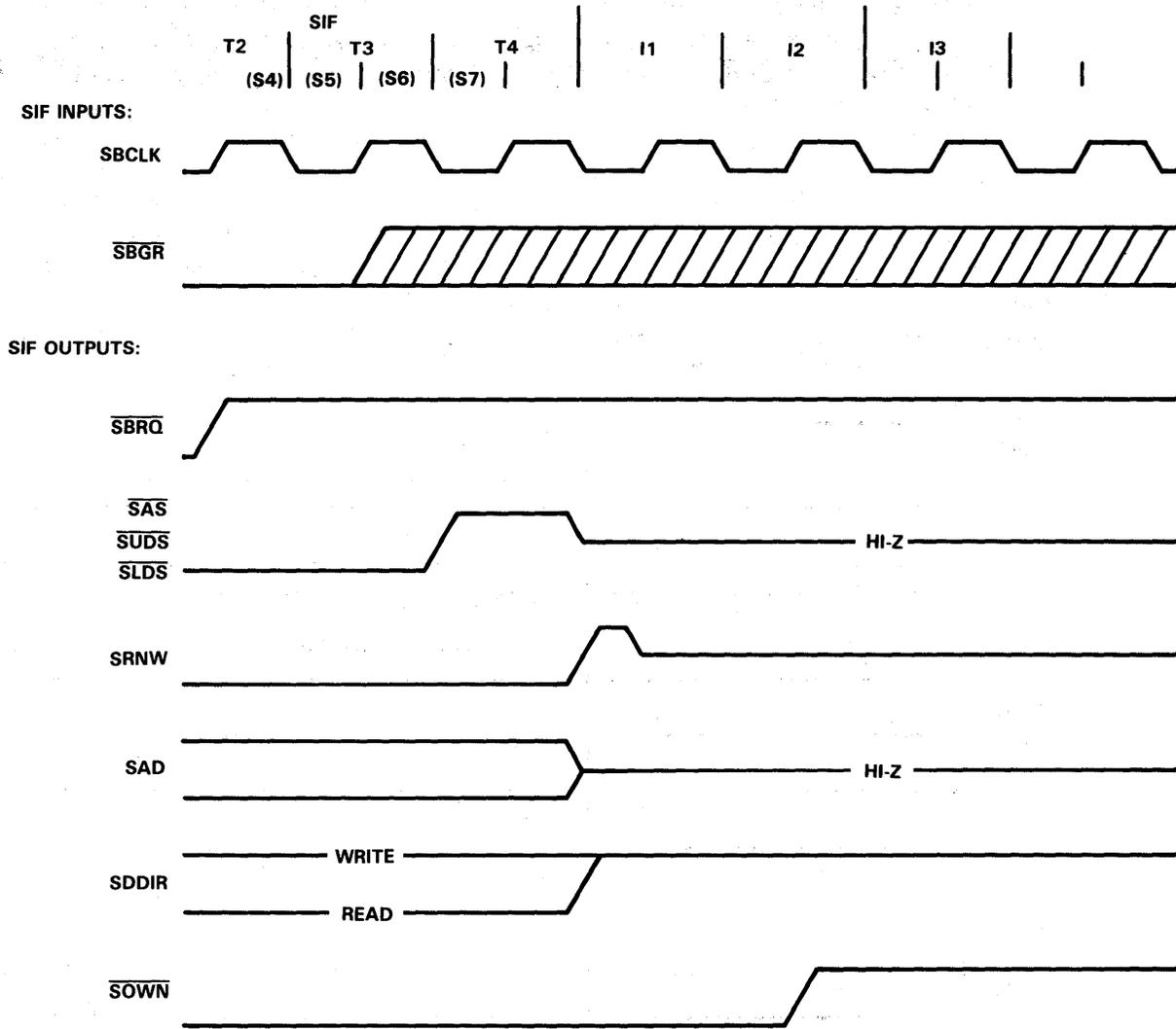
**FIGURE 4-23. ADAPTER RETURNS SYSTEM BUS – 680XX MODE**
