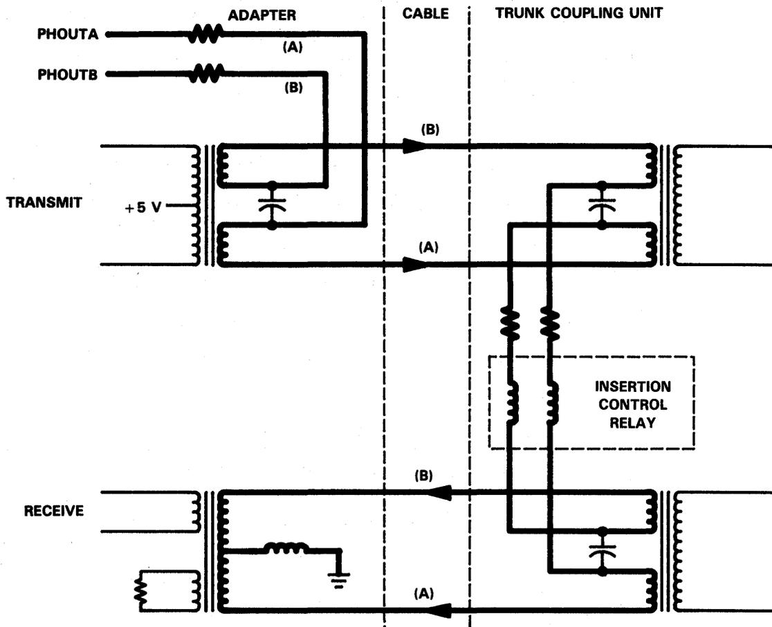
FIGURE 4-76. PHANTOM DRIVE PATH
