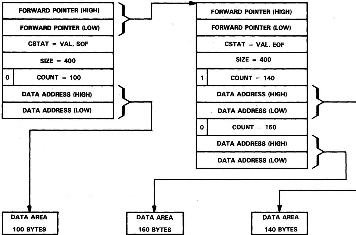
FIGURE 4-49. TRANSMIT LIST FORMAT: EXAMPLE 2
