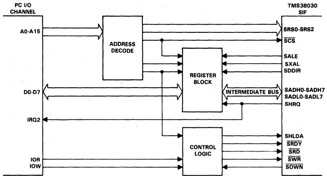
**FIGURE 2-1. I/O MAPPED DESIGN BLOCK DIAGRAM**
