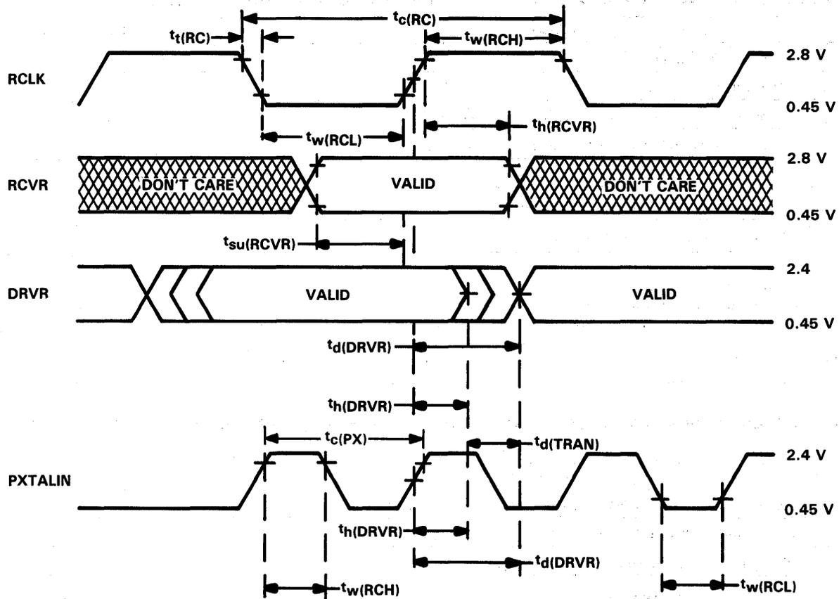
NOTE 19: The timing reference points for RCVR and RCLK are 2.6 V and 0.6 V. The timing reference points for PXTALIN are 2 V and 0.8 V. The intermediate reference point for RCLK and DRVR is 1.5 V.
