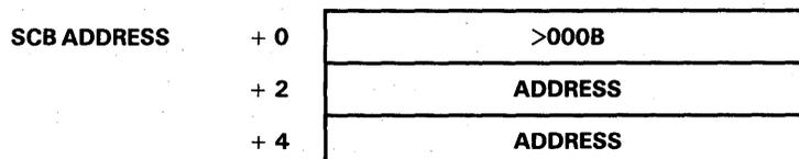
FIGURE 4-65. READ ADAPTER BUFFER COMMAND SCB
