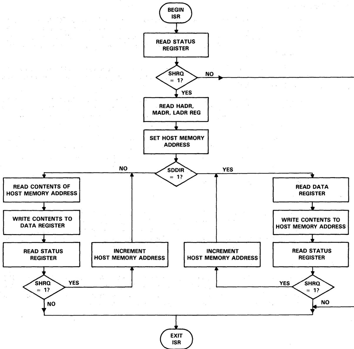
FIGURE 2-2. INTERRUPT SERVICE ROUTINE FLOWCHART – I/O MAPPED EXAMPLE
