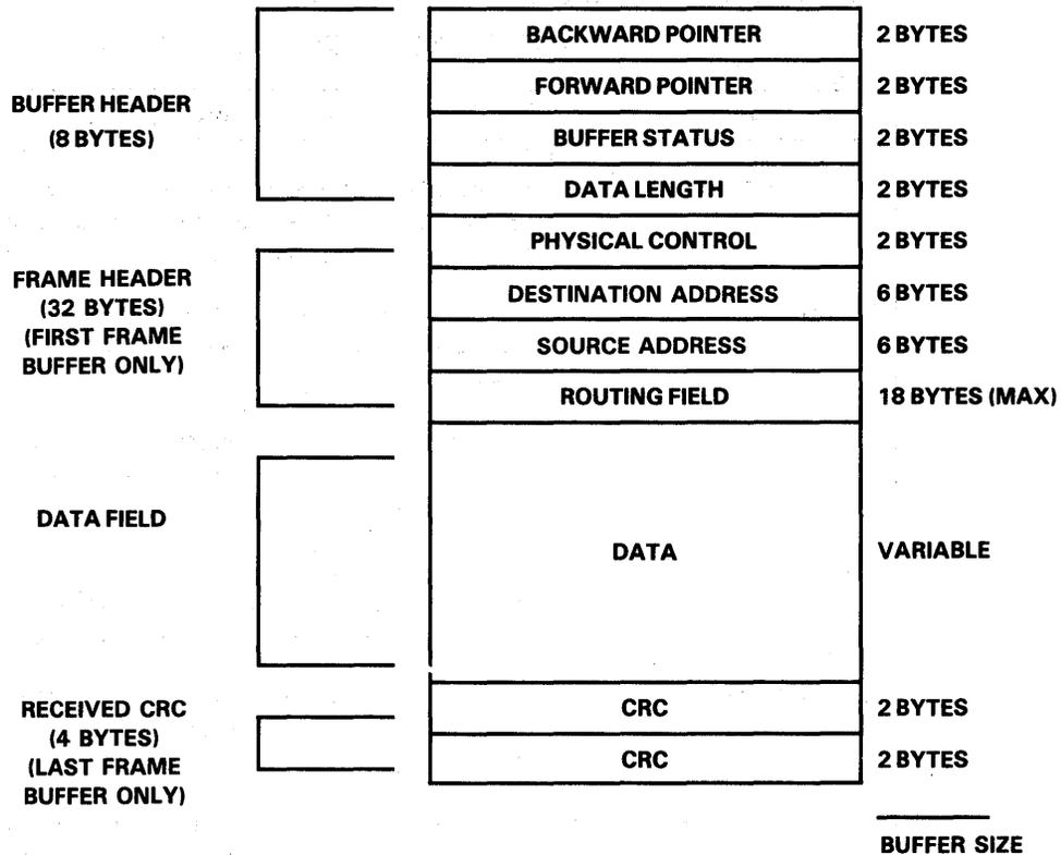
FIGURE 4-43. ADAPTER INTERNAL BUFFER FORMAT
