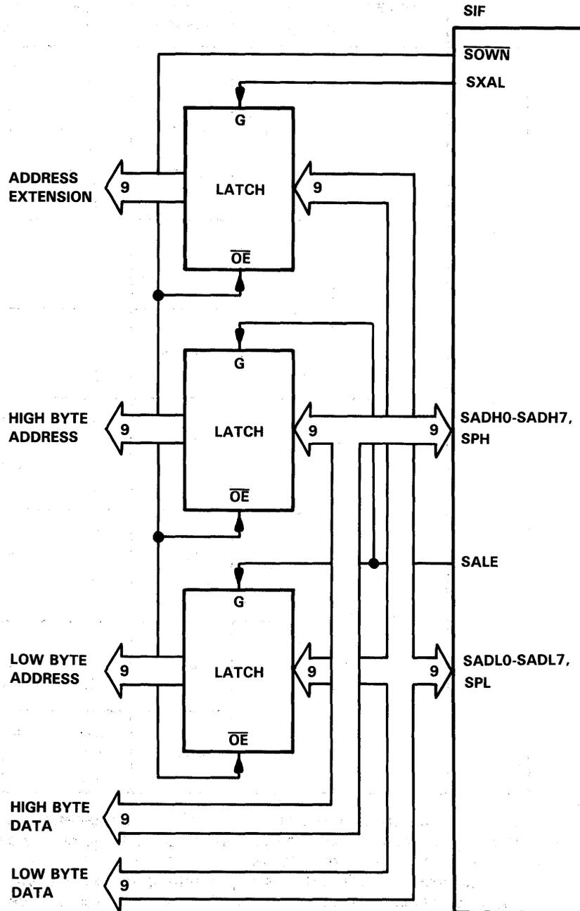
FIGURE 4-15. EXTERNAL TTL LATCHES DEMULTIPLEX ADDRESS/DATA BUS
