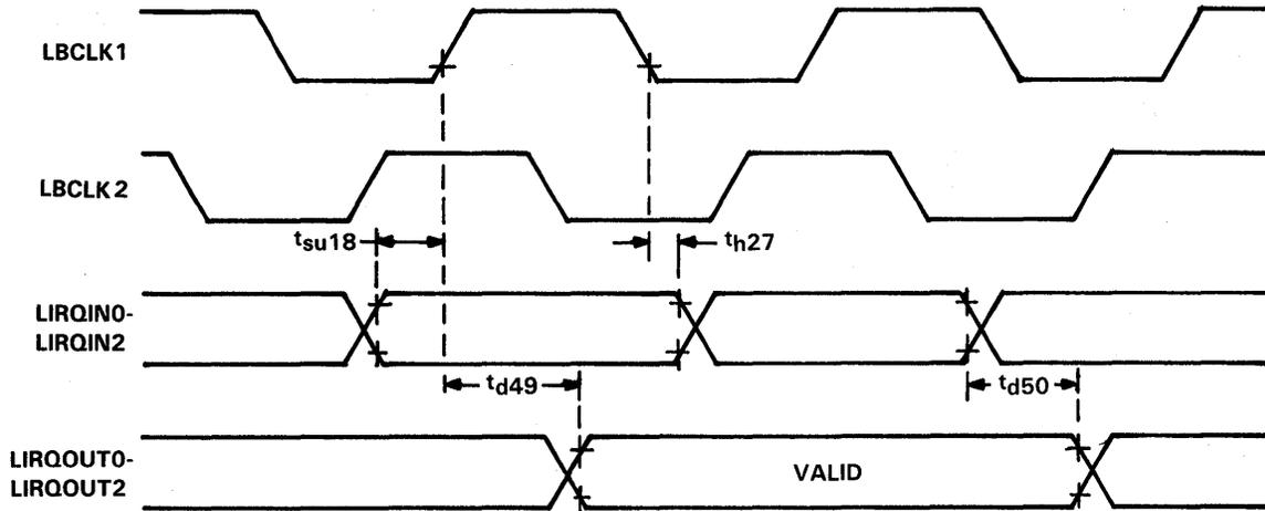
NOTE 10: LIRQOUTs may not follow LIRQINs because the TMS38030 prioritizes LIRQOUT0-LIRQOUT2 outputs between internal TMS38030 interrupts and LIRQINO-LIRQIN2.
