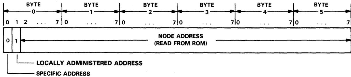
FIGURE B-1. BURNED-IN ADDRESS FORMAT
