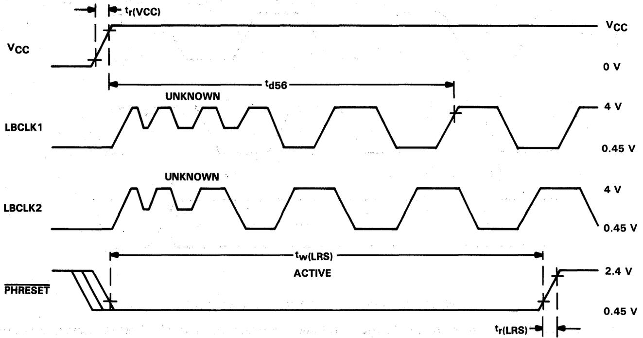
NOTE 11: The timing reference points for VCC are 4.5 V and 1.2 V. The timing reference points for LBCLK1 and LBCLK2 are 3 V and 0.8 V. The timing reference points for  $\overline{\text{PHRESET}}$  are 2 V and 0.8 V.
