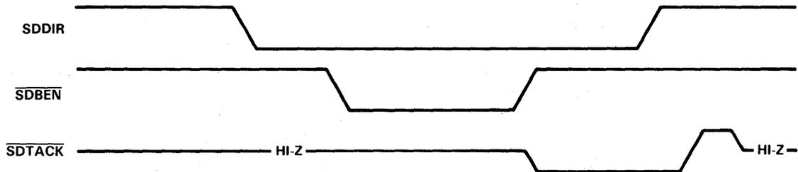
**FIGURE 4-12. 680XX MODE DIO WRITE CYCLE TIMING**
