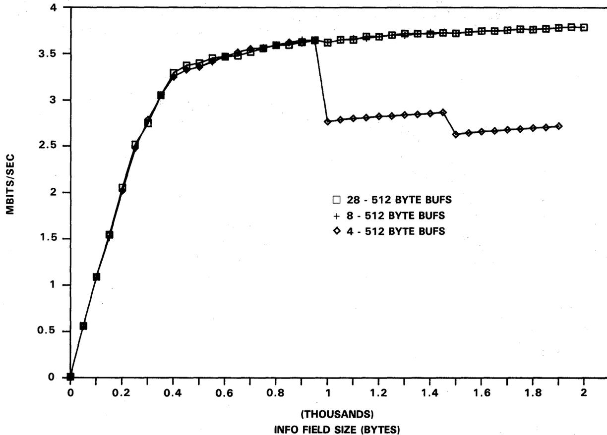
FIGURE 2-8. TRANSMIT THROUGHPUT — PC AT ADAPTER:
