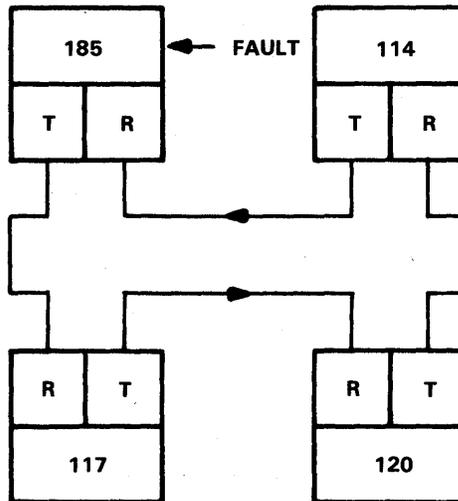
**FIGURE 3-45. ADAPTER 185 STREAMING CLAIM TOKEN FRAMES**
