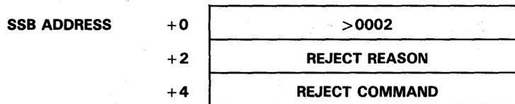
**FIGURE 4-36. COMMAND REJECT SSB FORMAT**
