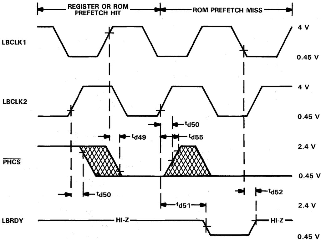
NOTE 10: The timing reference points for LBCLK1 and LBCLK2 are 3 V and 0.8 V. The timing reference points for the other waveforms are 2 V and 0.8 V.
