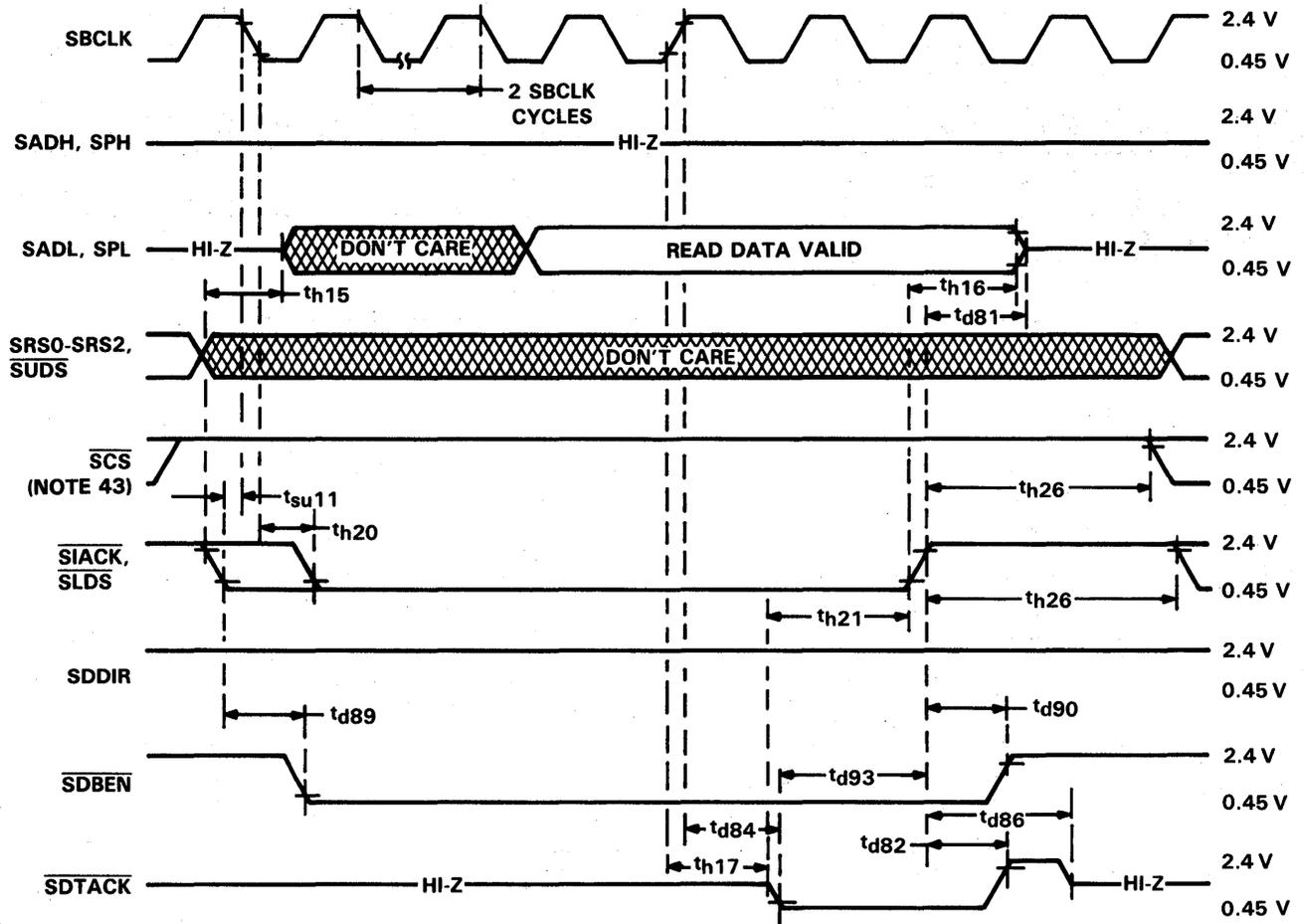
NOTE 43: The "inactive" chip select is  $\overline{SIACK}$  in DIO read and DIO write cycles, and  $\overline{SCS}$  in interrupt acknowledge cycles.
