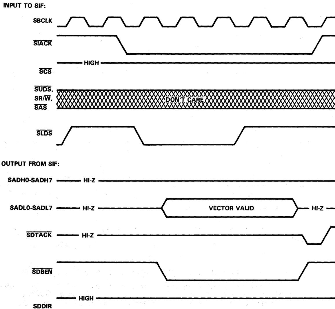
FIGURE 4-27. INTERRUPT ACKNOWLEDGE TIMING FOR 680XX MODE
