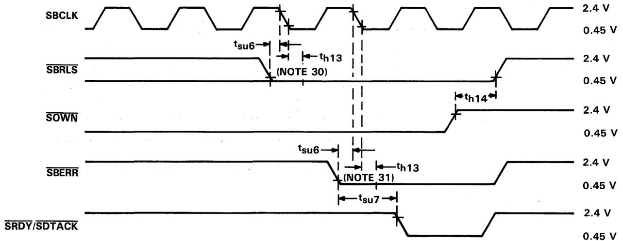
NOTES: 30. The TMS38030 ignores the assertion of  $\overline{SBRLS}$  if it does not own the system bus. If it does own the system bus, then when it detects the assertion of  $\overline{SBRLS}$  it will complete any internally started DMA cycle and relinquish control of the bus. If no DMA transfer has internally started, then the TMS38030 will release the bus before starting another.
