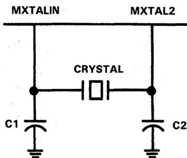
NOTE 7: C1 and C2 represent the total capacitance on these pins including strays and parasitics, but not the input capacitance of the device pins.
