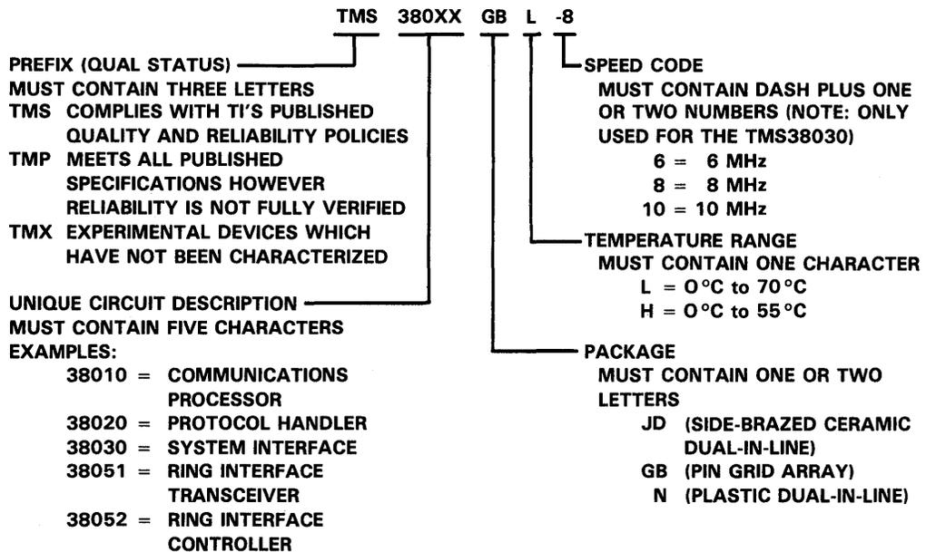
NOTE: The TMS38020 will include a ROM code level designator. (RC \_ \_ \_ \_ ).
