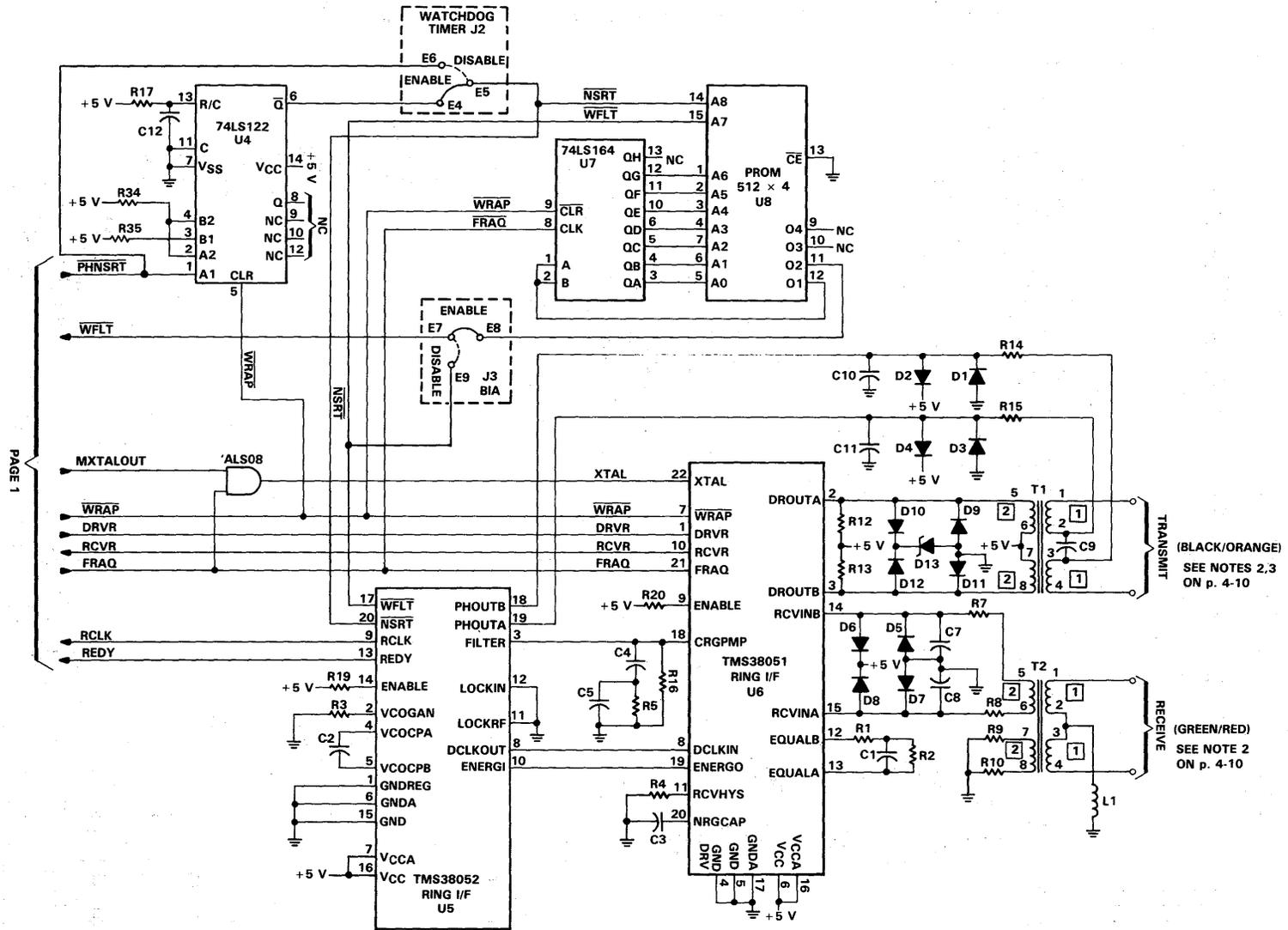
FIGURE 4-5. ADAPTER CHIP SET INTERCONNECT DIAGRAM (2 of 4)
