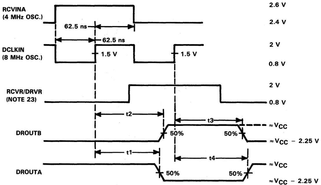
NOTE 23: For this test the RCVR output is tied directly to the DRVR input to test the asymmetry of the transmitter in a repeater configuration.
