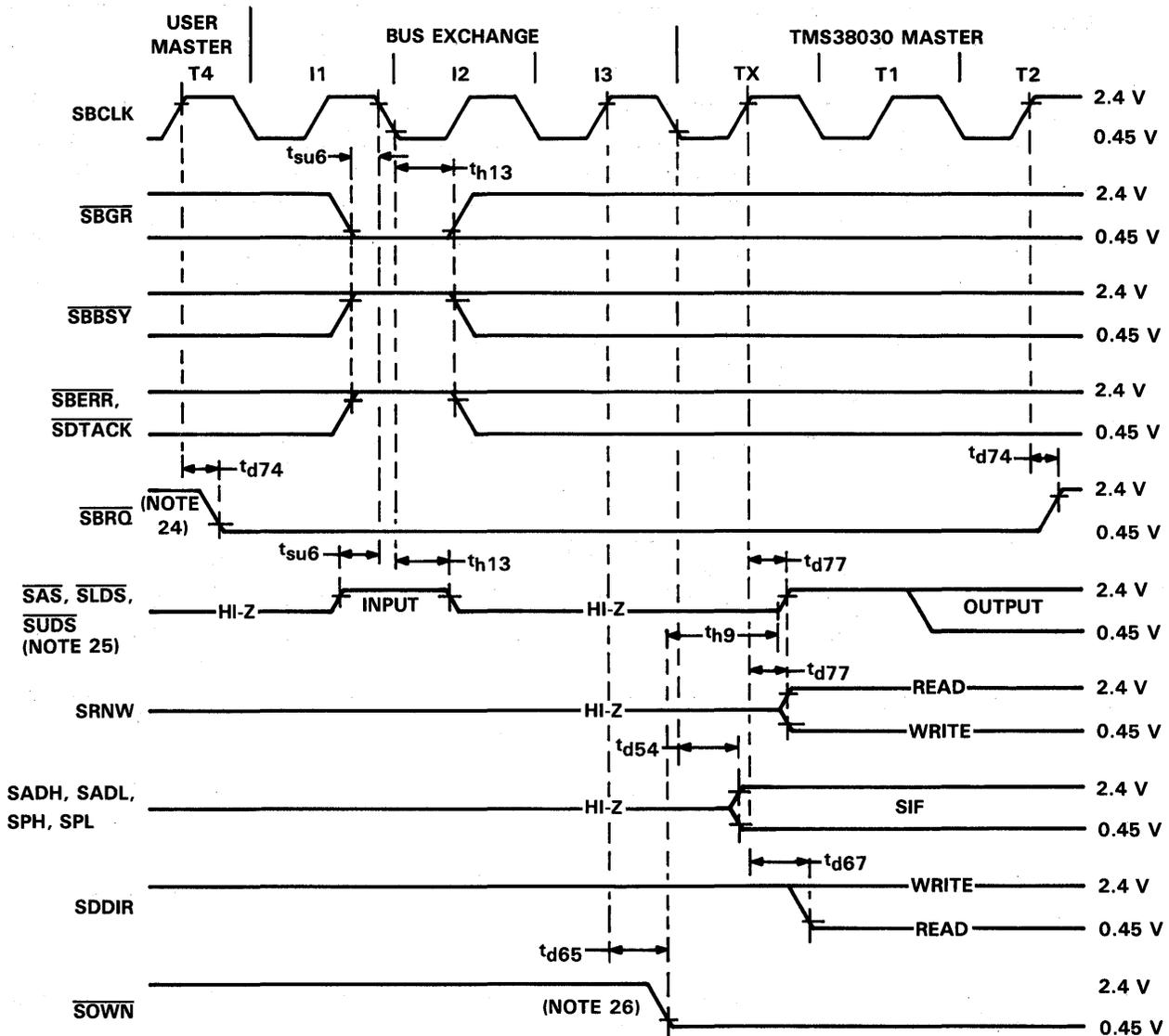
NOTES: 24. SHLDA/SBGR must be sampled in its deasserted state on the falling edge of SBCLK. The TMS38030 will then assert SHRQ/SBRQ on the second subsequent rising edge of SBCLK.
