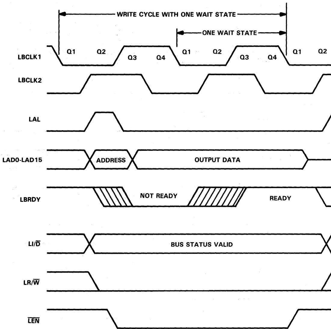
(b) LAN ADAPTER BUS WRITE CYCLE WITH WAIT STATE
