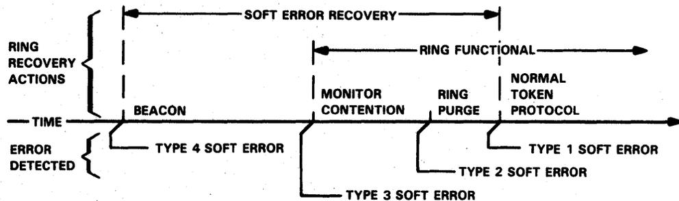
FIGURE 3-39. SOFT ERROR RECOVERY TIME LINE
