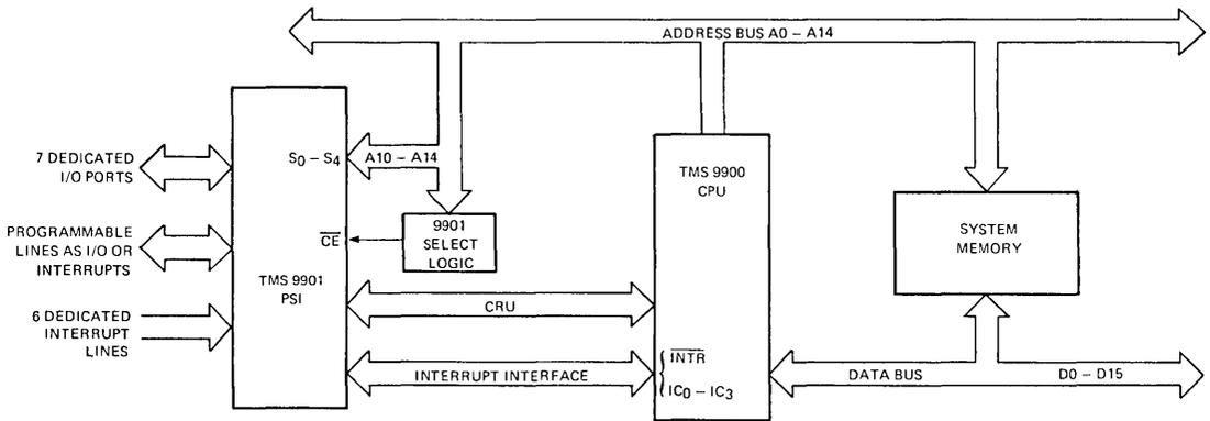
FIGURE 1— TYPICAL TMS 9901 PROGRAMMABLE SYSTEM INTERFACE (PSI) APPLICATION
