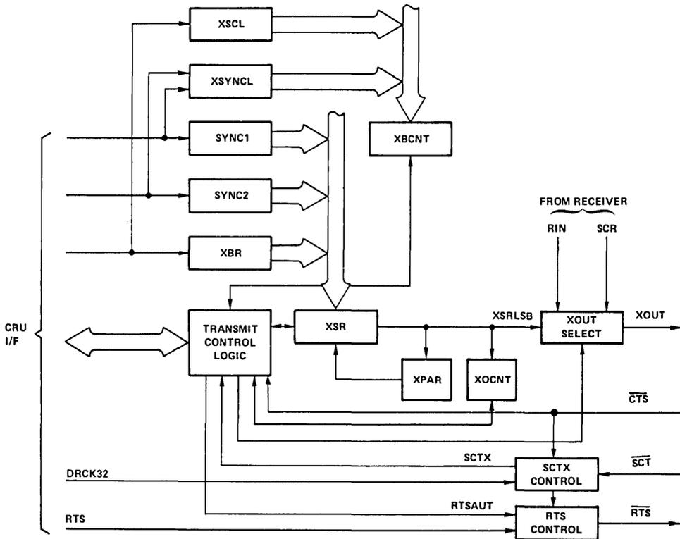
FIGURE 7. TMS 9903 SCC TRANSMITTER BLOCK DIAGRAM
