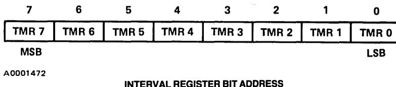
The figure below illustrates the establishment of the interval for the timer. For example, if the interval register is loaded with a value of  $40_{16}$  ( $64_{10}$ ) with  $t_{int} = 1 \mu s$ , the interval at which the timer decrements to zero and interrupts the CPU is
