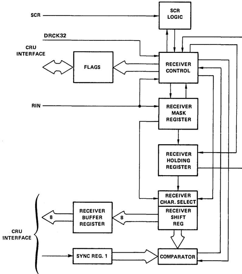
FIGURE 9. TMS 9903 RECEIVER BLOCK DIAGRAM
