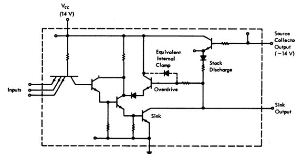
FIGURE 10. An Individual Sink Circuit
