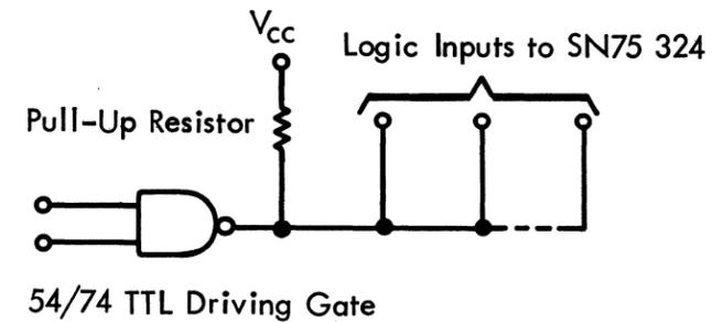
FIGURE 5. Input to SN75 324 from 54/74 TTL Using Pull-Up Resistor
