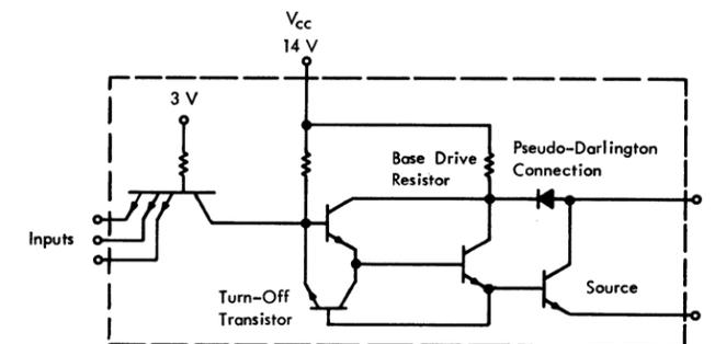
FIGURE 11. An Individual Source Circuit
