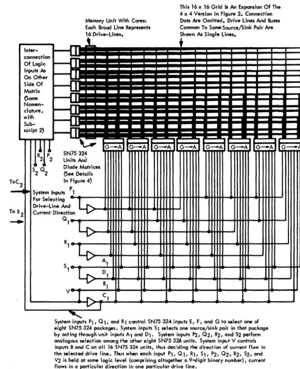
FIGURE 3. SN75 324 Serving 256 Drive Lines in a Magnetic Memory, with Hypothetical Logic Interconnections to Show Input Flexibility
