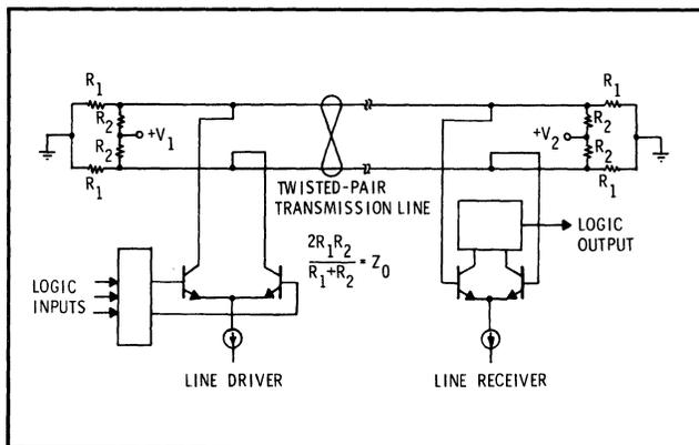
Figure 2 – A Basic High Speed Transmission System
