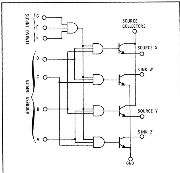
Figure 10 – 75 324 Monolithic Memory Driver Logic Diagram
