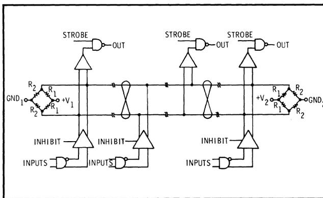
Figure 3 – Expansion of the Basic System to "Party-Line" Operation
