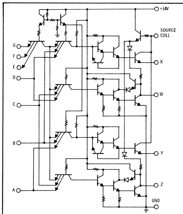
Figure 11 – Circuit Schematic of 75 324 Monolithic Memory Driver
