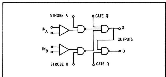
Figure 19 – Block Diagram of 7520
