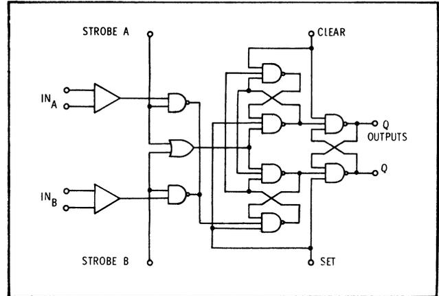
Figure 22 – Block Diagram of 7526
