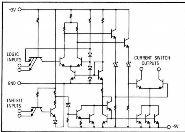
Figure 4 – 75 109 Line Driver Circuit
