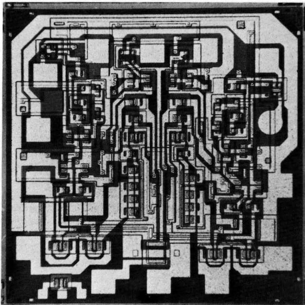
Figure 5 – Microphotograph of 75 109 Line Driver Chip
