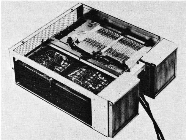
Figure 17 – Internal View of ICM-500 Memory Showing Board Layouts
