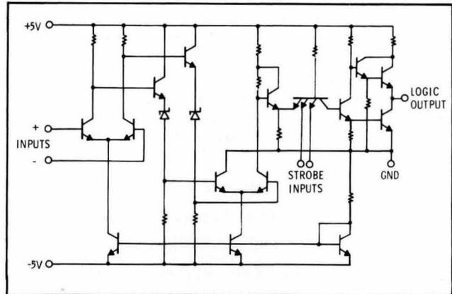
Figure 6 – 75 107 Line Receiver Circuit
