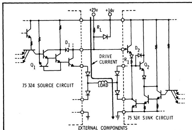
Figure 12 – 75 324 Source and Sink Circuit Connections in a Typical Application
