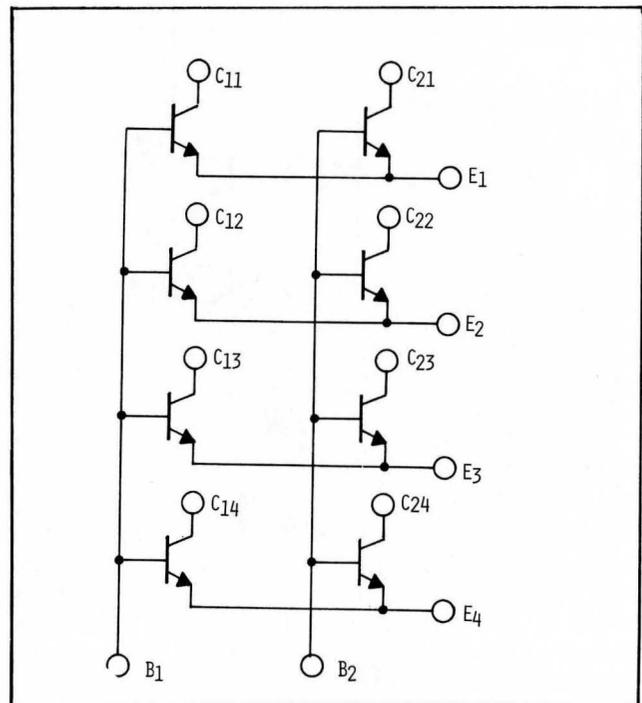
Figure 9 – 75 308 Transistor Array
