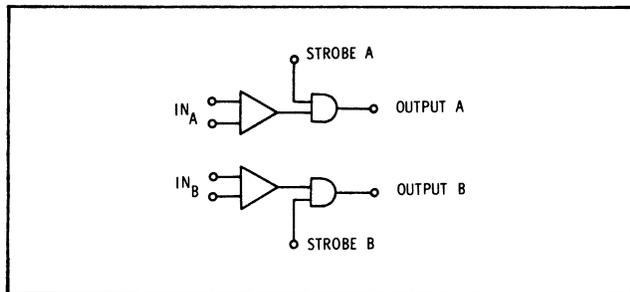
Figure 21 – Block Diagram of 7524
