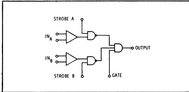
Figure 20 – Block Diagram of 7522
