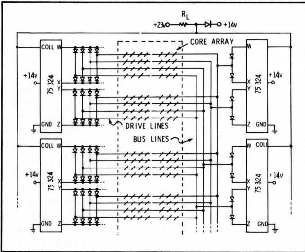
Figure 13 – Typical Application of 75 324's in a Memory Drive Line Selection Scheme
