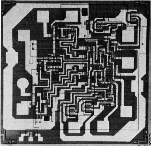
Figure 7 – Microphotograph of 75 107 Line Receiver Chip
