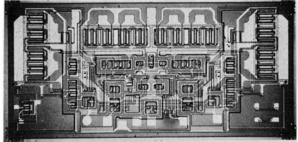
Figure 15 – Microphotograph of 75 324 Memory Driver Chip
