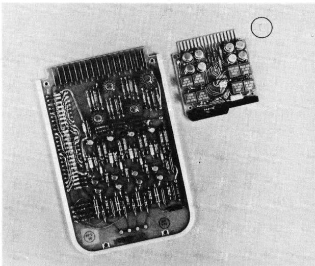
Figure 18 – Comparison of Integrated and Discrete Memory Drivers
