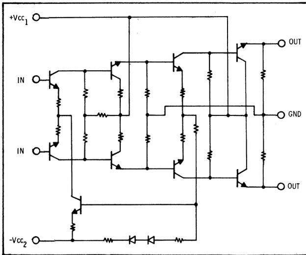
Figure 23 – Circuit Diagram of 5510
