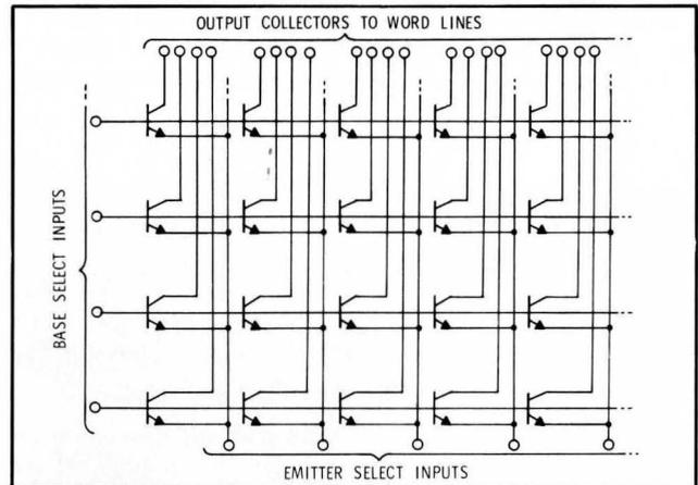
Figure 8 – Transistor Array for 2D Memory Applications
