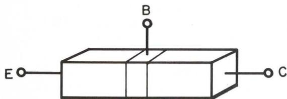
Fig. 1. Grown-Junction Transistor
