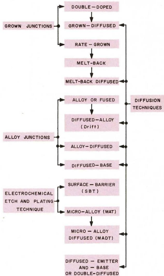
Fig. 4. Junction Transistor Classification Scheme
