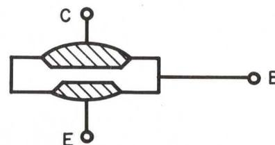
Fig. 2. Alloy-Junction Transistor
